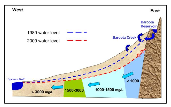
Figure 10. Schematic cross section of Baroota PWRA
