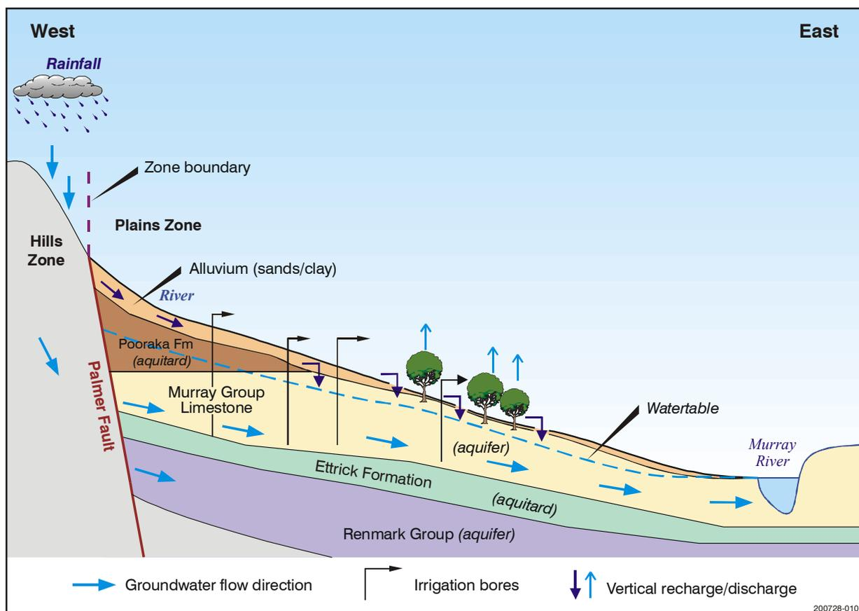
**Figure 8. Recharge and discharge mechanisms for the limestone aquifer**
