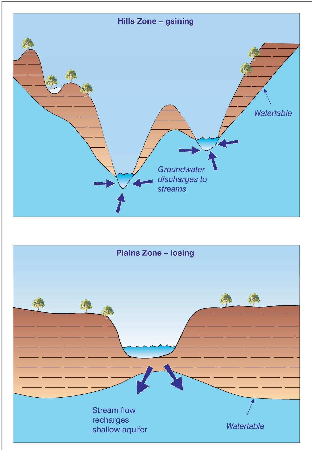
Figure 2. Groundwater - surface water interaction
