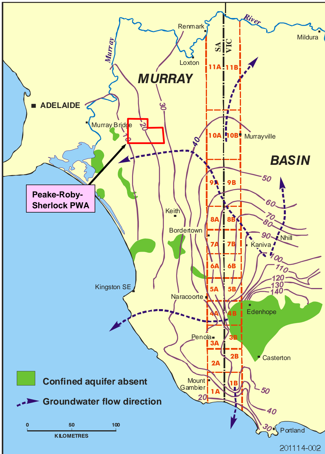
Figure 6. Regional potentiometric surface and flowpath for confined aquifer
