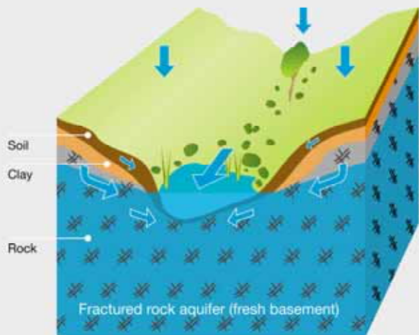
A cross-section of a wetland overlying a fractured rock aquifer.
