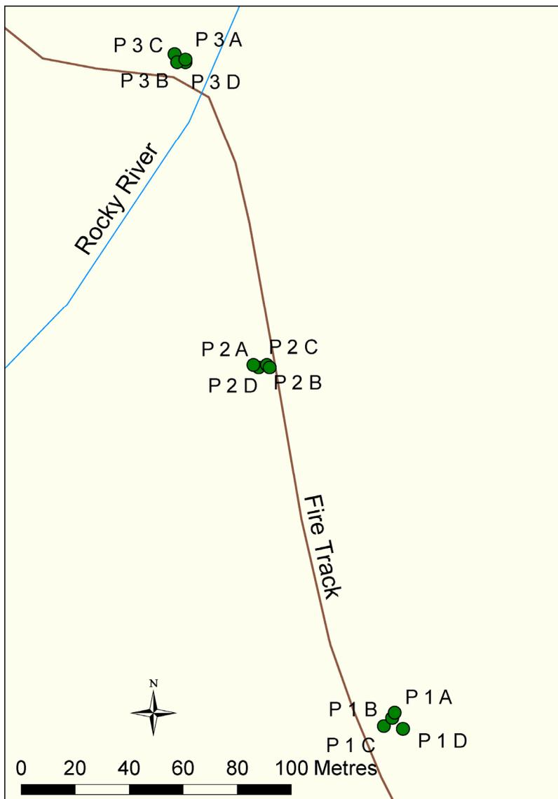
**Figure 5. Platypus site nested piezometer configuration**
