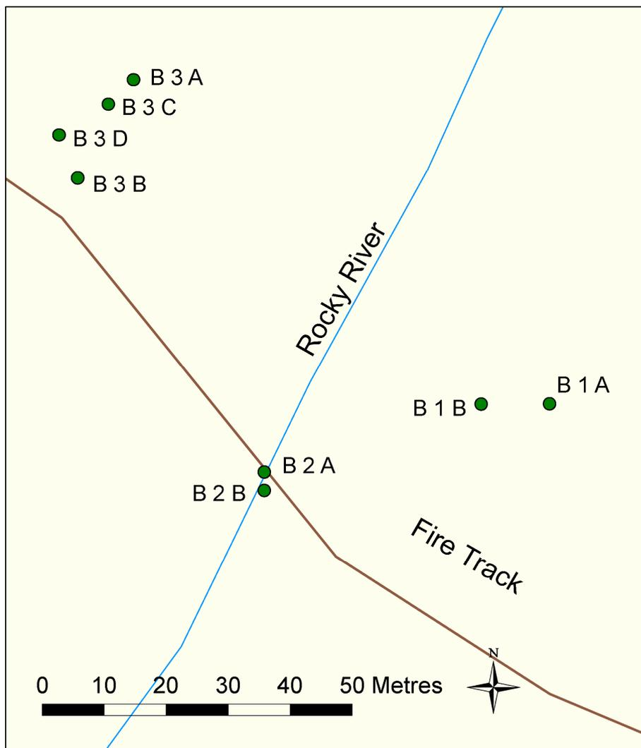
Figure 6. Bridge site nested piezometer configuration
