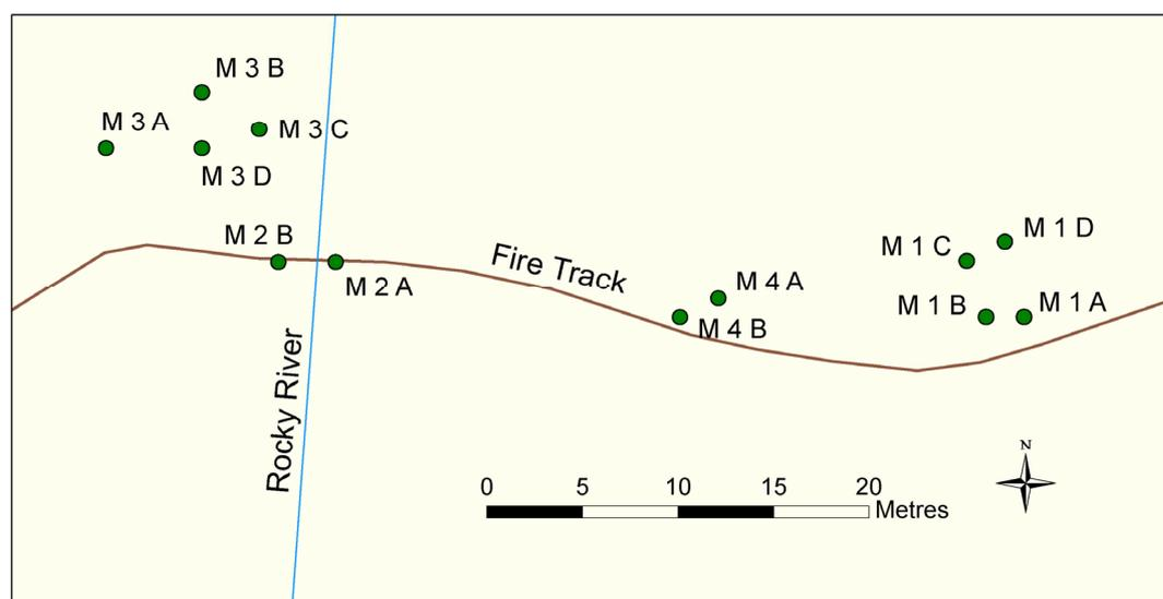
**Figure 4. Melrose site nested piezometer configuration**
