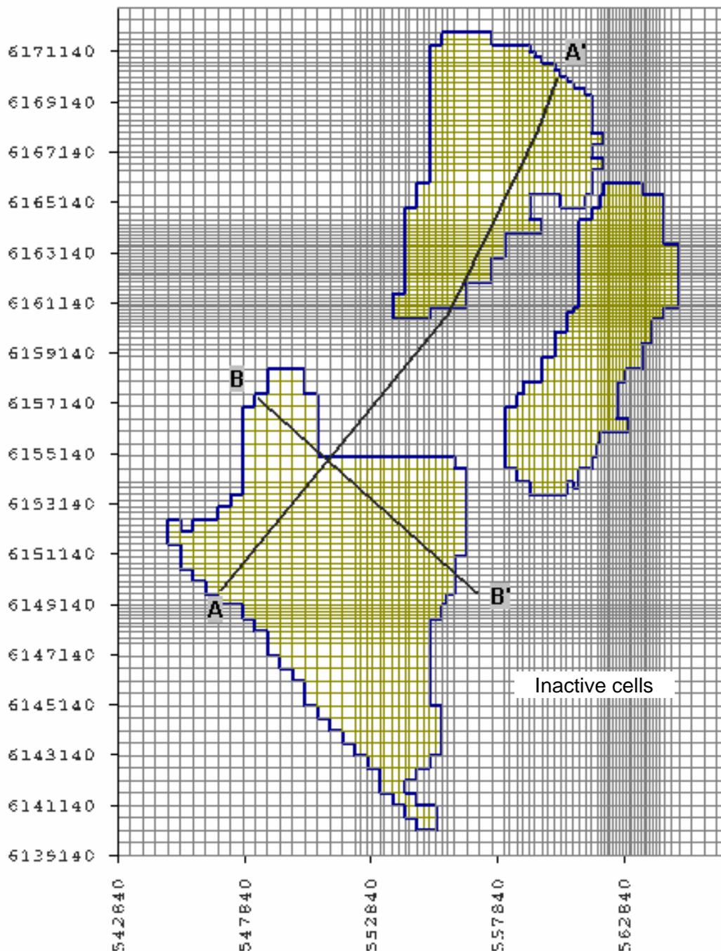
Figure 4. Model grid and domain of the Uley Basin from MODFLOW
