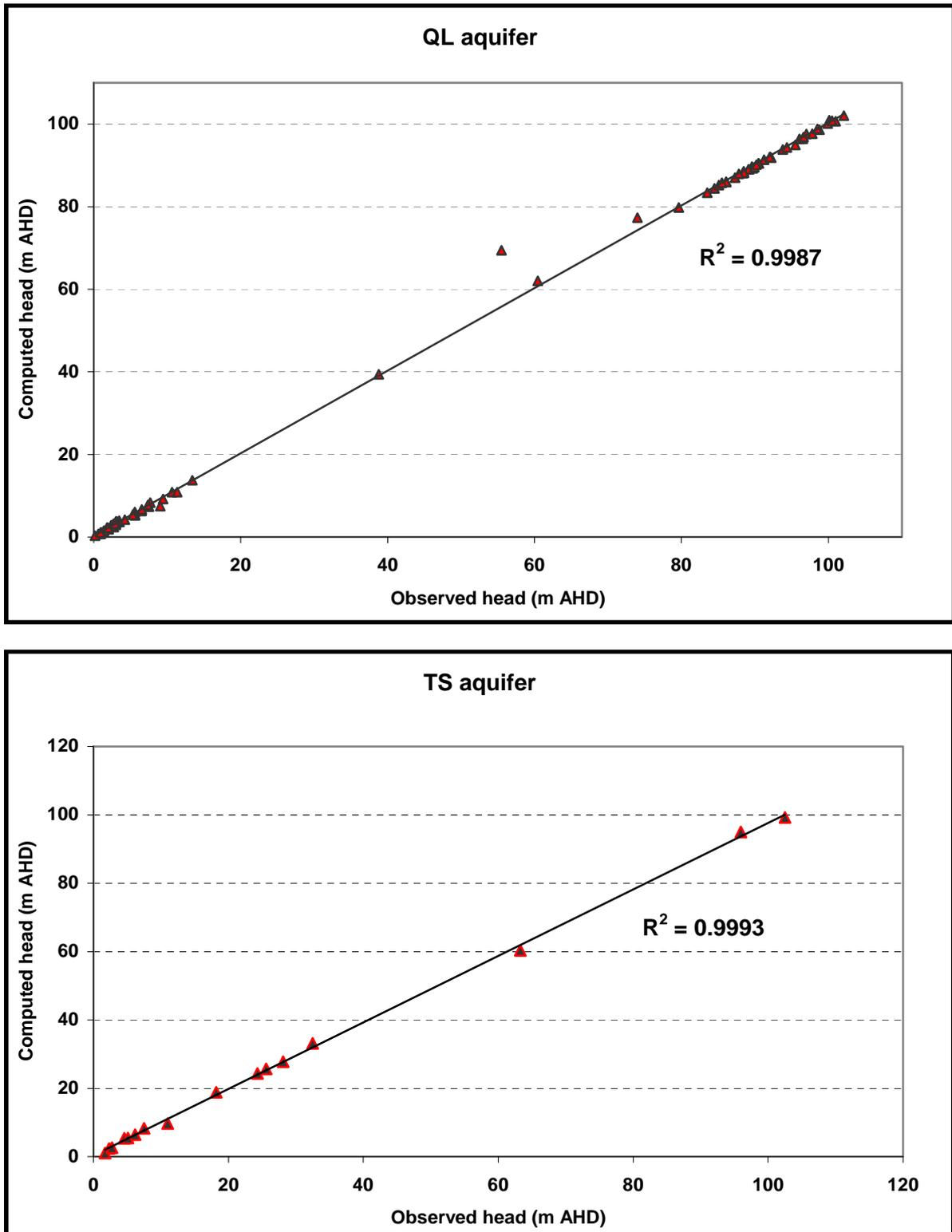
Figure 18. Steady state calibration results along 1:1 correlation line
