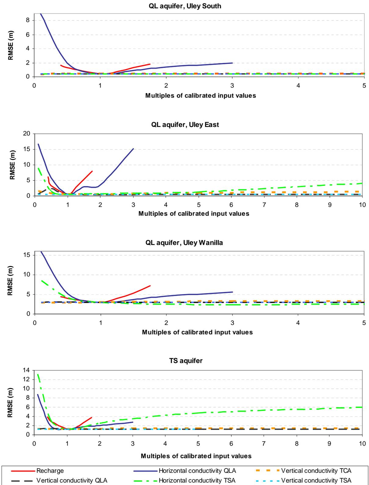
Figure 22. Steady state sensitivity analysis of Uley Basin model
