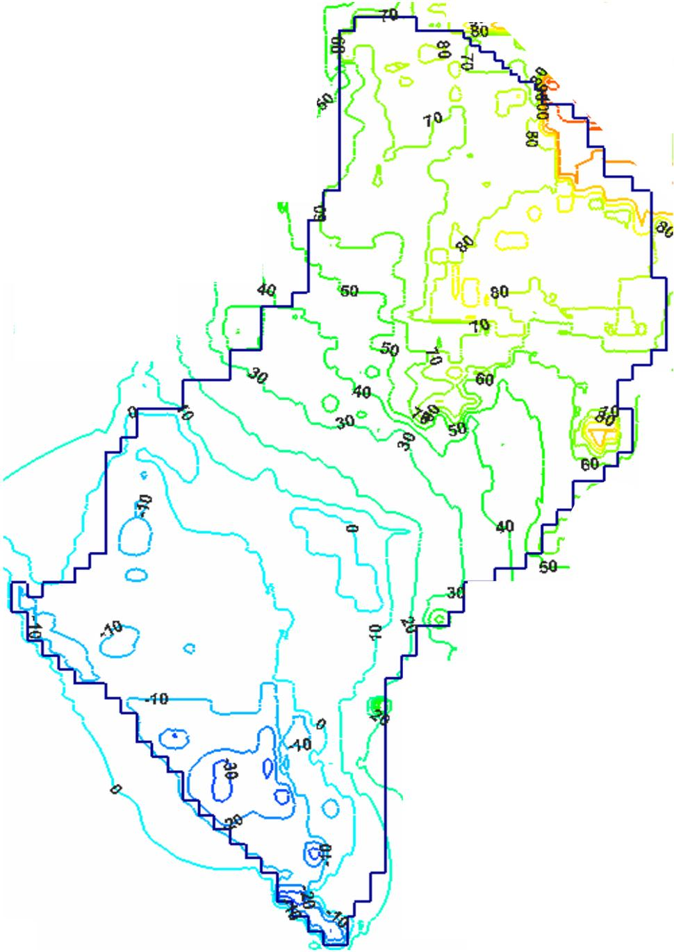
Figure 6. Bottom elevations (m AHD), QL aquifer, Uley Basin
