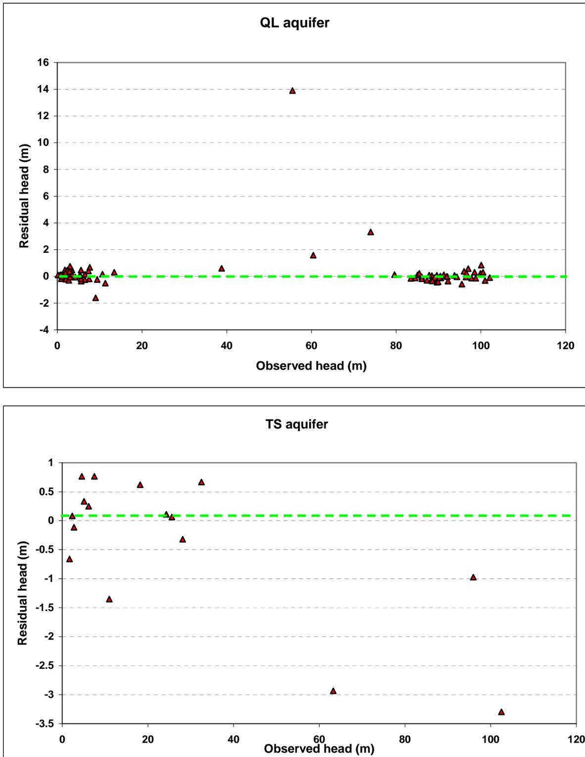
Figure 19. Steady state calibration results, residual versus observed heads
