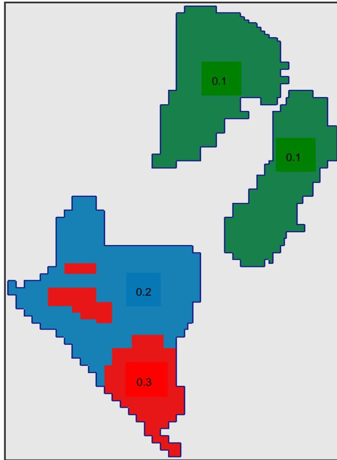
**Figure 20. Calibrated values of specific yield for the QL aquifer, Uley Basin**
