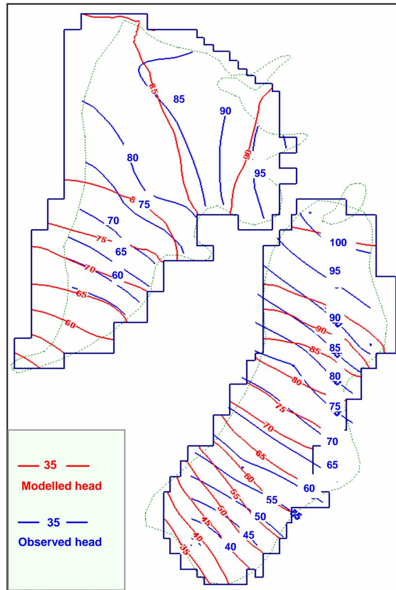
Figure 21. Observed and modelled potentiometric surface (m AHD) for QL aquifer, Uley Basin, May 2002
