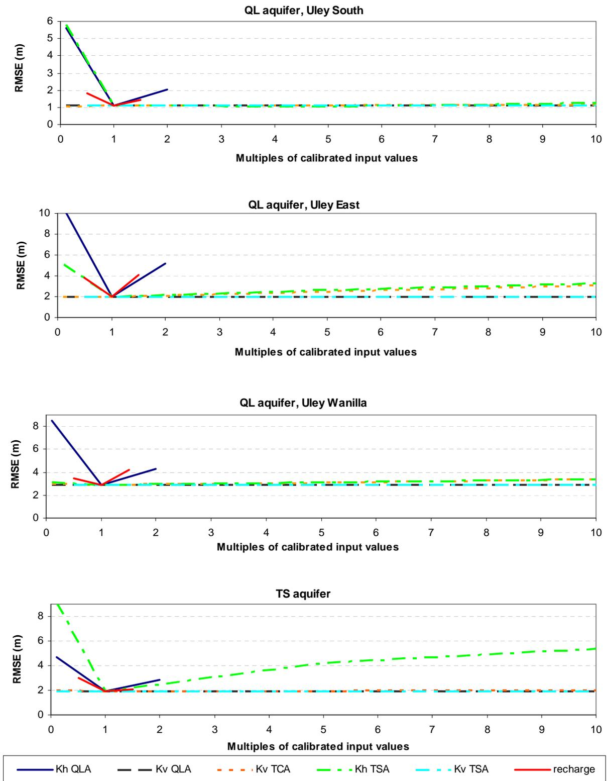
Figure 23. Transient state sensitivity analysis, Uley Basin model
