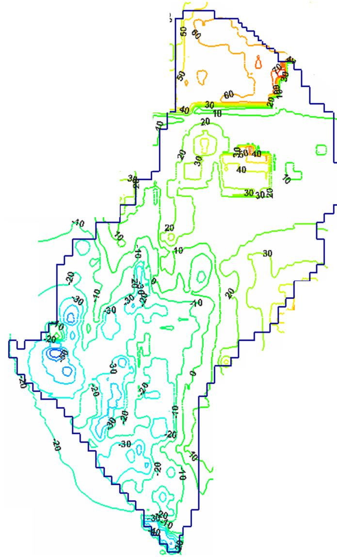
Figure 8. Bottom elevations (m AHD), TS aquifer, Uley Basin
