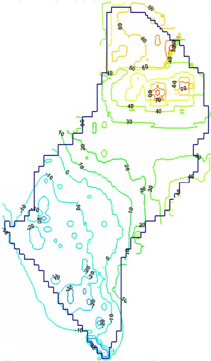
Figure 7. Bottom elevations (m AHD), TC aquitard, Uley Basin
