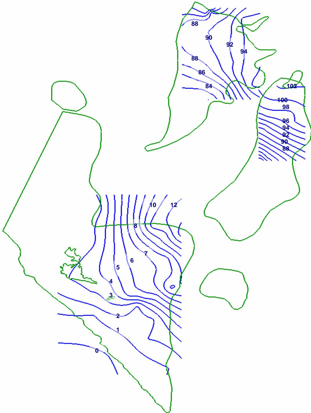
**Figure 3. Potentiometric surface map, September 1942 (Uley Wanilla and Uley East) and September 1963 (Uley South)**
