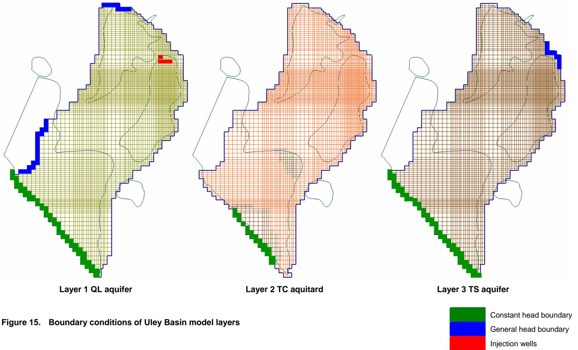
Figure 15. Boundary conditions of Uley Basin model layers
