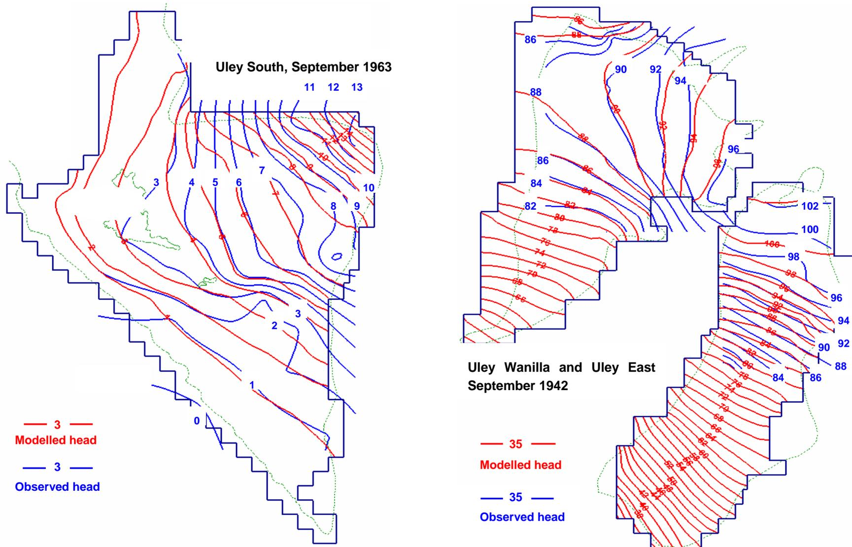
Figure 17. Calculated and observed potentiometric surface in the QL aquifer, Uley Basin
