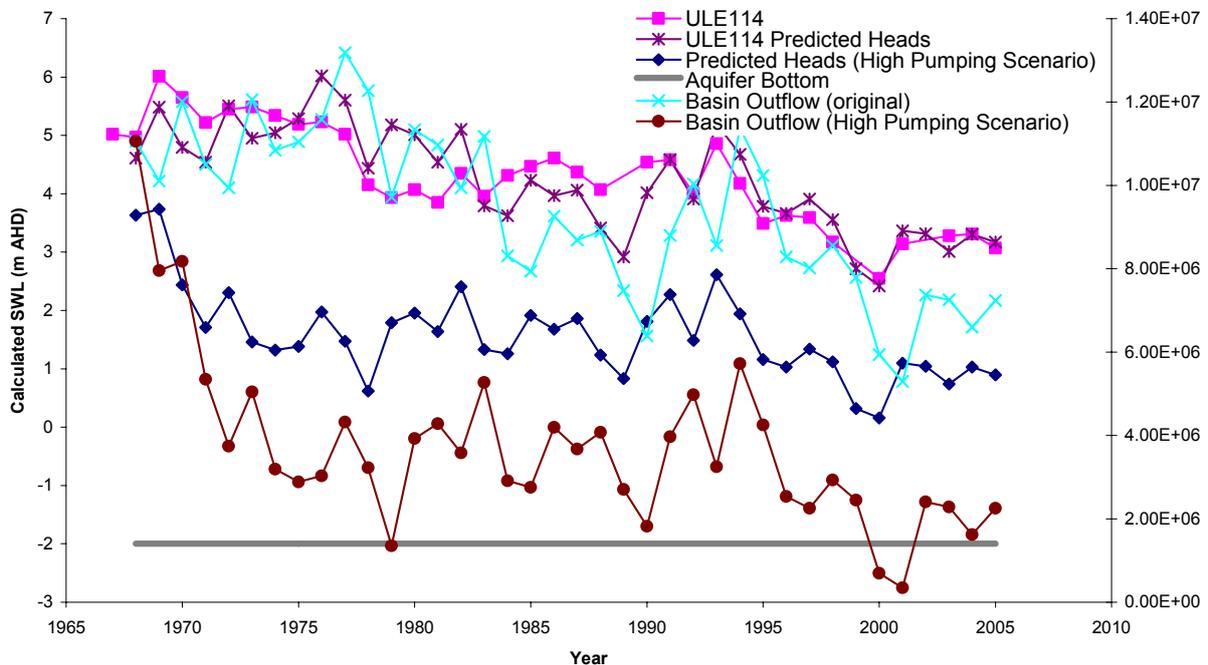
**Figure 6.3.** Observed and calculated hydraulic heads for ULE114, with predicted hydraulic heads under a higher groundwater extraction scenario (10 000 ML/y). Calculated variations in the basin outflow to the Southern Ocean are also shown for the current and increased extraction scenario.
