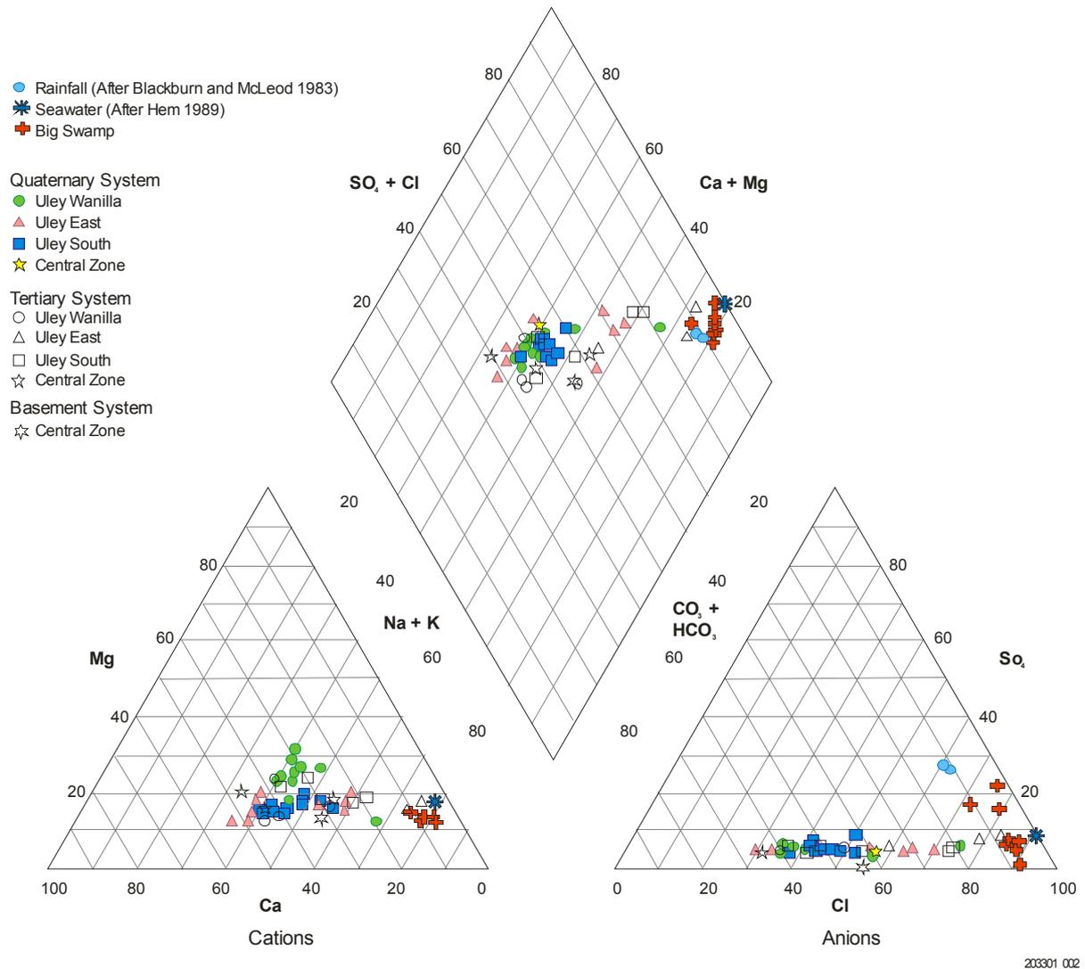
**Figure 4.8. Piper diagram displaying major ion compositions of Uley Basin groundwaters (from Evans, 1997).**
