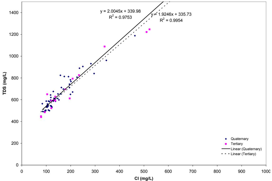
Figure 4.6. Plot of TDS/Cl vs Cl for all Quaternary and Tertiary groundwaters.
