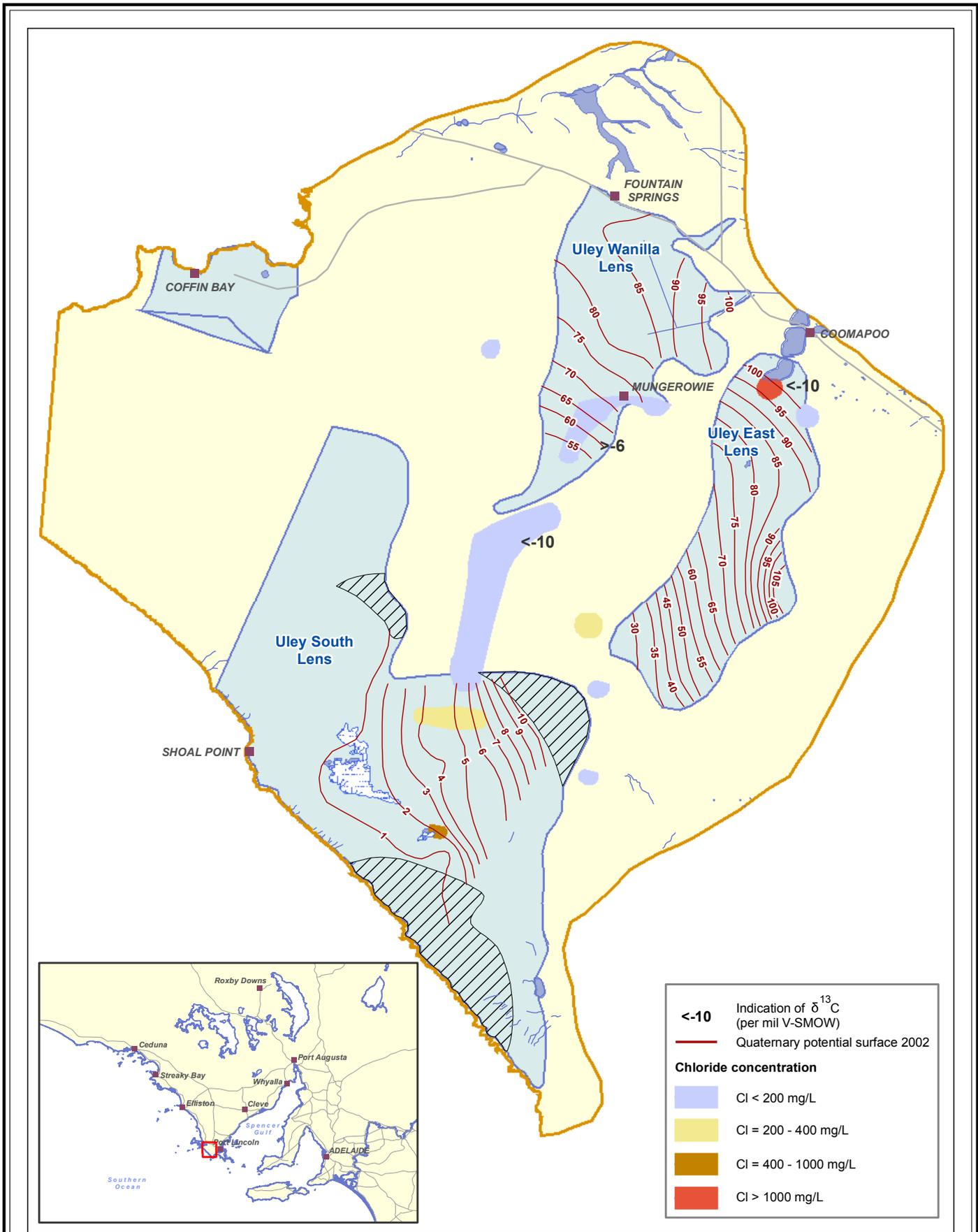
**Map 3. Groundwater chloride concentrations and  $\delta^{13}\text{C}$  in Tertiary sediments**
