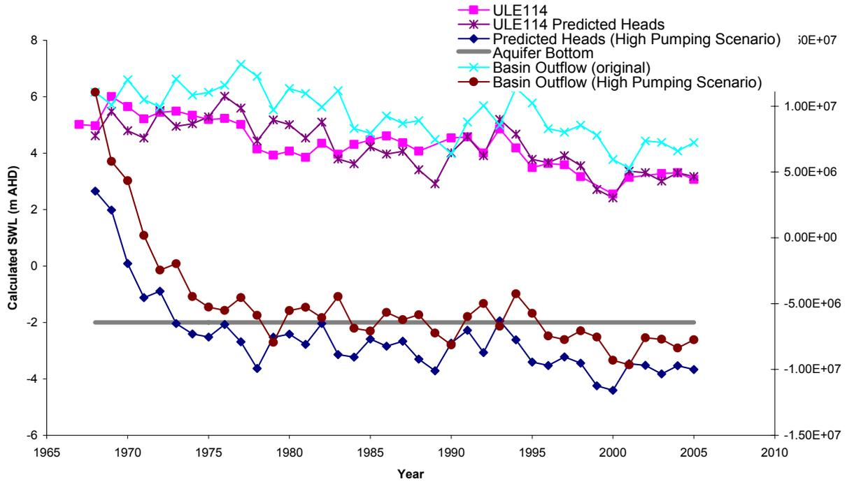
**Figure 6.4.** Predicted hydraulic heads under an extreme groundwater extraction scenario (20 000 ML/y), showing that groundwater levels drop below the base of the aquifer in this case.
