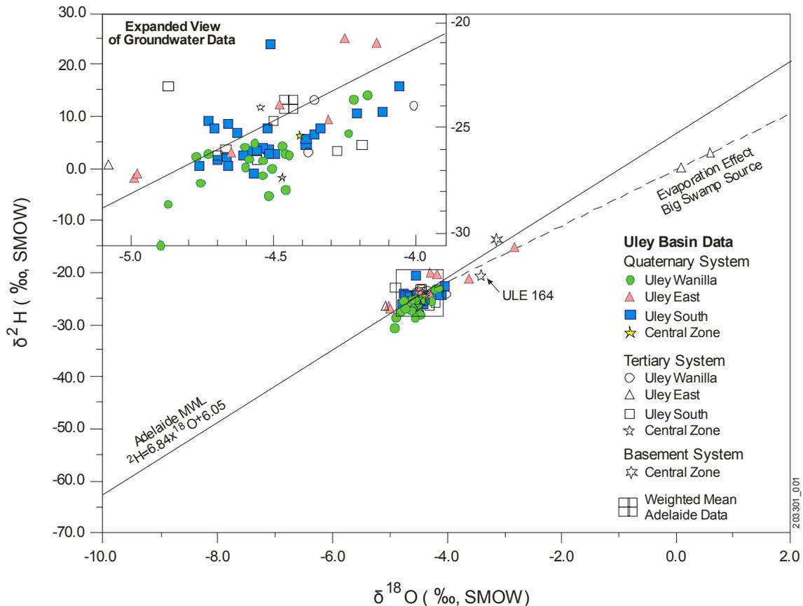
**Figure 4.7.  $\delta^2\text{H}$  vs  $\delta^{18}\text{O}$  for Uley Basin Groundwaters (from Evans, 1997).**
