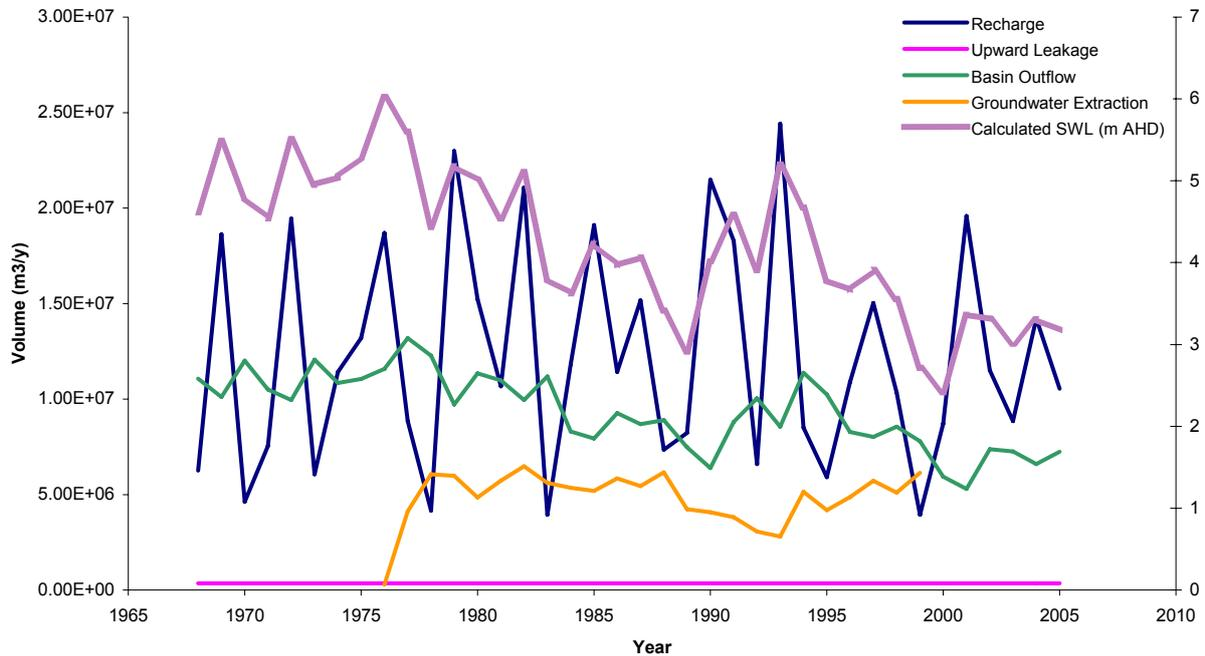
**Figure 6.2.** Variations in the magnitudes of the various water balance components for the Uley South lens, as calculated using the simple water balance model.
