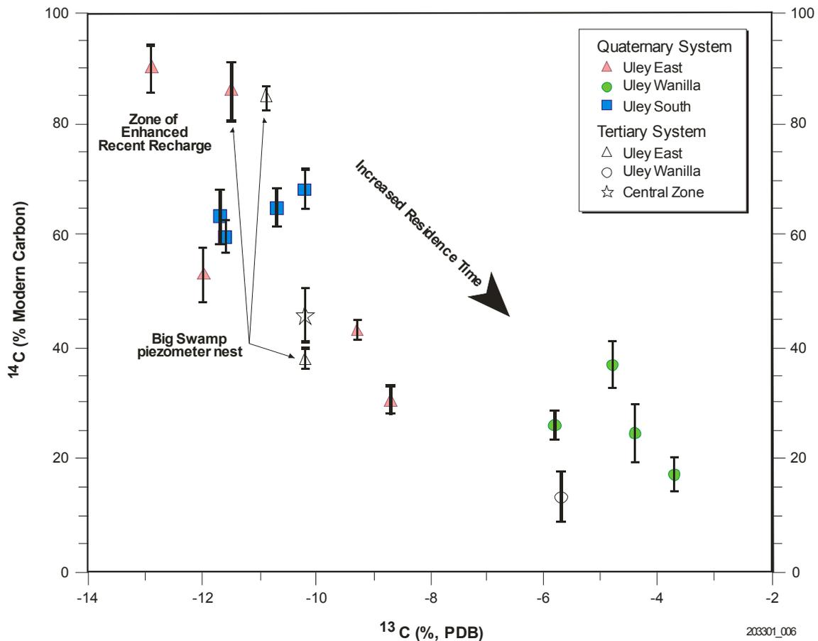
Figure 4.11.  $^{14}\text{C}$  vs  $\delta^{13}\text{C}$  for Uley Basin groundwaters (from Evans, 1997).
