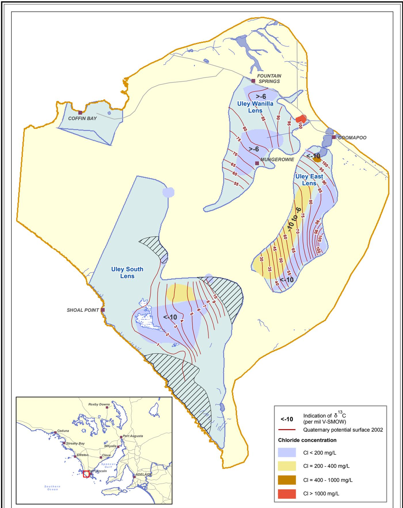
**Map 2. Groundwater chloride concentrations and  $\delta^{13}\text{C}$  in Quaternary groundwater sediments**
