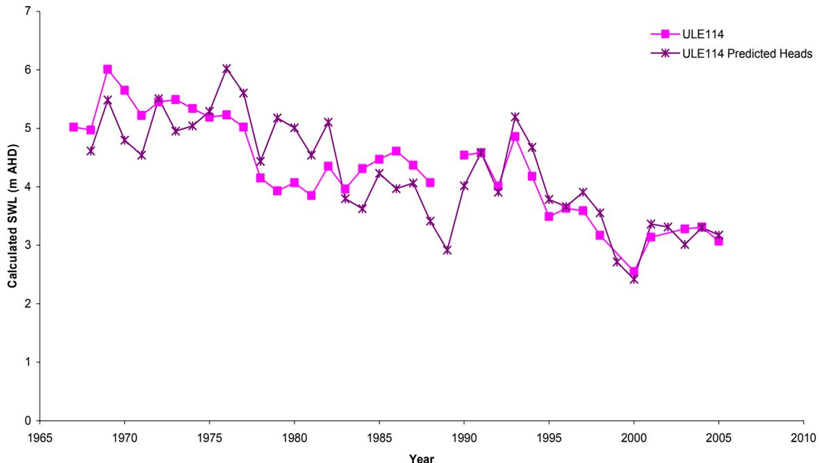
**Figure 6.1. Modelled hydraulic heads at observation well ULE114, calculated using the simple water balance model for the Uley South lens and compared with the observed groundwater hydrograph for ULE114.**
