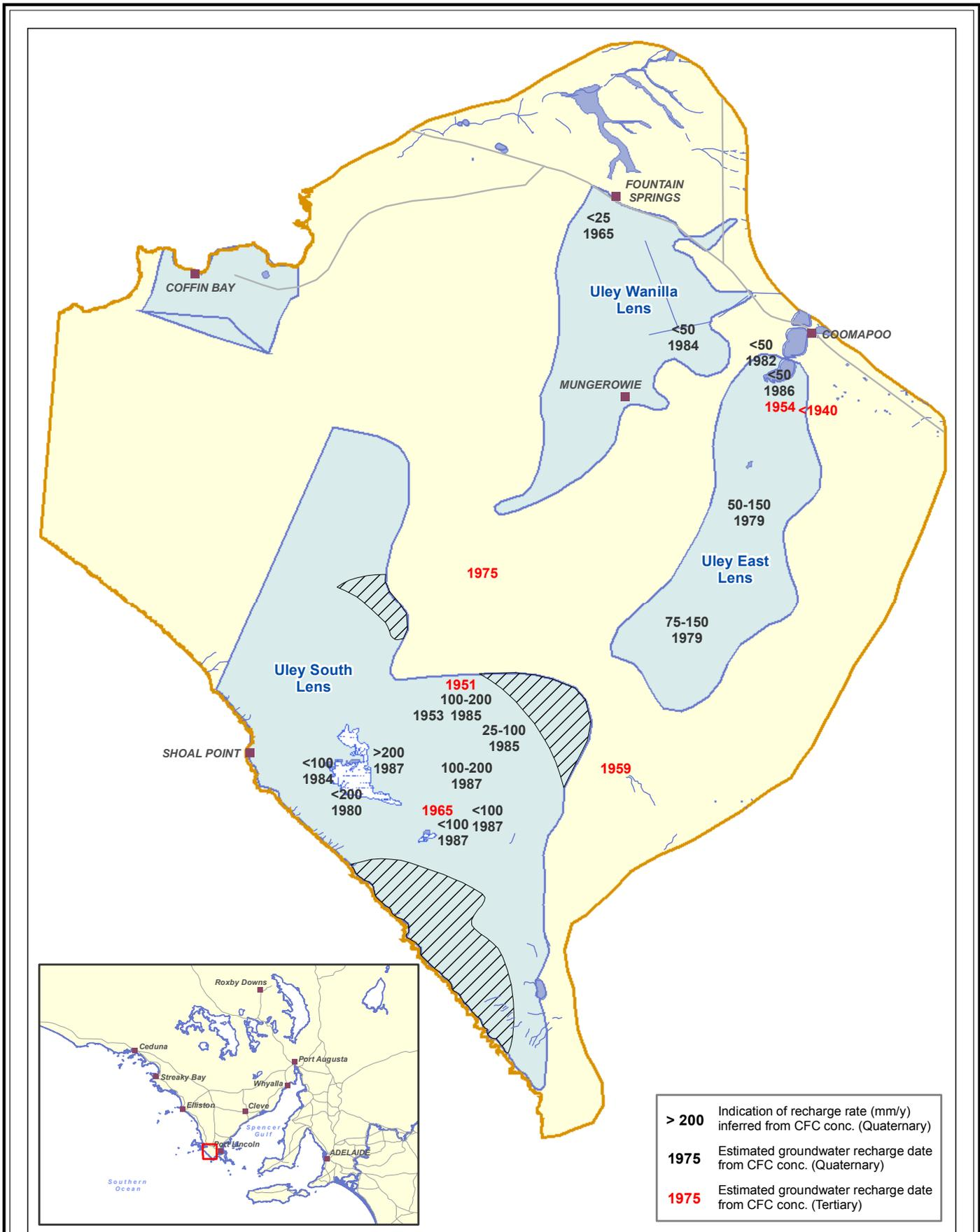
**Map 4. Groundwater recharge dates and recharge rates inferred from CFC data for the Quaternary lenses and Tertiary sediments**
