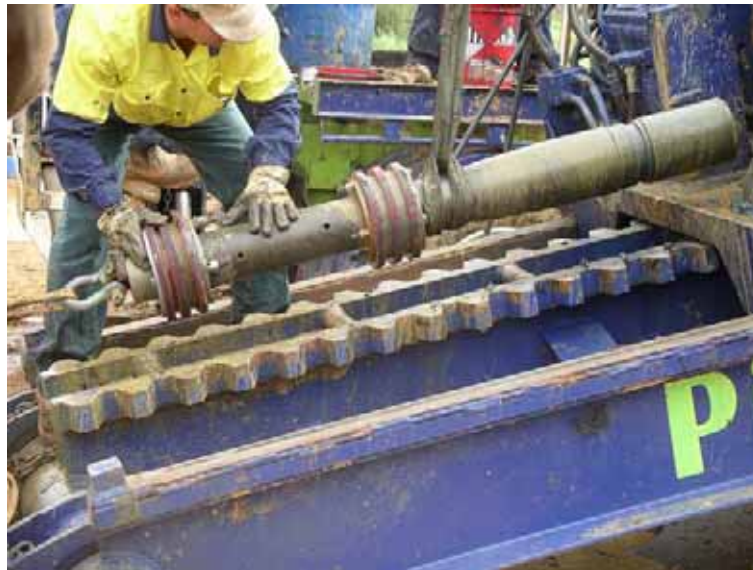
Figure 17. Development pig attached to drill string
