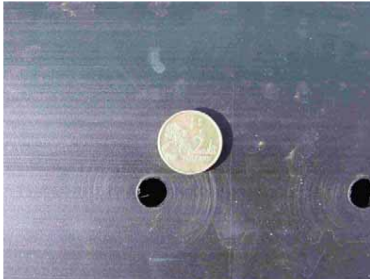
Figure 10. Outer product pipe drill holes
