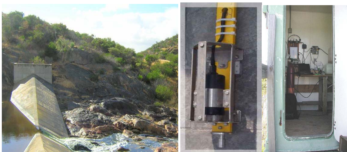
Figure 5. Photos (from left to right) show a stream gauging station on the Tod River (AW512500), an underwater sensor, and data logger.
