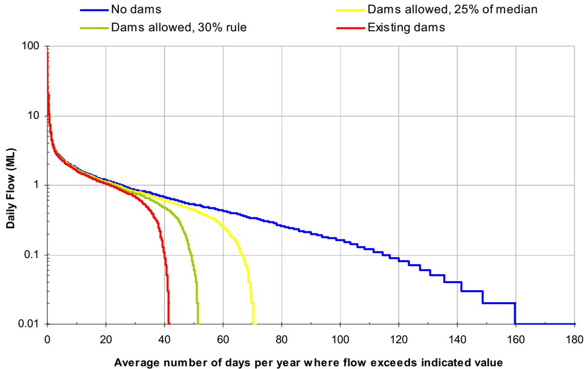
**Figure 26. Modelled daily flow duration curve for the study area showing comparison between the natural flow and that under three levels of development**
