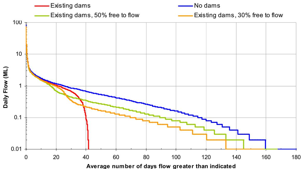
**Figure 29. Modelled daily flow duration curve for the study area showing comparison between the natural flow and that under three levels of development**
