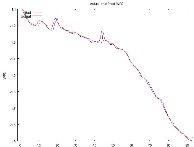
**Figure 16. Cochrane-Orcutt modelled (blue) and actual (red) groundwater level data for observation well WP2**
