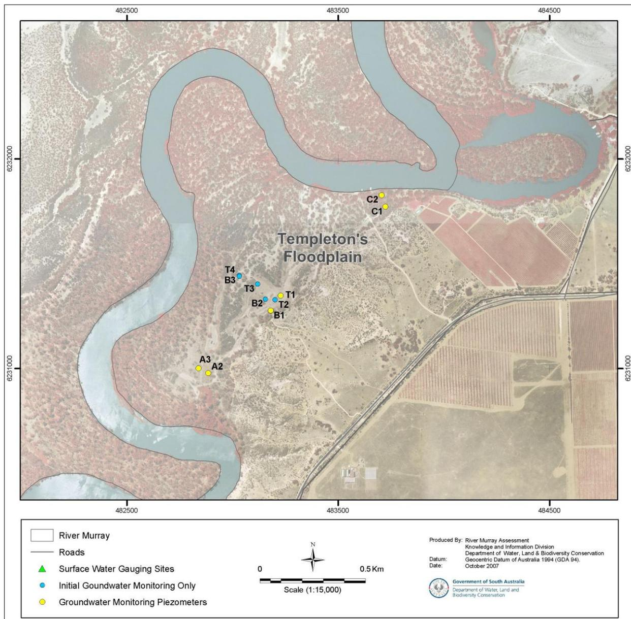
**Figure 8. Groundwater observation network on Templeton's Floodplain**
