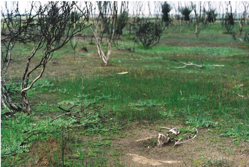
Figure 4. Piezometer tube in the Cummins-Wanilla Basin, melted by the bushfire (bottom of the photograph, taken in August 2005)
