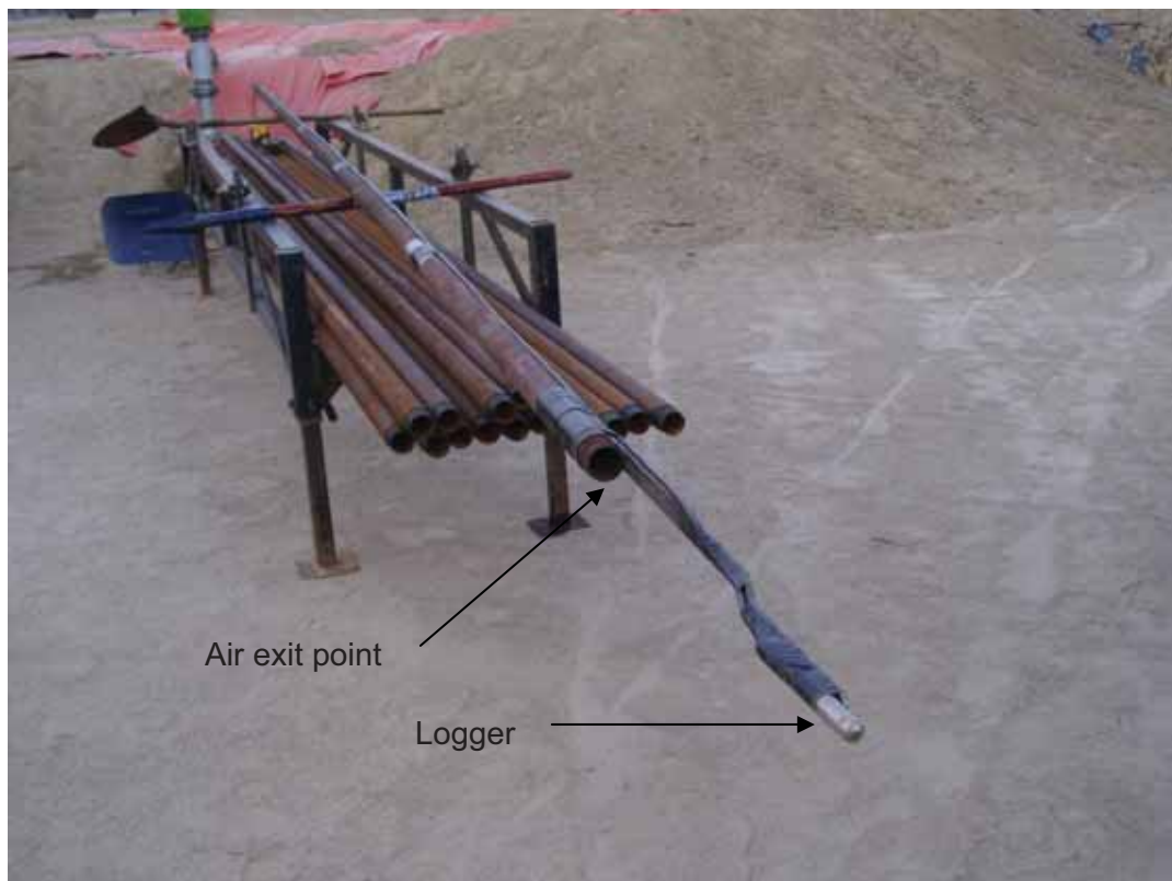
Figure 5. Downhole logger attached to the air-exit pipe
