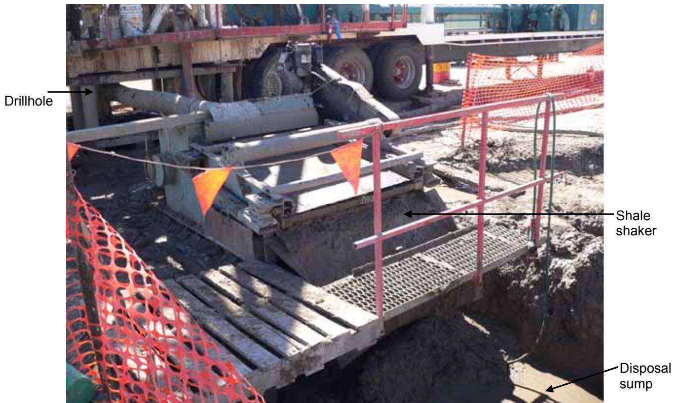
Figure 8. Shale Shaker used to separate the cuttings and drilling fluid for sample collection (photo courtesy of Tony Herbert)
