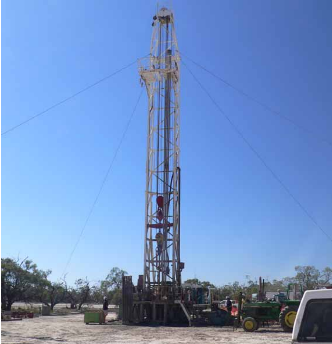
Figure 7. The GD 2500 Drill Rig used to construct WARINA 1
