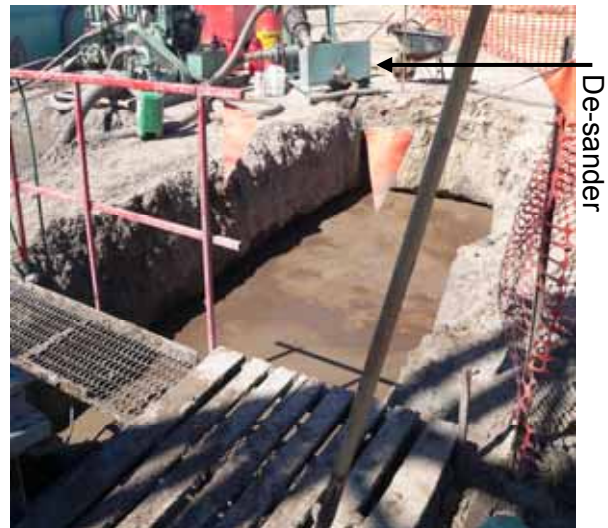
Figures 5, 6. Unlined holding dam and disposal sump (mud pit). The holding dam was used to store water during the mixing of drilling fluid; and to store water that was produced during development. The disposal sump collected unused sample cuttings as they passed over the shale shaker. The de-sander in the (top/middle) was used to separate the very fine material suspended in the drilling fluid that passed through the screen of the shale shaker (Photos courtesy Tony Herbert).
