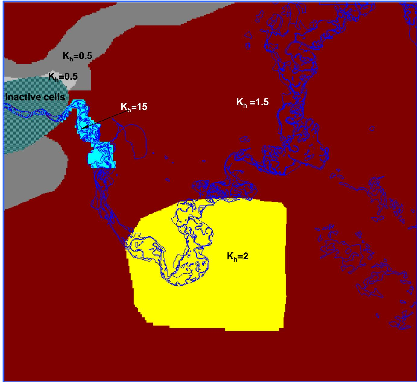
Figure 21: Model hydraulic conductivity zones and values (layer 4)
