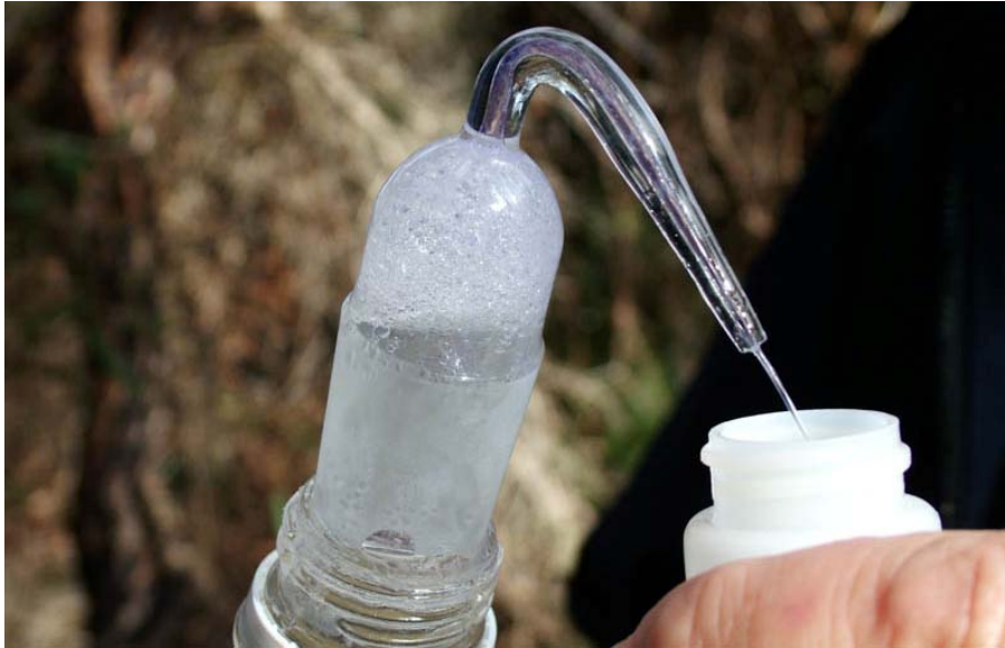
Figure 3.6 Decanting scintillant containing dissolved Rn from sample
