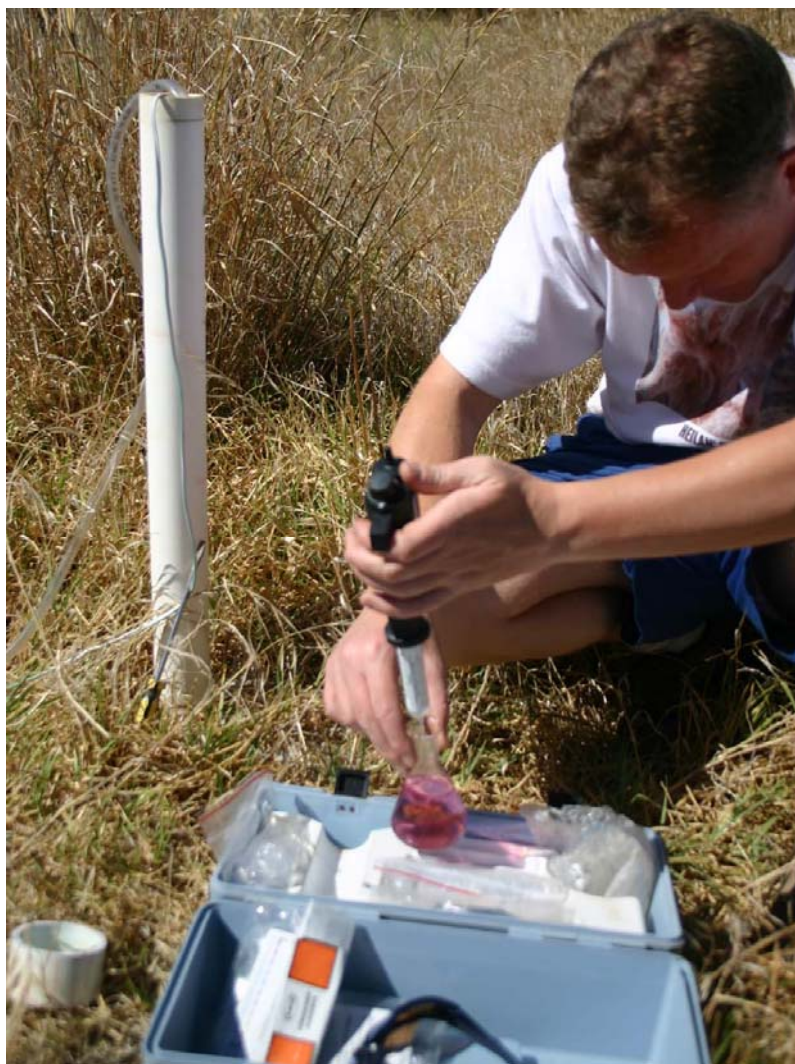
Figure 3.4 Measuring alkalinity in the field by acid titration
