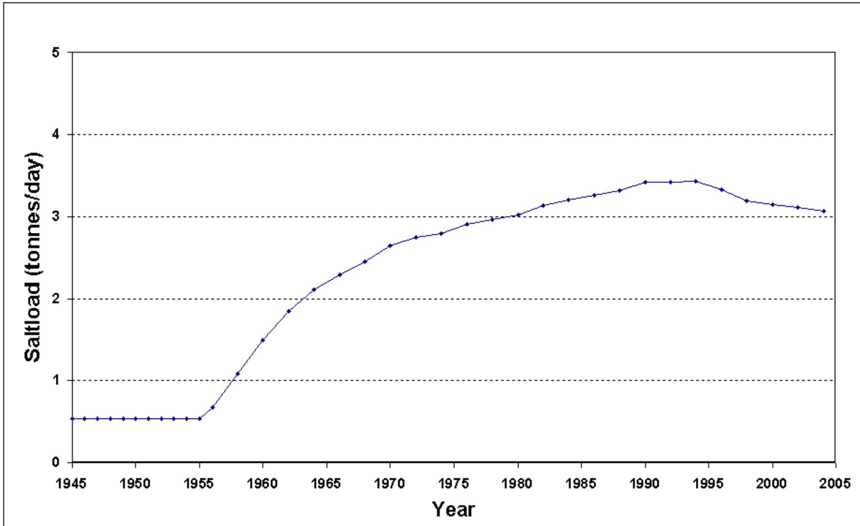
**Appendix A-2-5b** Graph of predicted total upward salt load (tonnes/day) entering the River Murray in Scenario-2 (Loxton Area)
