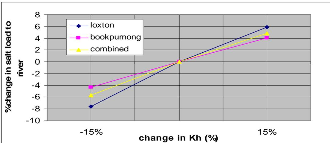
Figure 66: Model sensitivity to hydraulic conductivity of Loxton Sands
