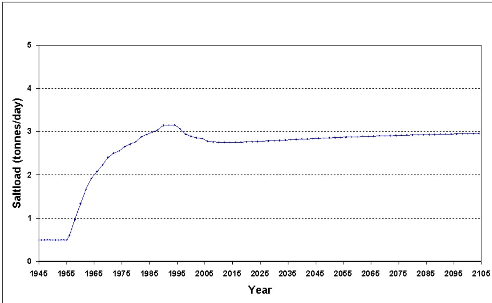
**Appendix A-4-5c** Graph of predicted total upward salt load (tonnes/day) entering the River Murray in Scenario-4 (Loxton Area)
