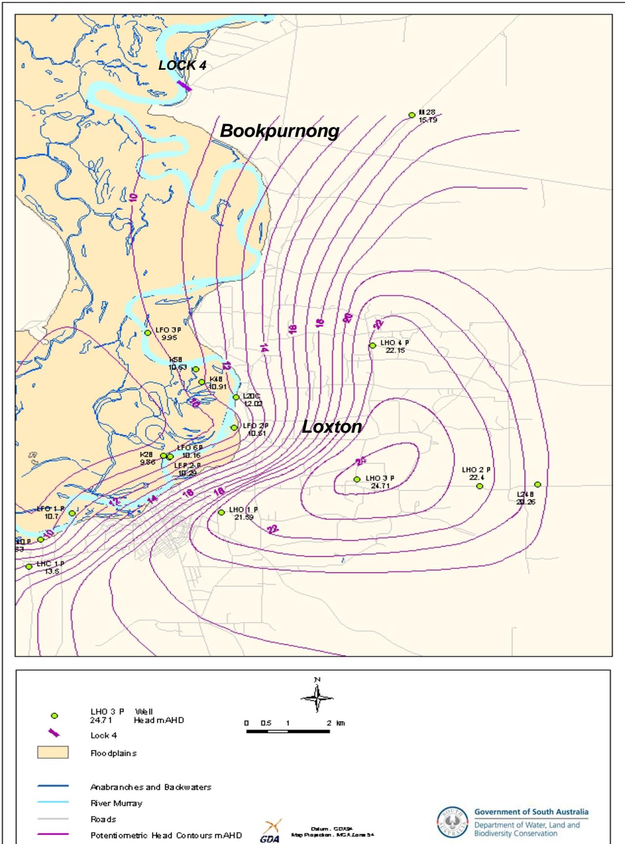
Figure 7: Pata Formation potentiometric surface, May 2004
