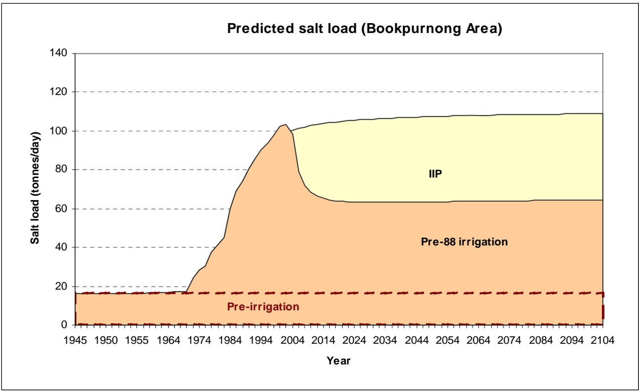
**Figure 71:** Predicted salt loads entering the River Murray resulting from pre 1988 irrigation development
