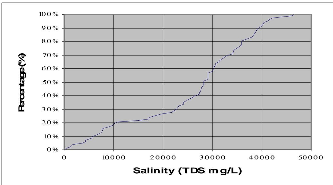
**Figure 70: Percentile distribution of all relevant groundwater salinity values (84 samples)**
