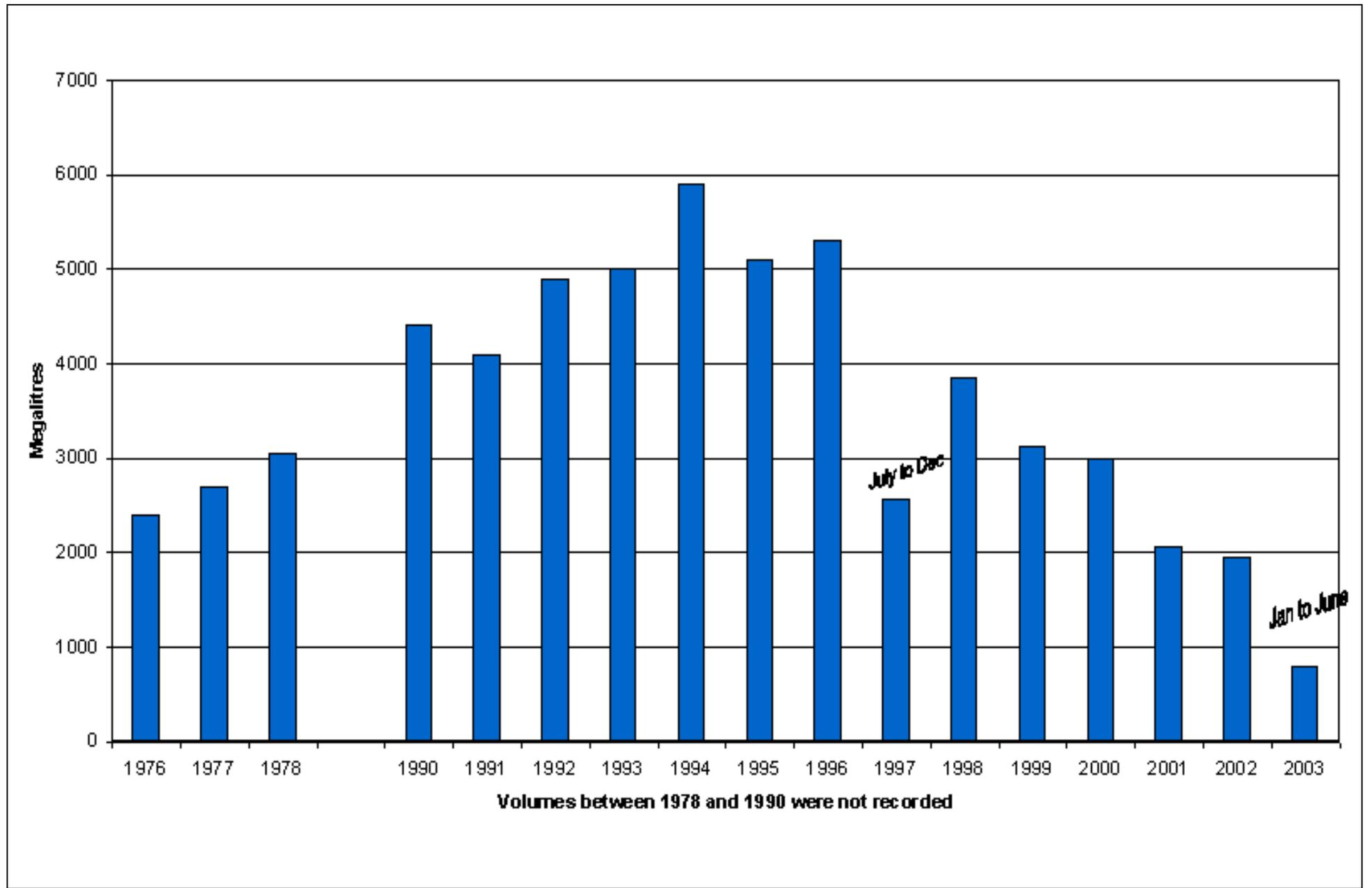
Figure 61: Annual pumped discharge from Loxton CDS
