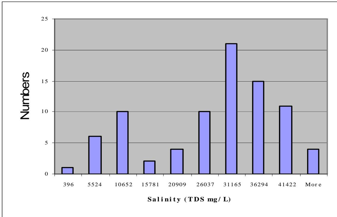
**Figure 69: Distribution histogram of relevant groundwater salinity values (84 samples)**
