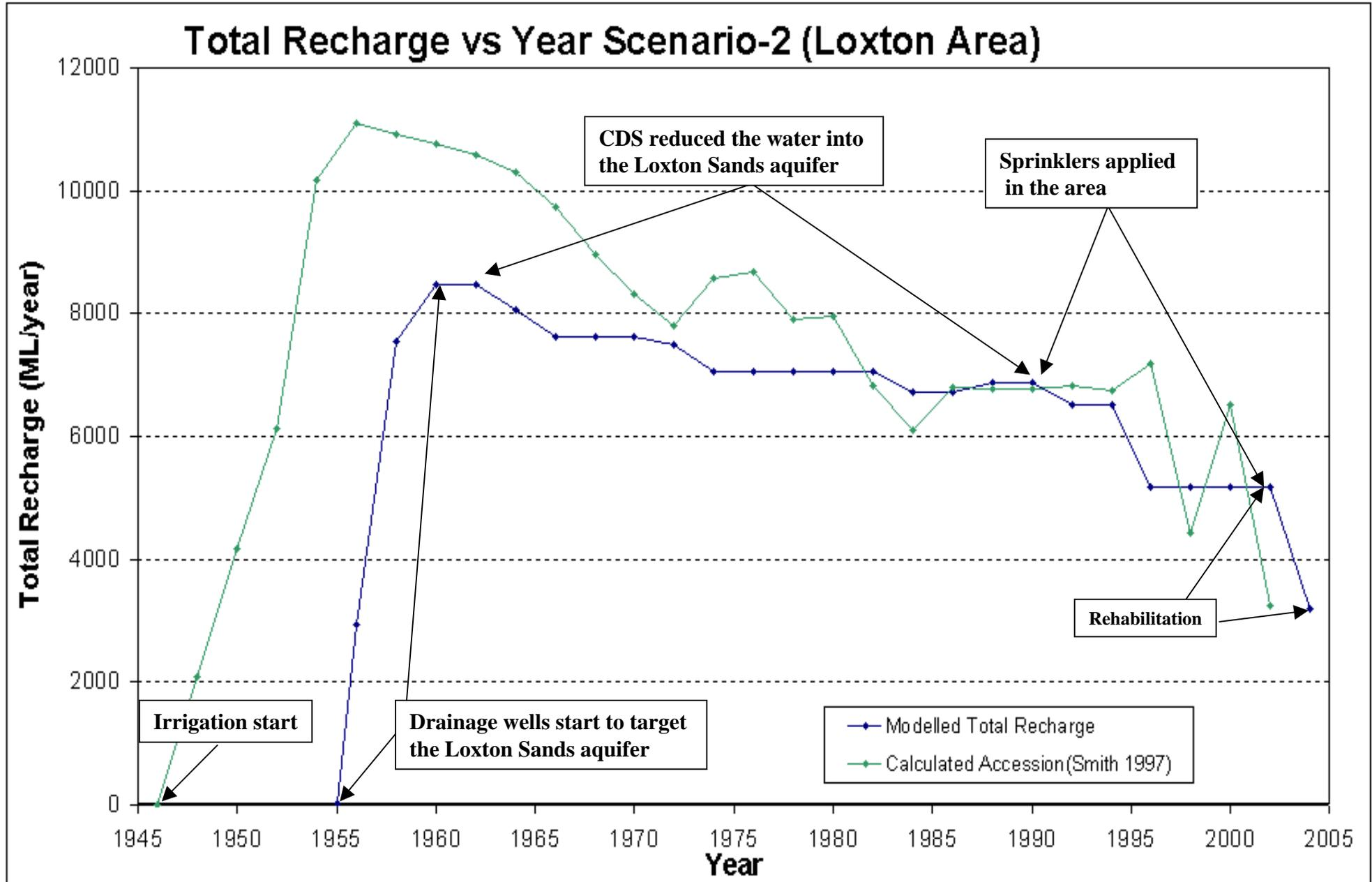
**Figure 56:** Modelled recharge volume to the Loxton Sands vs accession (Loxton area)
