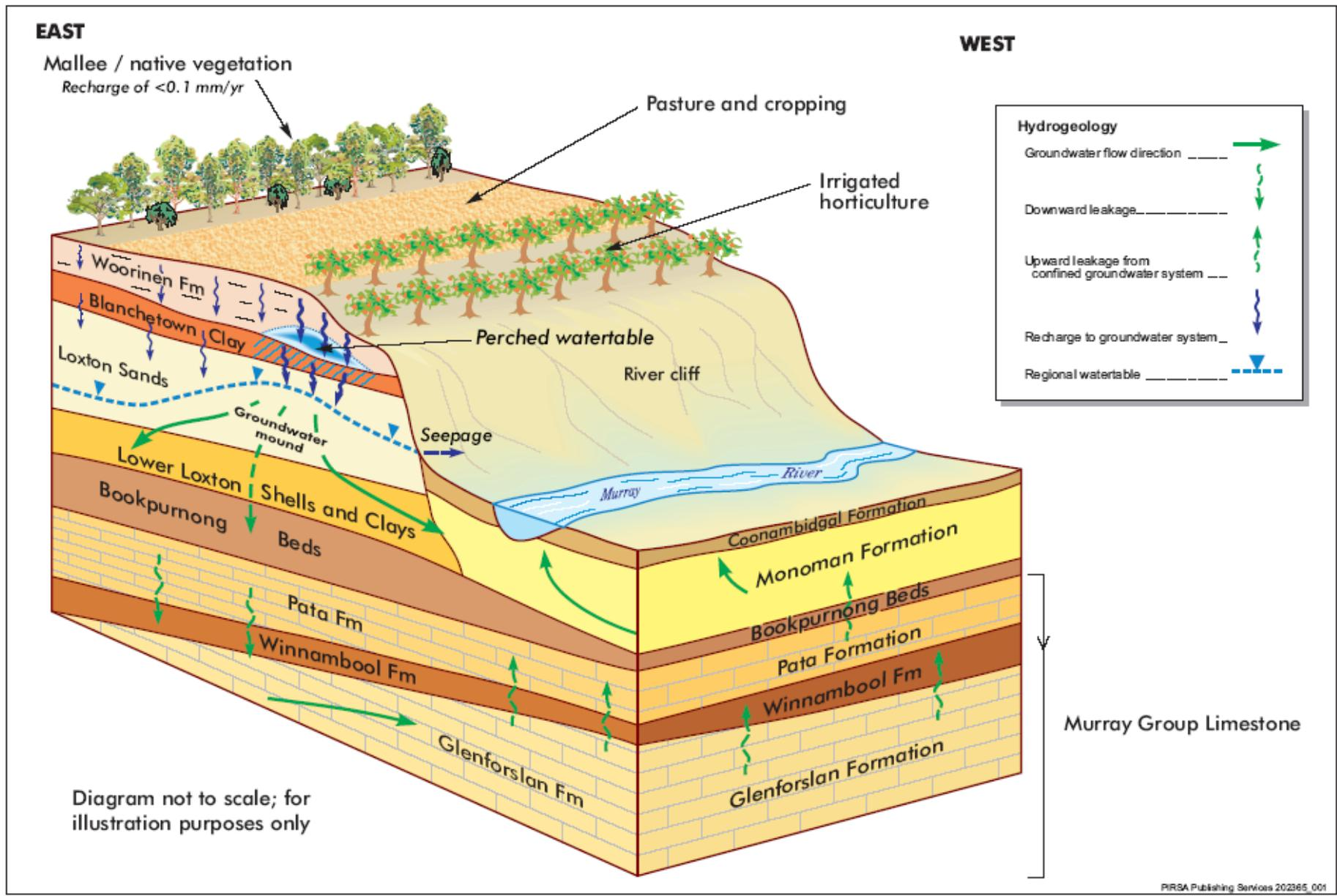
**Figure 5:** Elementary conceptual hydrogeological model
