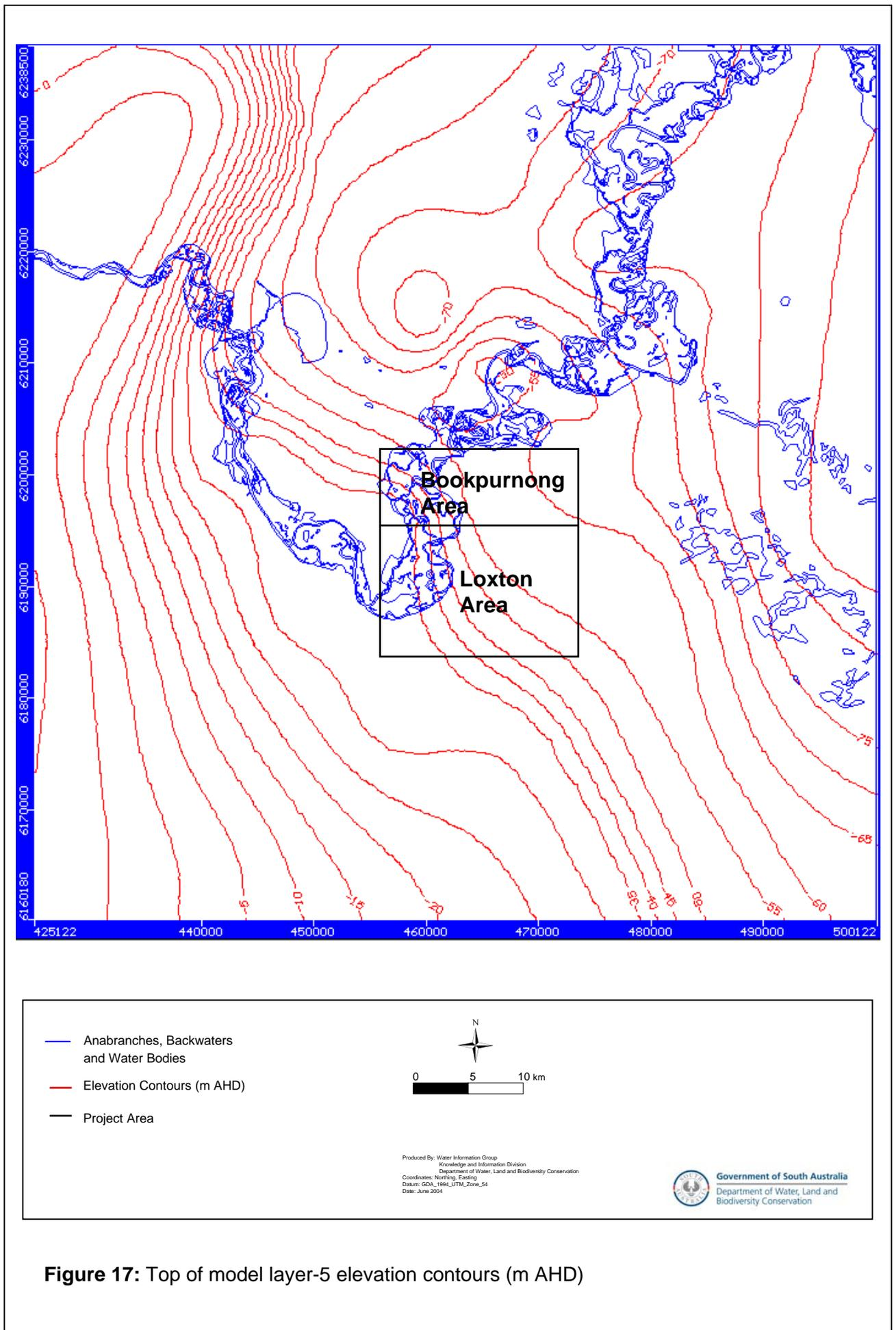
**Figure 17: Top of model layer-5 elevation contours (m AHD)**
