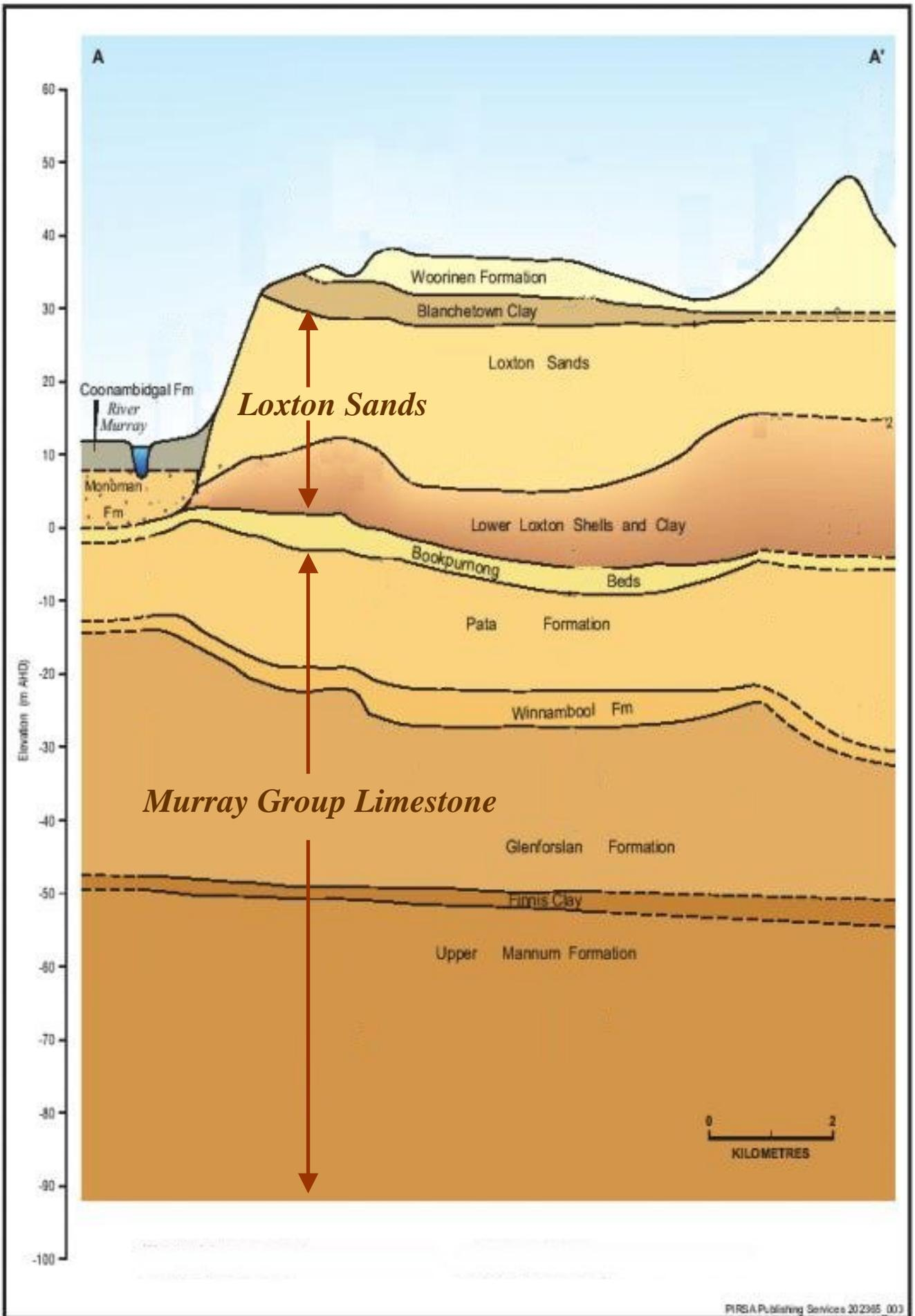
Figure 3: Hydrogeological cross-section (See Figure 1 for line of section)
