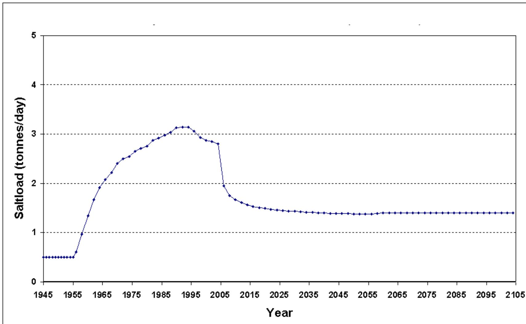
**Appendix A-7-5c** Graph of predicted total upward salt load (tonnes/day) entering the River Murray in Scenario-7 (Loxton Area)
