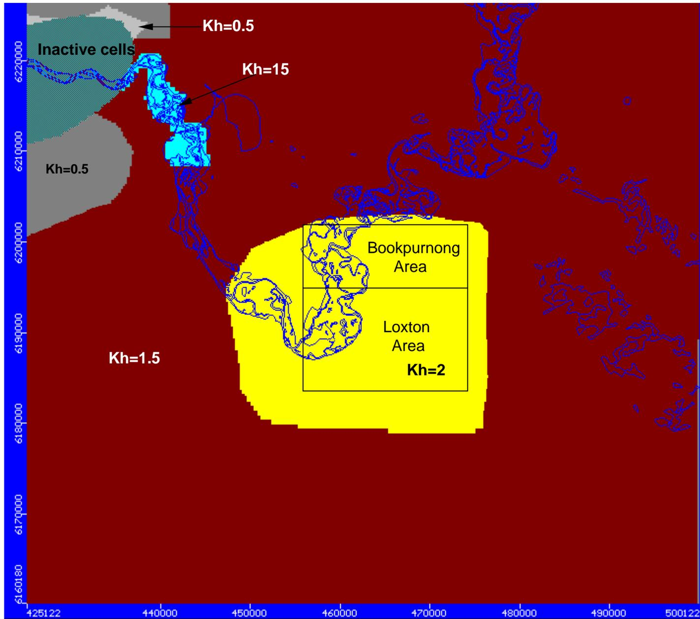
**Figure 22:** Model hydraulic conductivity zones and values (Layer-4)
