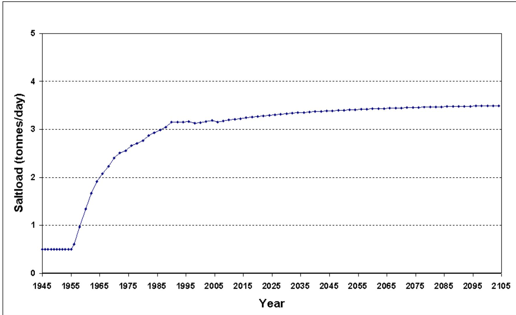
**Appendix A-3-5c** Graph of predicted total upward salt load (tonnes/day) entering the River Murray in Scenario-3 (Loxton Area)
