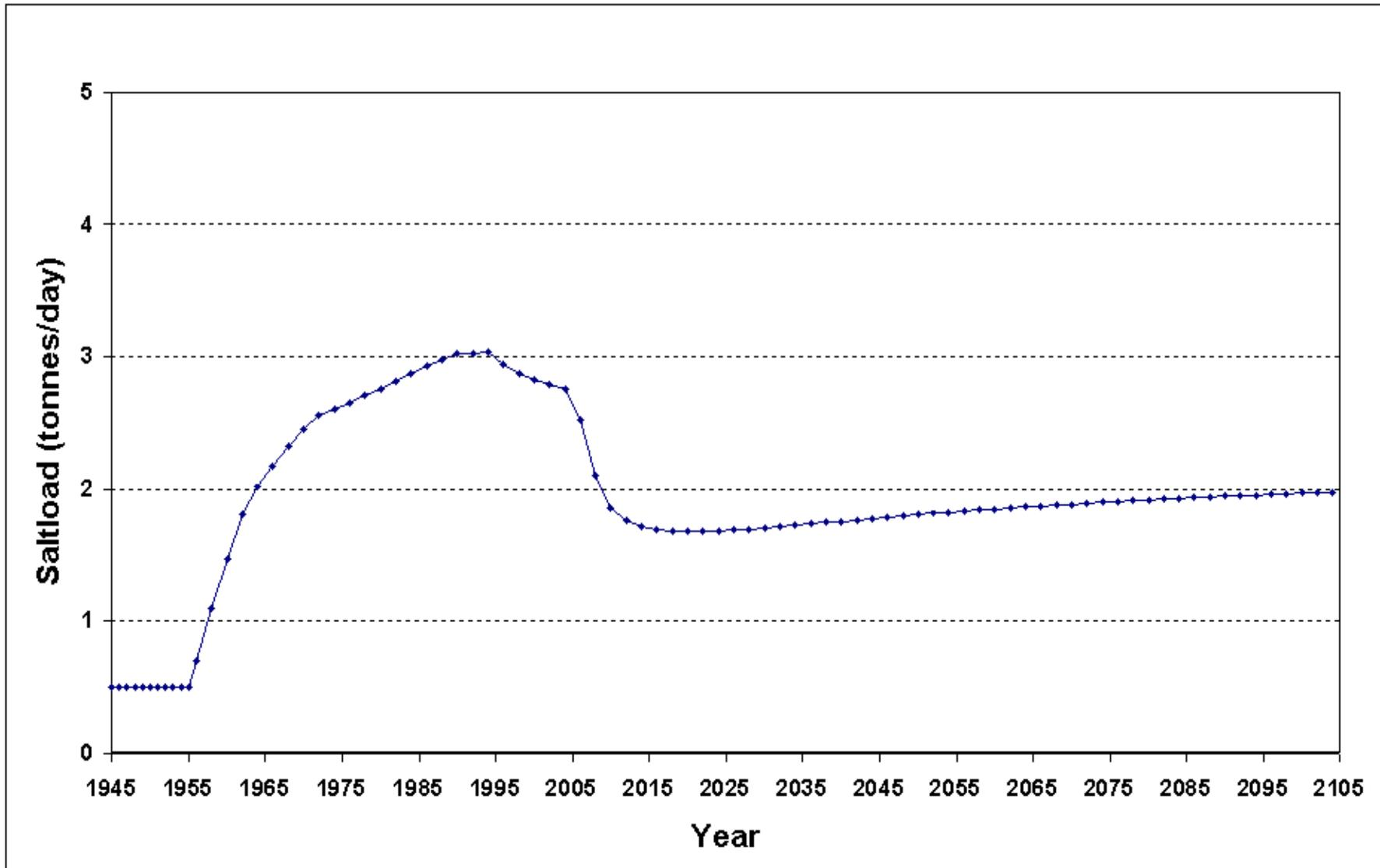
**Appendix A-8-5c** Graph of predicted total upward salt load (tonnes/day) entering the River Murray in Scenario-8 (Loxton Area)
