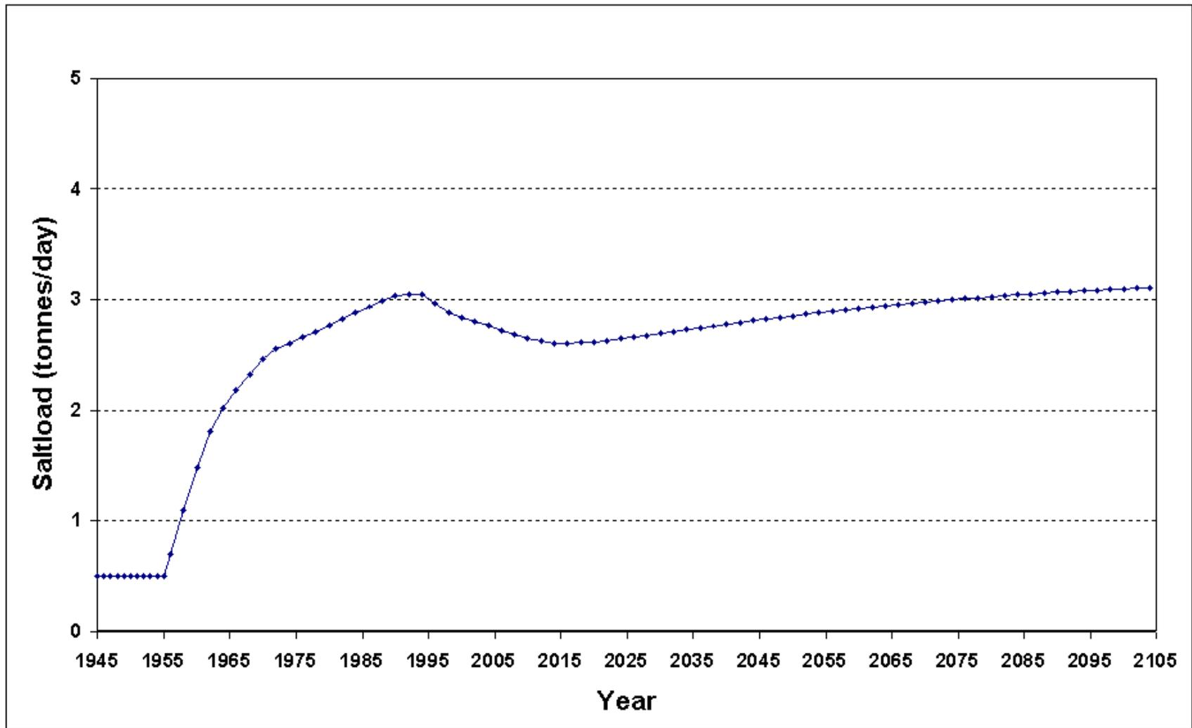
**Appendix A-6-5c** Graph of predicted total upward salt load (tonnes/day) entering the River Murray in Scenario-6 (Loxton Area)
