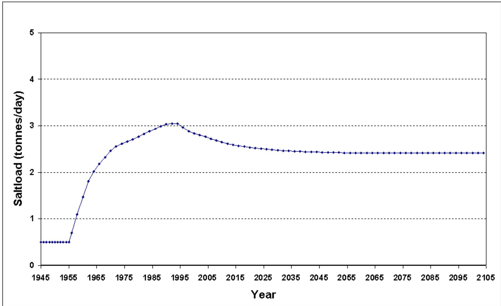
**Appendix A-5-5c** Graph of predicted total upward salt load (tonnes/day) entering the River Murray in Scenario-5 (Loxton Area)
