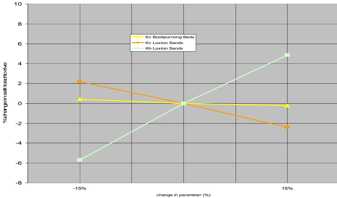
Figure 67: Model sensitivity to changes in hydraulic parameters of Loxton Sands
