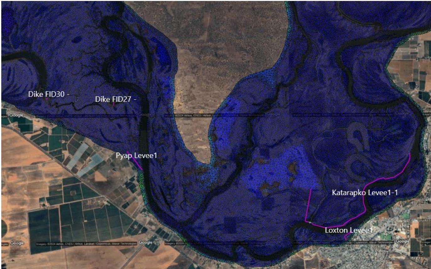
**Figure 6.9.** Features including tracks, roads and levee banks included in the model between Pyap and Loxton (shown in pink with IDs as named in the model).
