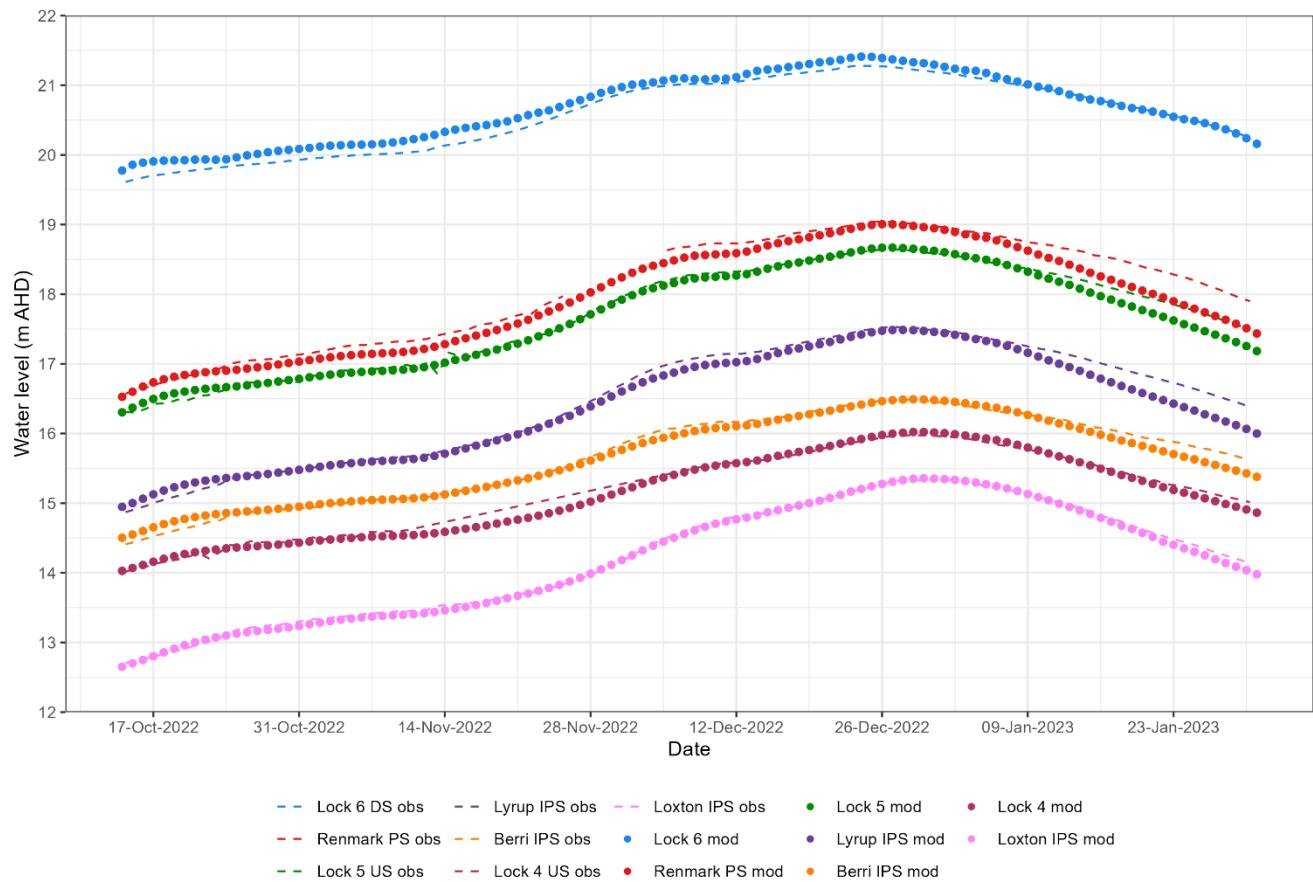
**Figure 6.18. Water level comparisons modelled ('mod') to observed ('obs') for 2022–23 flood event peak at active monitoring stations between Lock 3 and Lock 6.**
