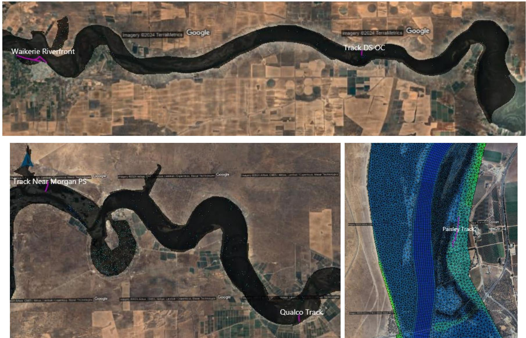
**Figure 6.1. Features including tracks, roads and levee banks included in the model between Morgan and Lock 3 (shown in pink with IDs as named in the model).**
