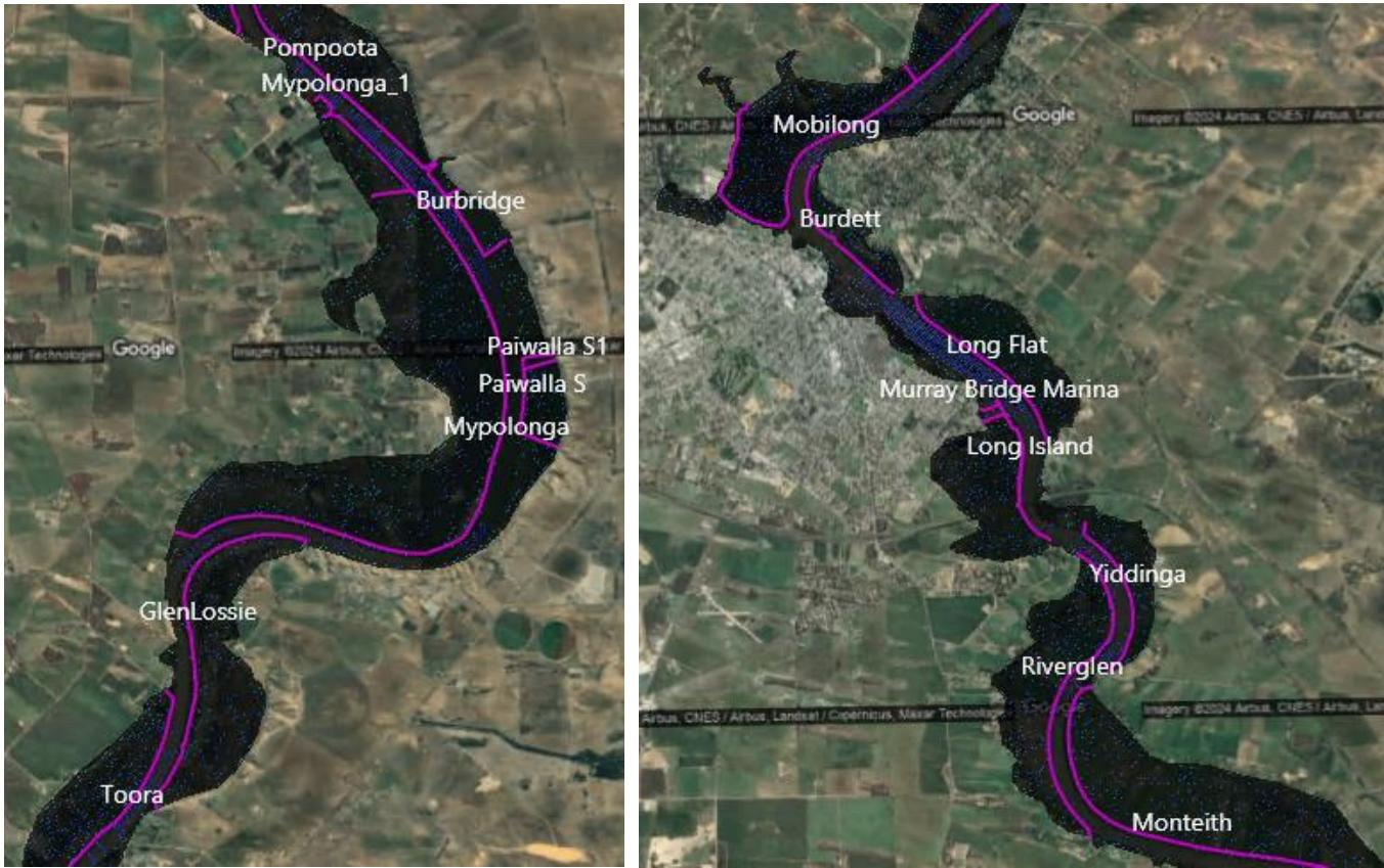
**Figure 6.3.** Features including tracks, roads and levee banks included in the model between Monteith and Pompoota (shown in pink with IDs as named in the model).
