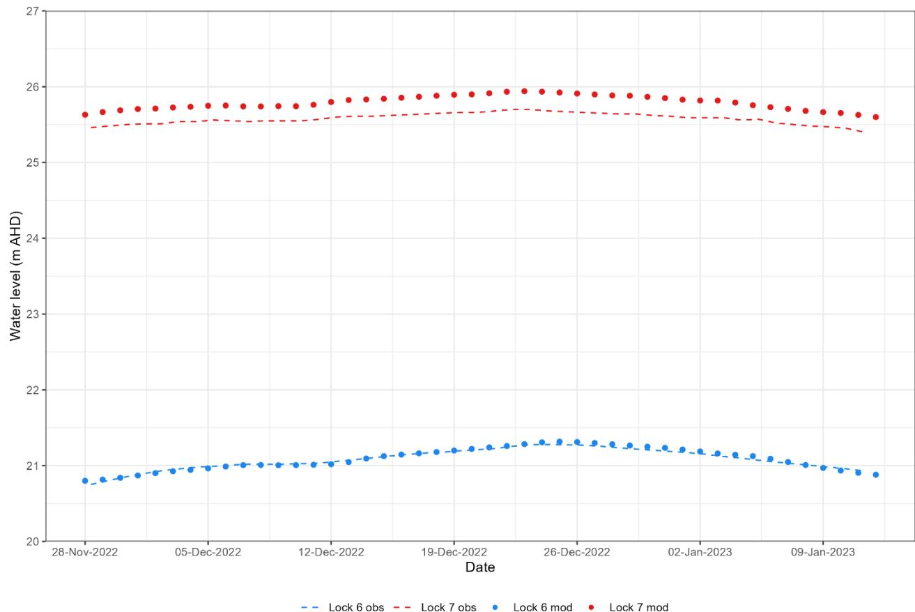
**Figure 6.21. Water level comparisons modelled ('mod') to observed ('obs') for 2022–23 flood event peak at active monitoring stations at Lock 6 and Lock 7. Lock 7 water level comparison impacted by model inflows distributed through River Murray, Lindsay River and Mullaroo Creek channels rather than spread across the floodplain under real-world conditions.**
