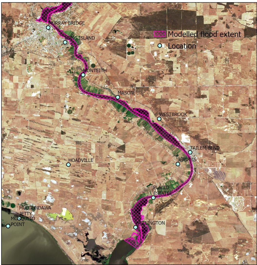
**Figure 6.17. Modelled inundation extent between Murray Bridge and Wellington superimposed on satellite imagery of flood inundation at 1 January 2023 (Copernicus Sentinel data 2024).**
