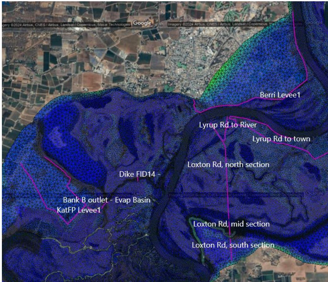
**Figure 6.7.** Features including tracks, roads and levee banks included in the model at Katarapko, Gurra Gurra and Berri (shown in pink with IDs as named in the model).
