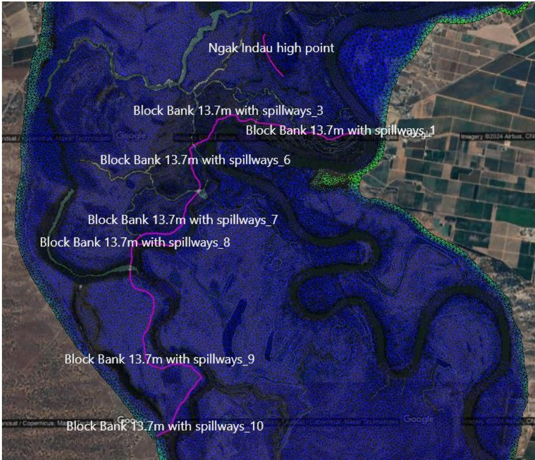
Figure 6.8. Features including tracks, roads and levee banks included in the model at Katarapko (shown in pink with IDs as named in the model).
