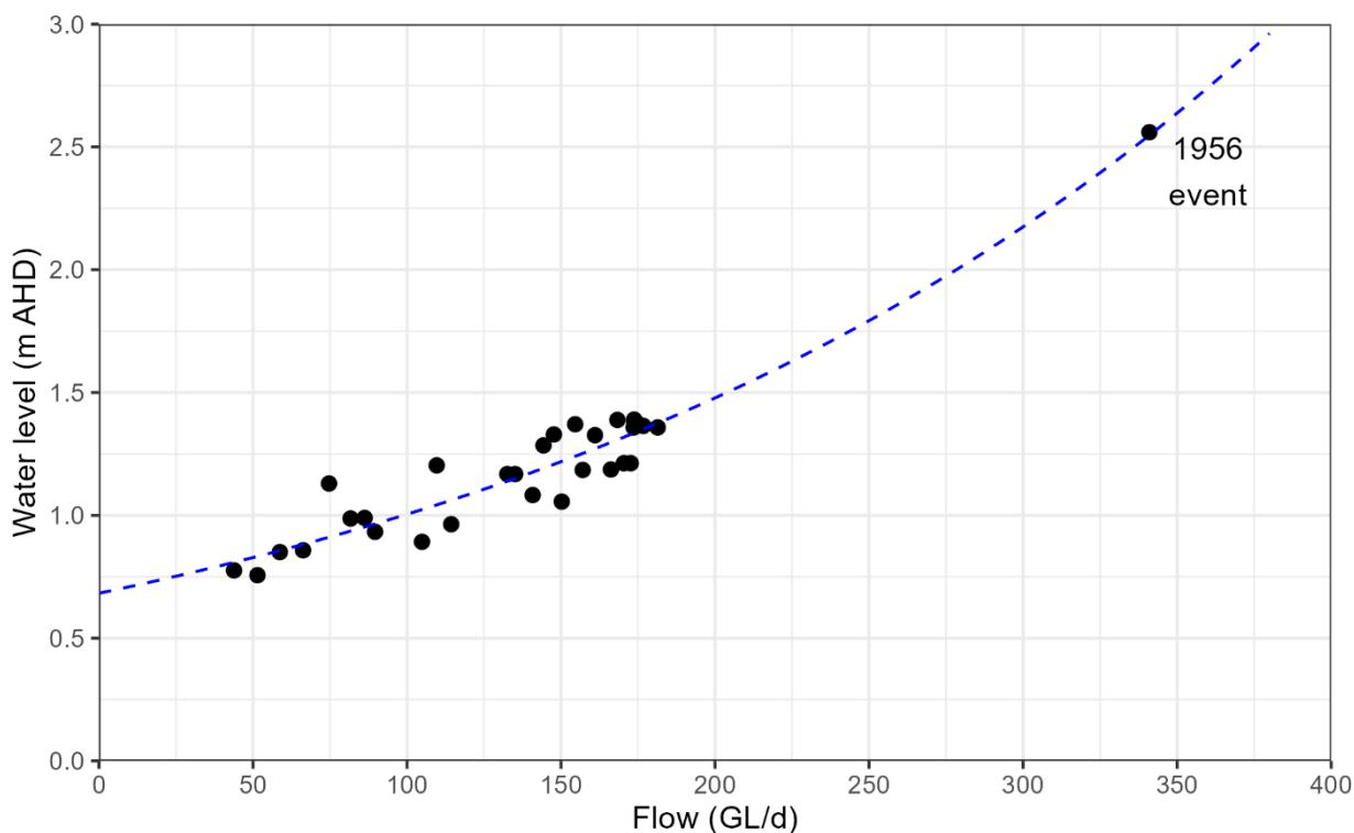
**Figure 2.3. Relationship of observed water level at Wellington and River Murray gauged flow at Lock 1.**
