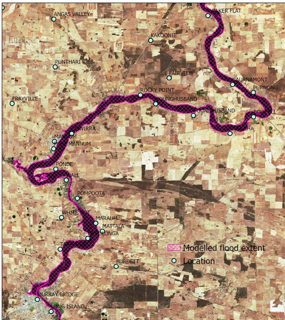
**Figure 6.16. Modelled inundation extent between Walker Flat and Murray Bridge superimposed on satellite imagery of flood inundation at 1 January 2023 (Copernicus Sentinel data 2024).**
