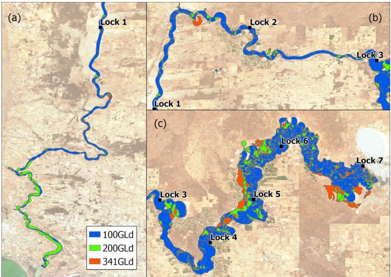
**Figure 3.1. Selected modelled inundation extents in reaches (a) Wellington to Lock 1, (b) Lock 1 to Lock 3, and (c) Lock 3 to Lock 7.**
