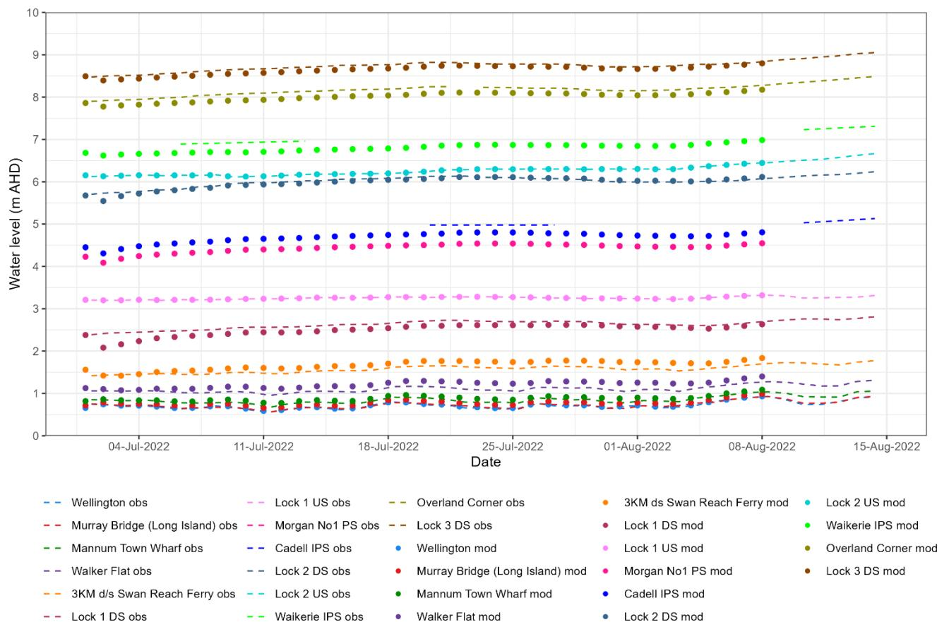
**Figure 6.13. Water level comparisons modelled ('mod') to observed ('obs') for July to August 2022 at active monitoring stations between Wellington and Lock 3.**
