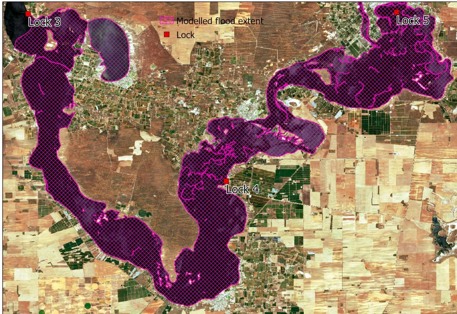
**Figure 6.20.** Modelled inundation extent between Lock 3 and Lock 5 superimposed on satellite imagery of flood inundation at 27 December 2022 (Copernicus Sentinel data 2024).
