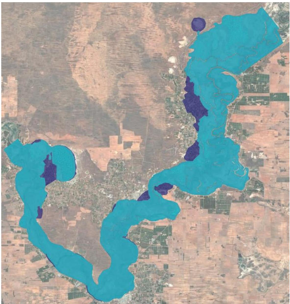
**Figure 6.5. Initial mesh extent (light blue) and expanded areas (dark blue).**
