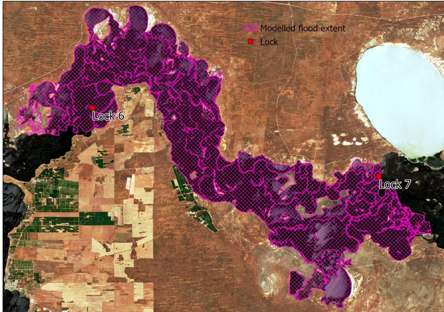
**Figure 6.22. Modelled inundation extent for Lock 6 to Lock 7 model superimposed on satellite imagery of flood inundation at 27 December 2022 (Copernicus Sentinel data 2024).**
