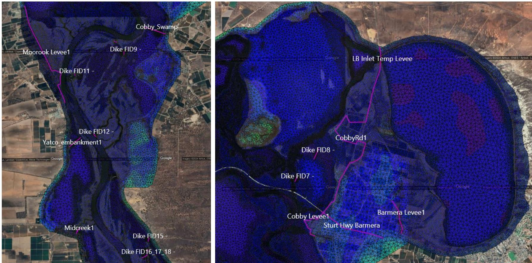
**Figure 6.10.** Features including tracks, roads and levee banks included in the model between Yatco Lagoon and Lake Bonney (shown in pink with IDs as named in the model).
