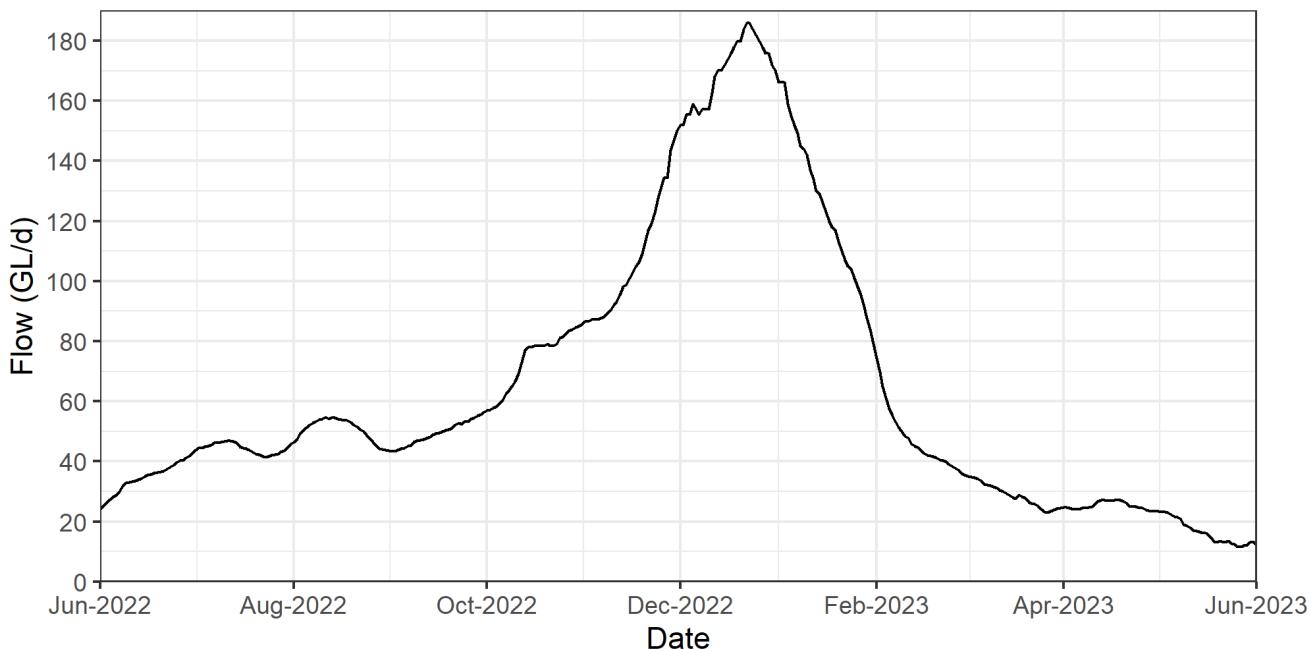
**Figure 1.1. QSA hydrograph of 2022–23 flood event.**
