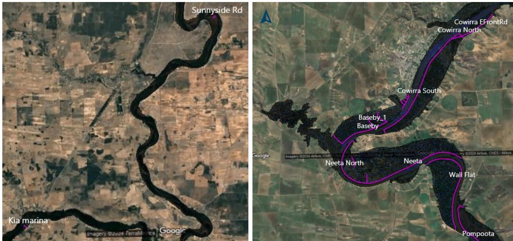
**Figure 6.2.** Features including tracks, roads and levee banks included in the model between Pompoota and Swan Reach (shown in pink with IDs as named in the model).
