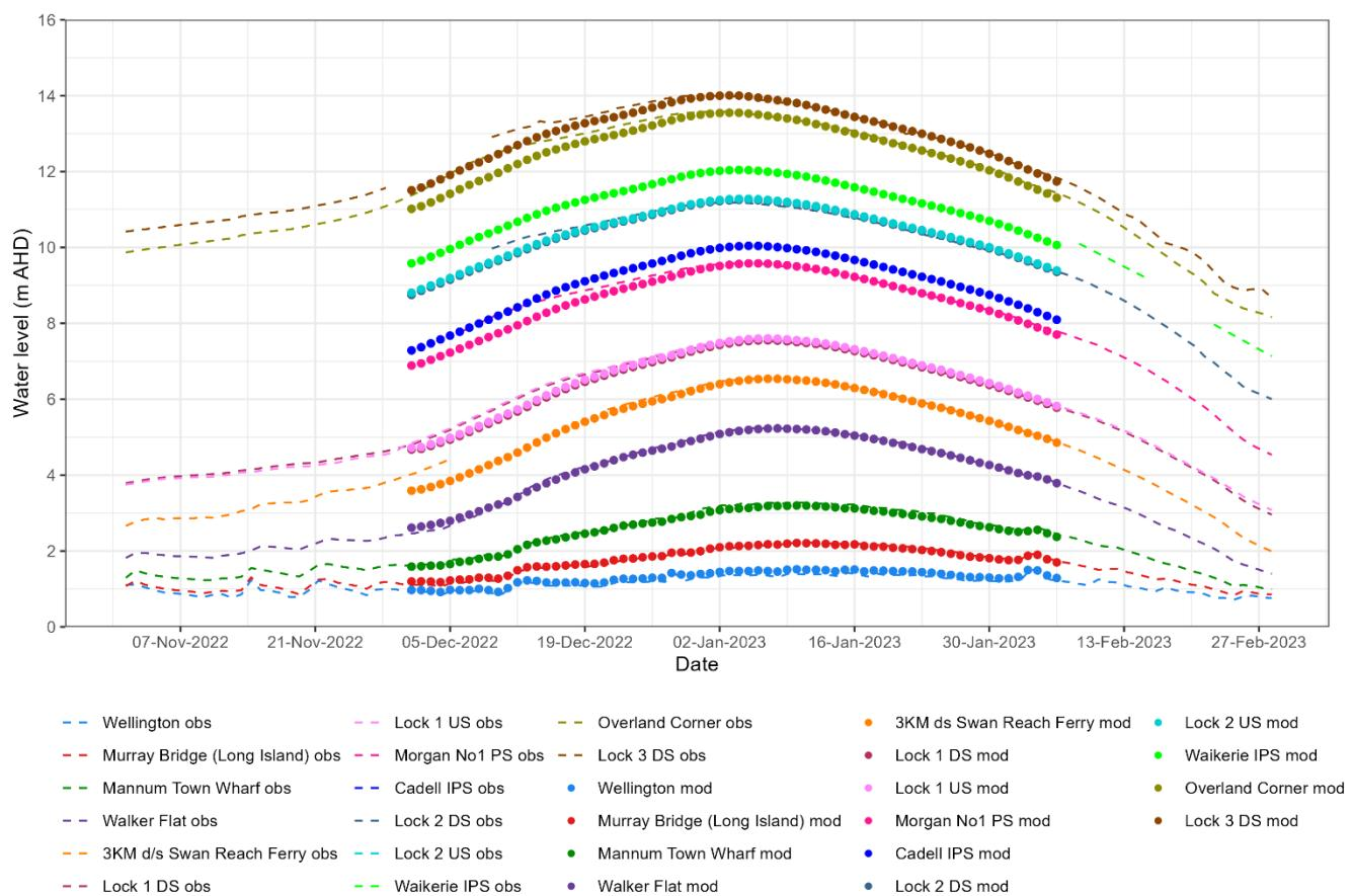
**Figure 6.12. Water level comparisons modelled ('mod') to observed ('obs') for 2022–23 flood event peak at active monitoring stations between Wellington and Lock 3.**
