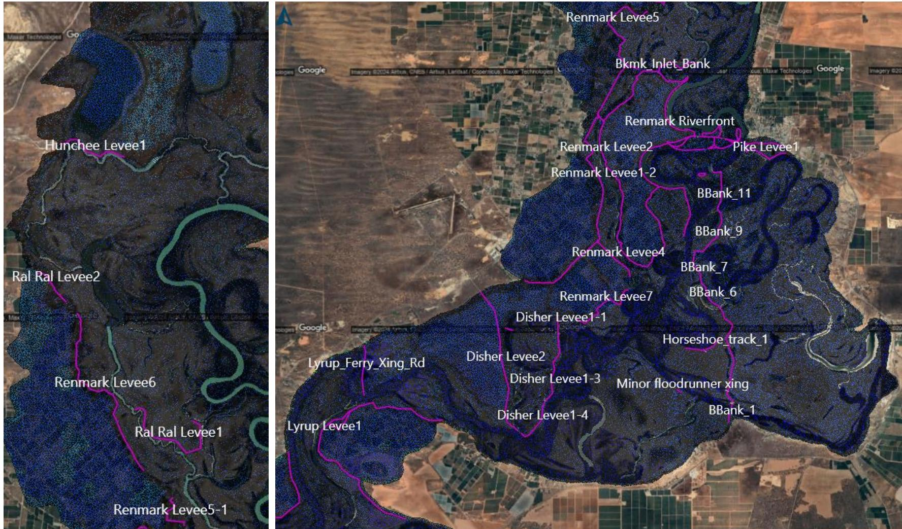
**Figure 6.6. Features including tracks, roads and levee banks included in the model from Renmark to Lyrup and Pike Floodplain (shown in pink with IDs as named in the model).**
