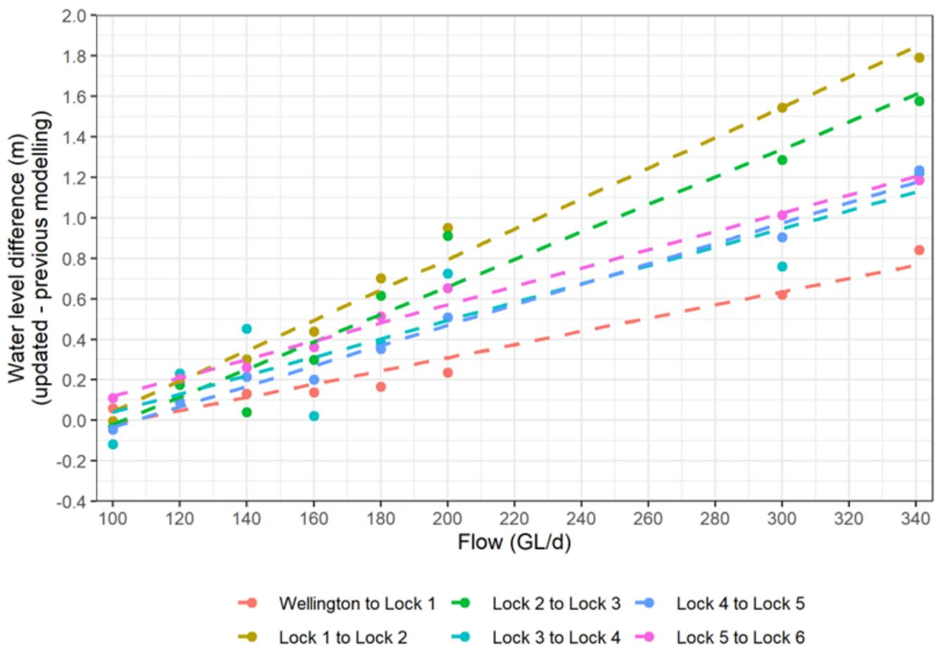
**Figure 3.4. Average differences in modelled water levels between updated and previous modelling outputs by lock weir pool reach and river flow.**
