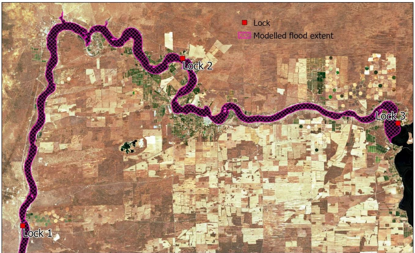
**Figure 6.14. Modelled inundation extent between Lock 1 and Lock 3 superimposed on satellite imagery of flood inundation at 1 January 2023 (Copernicus Sentinel data 2024).**
