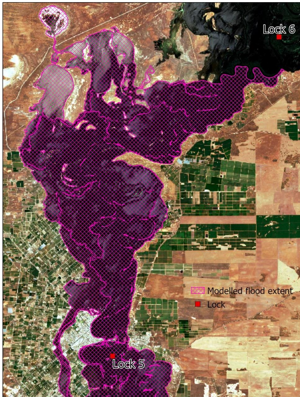
**Figure 6.19. Modelled inundation extent between Lock 5 and Lock 6 superimposed on satellite imagery of flood inundation at 27 December 2022 (Copernicus Sentinel data 2024).**
