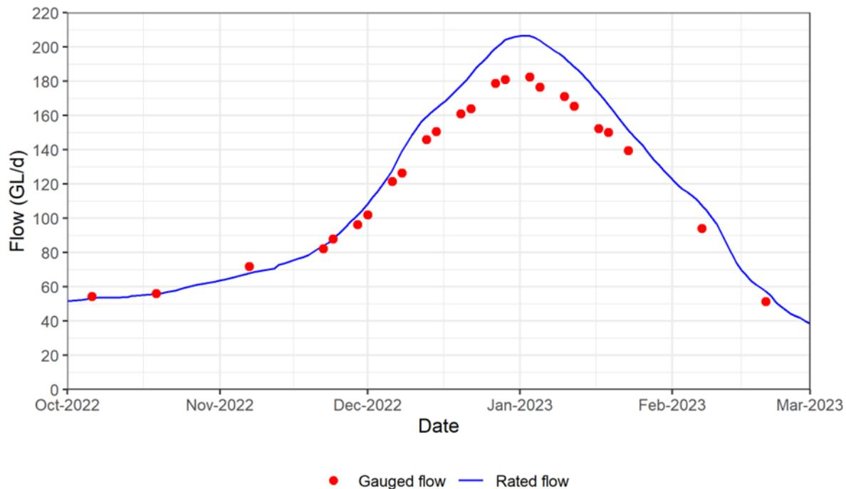
**Figure 1.2. Comparison of gauged and calculated flow using the existing rating at Overland Corner gauging station (A4260528) during the 2022–23 flood event.**
