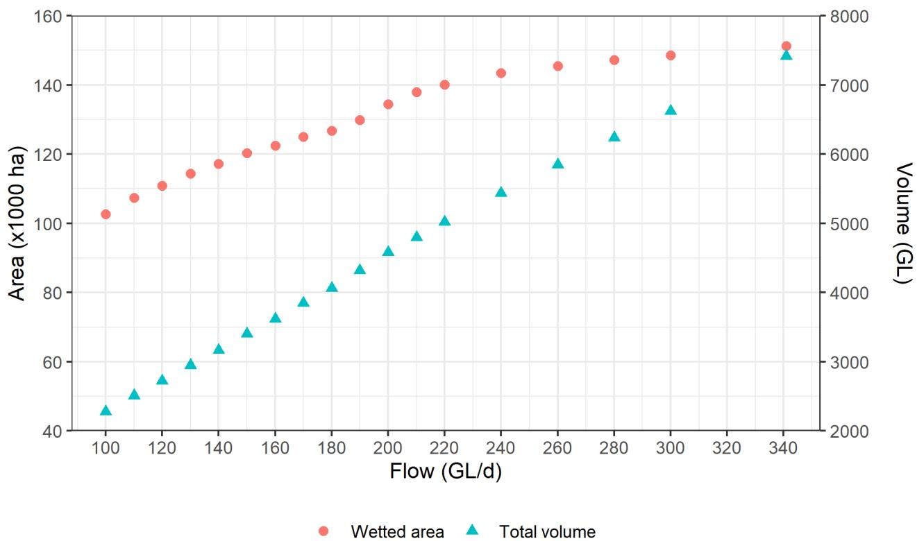
**Figure 3.2. Wetted areas and volumes between Wellington and Lock 7 for modelled flows from 100 to 341 GL/d.**
