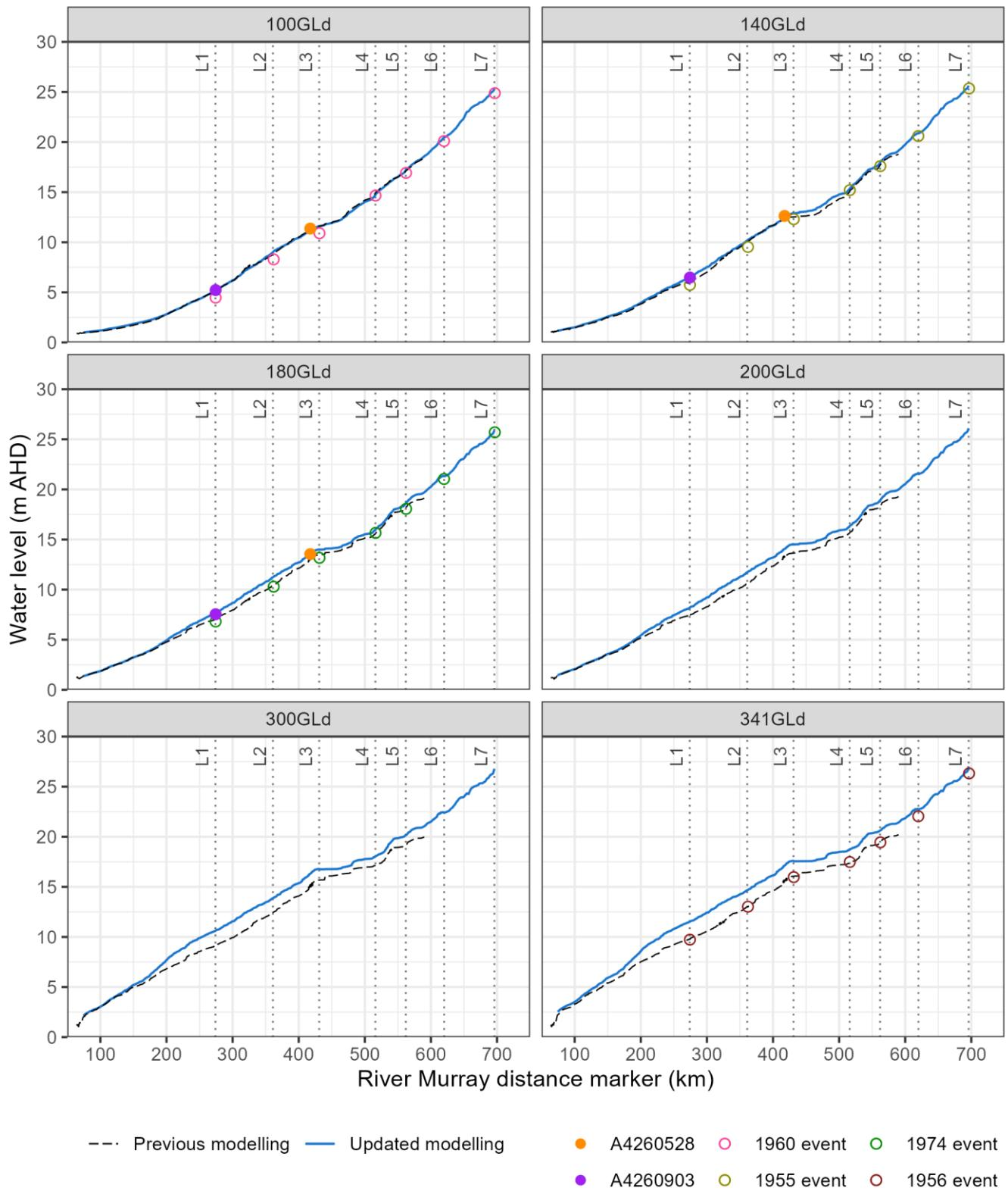
**Figure 3.3. River Murray water level profiles between Wellington and Lock 7 at various flows, with lock locations indicated (dotted lines). Observed water levels shown from the 2022–23 flood event at Lock 1 (A4260903) and Overland Corner (A4260528) gauging stations at 100, 140 and 180 GL/d; and from peak levels observed at locks from flood events in 1960 (96 GL/d), 1955 (147 GL/d), 1974 (182 GL/d) and 1956 (341 GL/d).**
