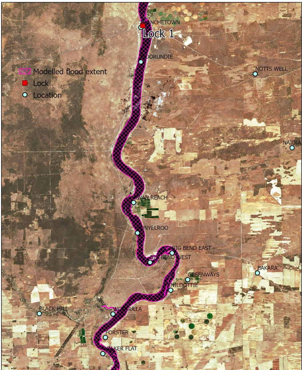
**Figure 6.15. Modelled inundation extent between Lock 1 and Walker Flat superimposed on satellite imagery of flood inundation at 1 January 2023 (Copernicus Sentinel data 2024).**
