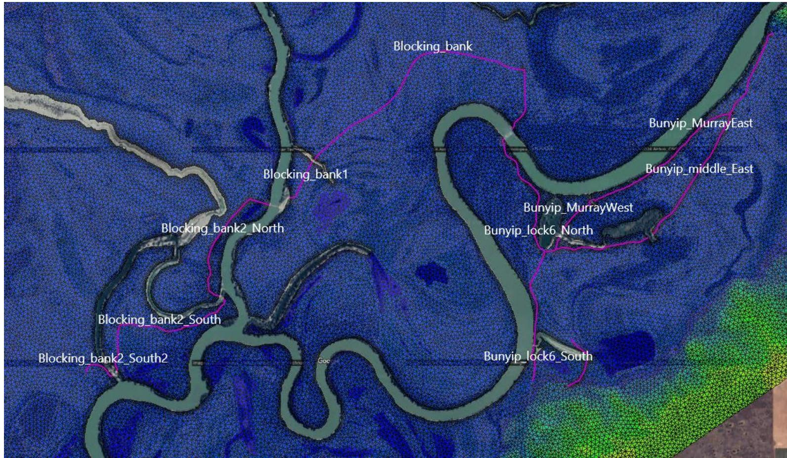
**Figure 6.11.** Features including tracks, roads and levee banks included in the model at Chowilla (shown in pink with IDs as named in the model).
