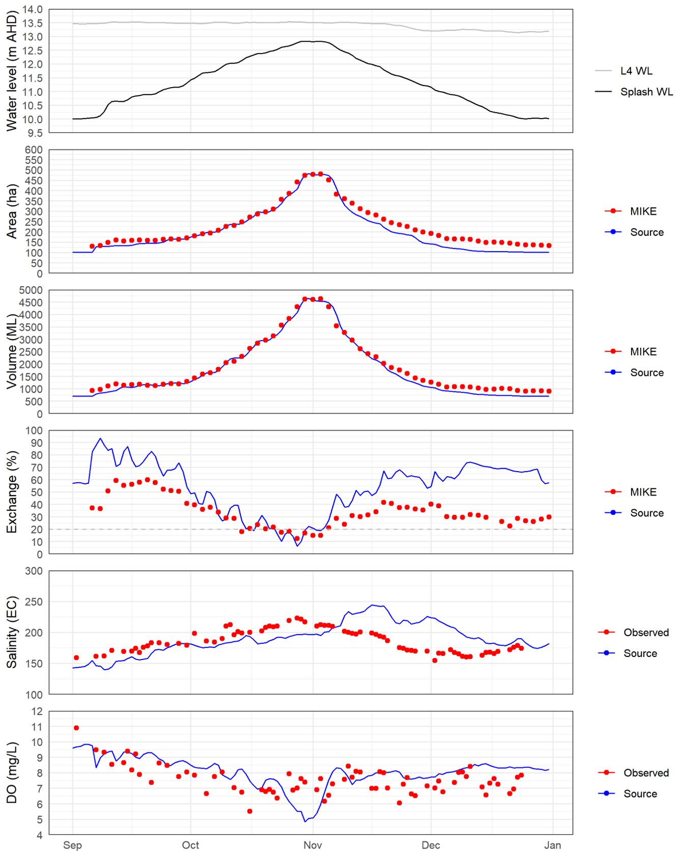
**Figure 3.9** Modelled daily outputs at Katarapko Floodplain for 2020 event simulation. Manual salinity and DO readings from upstream of Splash environmental regulator were used as observed data for comparison against daily modelled data.
