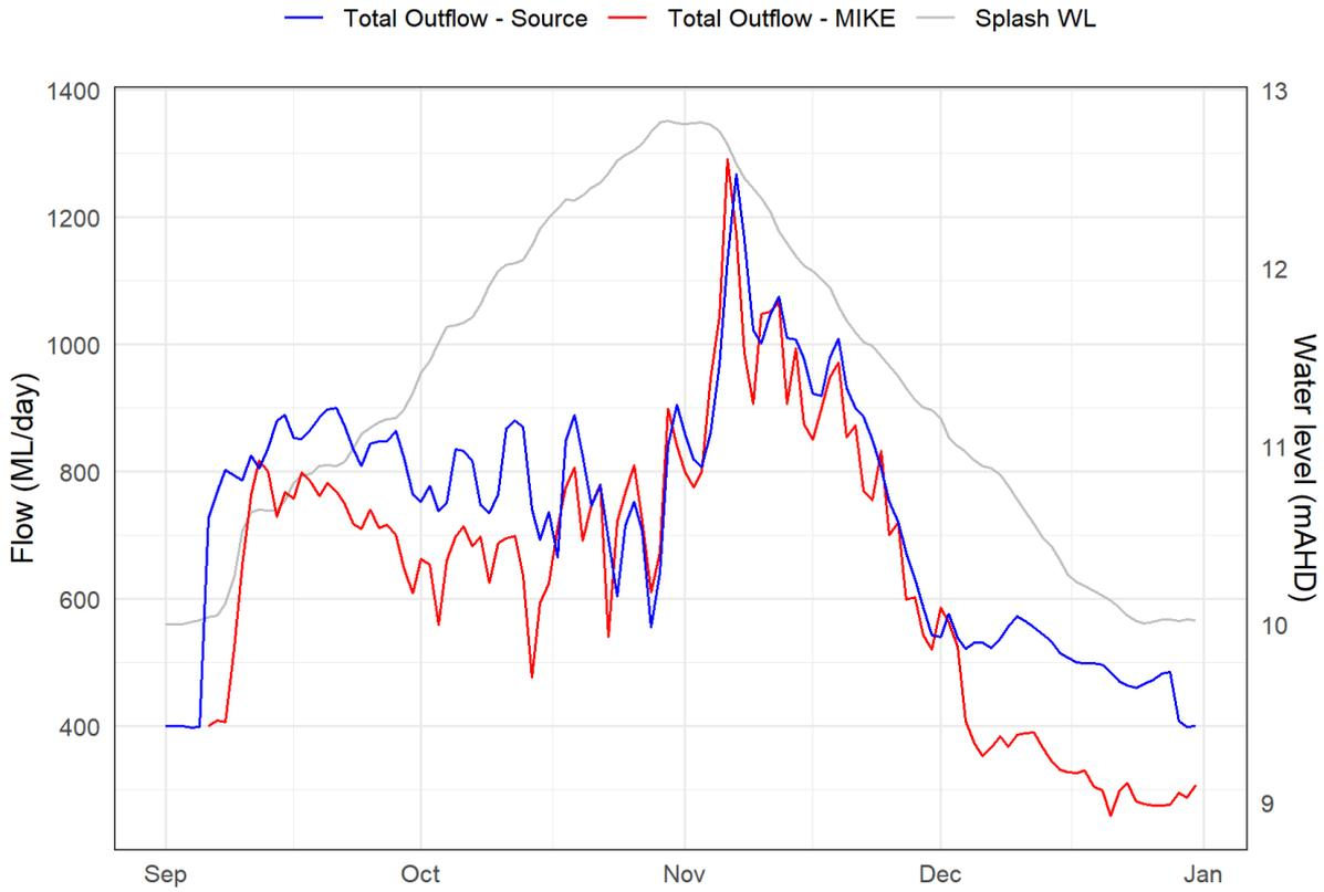
**Figure 3.10 Comparison of total modelled outflows using MIKE and Source models**
