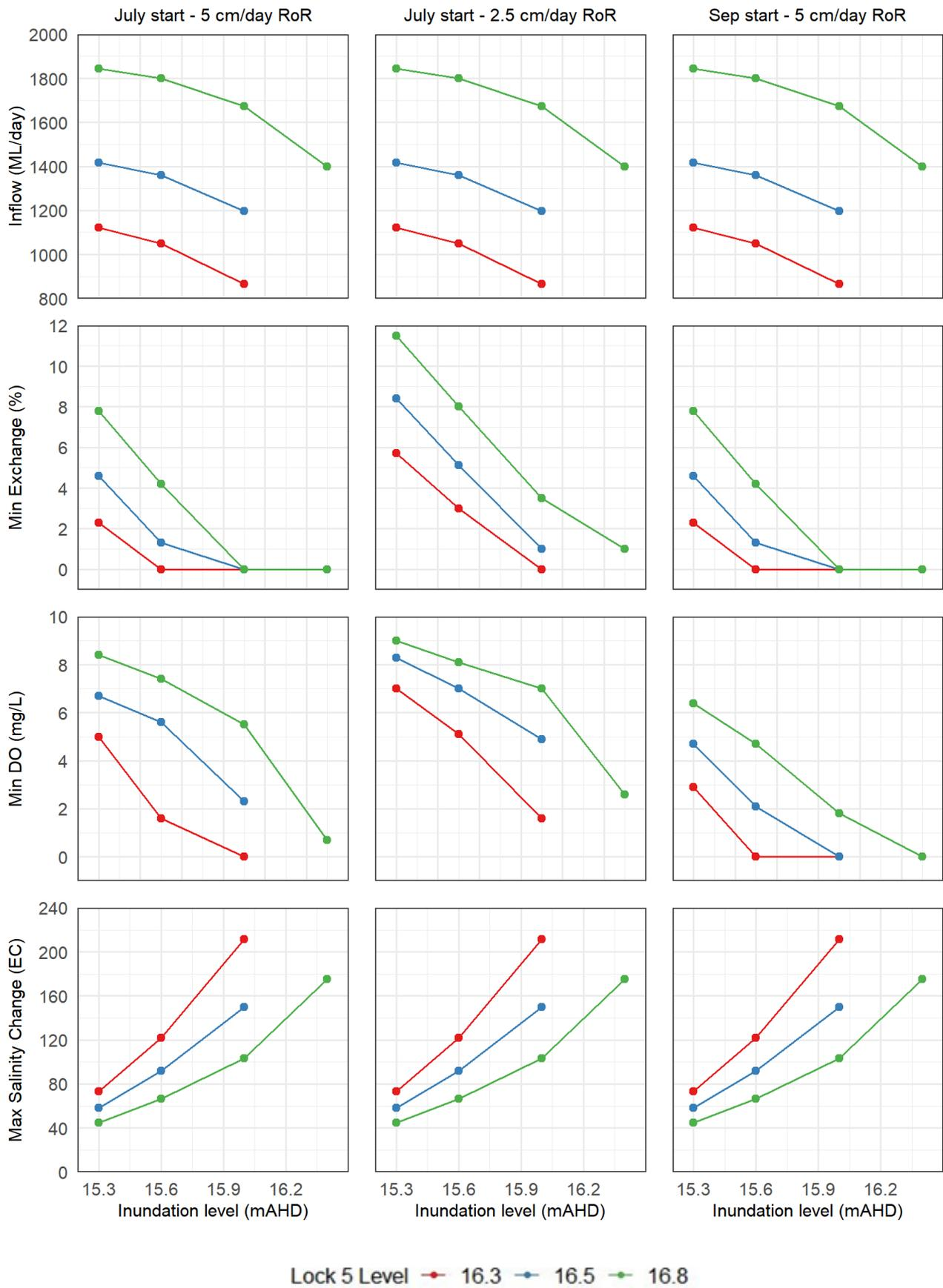
**Figure 4.1** Impact of operations at Pike Floodplain on inflow, Min exchange rate, Min DO and Max Salinity
