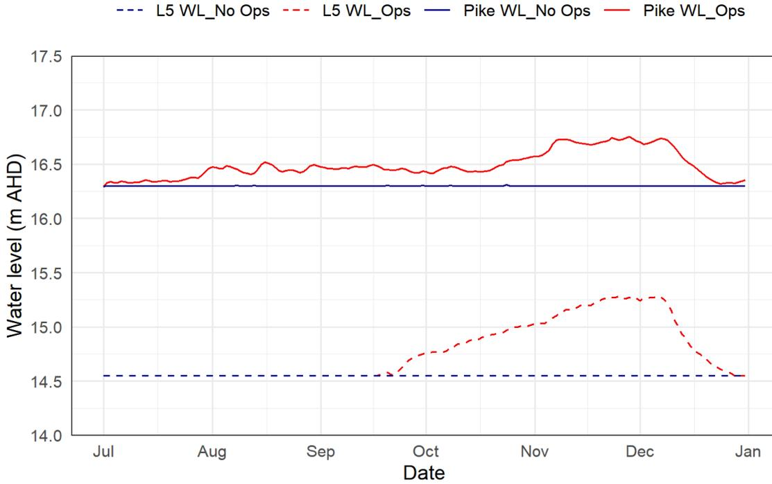
**Figure 3.14 Water elevation at Pike Floodplain and Lock 5**
