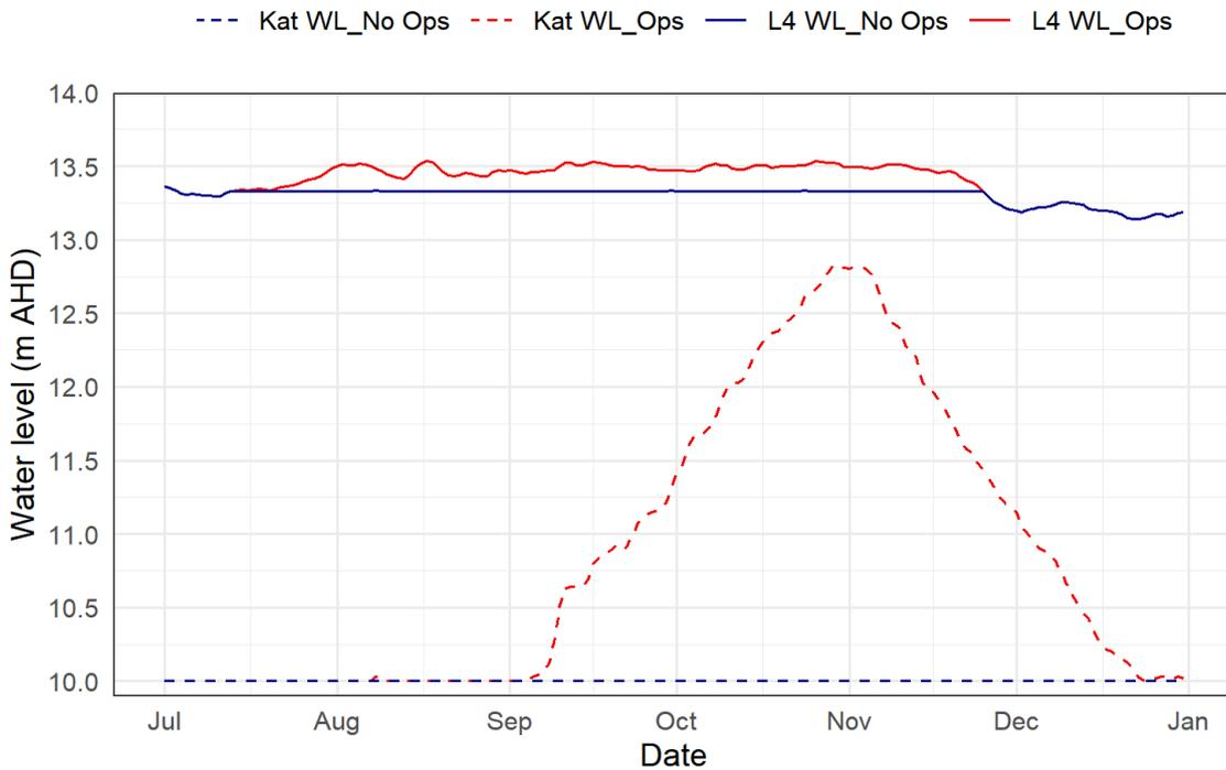
**Figure 3.15 Water elevation at Katarapko Floodplain and Lock 4**
