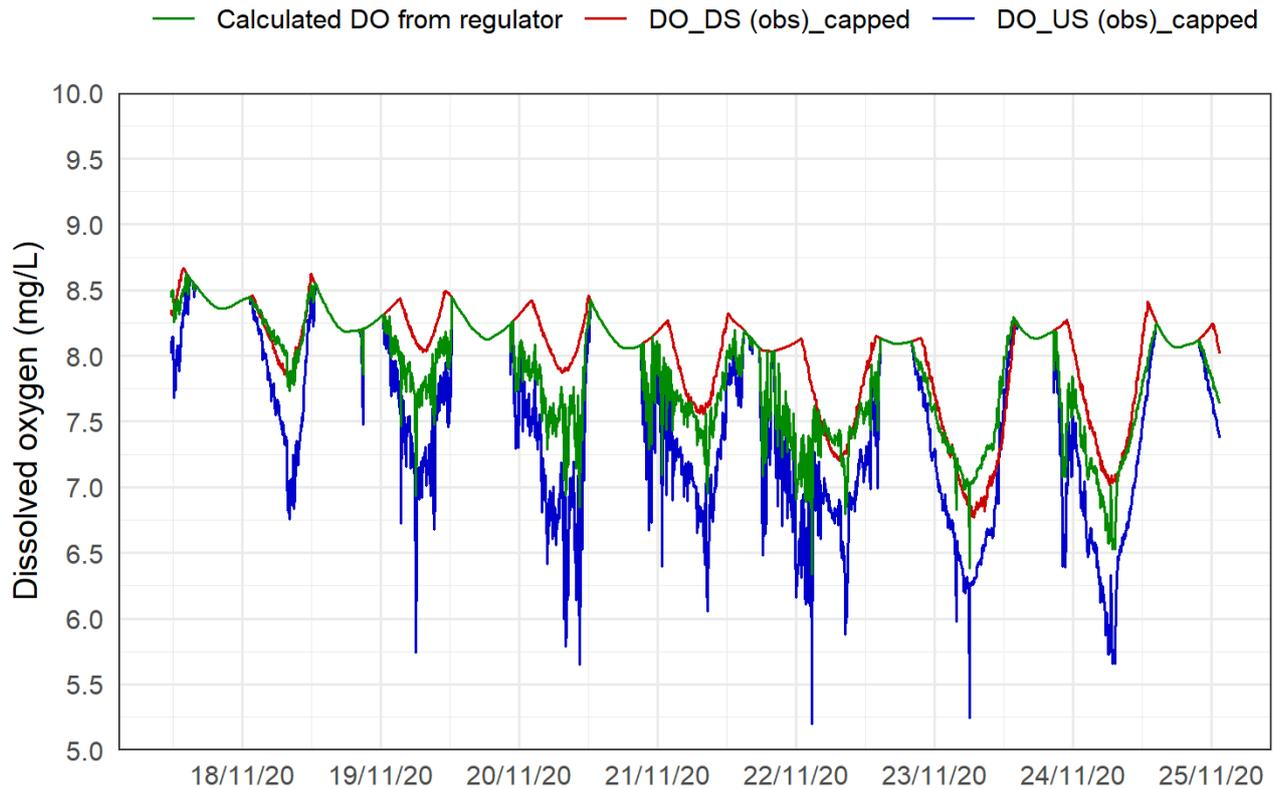
**Figure 3.13 Comparison of observed DO and calculated DO below the Sawmill Regulator. Note that the observed DO has been capped at the saturated DO concentration based on water temperature.**
