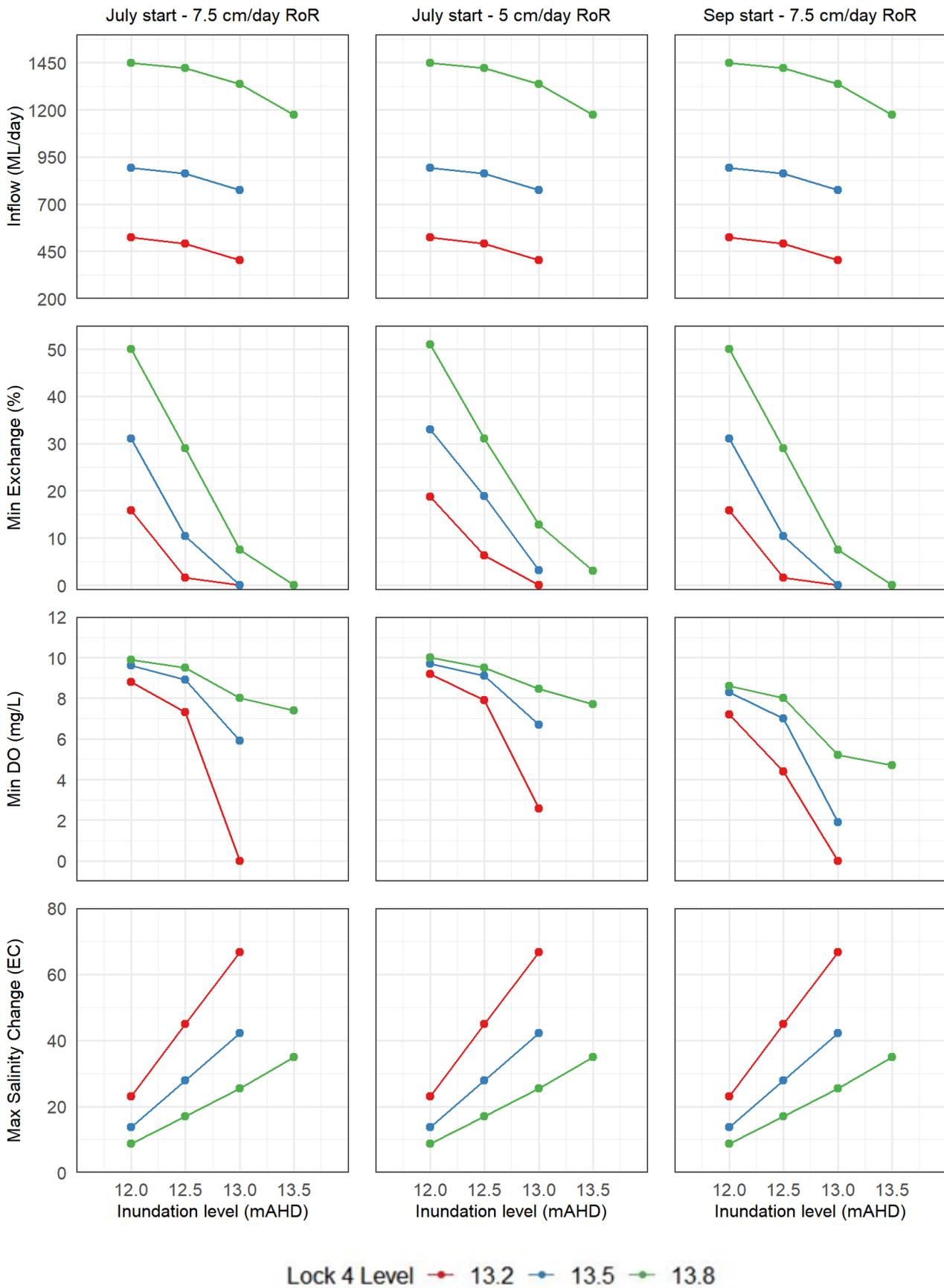
**Figure 4.2** Impact of operations at Katarapko Floodplain on inflow, Min exchange rate, Min DO and Max Salinity
