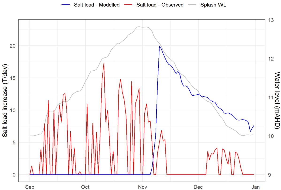
**Figure 3.11 Modelled salt load vs. observed salt load due to operation at Katarapko Floodplain**
