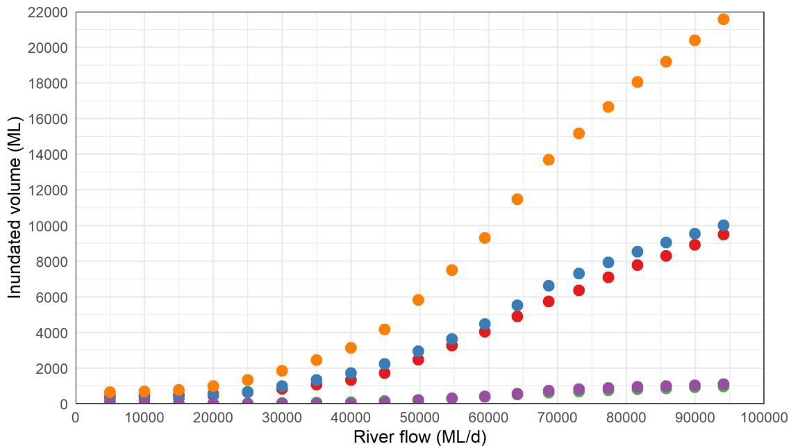
**Figure 3.27. Variation of storage volume upstream of the Katarapko blocking alignment with River Murray flow.**
