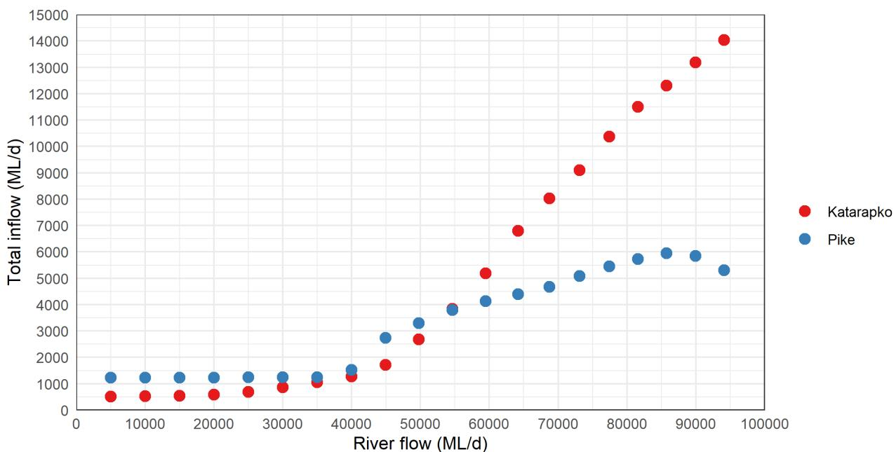
**Figure 3.23. Variation of total flow through various inlets at Katarapko and Pike with River Murray flow (based on flow through 1D model branches).**
