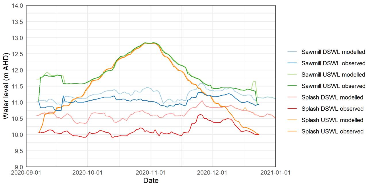
**Figure 3.20. Katarapko Floodplain environmental regulator upstream and downstream water levels, observed versus modelled.**
