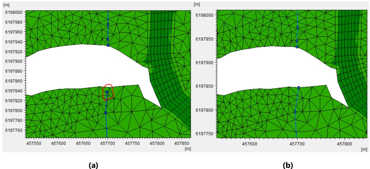
**Figure 6.3.** Modification of dike structure at right bank of The Splash, Katarapko Floodplain.
