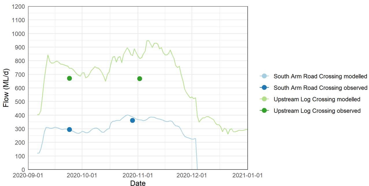
**Figure 3.18. Katarapko floodplain flows comparison, gauged versus modelled.**
