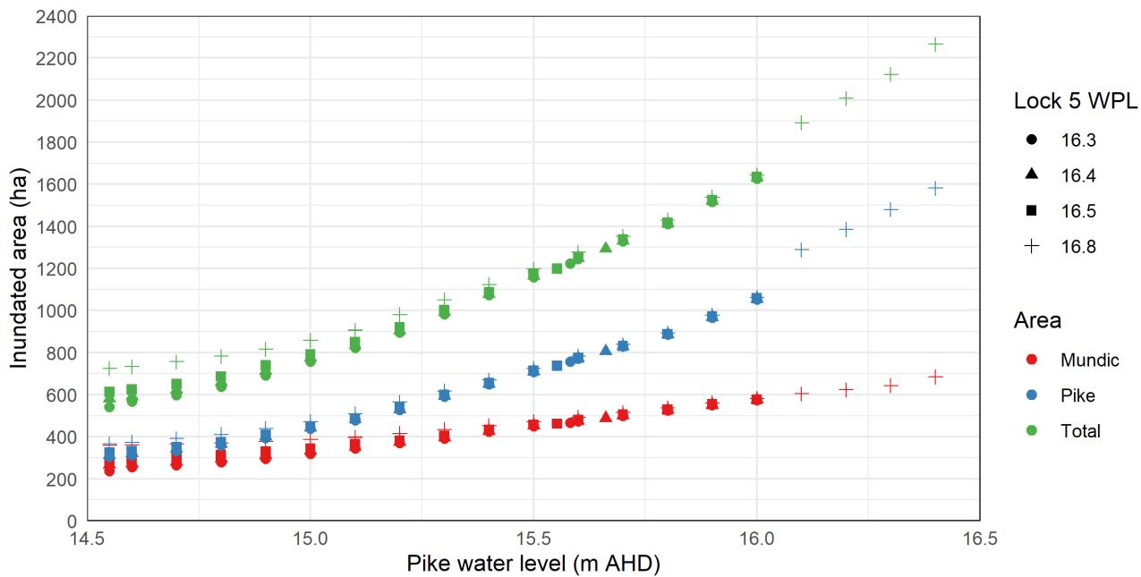
**Figure 3.30. Pike Floodplain inundated area versus Pike water level at various Lock 5 weir pool levels and 10 000 ML/d QSA.**
