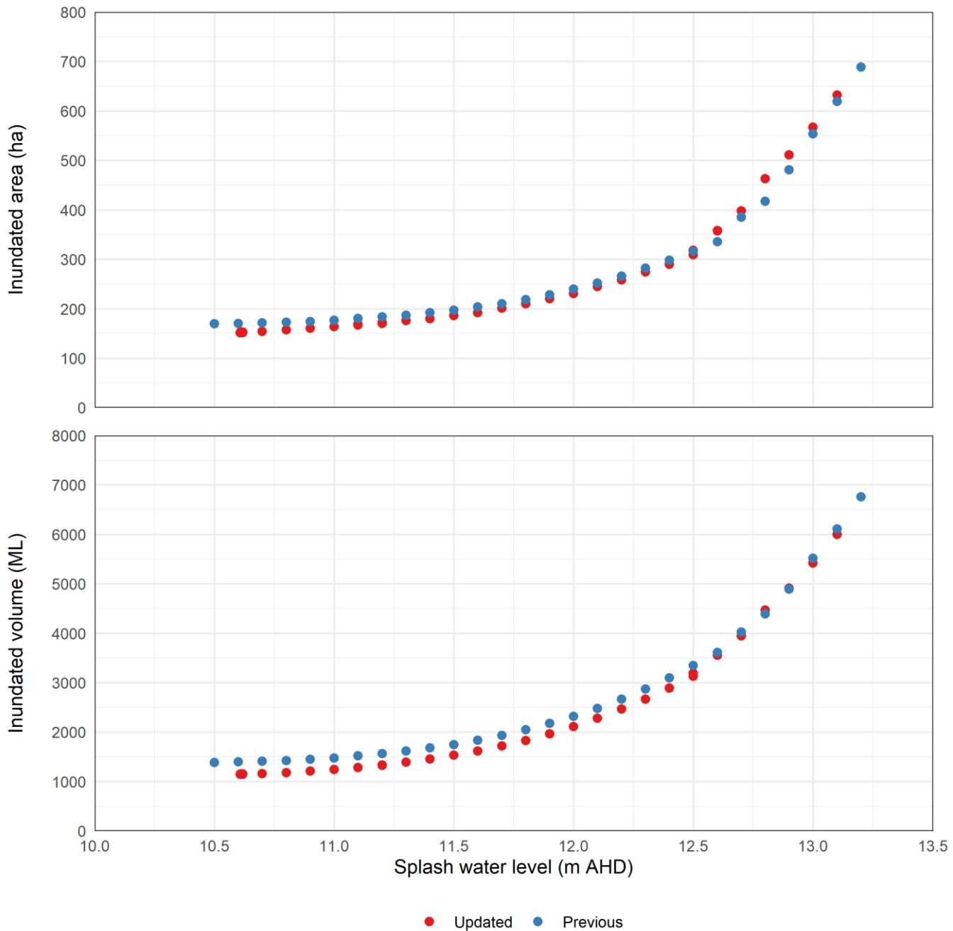
**Figure 3.35. Comparison between updated and previous modelled results of Katarapko Floodplain inundated area and volume versus The Splash water level at Lock 4 weir pool level = 13.5 m AHD and 10 000 ML/d River Murray flow.**
