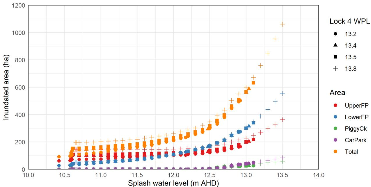
**Figure 3.33. Katarapko Floodplain inundated area versus Splash water level at various Lock 4 weir pool levels and 10 000 ML/d QSA.**
