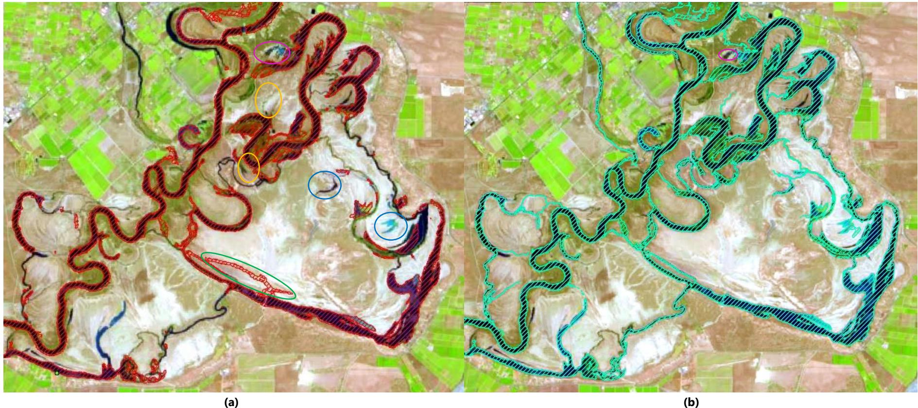
**Figure 3.6.** Pike imagery for 17 November 2020, compared to (a) base and (b) updated model outputs from simulation of 2020 event. Circled areas indicate discrepancy between observed and modelled.
