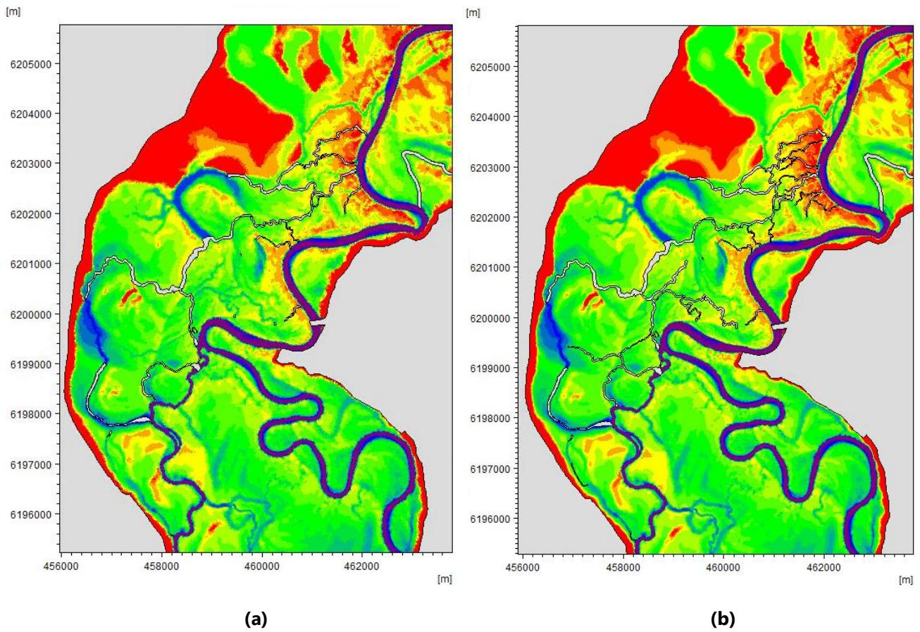
**Figure 6.2.** Flexible mesh at Katarapko floodplain (a) initial, (b) updated.
