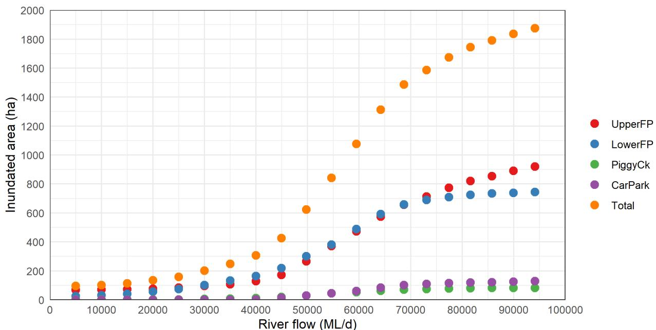
**Figure 3.26. Variation of inundated area upstream of the Katarapko blocking alignment with River Murray flow.**
