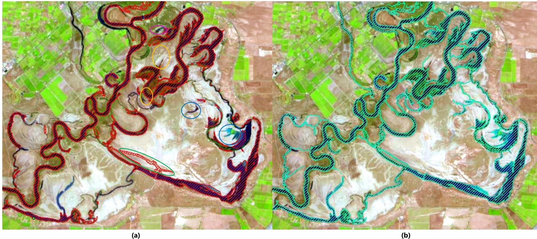
**Figure 3.7.** Pike imagery for 27 November 2020, compared to (a) base and (b) updated model outputs from simulation of 2020 event. Circled areas indicate discrepancy between observed and modelled.
