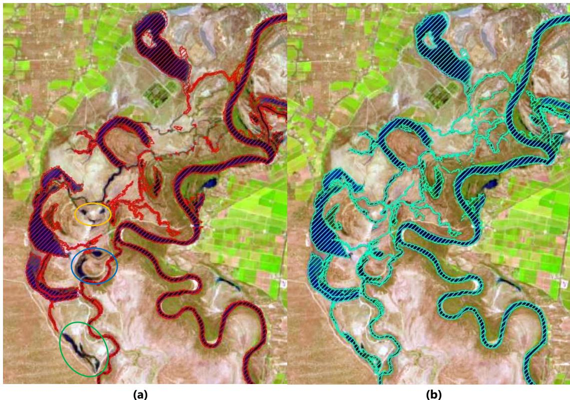
**Figure 3.3.** Katarapko imagery for 2 November 2020, compared to (a) base and (b) updated model outputs from simulation of 2020 event. Circled areas indicate discrepancy between observed and modelled.
