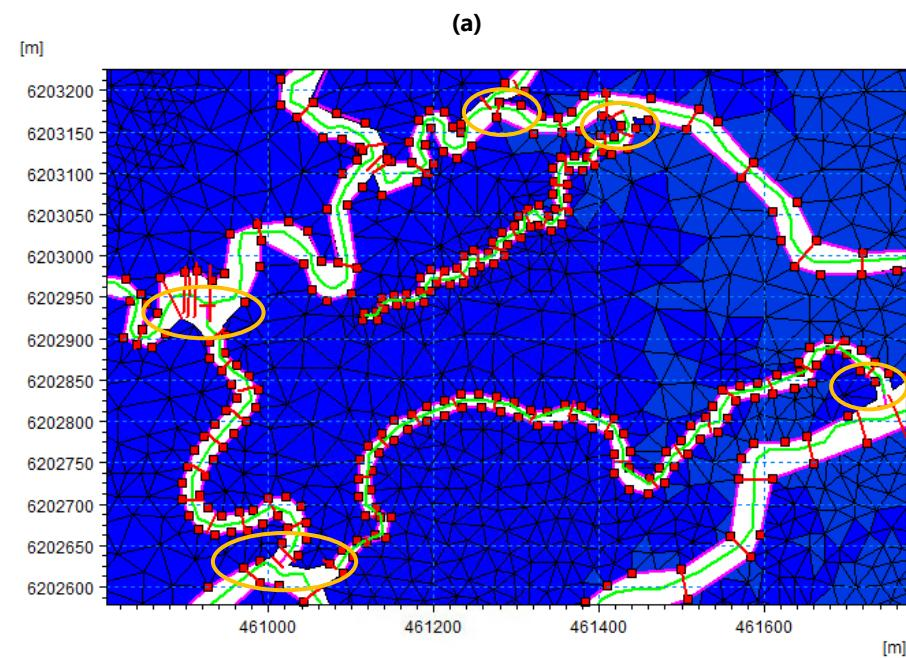
**Figure 6.7.** Adjustment of (a) existing lateral links to accommodate (b) new branches (adjustment locations circled in orange).
