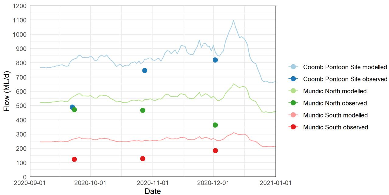
**Figure 3.12. Pike floodplain flows comparison, gauged versus modelled.**
