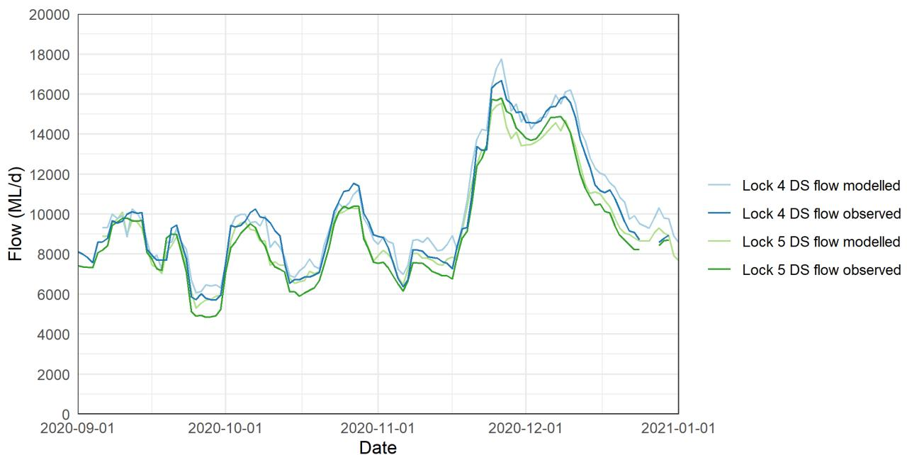
**Figure 3.9. River flows downstream of Locks 4 and 5 comparison, observed versus modelled.**
