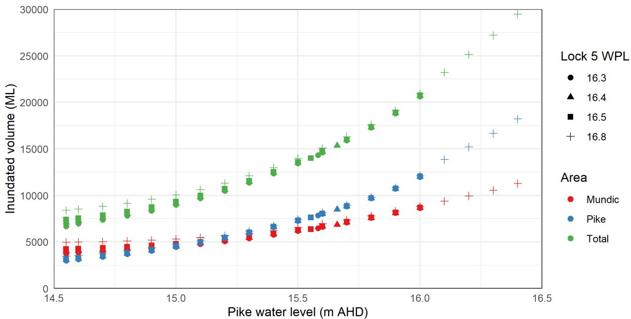
**Figure 3.31. Pike Floodplain inundated volume versus Pike water level at various Lock 5 weir pool levels and 10 000 ML/d QSA.**
