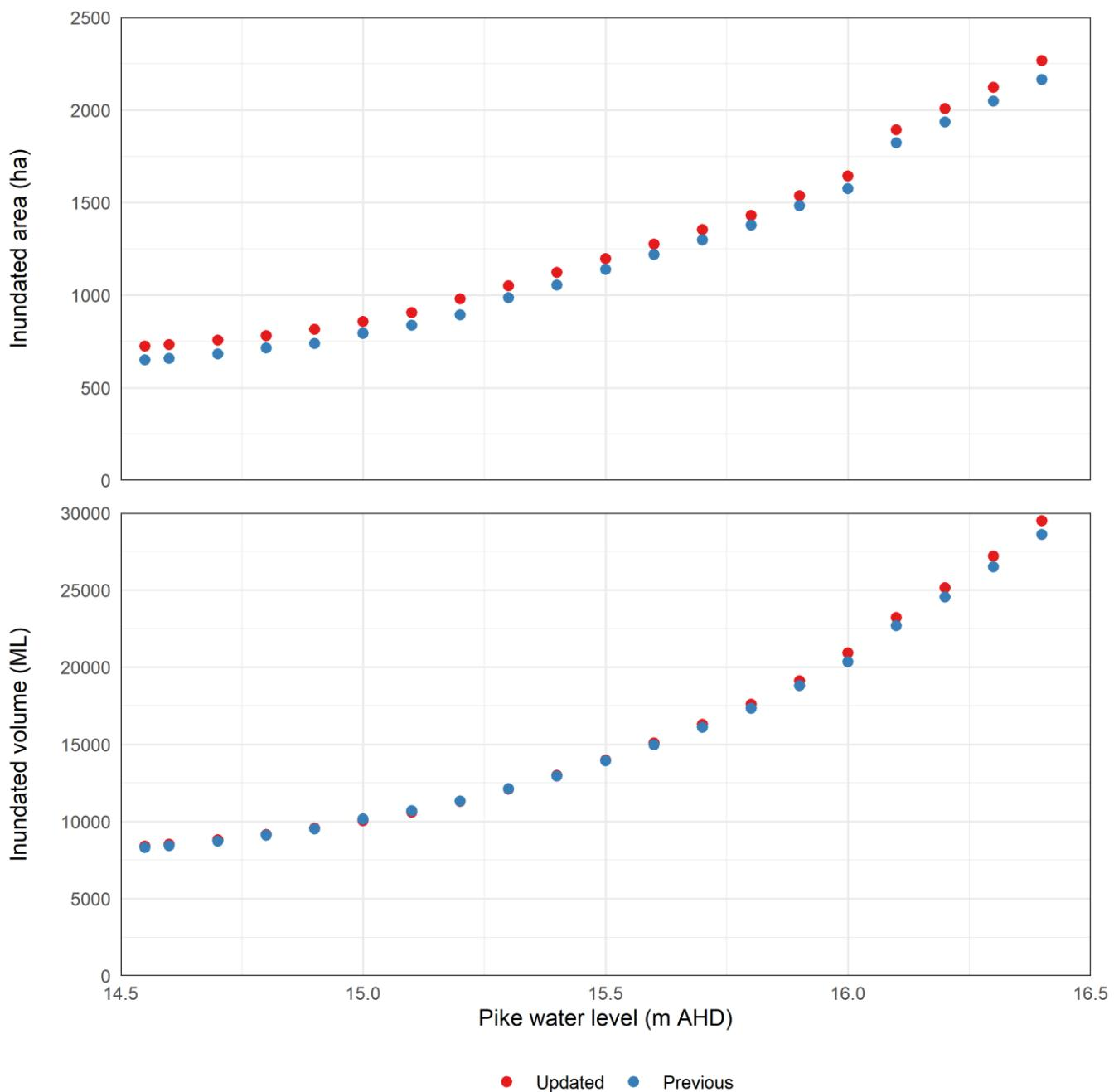
**Figure 3.32. Comparison between updated and previous modelled results of Pike Floodplain inundated area and volume versus Pike regulator water level at Lock 5 weir pool level = 16.8 m AHD and 10 000 ML/d River Murray flow.**
