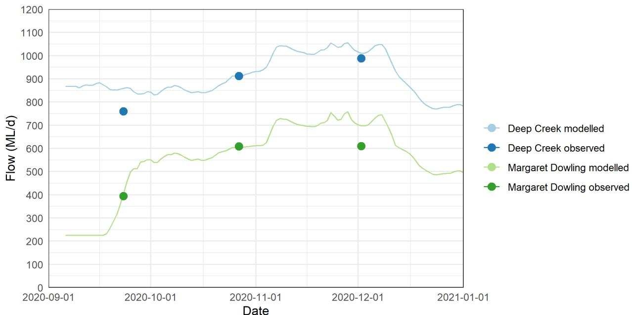
**Figure 3.11. Pike inlets flows comparison, gauged versus modelled.**
