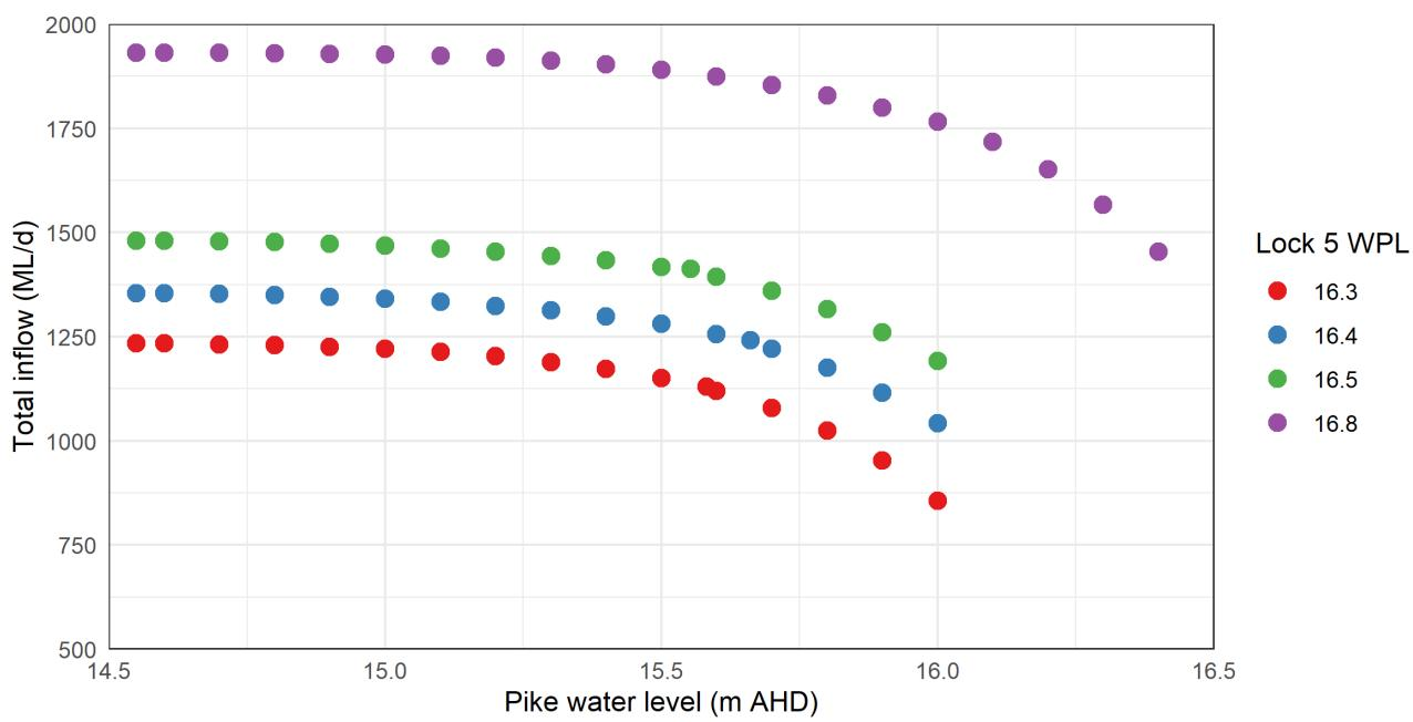
**Figure 3.28. Pike Floodplain total inflow versus Pike water level at various Lock 5 weir pool levels and 10 000 ML/d QSA.**
