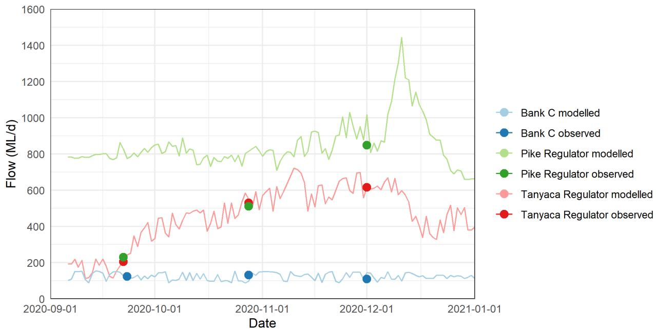
**Figure 3.13. Pike outflows comparison, gauged versus modelled.**
