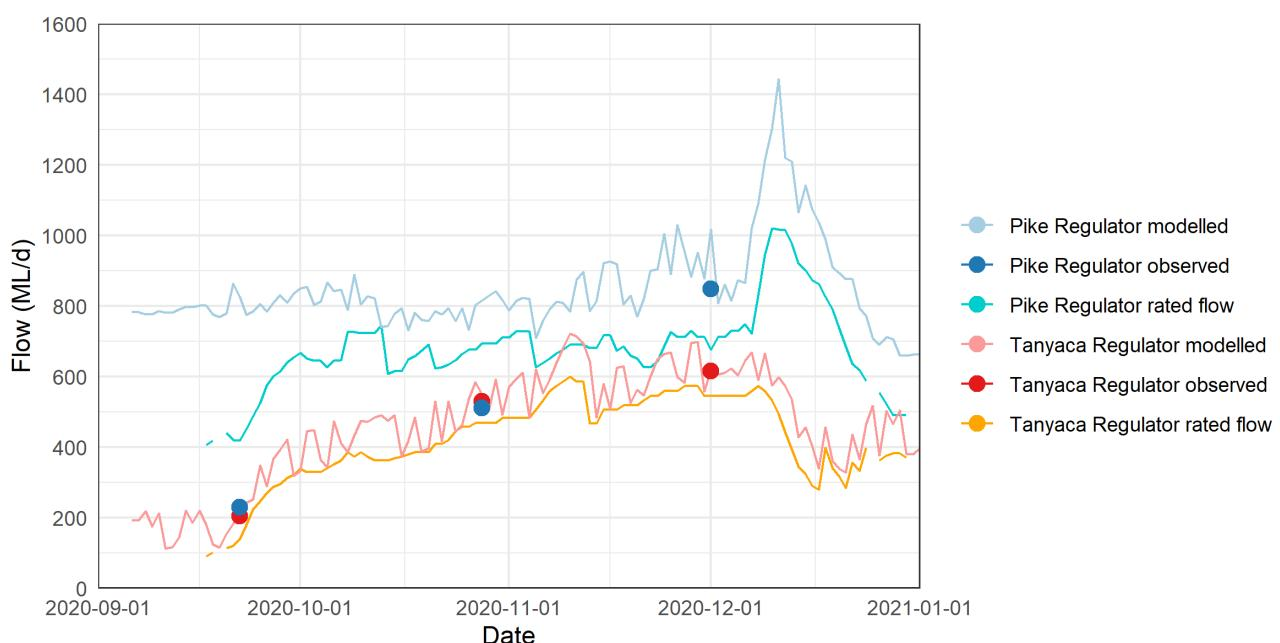
**Figure 3.14. Pike regulator outflows comparison, modelled, gauged and rated flows.**
