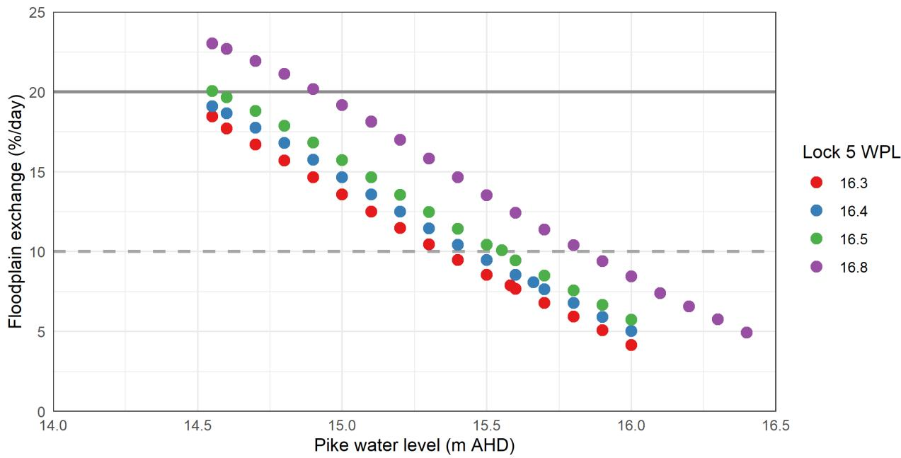
**Figure 3.36. Pike floodplain approximate maximum daily exchange versus Pike regulator water level and Lock 5 weir pool level, at QSA of 10 GL/d.**
