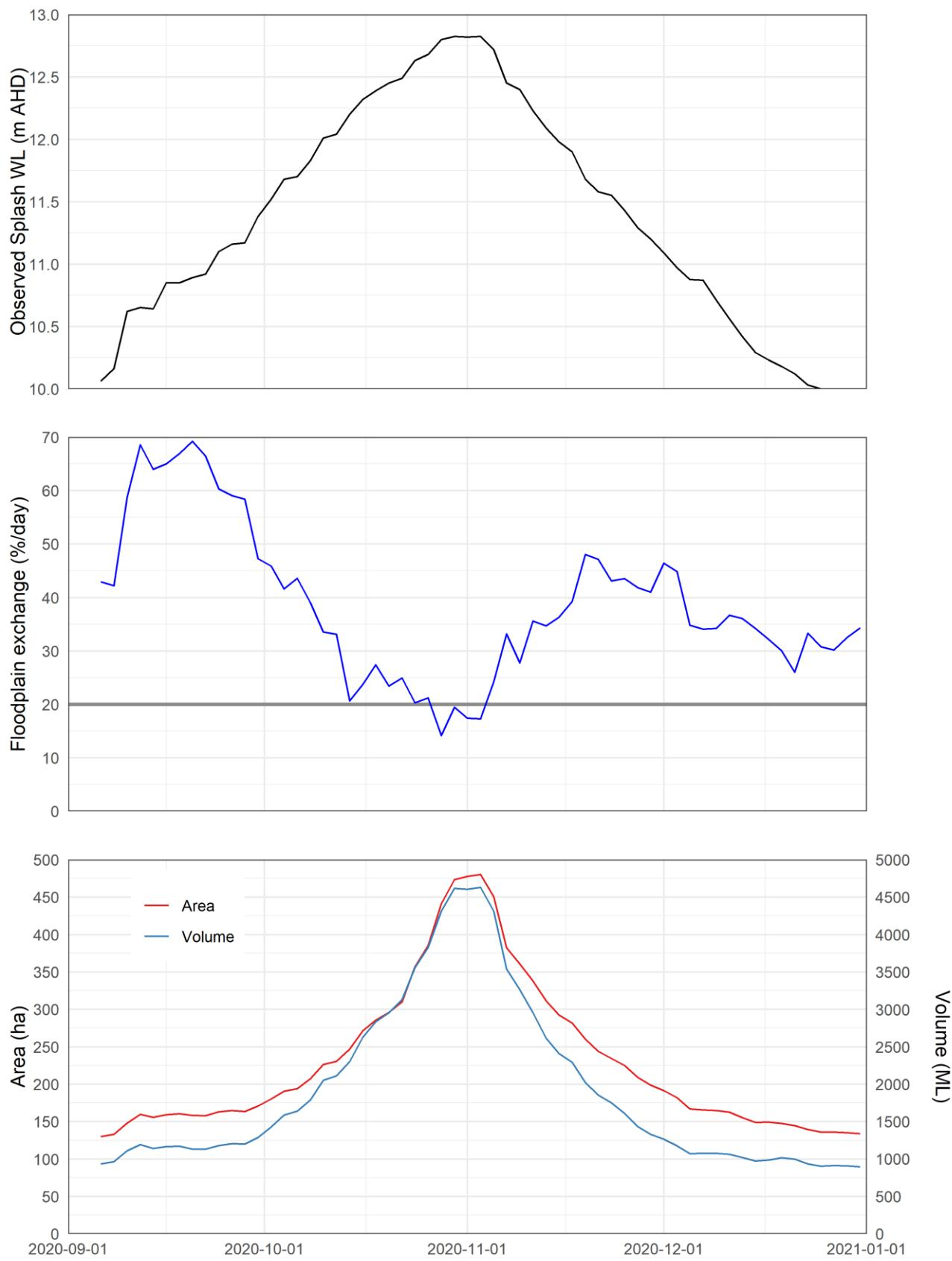
**Figure 3.22. Modelled daily exchange, inundated area and storage volume at Katarapko floodplain for 2020 event simulation.**
