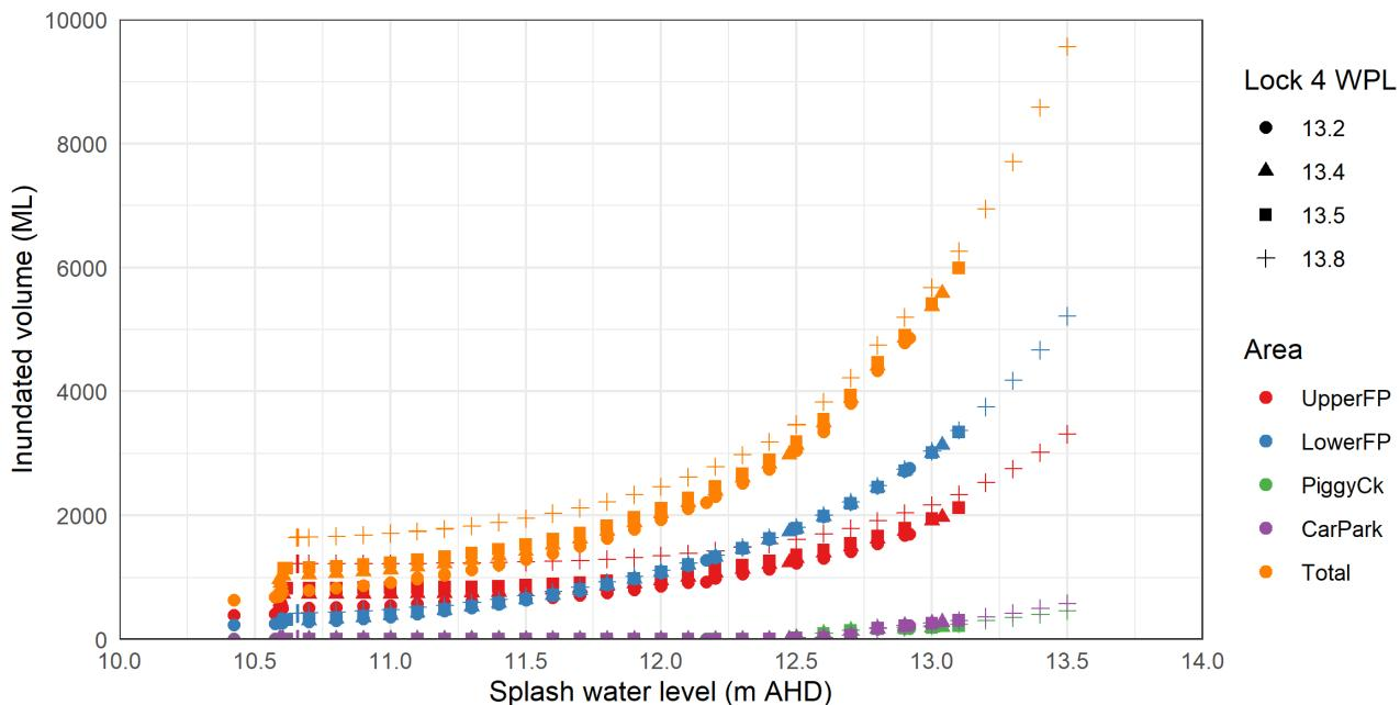
**Figure 3.34. Katarapko Floodplain inundated volume versus Splash water level at various Lock 4 weir pool levels and 10 000 ML/d QSA.**
