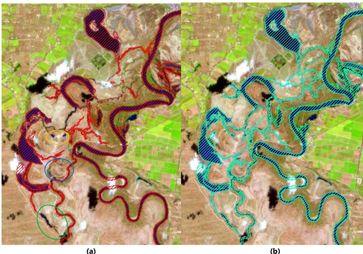
**Figure 3.2.** Katarapko imagery for 28 October 2020, compared to (a) base and (b) updated model outputs from simulation of 2020 event. Circled areas indicate discrepancy between observed and modelled.
