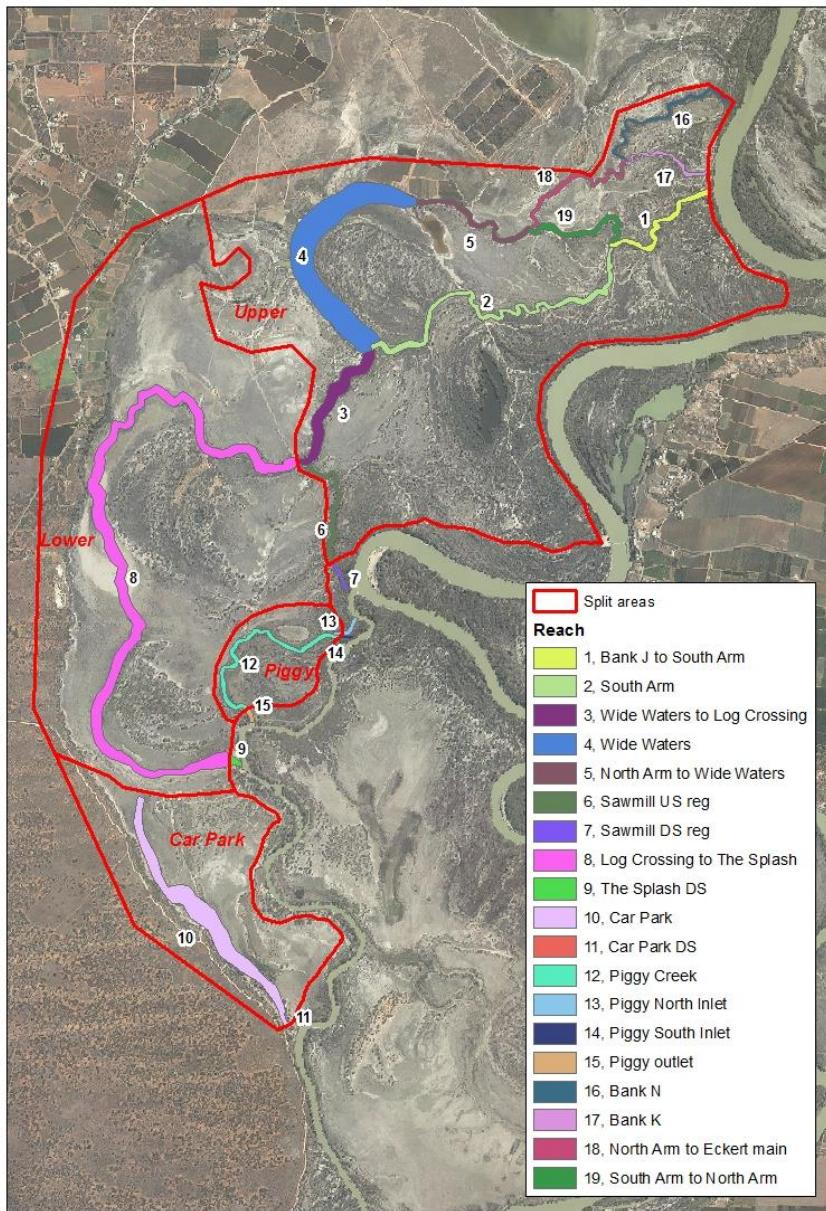
**Figure 2.3. Katarapko floodplain sub-area definitions for area and volume calculations, and reach numbering for velocity analysis.**
