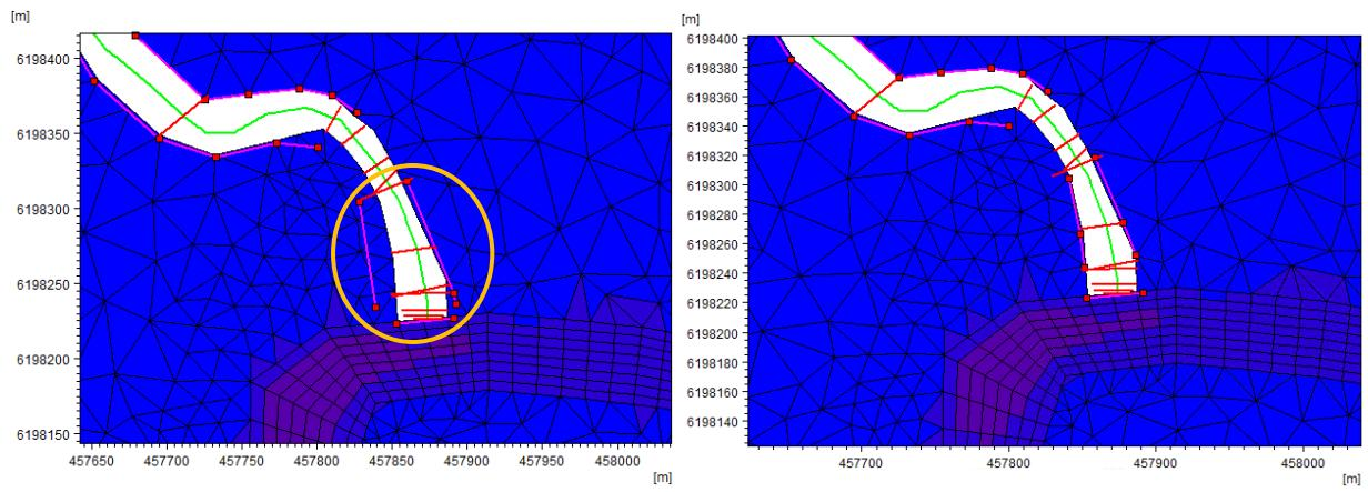
**Figure 6.8. Example of lateral link realignment at Piggy Creek outlet, from (a) existing to (b) adjusted links.**
