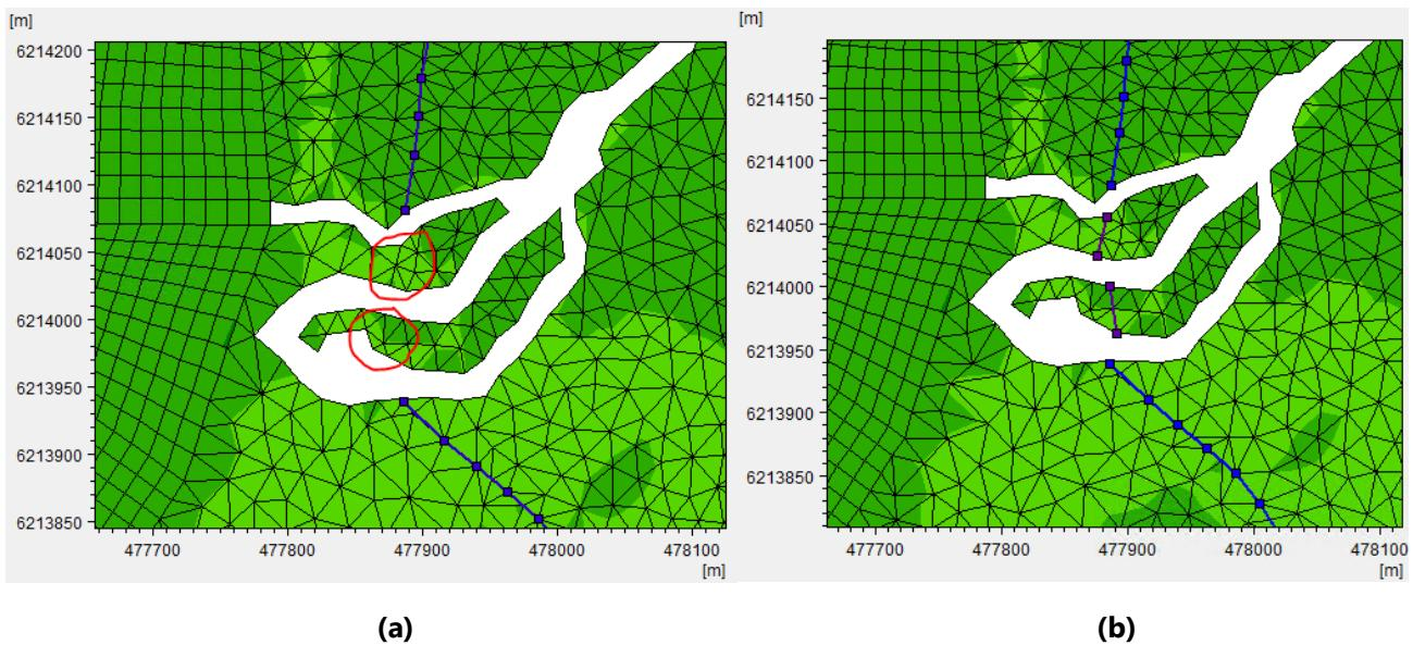
**Figure 6.4. Addition of dike segments at Bank C, Pike Floodplain.**
