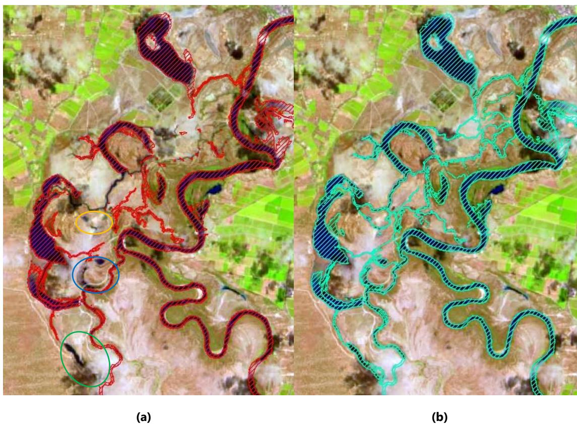
**Figure 3.4.** Katarapko imagery for 7 November 2020, compared to (a) base and (b) updated model outputs from simulation of 2020 event. Circled areas indicate discrepancy between observed and modelled.
