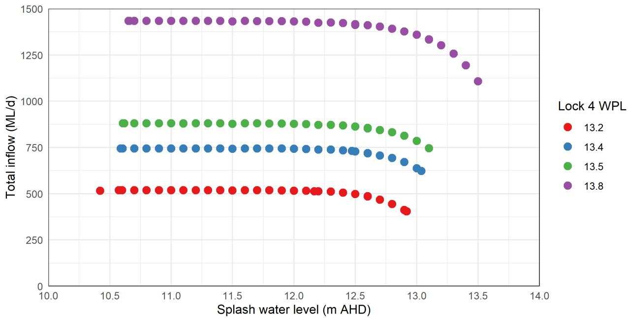
**Figure 3.29. Katarapko Floodplain total inflow versus Splash water level at various Lock 4 weir pool levels and 10 000 ML/d QSA.**
