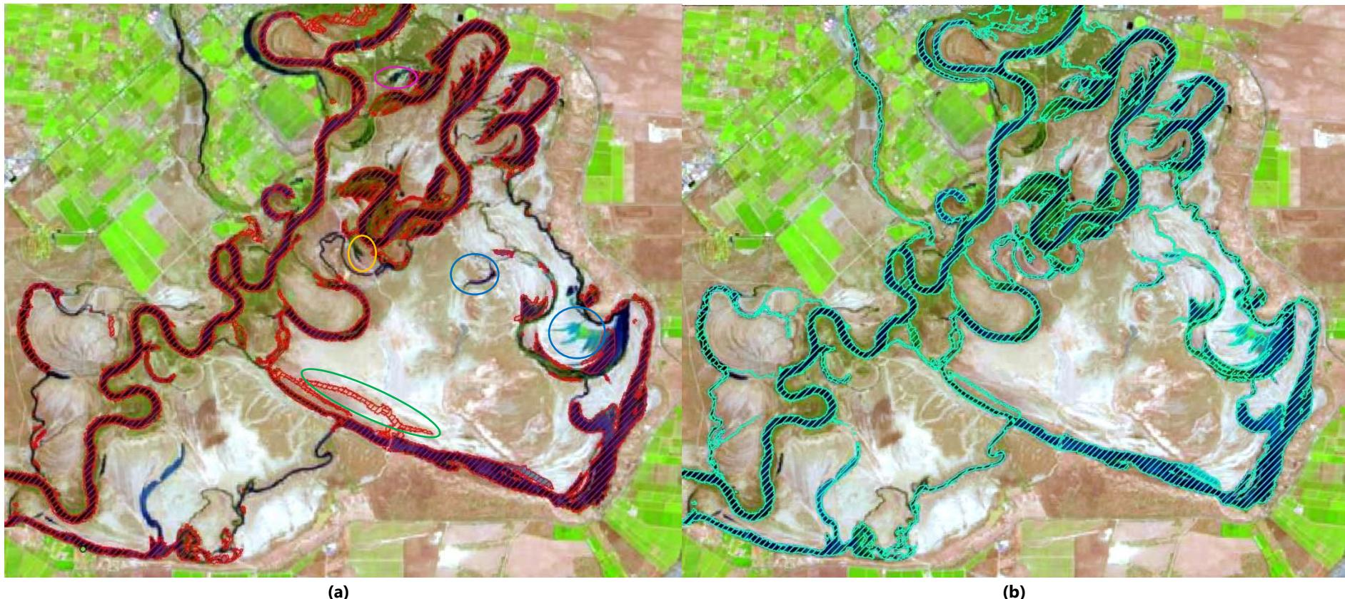
**Figure 3.8.** Pike imagery for 2 December 2020, compared to (a) base and (b) updated model outputs from simulation of 2020 event. Circled areas indicate discrepancy between observed and modelled.
