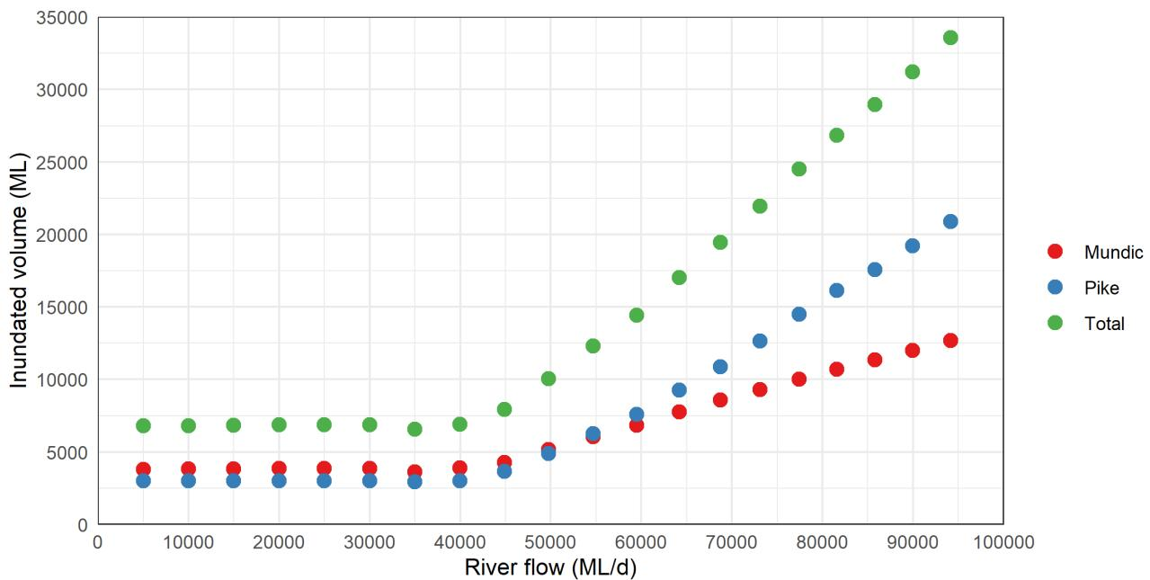
**Figure 3.25. Variation of storage volume upstream of the Pike blocking alignment with River Murray flow.**
