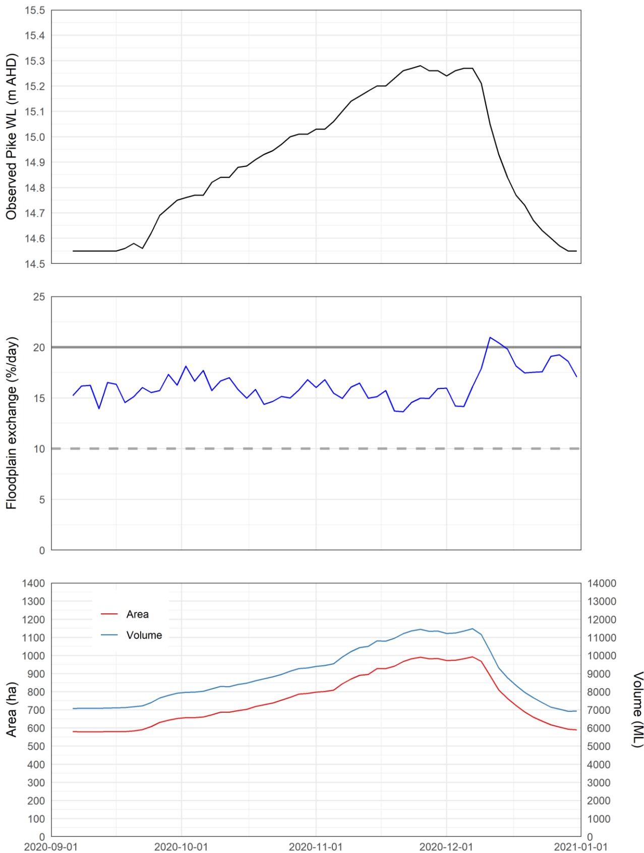
**Figure 3.21. Modelled daily exchange, inundated area and volume at Pike floodplain for 2020 event simulation.**
