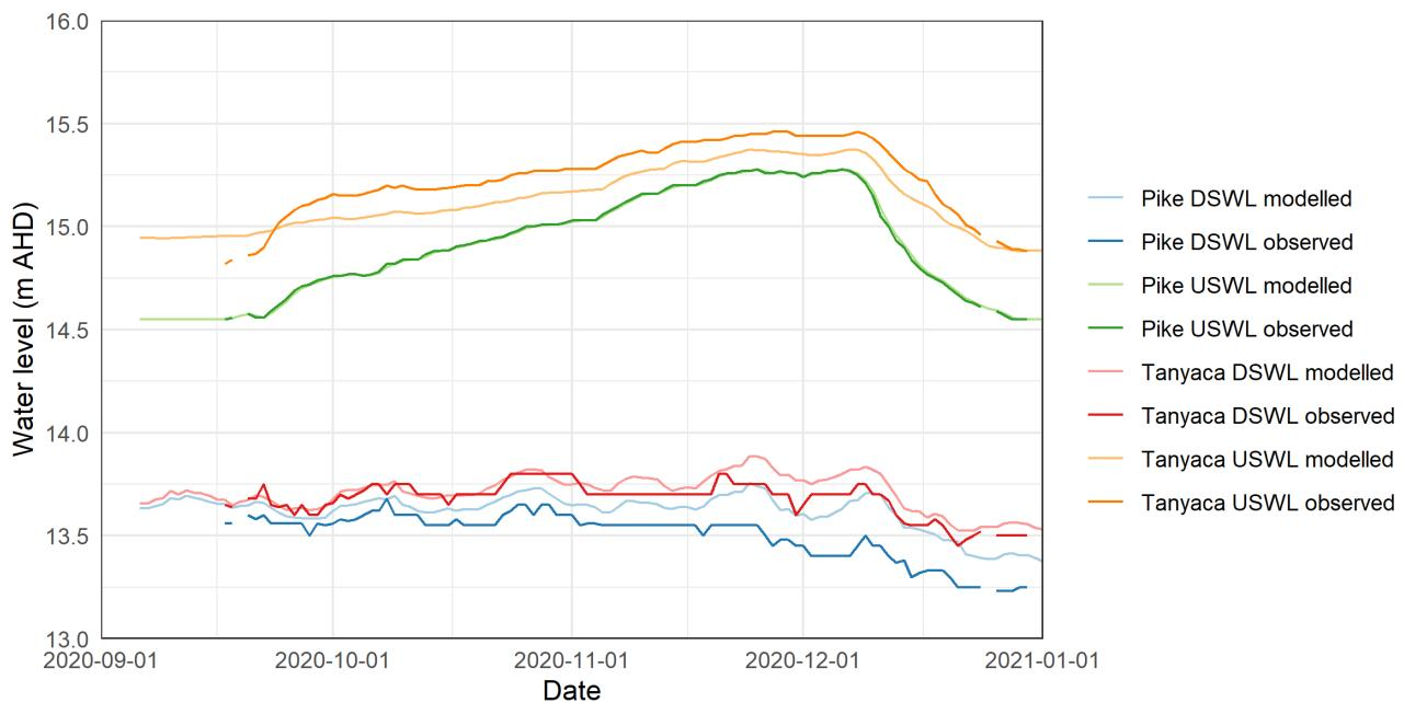
**Figure 3.15. Pike Floodplain environmental regulators, upstream and downstream levels, observed versus modelled.**
