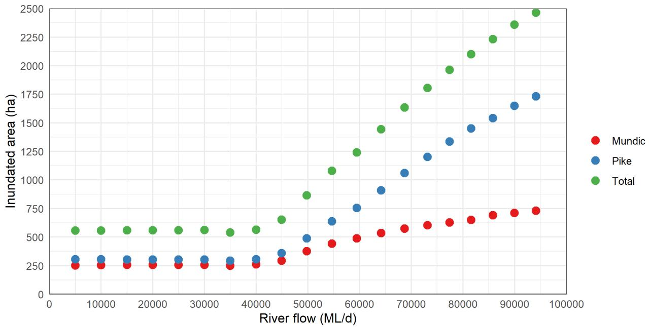
**Figure 3.24. Variation of inundated area upstream of the Pike blocking alignment with River Murray flow.**
