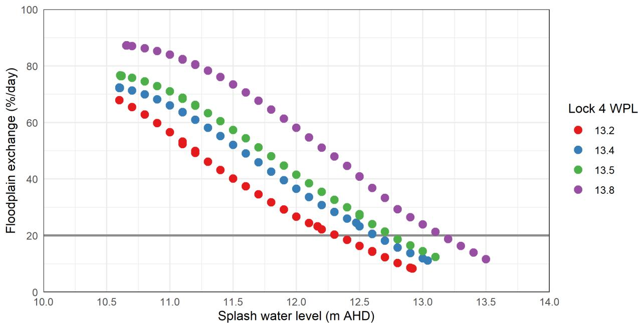
**Figure 3.37. Katarapko floodplain approximate maximum daily exchange versus The Splash regulator level and Lock 4 weir pool level, at QSA of 10 GL/d.**
