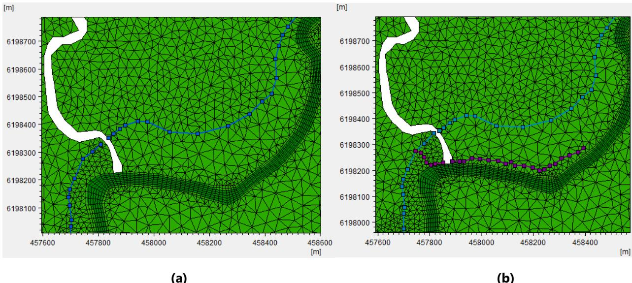
**Figure 6.5. Addition of dike structures at Piggy Creek tiered watering site, Katarapko Floodplain.**
