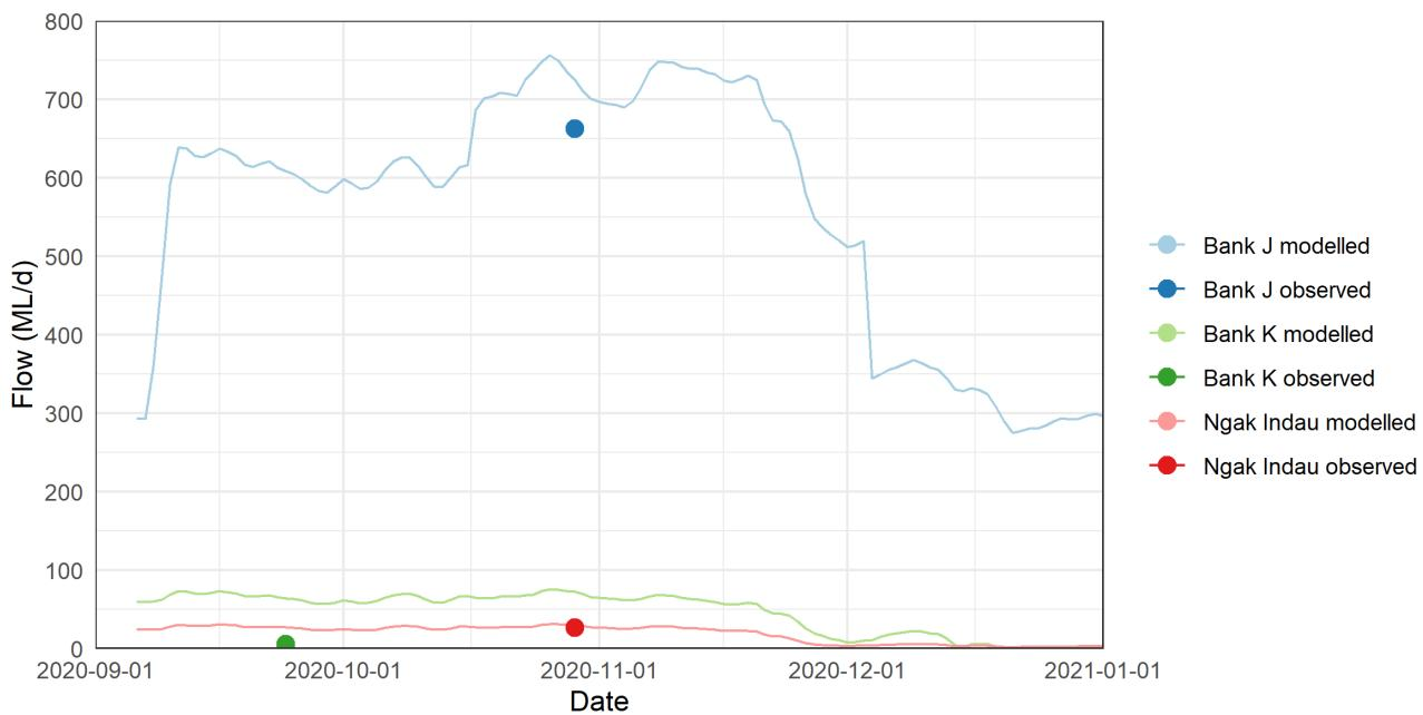
**Figure 3.17. Katarapko inlet flows comparison, gauged versus modelled.**
