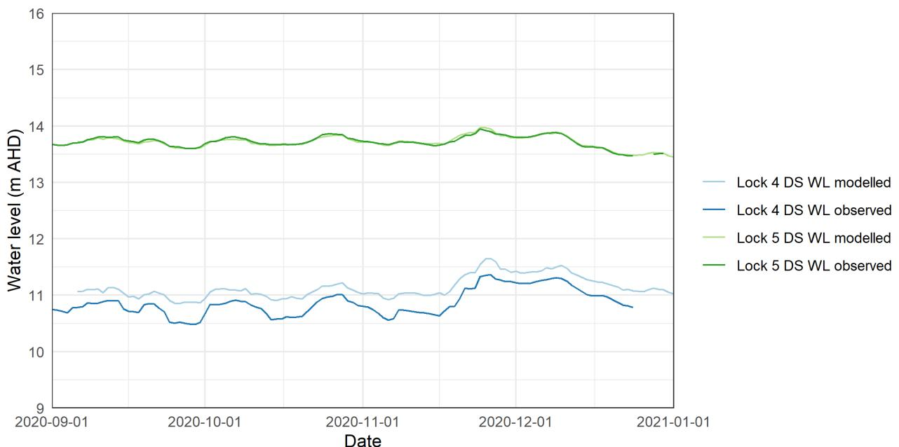
**Figure 3.10. River levels downstream of Locks 4 and 5 comparison, observed versus modelled.**
