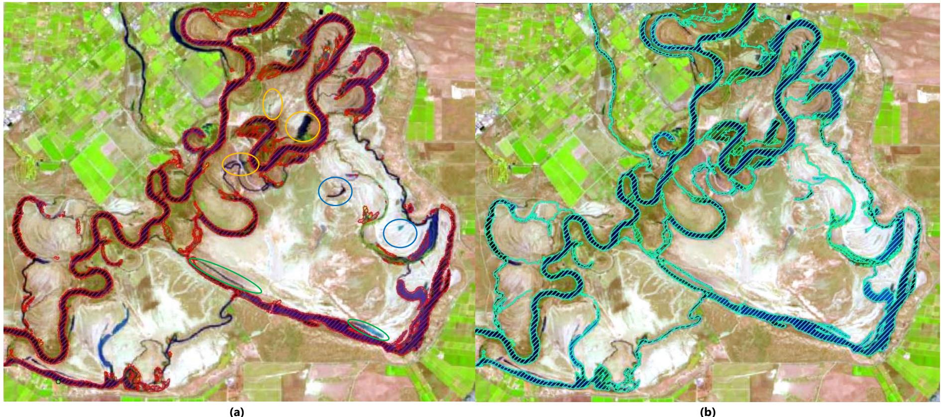
**Figure 3.5.** Pike imagery for 2 November 2020, compared to (a) base and (b) updated model outputs from simulation of 2020 event. Circled areas indicate discrepancy between observed and modelled.
