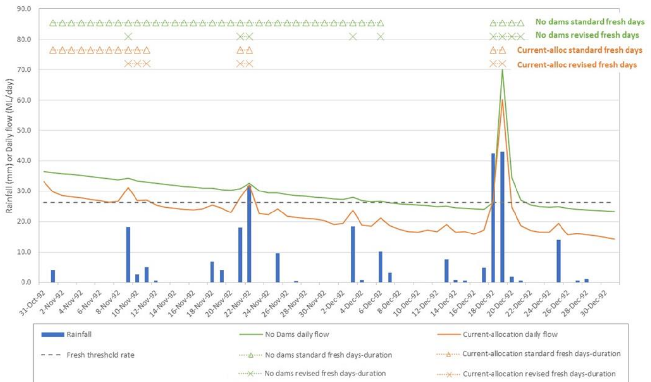
Figure 8. Rainfall, modelled daily flow and duration of standard and revised fresh events for Tookayerta zone 426TC005, for No-dams and Current-allocation (no LFR) scenarios, for T2 (transition high to low) flow season for 1992
