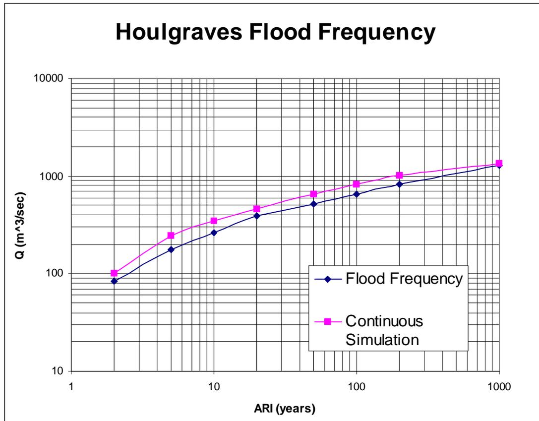
**Figure 2 Comparison of Houlgraves Log - Normal and Continuous Simulation Flood Frequency**
