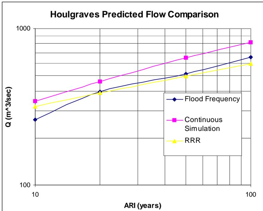
**Figure 6 Comparison of Houlgraves Flood Frequency, Continuous Simulation and RRR Flows (to 100 year ARI)**
