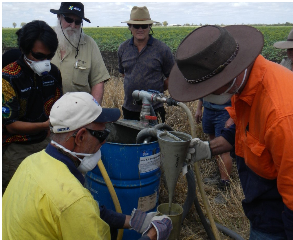
Measuring viscosity using a Marsh funnel
