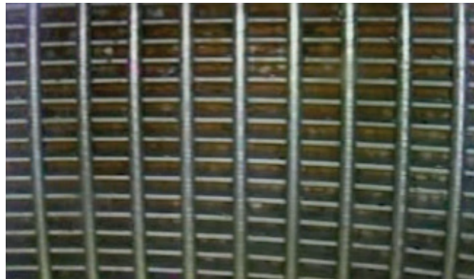
Downhole images of screens and gravel packs. Photos courtesy of Age Developments Pty Ltd
