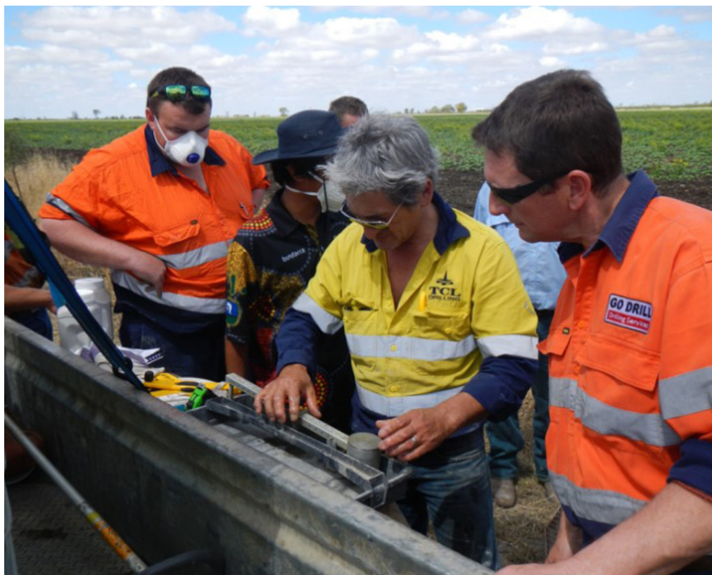
Measuring mud weights using a mud balance
