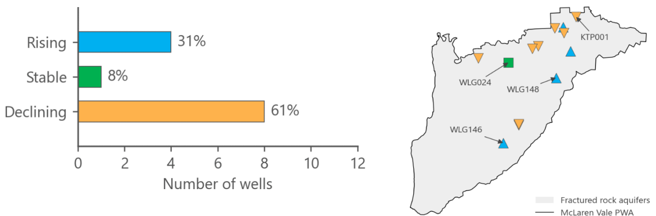
Figure 4.10 2015-2019 trend in recovered water levels for wells in fractured rock aquifers
