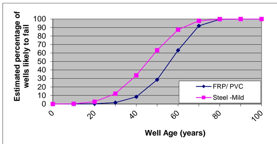
**Figure 1.1 Estimated effect of production casing type on failure rate of wells of varying age**
