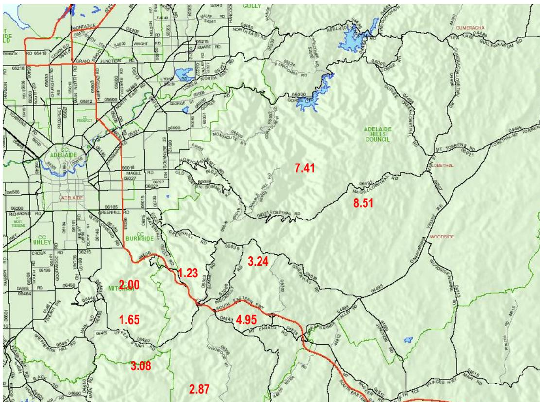
**Figure 10 Relative Magnitudes of 1:100 AEP Flows From Flood Frequency Analysis ( $1:100 \text{ AEP flow}/A^{0.73}$ )**
