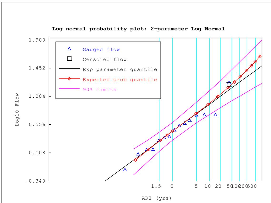
**Figure 9 Brown Hill Creek Flood Frequency Distribution**
