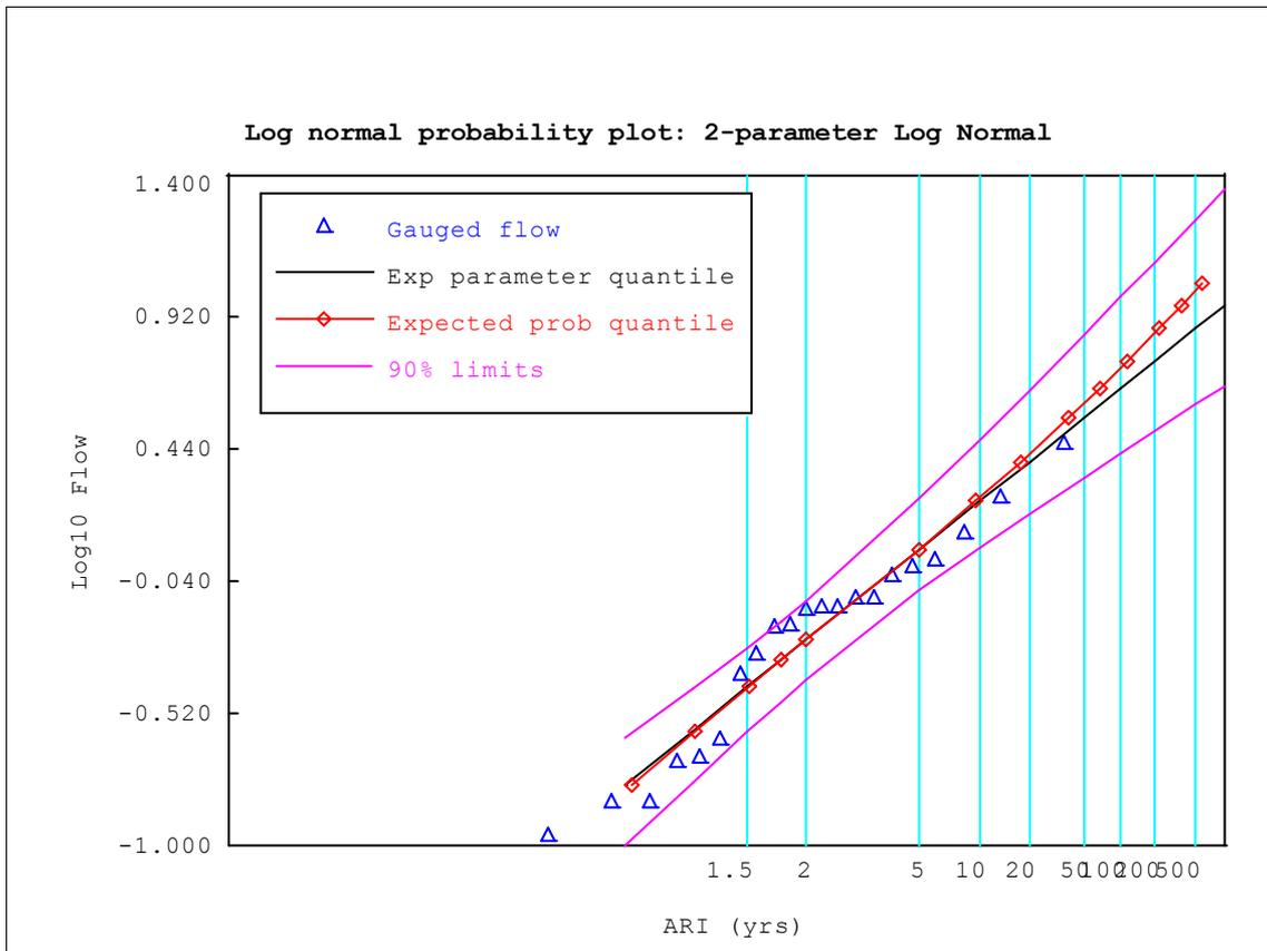
**Figure 7 First Creek Flood Frequency - 1983 Flood Excluded**
