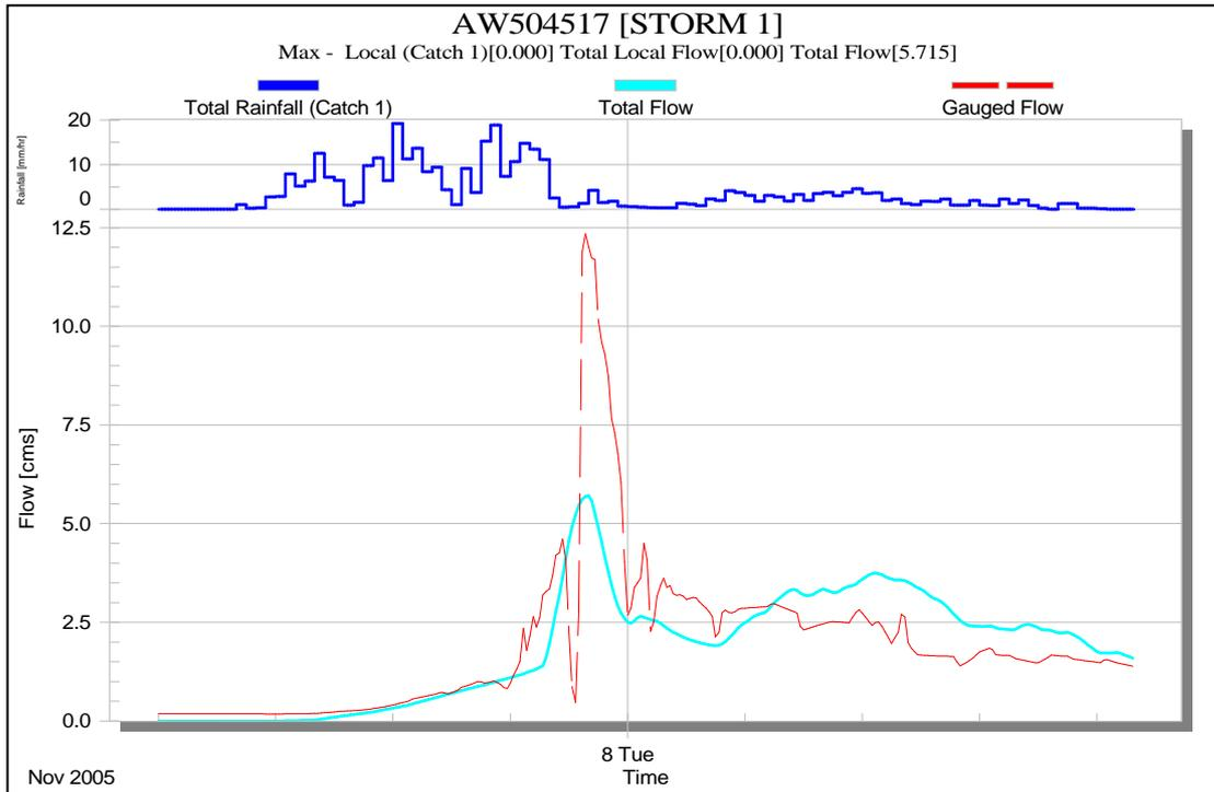
**Figure 18 First Creek at Waterfall - Total Runoff at Peak**
