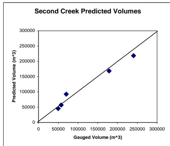
**Figure 3 Second Creek Stepney - Calibrated RRR Model Fit**
