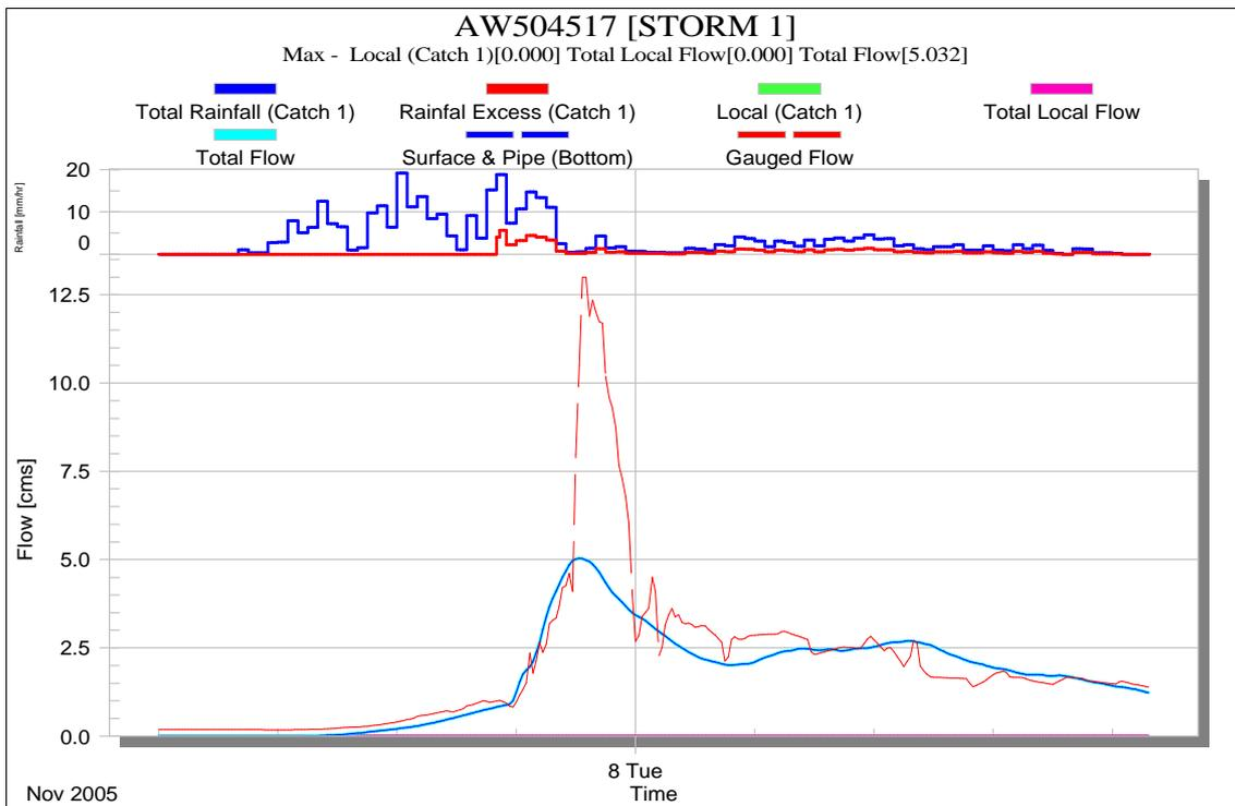
**Figure 19 First Creek at Waterfall - Detailed Model**
