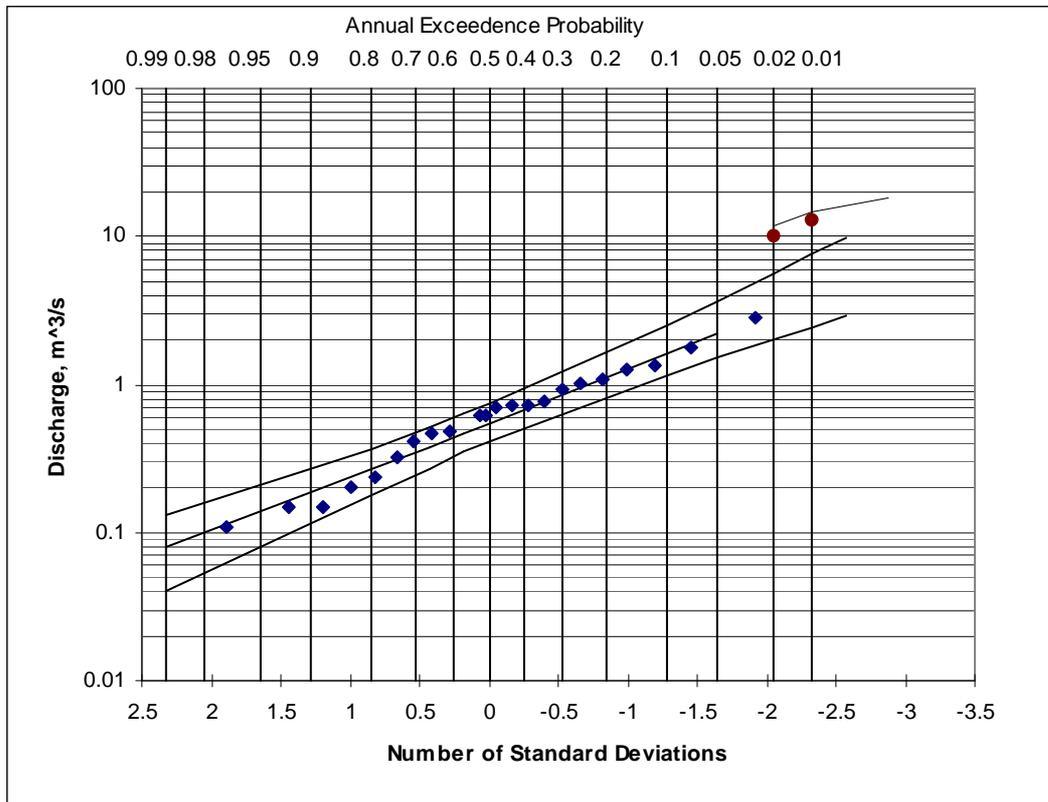
**Figure 21 Flood Frequency Analysis First Creek at Waterfall – With Split Distribution**
