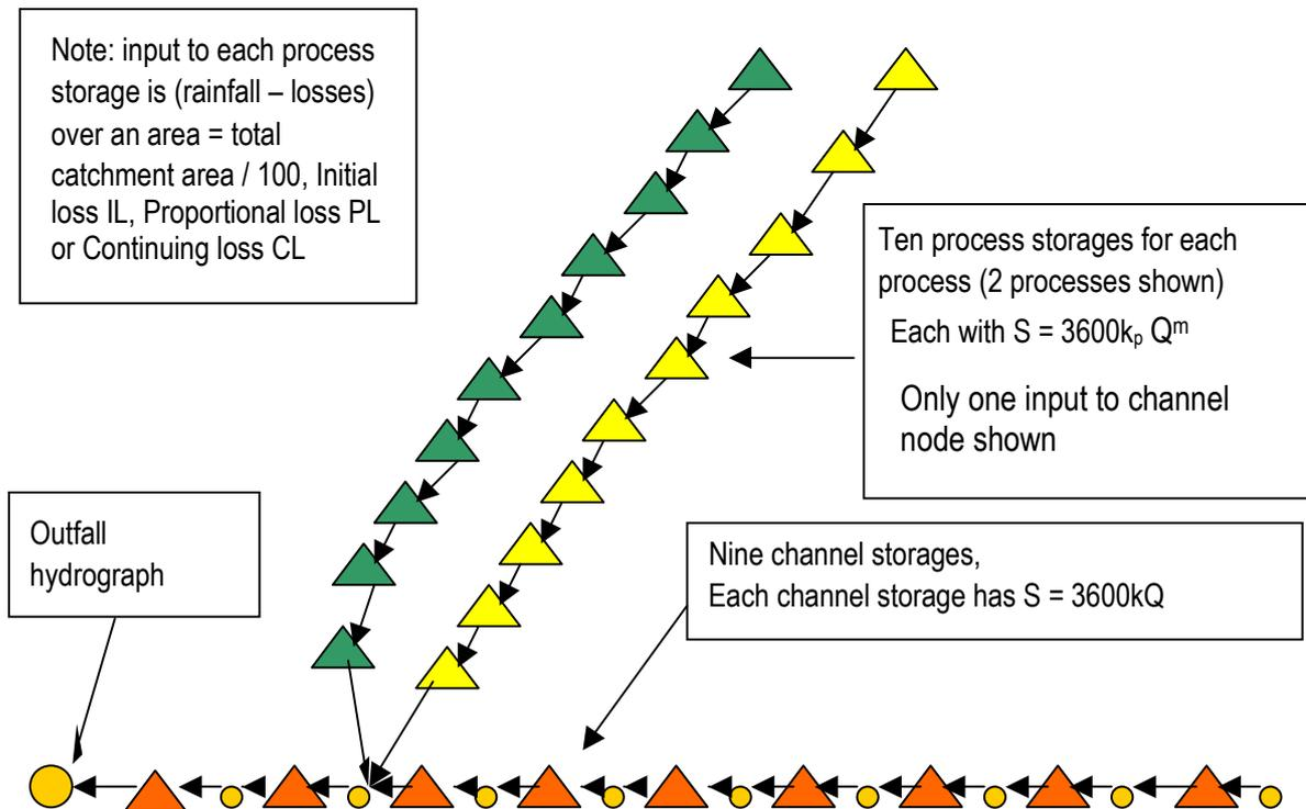
**Figure 1 Structure of the RRR Model**
