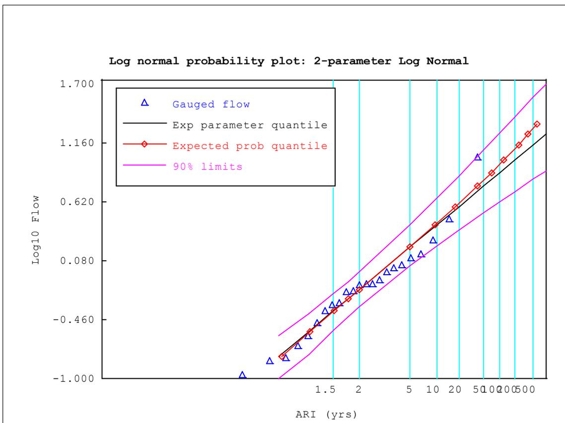
**Figure 6 First Creek Flood Frequency - 1983 Flood Included**
