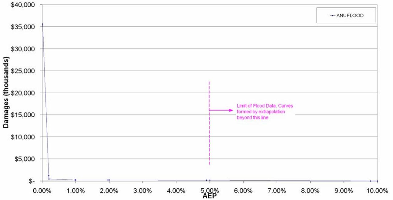
Figure 2-5 Existing Condition Probability Damages Curve (Fifth Creek)
