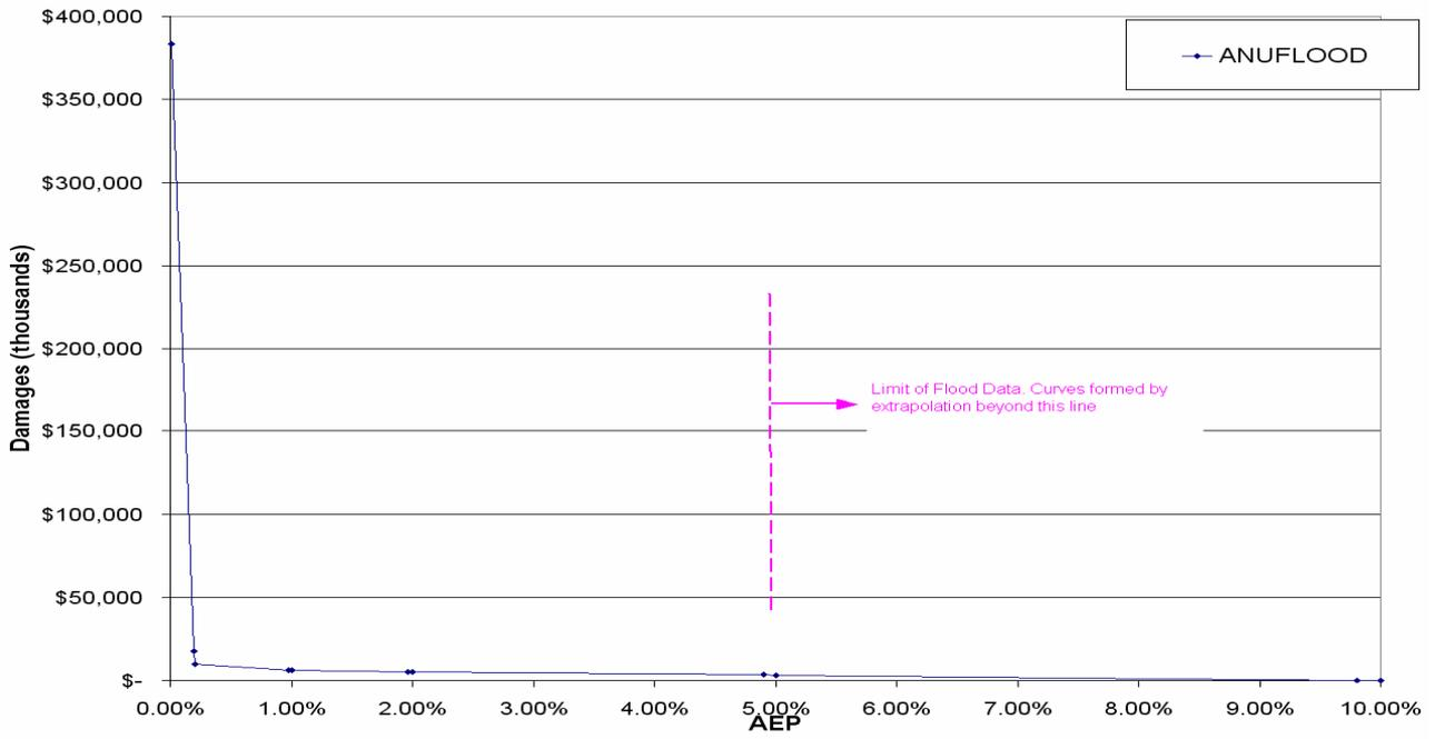
Figure 2-3 Existing Condition Probability Damages Curve (Third Creek)
