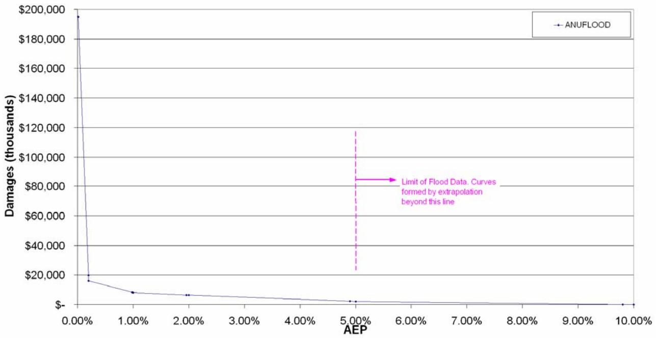
Figure 2-1 Existing Condition Probability Damages Curve (First Creek)
