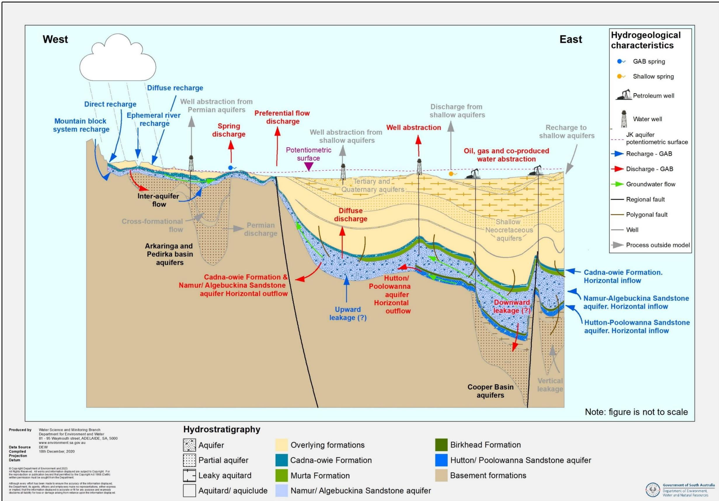
**Figure 7.2: Schematic conceptual cross-section of recharge and discharge processes interpreted to occur within the study area**
