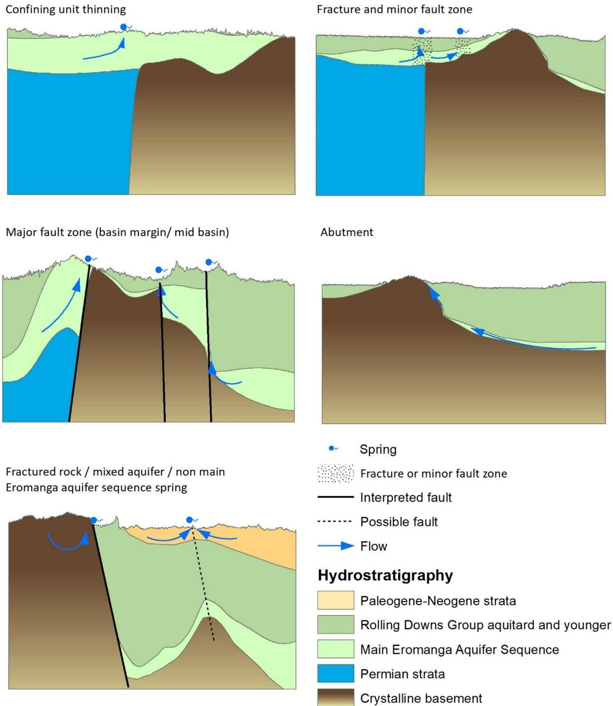
**Figure 4.1: Schematic diagrams of various geological classifications**
