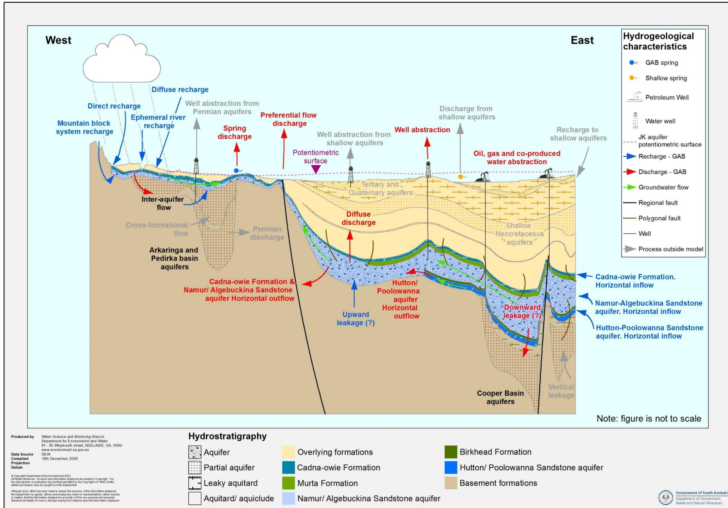
• **Figure 2:** Schematic conceptual cross-section of recharge and discharge processes interpreted to occur within the study area
