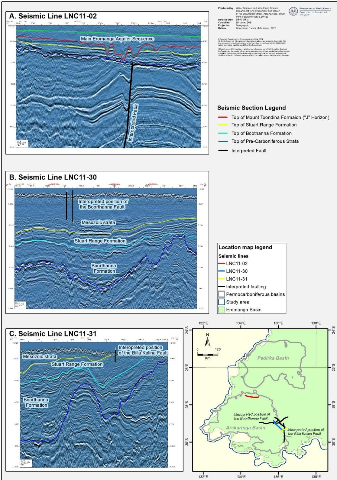
**Figure 5.5: Selected seismic lines from within the study area. One shot point is approximately 30 metres. A) Section across the northern margin of the Boothanna Trough. B) and C) Interpreted seismic reflection section across the previously interpreted positions of the Boothanna and Billa Kalina Faults)**
