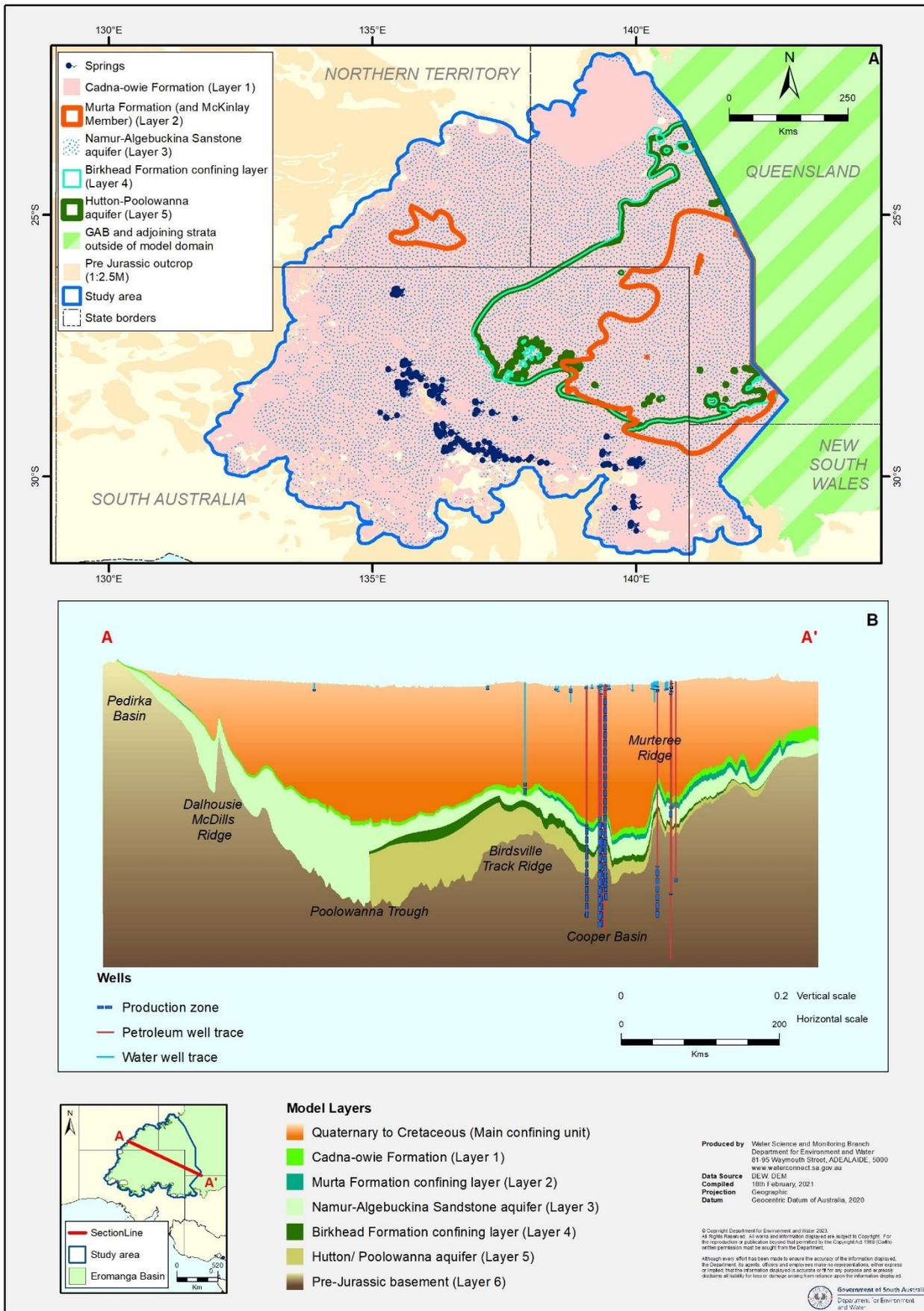
**Figure 2: A) Plan view of structure surface outlines used in numerical model. B) Cross-section through study area showing model layers and key structures**
