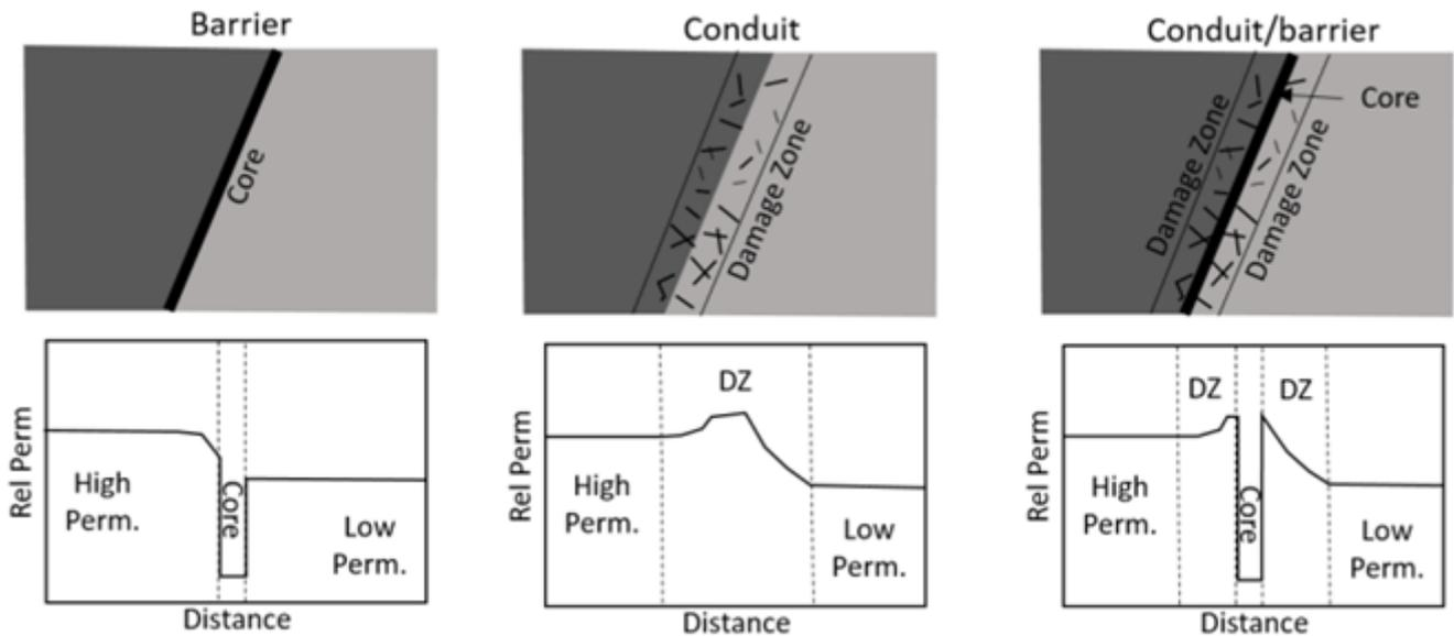
**Figure 7.1: Schematic description of a fault, highlighting the fault core and damage zone and its relationship to porosity and permeability differences**
