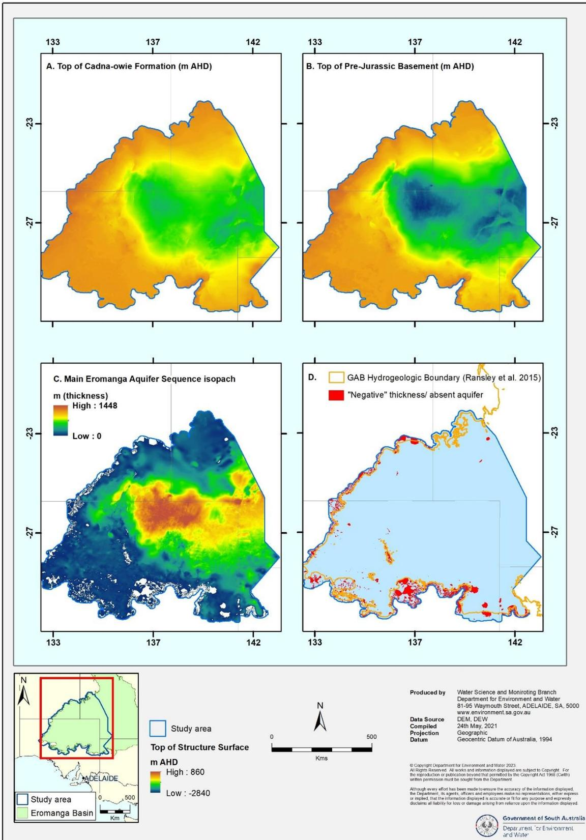
**Figure 6.1: Intra-aquifer structure surfaces developed for study area. A) Top of the Cadna owie Formation (layer 1). B) Top of the Pre-Jurassic Basement (layer 6). C) Isopach of the Main Eromanga Aquifer Sequence. D) Structure surface quality control data indicating where a “negative” thickness exists, indicative of an absence of Main Eromanga Aquifer Sequence strata.**
