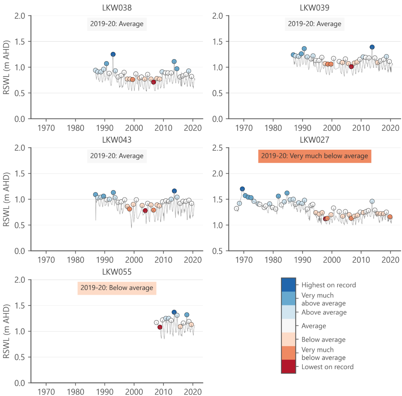
Figure 4.13. Selected hydrographs for wells in the QL aquifer in the Coffin Bay Consumptive Pool
