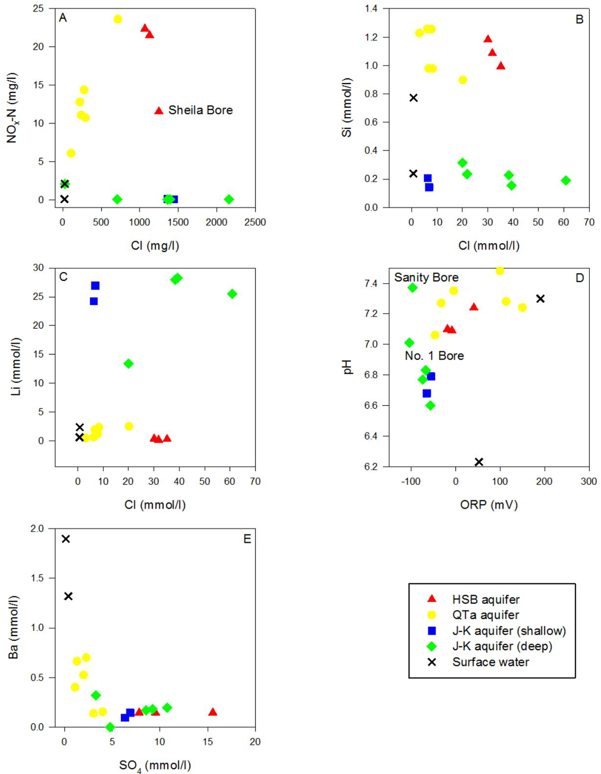
**Figure 4-1: Scatter plots of A) Cl<sup>-</sup> (mg/l) vs NO<sub>x</sub>-N (mg/l), B) Si (mmol/l) vs Cl (mmol/l), C) Li (mmol/l) vs Cl (mmol/l) D) pH vs ORP (mV) and E) Ba (mmol/l) vs SO<sub>4</sub> (mmol/l)**
