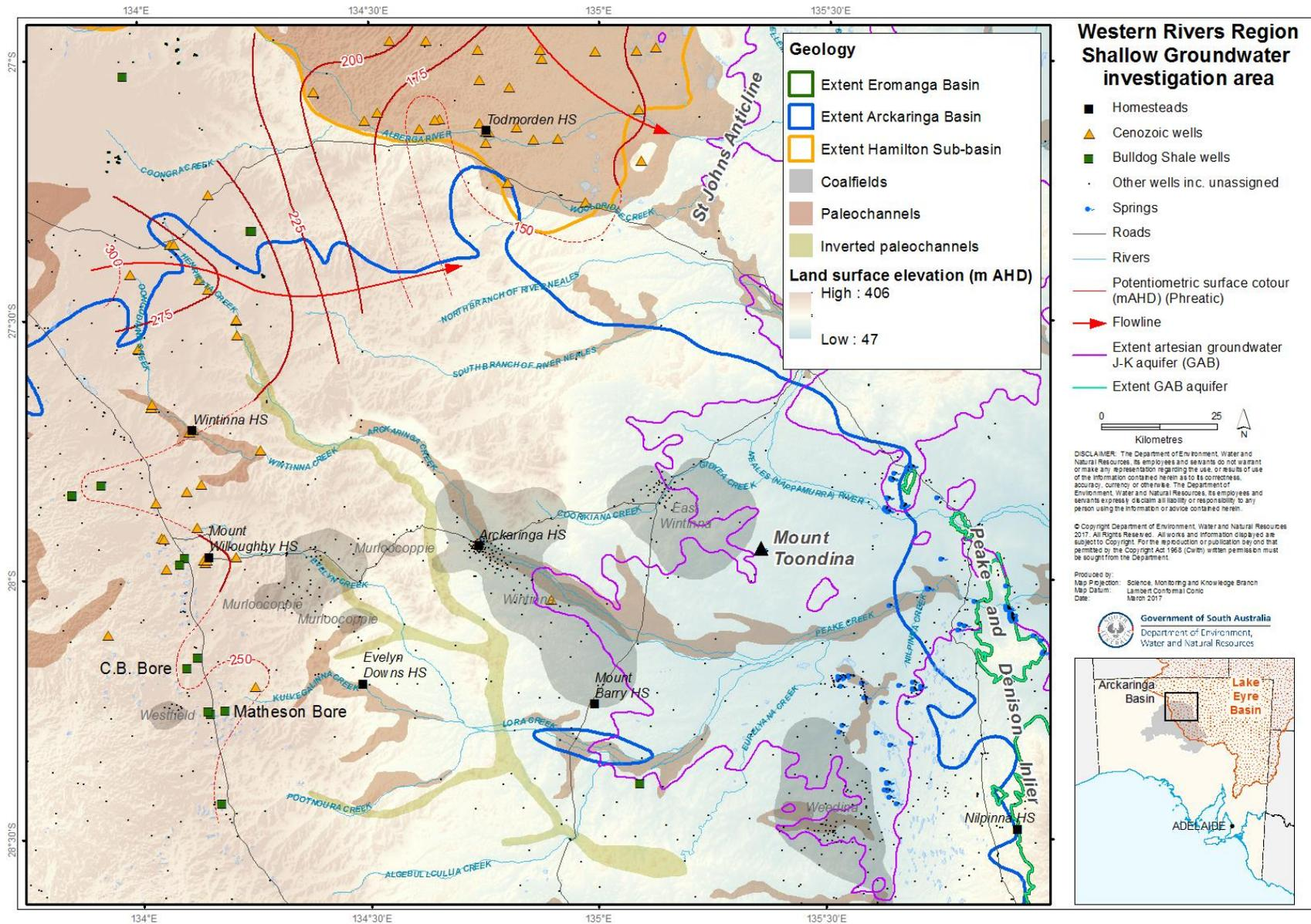
**Figure 2-5: Potentiometric surface contour interpretation of phreatic groundwater based on reduced standing water level (RSWL) (m AHD) data**
