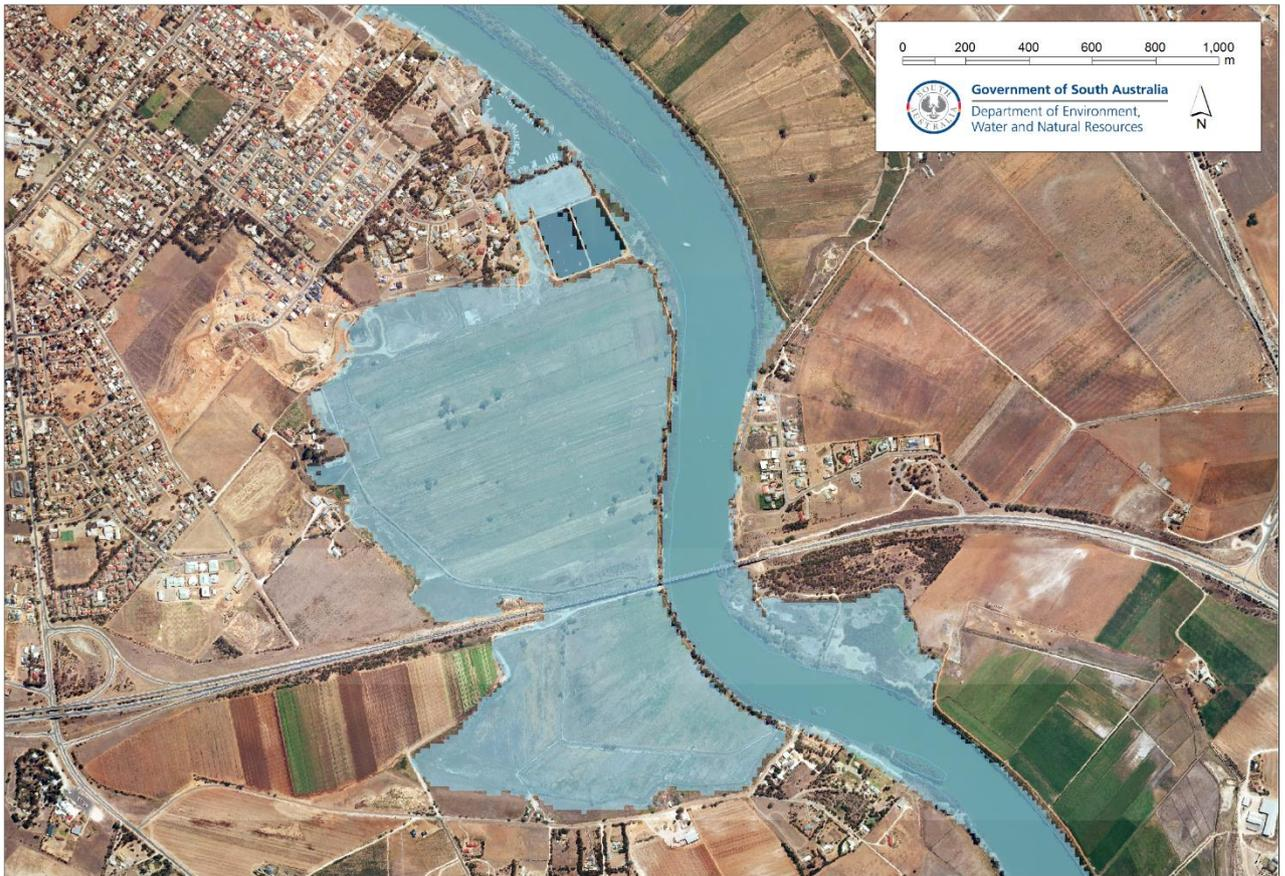
**Figure 4.2** The modelled flood extent indicates where widespread inundation occurs behind localised overtopping of levee banks (120,000 ML/d flood at Murray Bridge)
