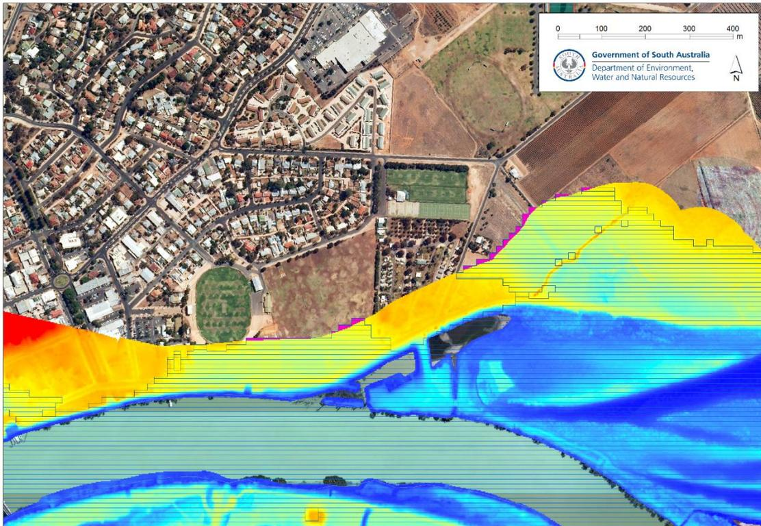
**Figure 4.1 Pink shading indicates where the flood extent has reached the edge of the DEM (1956 flood at Berri) (colour shading is floodplain DEM, hatched is inundation extent)**
