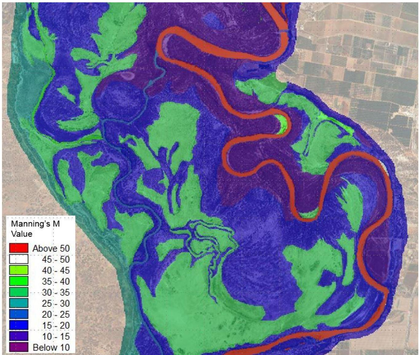
**Figure 3.2 Example of a roughness coefficient map**
