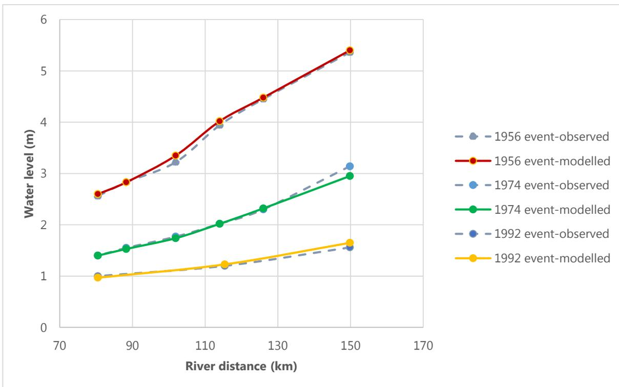
**Figure 3.3 Modelled and recorded water levels for Model Section 1 Wellington to Mannum**
