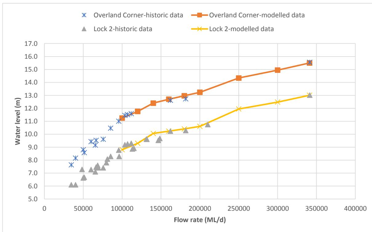
Figure 3.5 Rating curves for Lock 2 and Overland Corner
