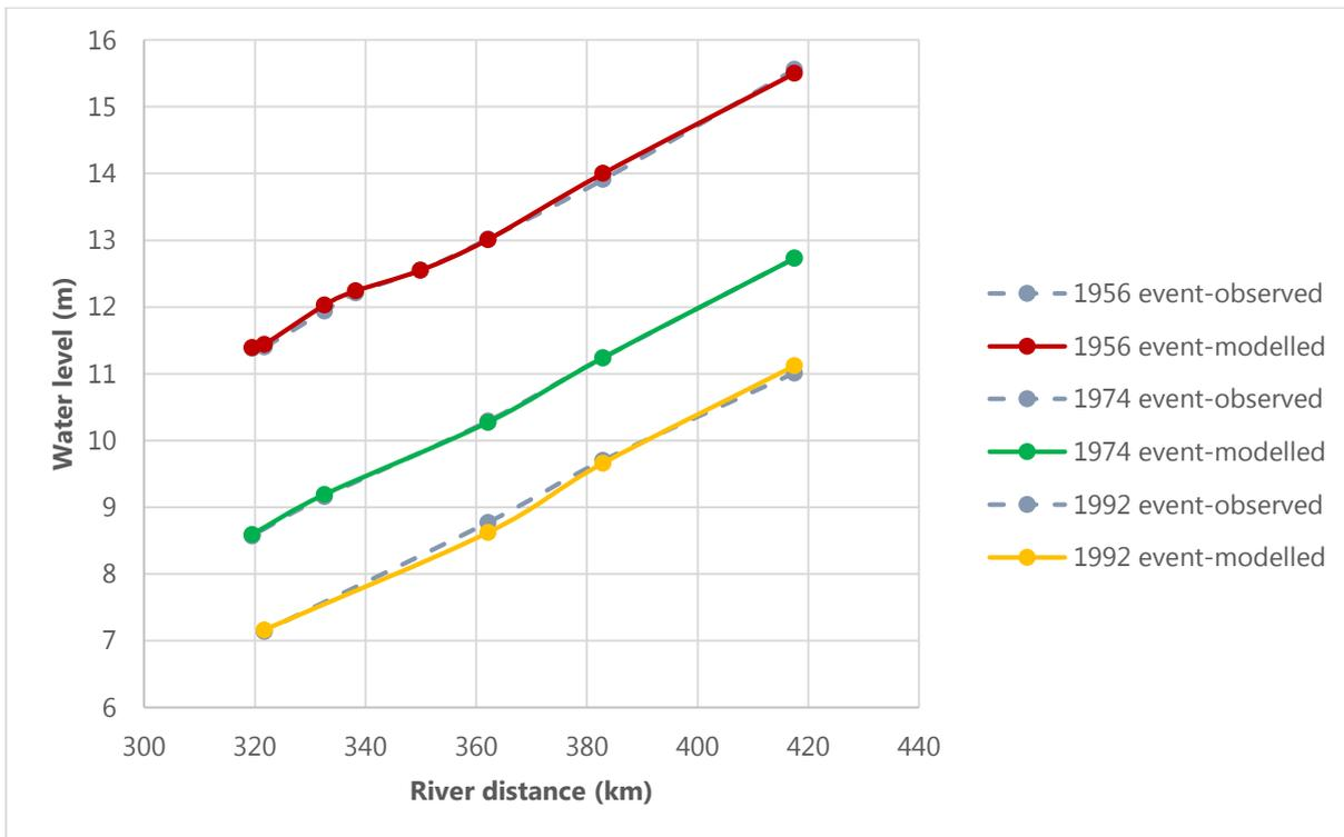
**Figure 3.4 Modelled and recorded water levels for Model Section 4 Morgan to Overland Corner**
