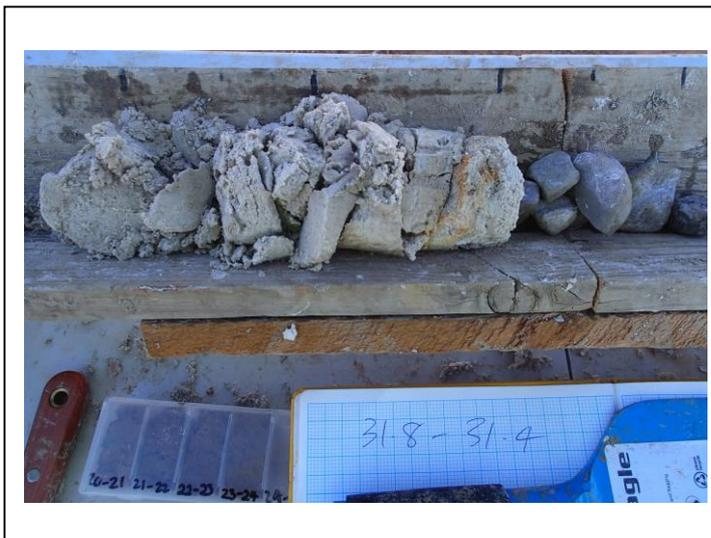
J-K aquifer (31.4-31.8 m): SAND, light grey with orange-brown mottling, medium to coarse grained quartz sand, sub-angular quartz and sandstone gravels < 50 mm.
