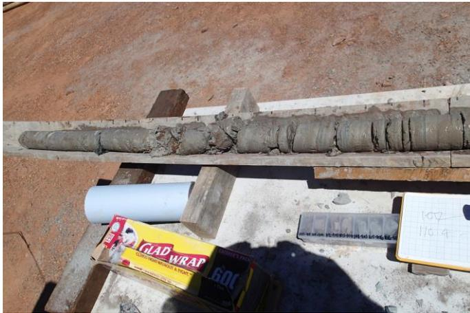
Boorthanna Formation (107.4-110.4 m): SANDSTONE, light grey with white sand, medium to coarse grained sand lenses of variable and uncertain thickness, light grey and grey wavy bedding, trace dark grey claystone 10 mm thick interbeds, fine to coarse grained sand, moderate percentage of sub-rounded to sub-angular granitic gravels < 15 mm, pyritic inclusions adjacent to gravels, pyritic gravels, poorly sorted.
