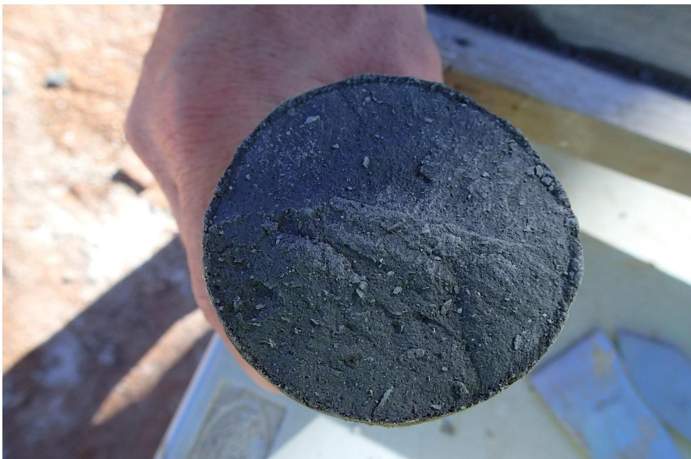
**Figure 3-4 Core sub-portion from interval 47–48.5 m BGS, showing the outer 1–2 mm impacted by drilling fluids (darkened)**
