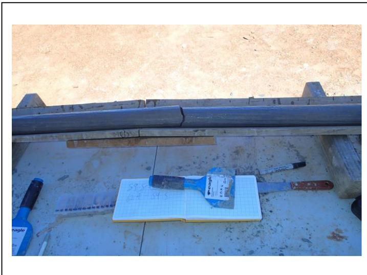
Stuart Range Formation (59.5-62.4 m): CLAYSTONE, grey, consolidated, trace fine to medium grained sand, trace sub-rounded to sub-angular quartz and sandstone gravels < 50 mm.
