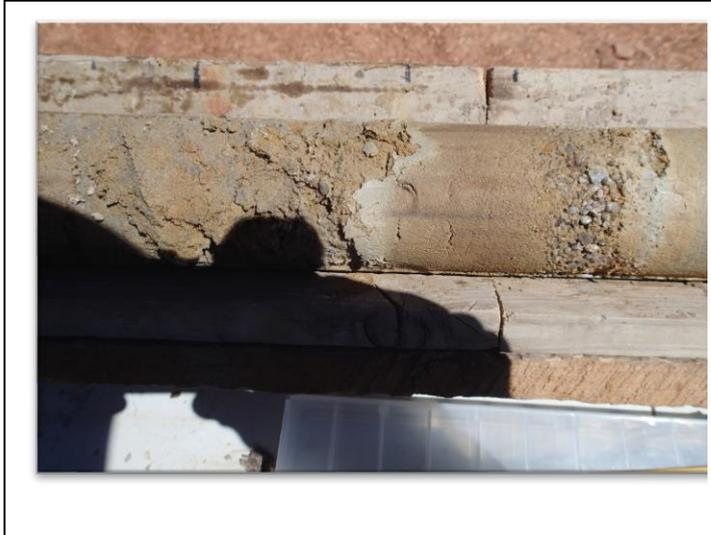
J-K aquifer (18-19.4 m): SAND, grey with orange-brown mottling, increase in fine to medium grain, some coarse grains (fining downwards), poorly sorted, trace clay, trace sub-rounded quartz gravel < 25 mm.
