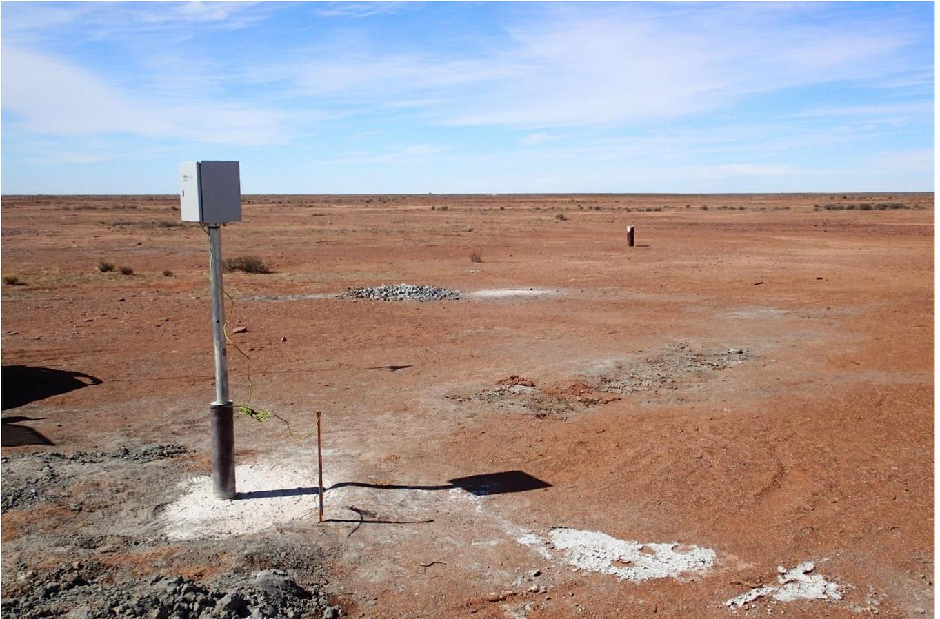
**Figure 3-3 6038-519 VWP datalogger box, with groundwater monitoring well RMS-7 (formerly VMS-2) in the background**
