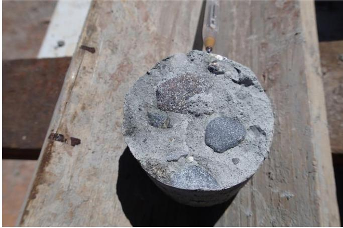
Boorthanna Formation (106.6-107 m): SANDSTONE, grey, fine to coarse grained sand, moderate percentage of sub-rounded to sub-angular granitic gravels < 15 mm, pyritic inclusions adjacent to gravels, pyritic gravels, poorly sorted.
