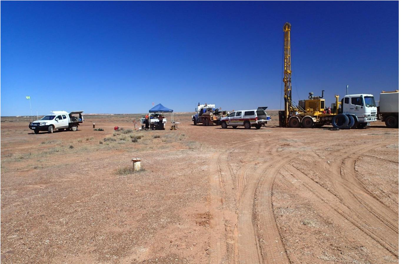
**Figure 3-2 Boart Longyear LF90 rig and support vehicles during drilling**
