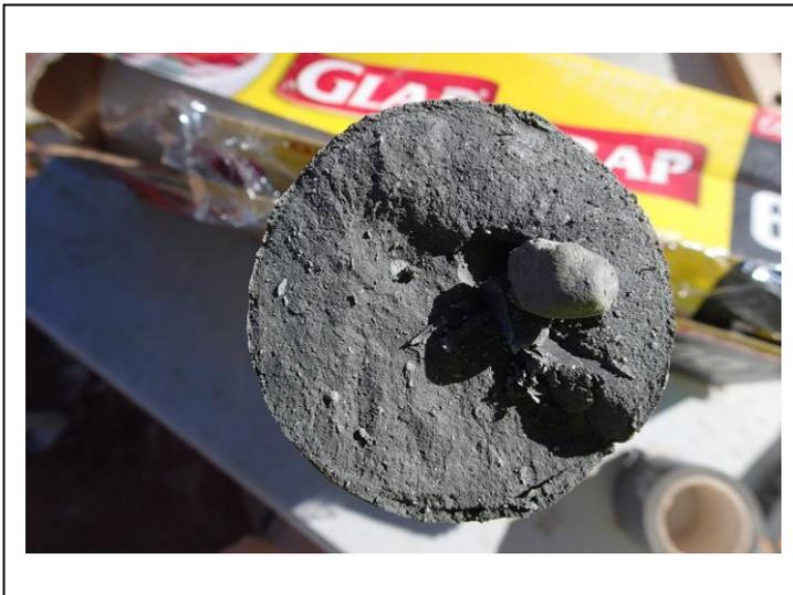
Stuart Range Formation (47-48.5 m): CLAYSTONE, grey with trace orange-brown mottling, consolidated, trace sand, trace sub-rounded to sub-angular quartz and sandstone gravels < 10 mm.
