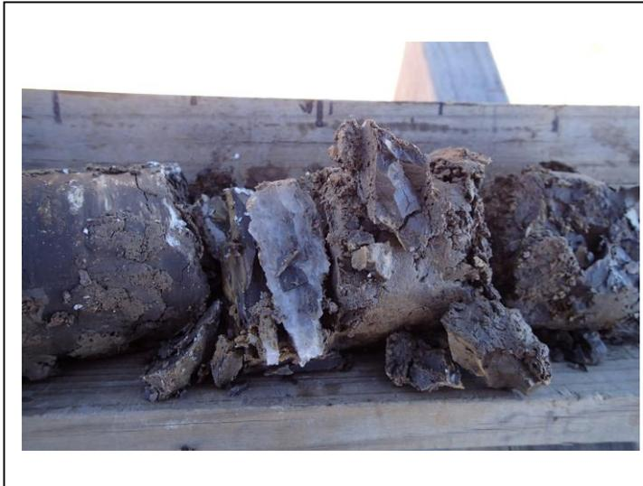
Bulldog Shale (12.4-14.4 m): CLAY, dark grey-brown with increased yellow and red-brown mottling, medium to high plasticity, friable, but becoming less friable with depth, blocky, less frequent white gypsum crystal veining < 3 mm, trace sand.
