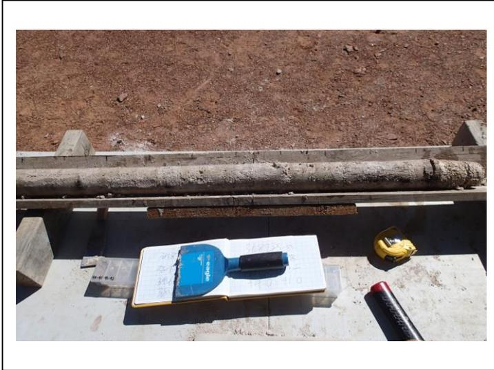
J-K aquifer (41-44 m): SAND, white-light grey, medium to coarse grained, trace sub-angular quartz gravels < 20 mm, trace clay.
