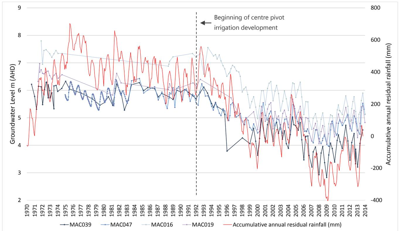
**Figure 4.1** Groundwater levels in long-term monitoring wells up-gradient of the Middlepoint Swamp GDE case study site, compared with accumulative annual residual rainfall
