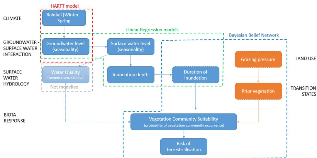
**Figure B The conceptual model of hydrological function for Middlepoint Swamp, and modelling approach**
