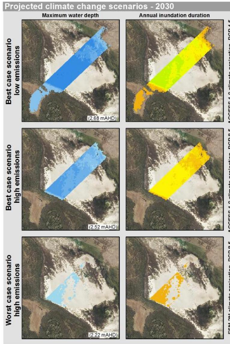
**Figure 4.6 Spatial representation of predicted surface water level extent, depth and duration for 2030 climate change scenarios at Middlepoint Swamp. Surface water levels in m AHD indicated for each scenario**
