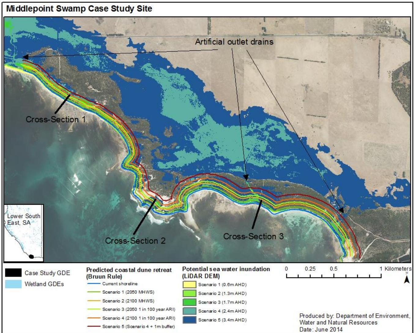
**Figure 3. Results of Bruun Rule calculations of coastal dune retreat from sea level rise scenarios. Concentric coastal lines indicate dune retreat. Potential sea water inundation extent displayed using 2 m LiDAR DEM**
