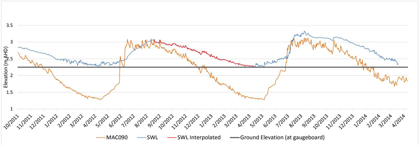
**Figure 4.3 Surface water (SWL) and groundwater (MAC090) hydrograph for Middlepoint Swamp collected as part of the GDE monitoring project (DEWNR)**
