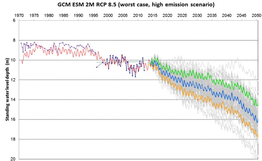
Projected groundwater levels: 90th percentile (orange line), Average (blue line), 10th percentile (green line)
