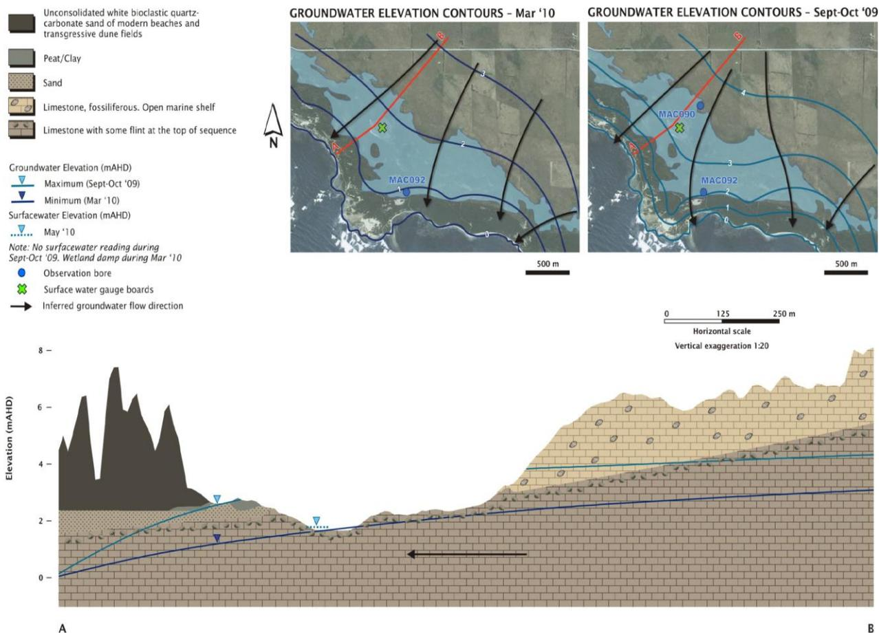
**Figure 3.3 Middlepoint Swamp conceptual diagram of groundwater interaction with the TLA for the 2009-10 monitoring period (sourced from SKM 2010)**
