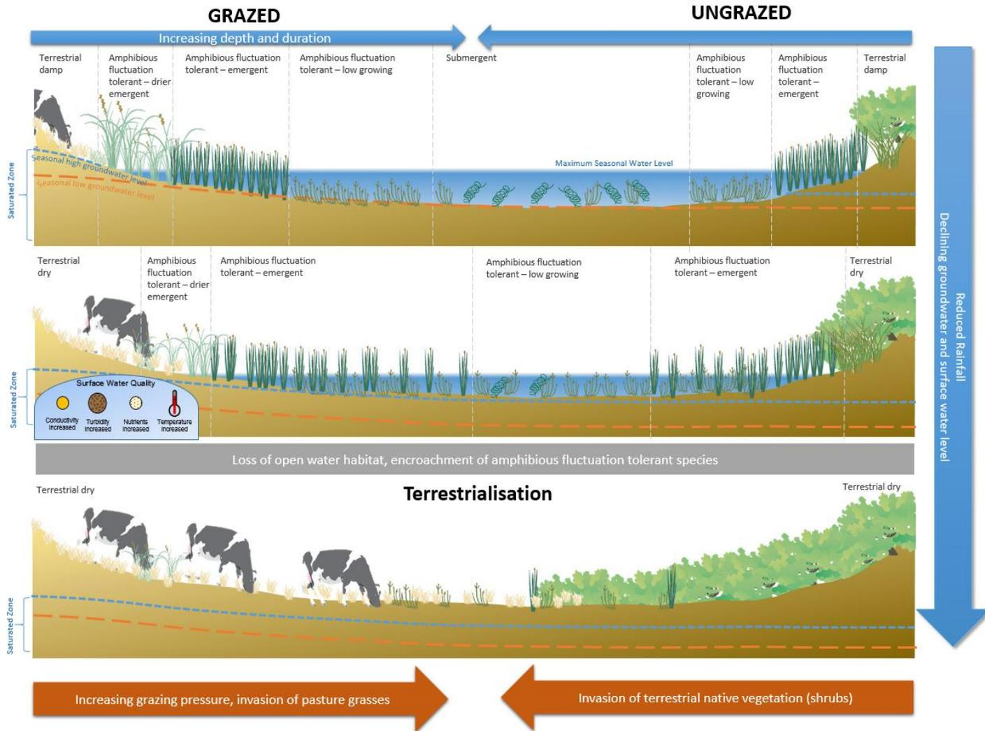
**Figure 4.10** Conceptual diagram of the impact of hydrological change on vegetation communities along a cross-section of Middlepoint Swamp, depicting current and future groundwater level scenarios
