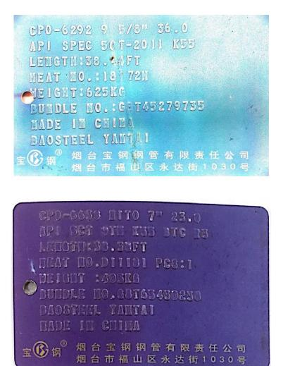
Figure 5. Tags from artesian control and production casing
