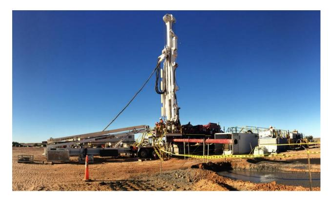
Figure 4. Rod loading, blooey line and mud system used for Mulka Bore No. 2
