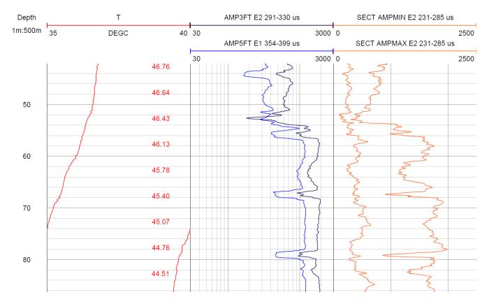
Figure 8. Initial tremie cement bond log results from 21 April 2016. The bottom of the tremie line cement job was picked at 67 m based on coincident rises in the AMP3FT, AMP5FT, and maximum radial (SECT) receiver amplitudes. The regular drops in amplitude at 168, 178.5, 189.5, and 200 m are casing joints.
