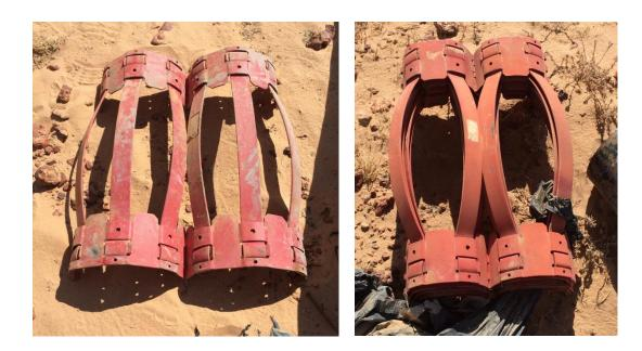
Figure 6. Centralizers used for artesian control casing (left) and production casing (right)
