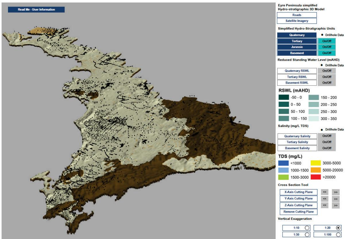
Figure 6. EP hydrostratigraphic unit thickness (1:20 vertical exaggeration)
