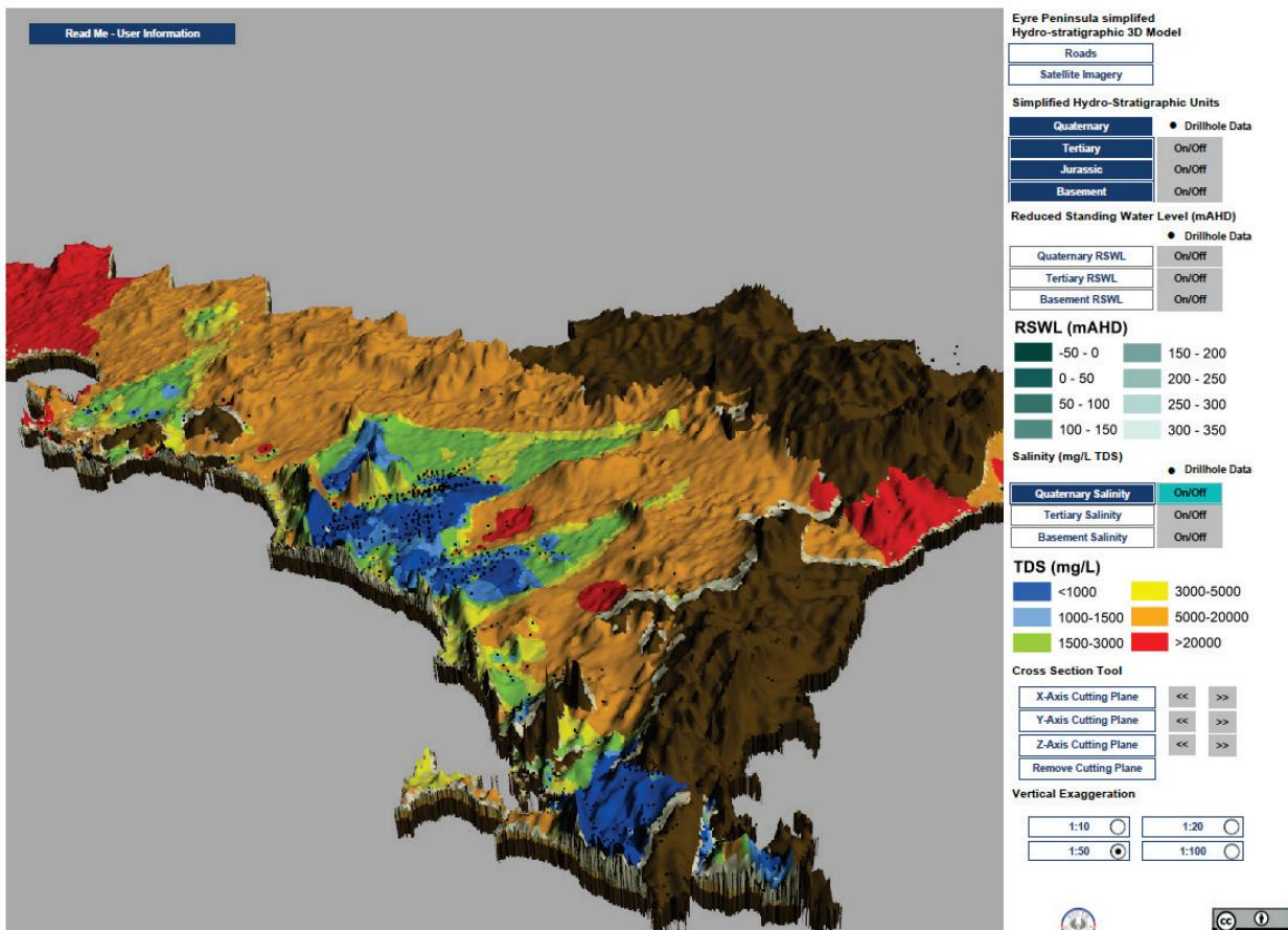
Figure 7. Salinity of EP Quaternary hydrostratigraphic unit (1:50 vertical exaggeration)
