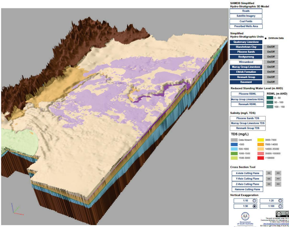
**Figure 12. SA MDB hydrostratigraphic unit thicknesses (1:50)**
