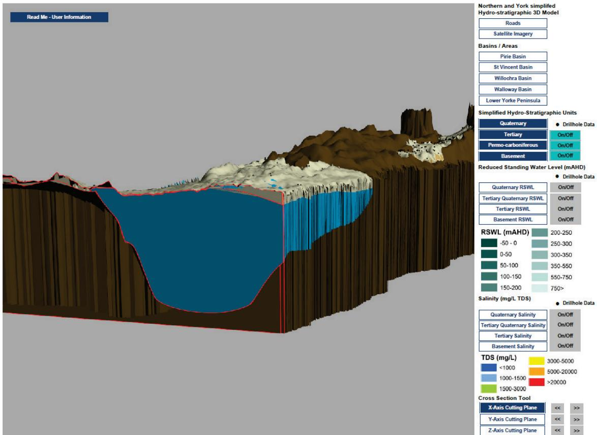
Figure 9. Cross Section displaying NY Permian hydrostratigraphic thickness (1:50 vertical exaggeration)
