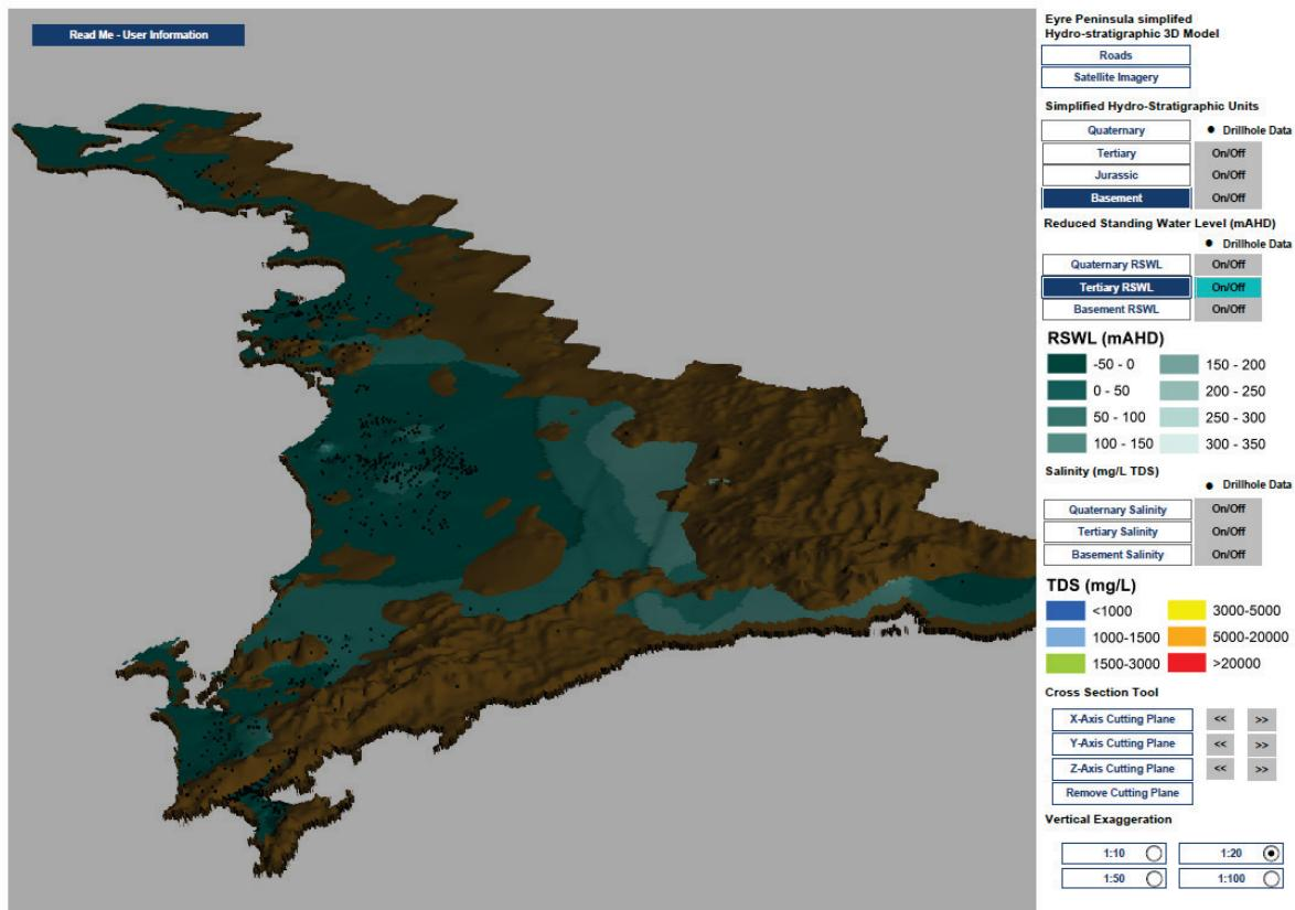
Figure 8. EP Tertiary RSWL water elevation surface (1:20 vertical exaggeration)
