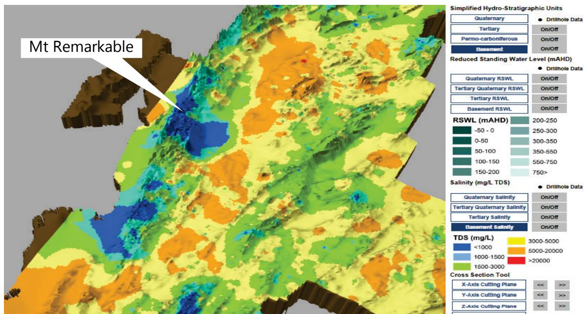
**Figure 15. Zones of fresh groundwater zones in the basement aquifer around Mt Remarkable**
