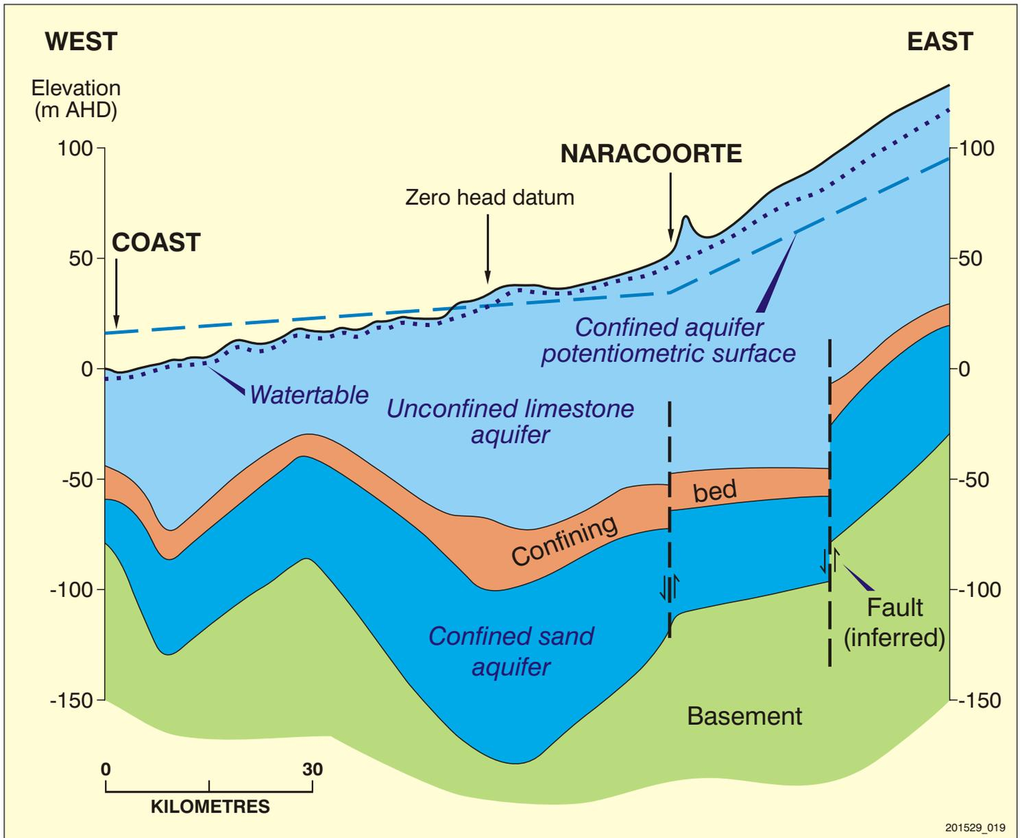
Figure 3 Schematic cross-section of southeast groundwater.
