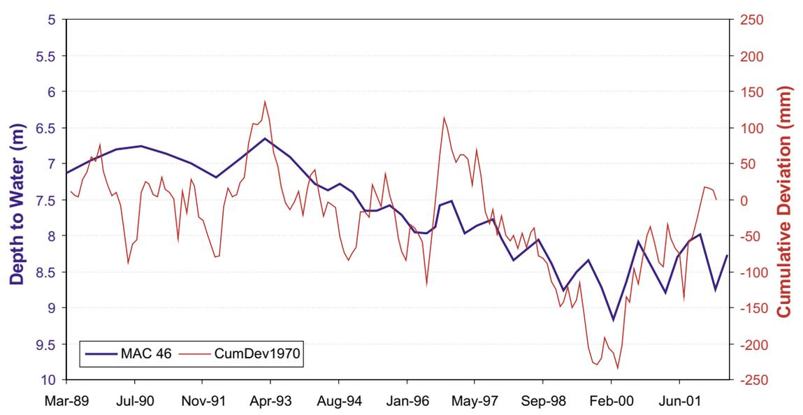
**Figure 12** Unconfined aquifer hydrographs compared to cumulative deviation (taken from data collected in 1970)
