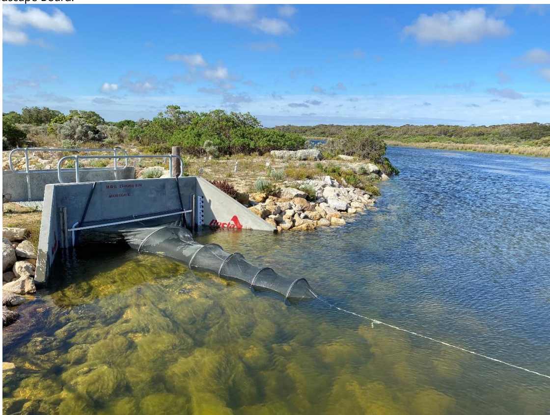
Figure 1: A fyke net being used at the Morella Creek fishway in the South East to monitor fish moving between the South East Drainage network and the Coorong (Qifeng Ye, SARDI)
