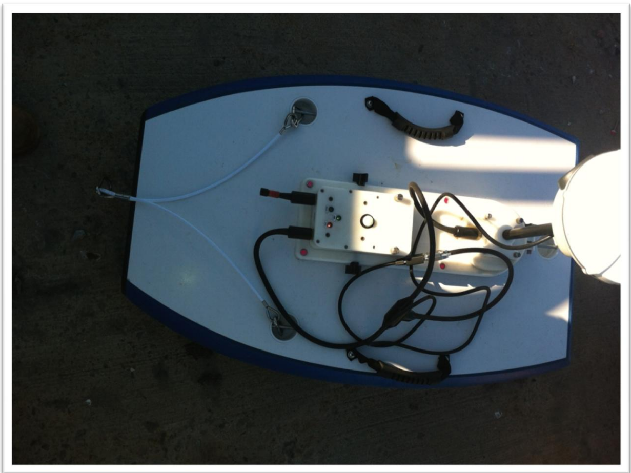
Fig.2 YSI M9 with RTK rotor head
