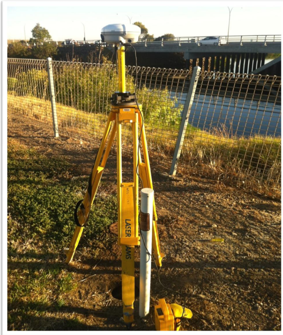
Fig.4 RTK Base Station setup at Benchmark 66287679
