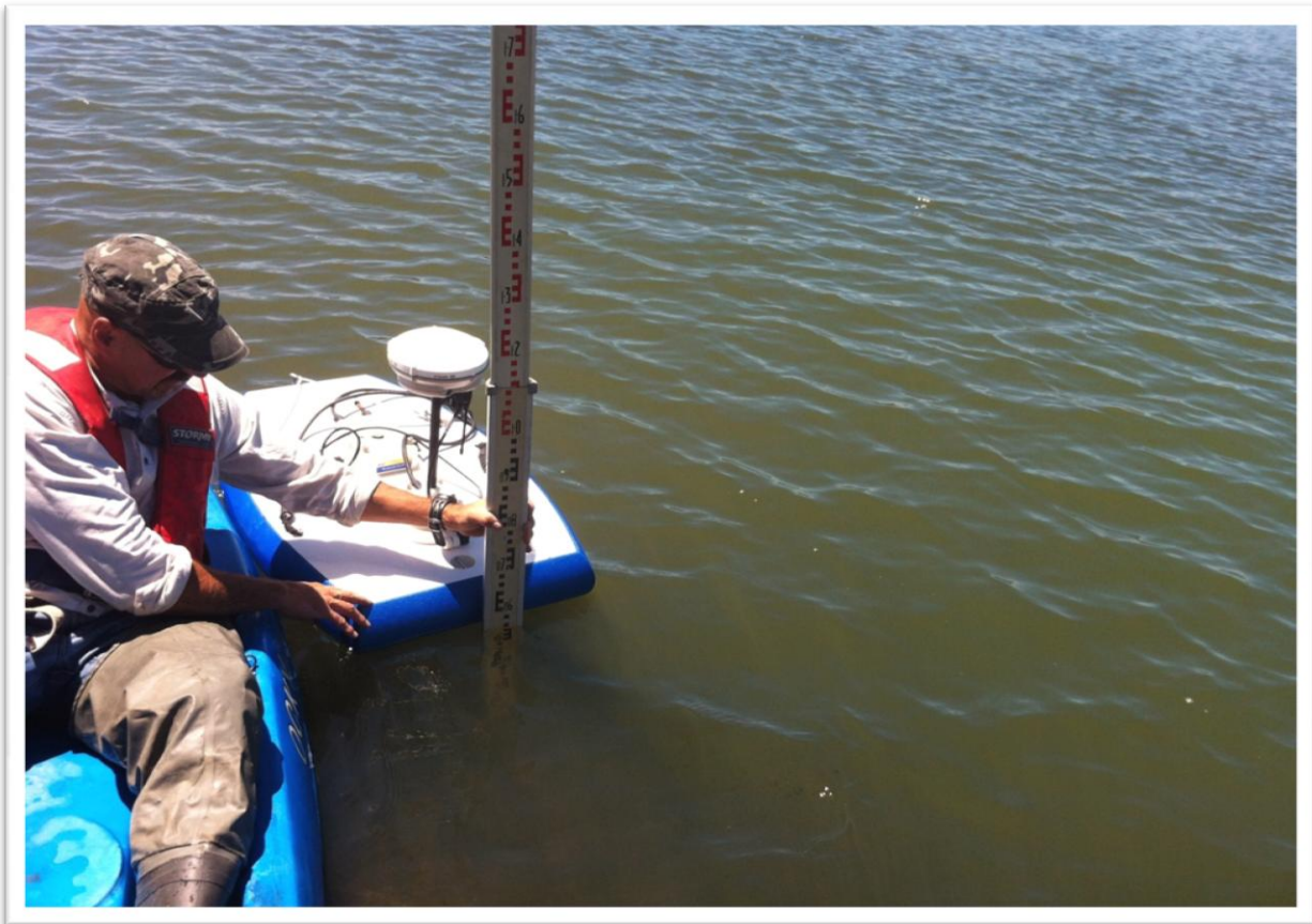
Fig.10 Spot check between YSI M9 and manual survey staff to confirm accurate consistency
