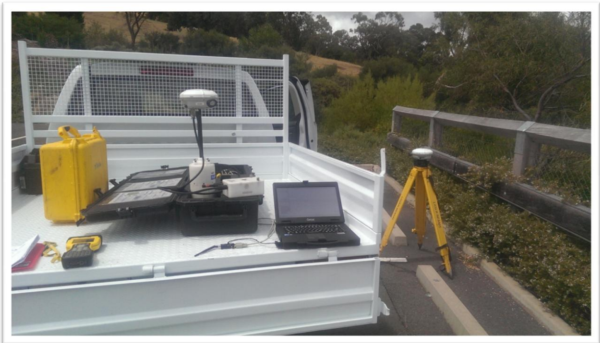
Fig.8: Research and development; pairing M9 and R8 GPS system with custom cable and settings
