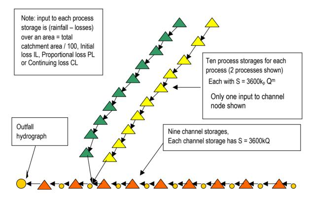
Figure 1 Structure of the RRR Model
