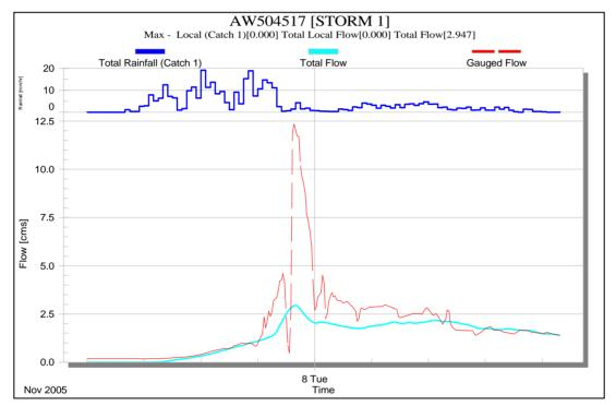
Figure 17 First Creek at Waterfall - Adjusted Initial Loss Only
