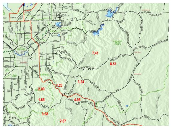
Figure 10 Relative Magnitudes of 1:100 AEP Flows From Flood Frequency Analysis (1:100 AEP flow/A<sup>0.73</sup>)
