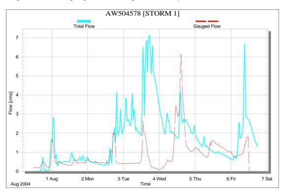
Figure 11 shows the recorded hydrograph, and the preliminary RRR model result. The correspondence is satisfactory until the afternoon of Monday 2 August, when the gauged flow diverges from the predicted flow.
