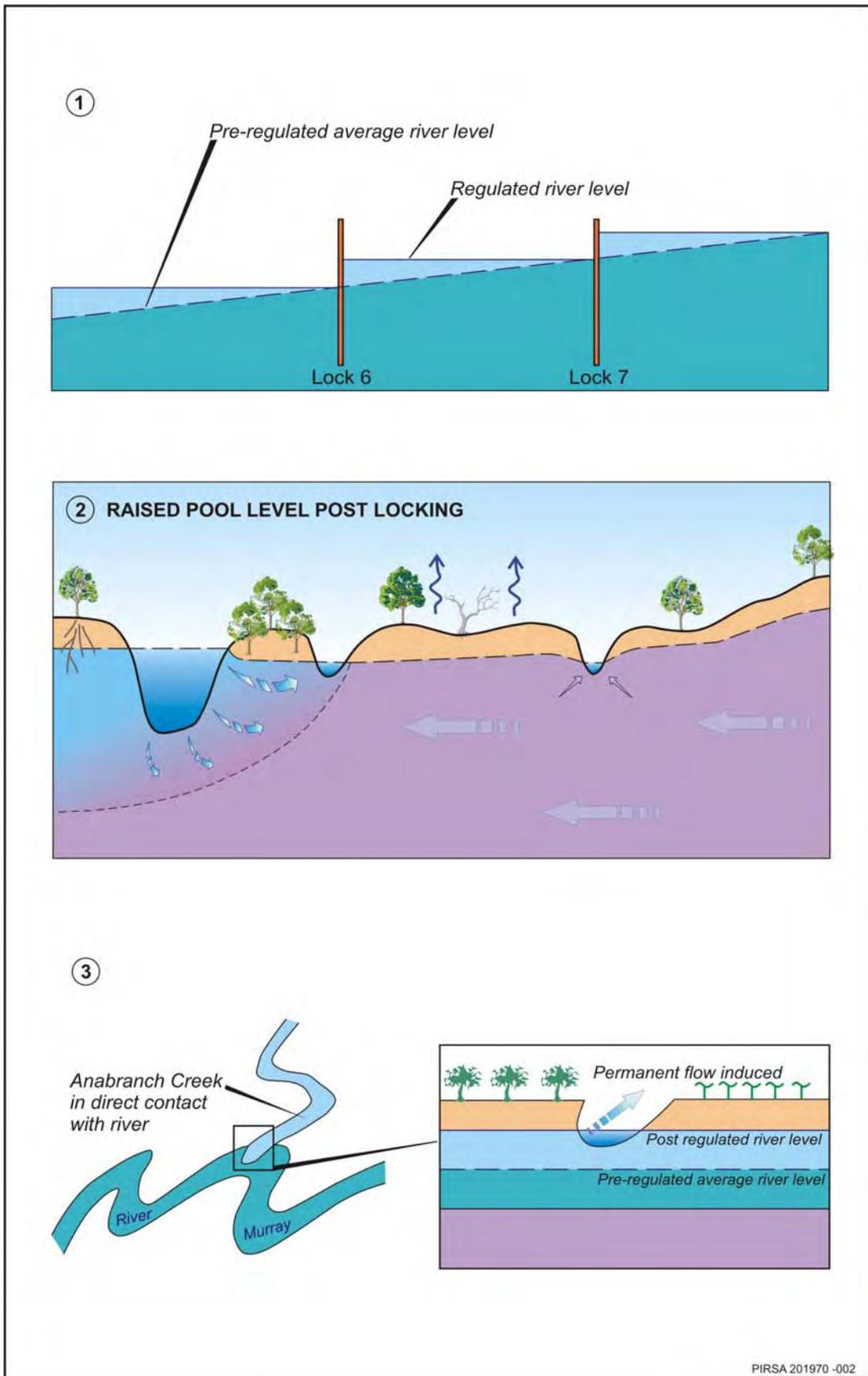
**Figure 3b** Post river locking, the river, creek and groundwater interaction
