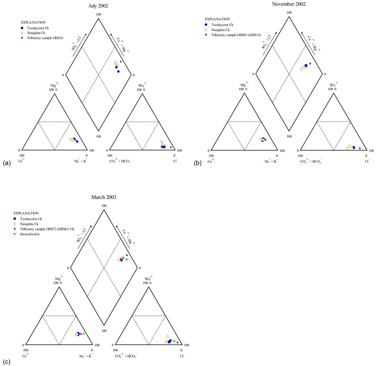
**Figure 21. Piper diagrams showing surface water major ion compositions for each of the sampling stages 1 (a) through to 3 (c) in Tookayerta Creek Catchment. The composition of one groundwater sample is also provided in (c)**
