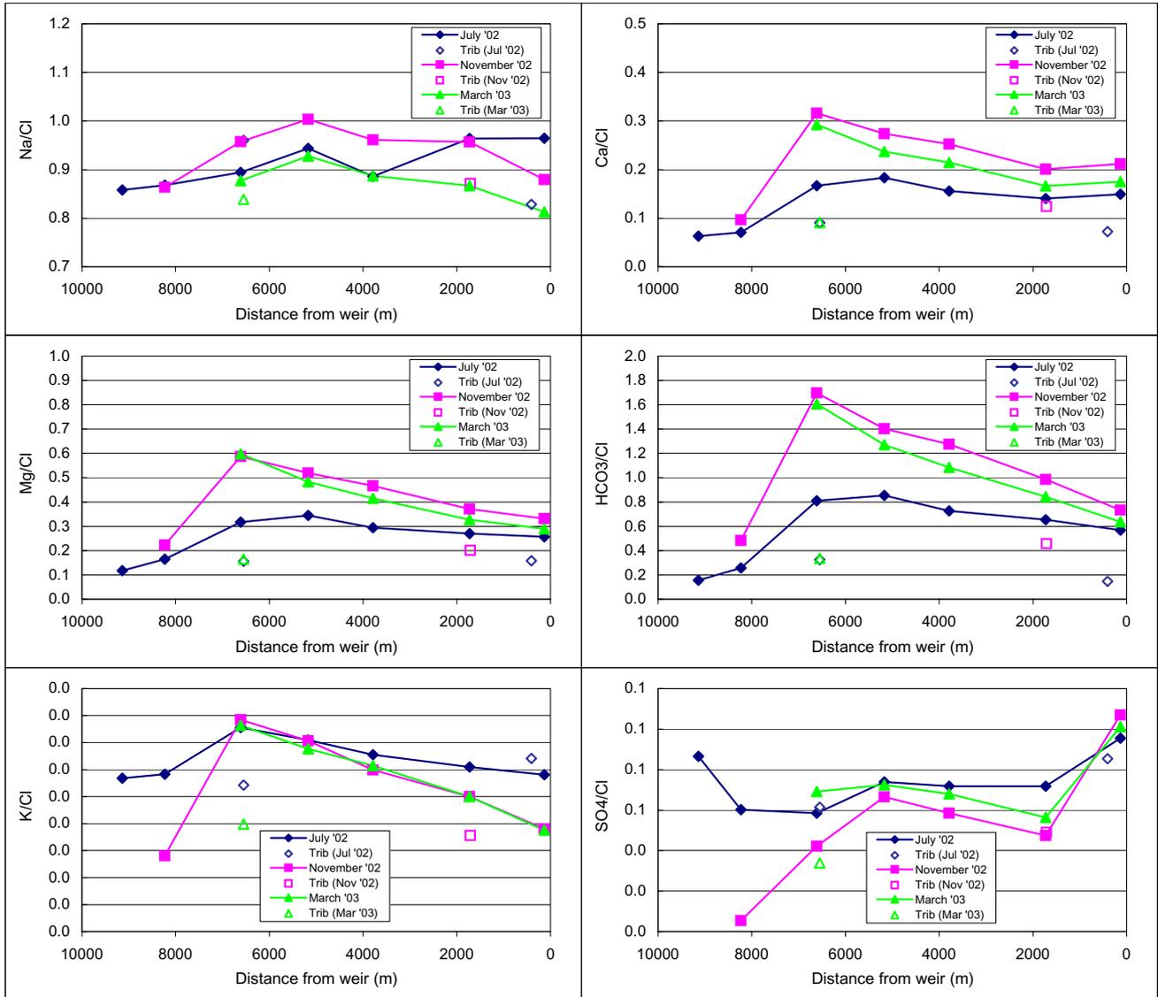
**Figure 9. Surface water ion/Cl ratios obtained during each run-of-river sampling stage in the Scott Creek Sub-catchment. Most significant variations along the creek are for Ca/Cl, Mg/Cl and HCO<sub>3</sub>/Cl, probably reflecting groundwater discharge from or via the Skillogalee Dolomite**
