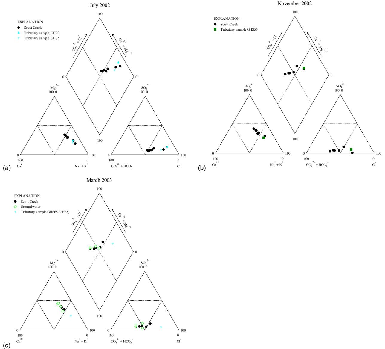
**Figure 8. Piper diagrams showing surface water major ion compositions for each of the sampling stages 1 (a) through to 3 (c) in Scott Creek Sub-catchment. Groundwater compositions from several wells are provided in (c).**
