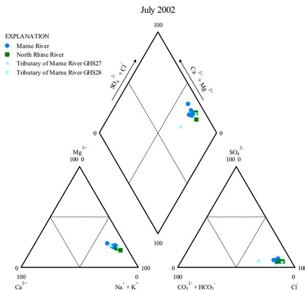
**Figure 15. Piper diagram showing surface water major ion compositions for sampling stage 1 in Marne River Catchment**
