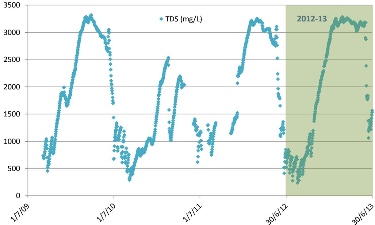
Figure 39. Salinity data at Inman River u/s sewage treatment works from 2009–13
