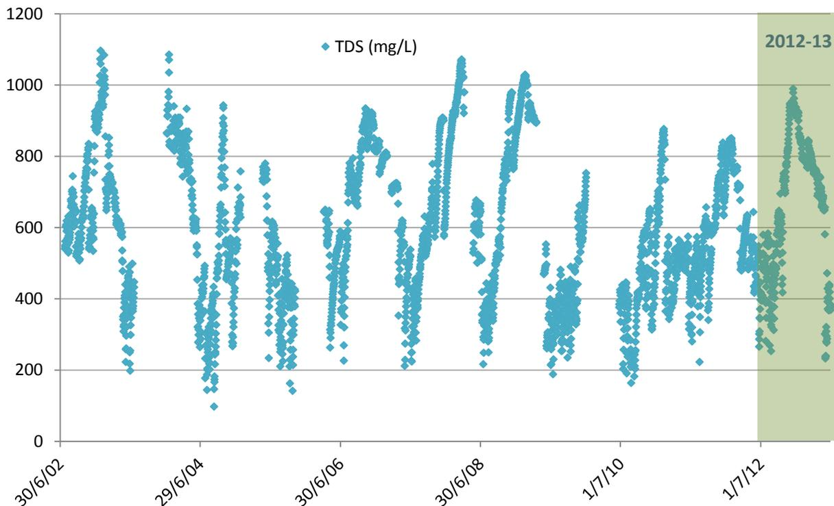
Figure 38. Salinity data at Onkaparinga River u/s Hahndorf Dissipater from 2002–13
