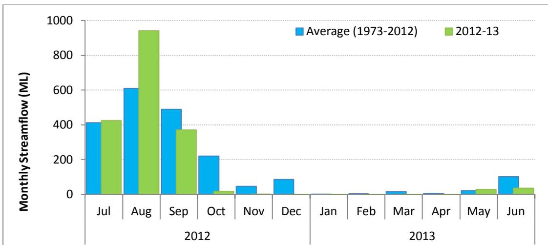
Figure 20. Torrens River monthly streamflow (ML)
