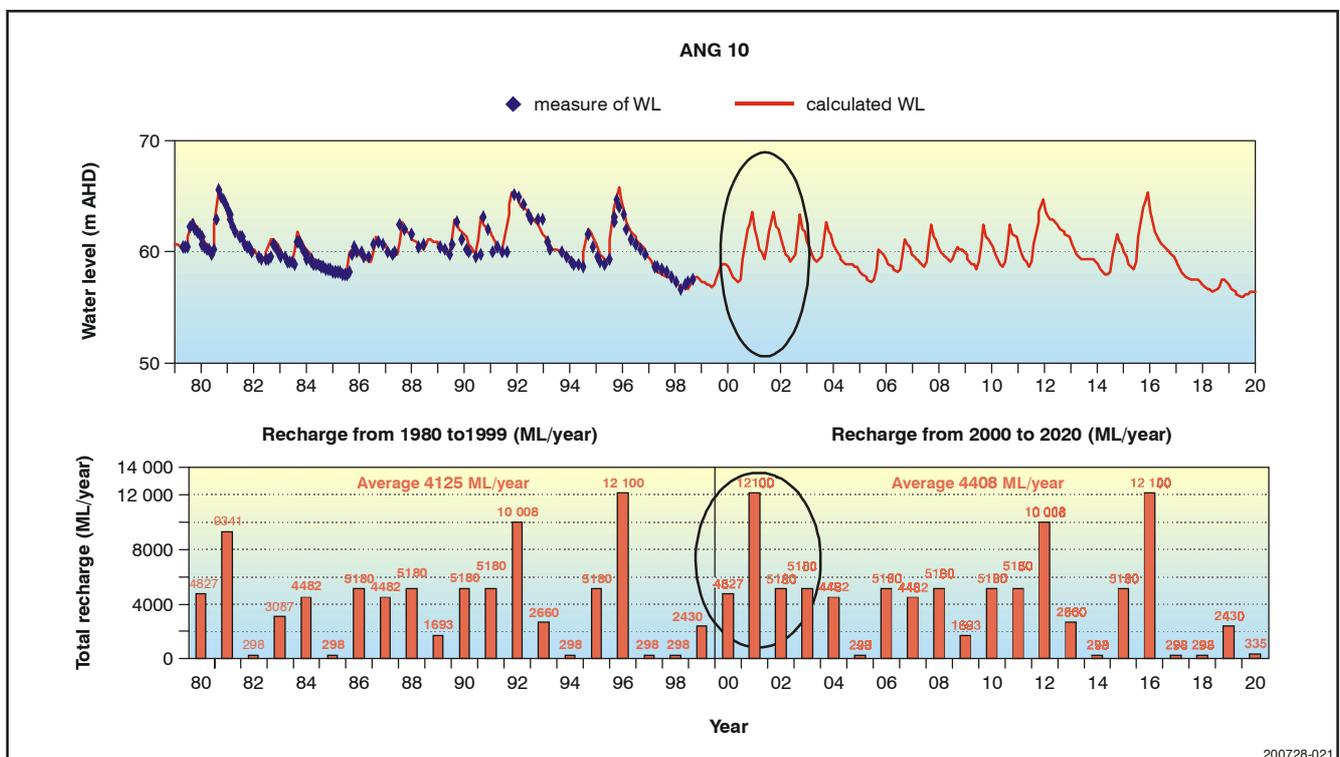
Figure 21 Model results for Scenario 3 (average streamflow for 3 years)
