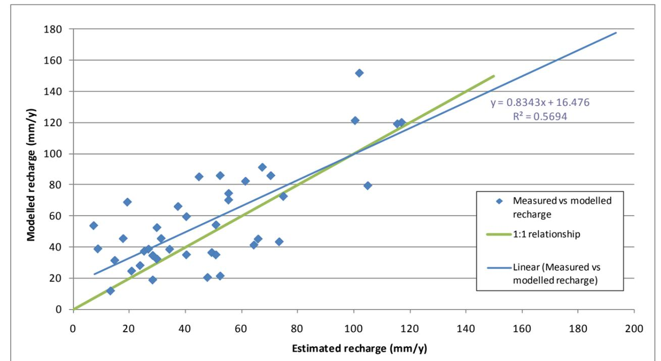
Figure 85. LEACHM modelled recharge for soil B3 versus estimated recharge for Obswell ULE101
