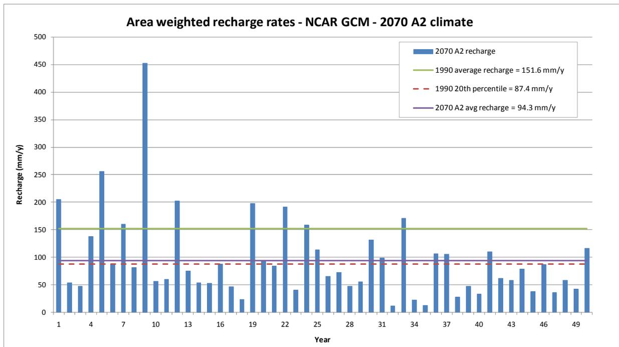
**Figure 48. Annual area-weighted recharge rates produced by the LEACHG model for the Southern Basins PWA, using rainfall and PET input data generated by the NCAR-CCSM3 GCM for a 2070 climate and A2 emissions**
