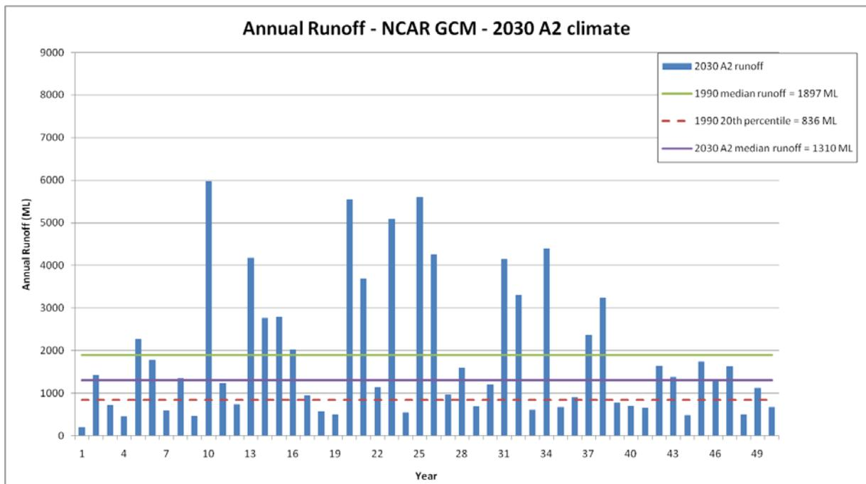
Figure 53. Annual runoff simulated for the Tod Reservoir, based on rainfall and PET input data generated by the NCAR-CCSM3 GCM for a 2030 climate and A2 emissions
