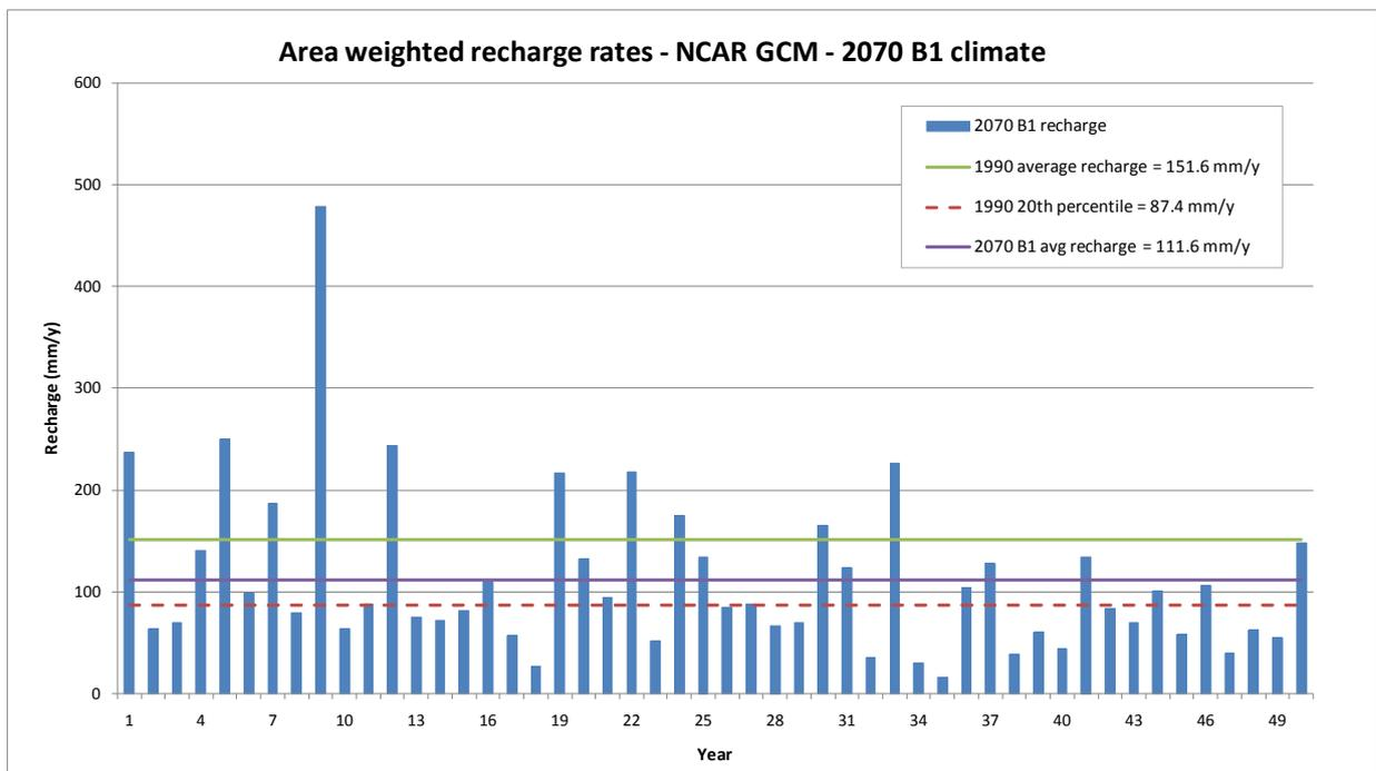
Figure 47. Annual area-weighted recharge rates produced by the LEACHG model for the Southern Basins PWA, using rainfall and PET input data generated by the NCAR-CCSM3 GCM for a 2070 climate and B1 emissions
