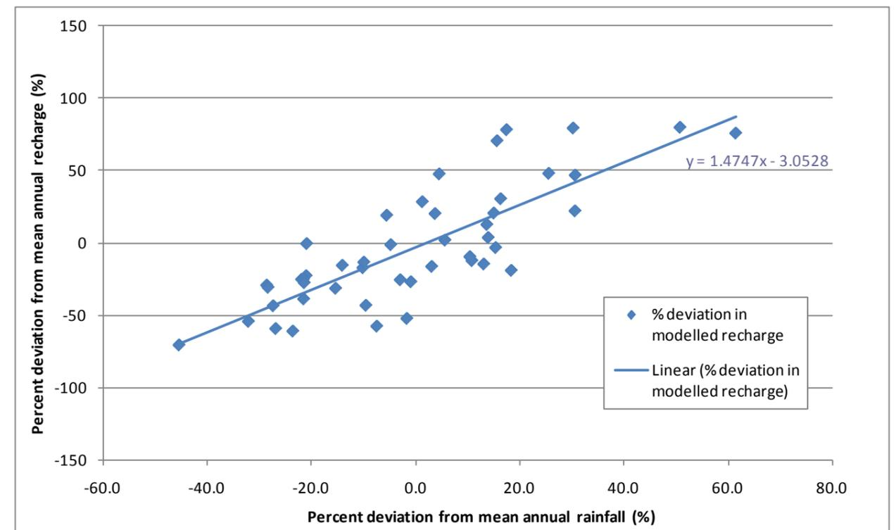
Figure 83. Modelled percent deviation in mean annual recharge versus percent deviation in mean annual rainfall for the H1 model with no crop cover (i.e. bare carbonate sand surface)
