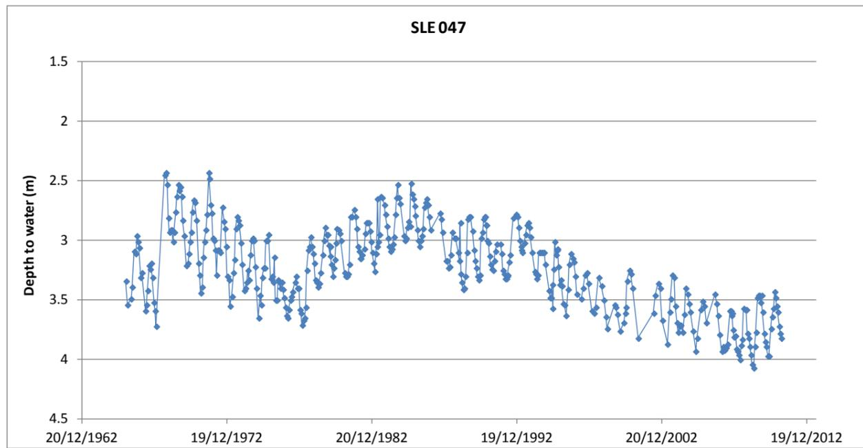
Figure 76. Observed groundwater levels in Obswell SLE047
