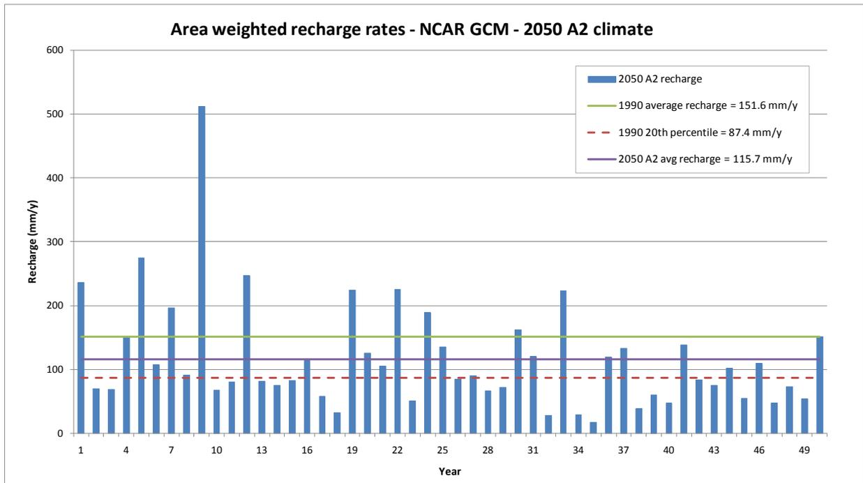
Figure 46. Annual area-weighted recharge rates produced by the LEACHG model for the Southern Basins PWA, using rainfall and PET input data generated by the NCAR-CCSM3 GCM for a 2050 climate and A2 emissions
