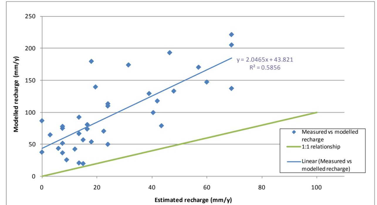
Figure 71. LEACHM modelled recharge for soil B2 versus estimated recharge for Obswell WAY054
