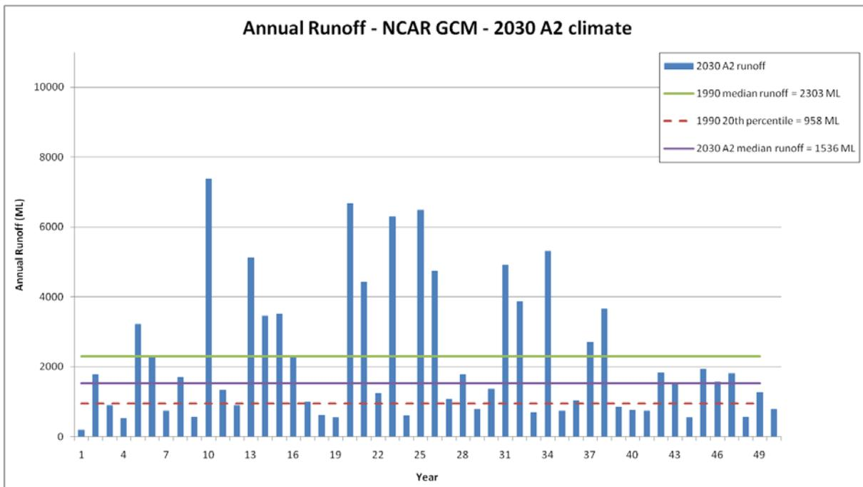
Figure 90. Annual runoff simulated for the Tod Reservoir, based on rainfall and PET input data generated by the NCAR-CCSM3 GCM for a 2030 climate and A2 emissions
