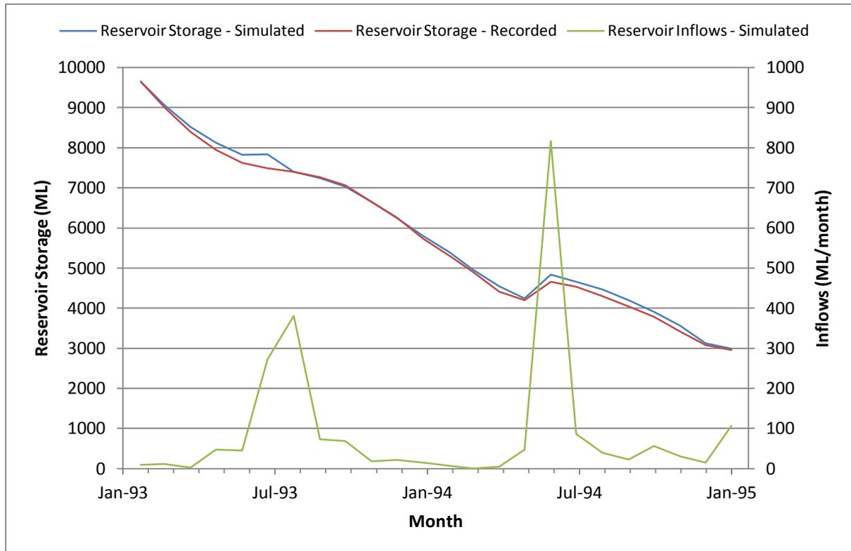
Figure 19. Simulated and observed water level, with inflows, for the Tod Reservoir
