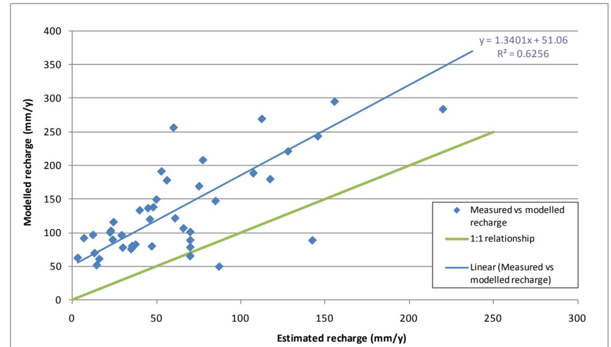
Figure 68. LEACHM modelled recharge for soil B1 versus estimated recharge for Obswell ULE134
