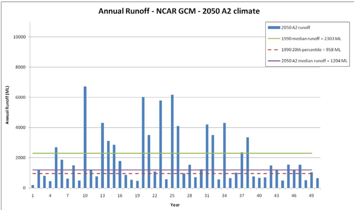
Figure 92. Annual runoff simulated for the Tod Reservoir, based on rainfall and PET input data generated by the NCAR GCM for a 2050 climate and A2 emissions
