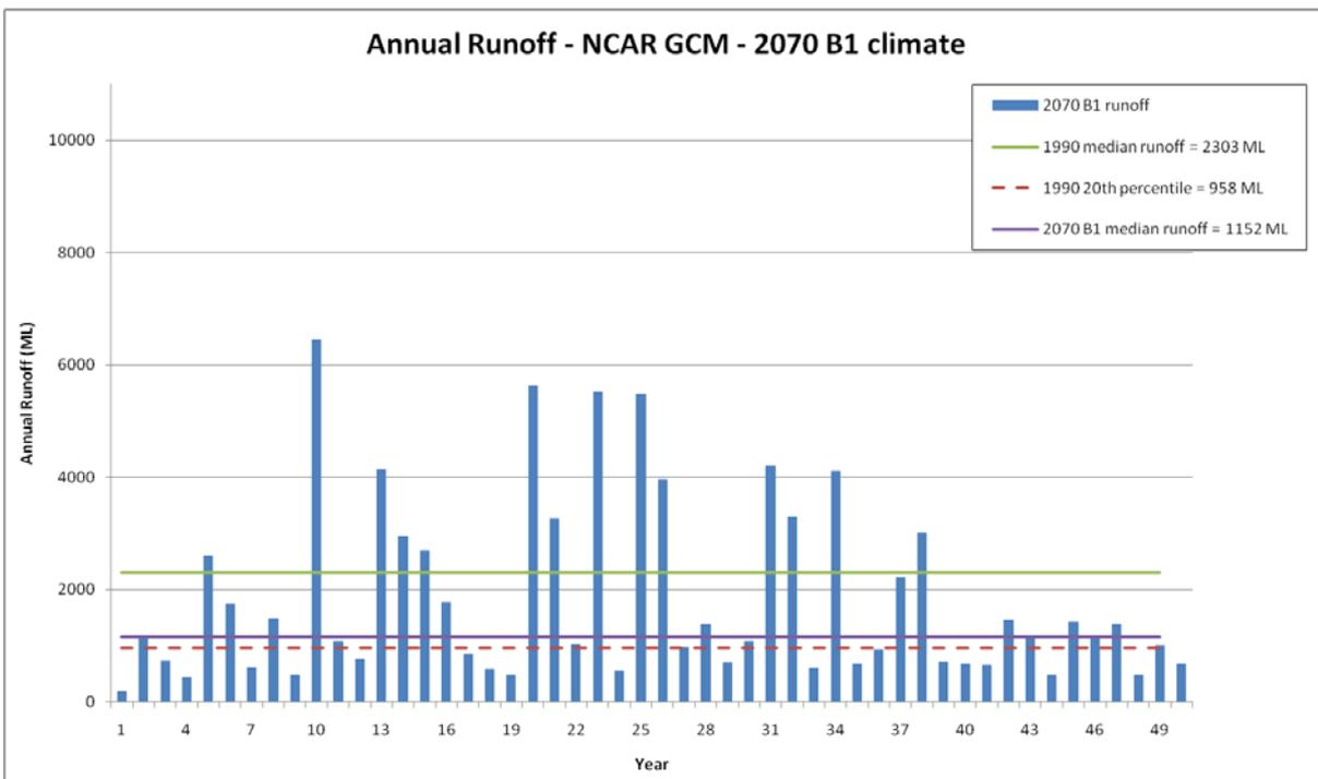
Figure 93. Annual runoff simulated for the Tod Reservoir, based on rainfall and PET input data generated by the NCAR-CCSM3 GCM for a 2070 climate and B1 emissions
