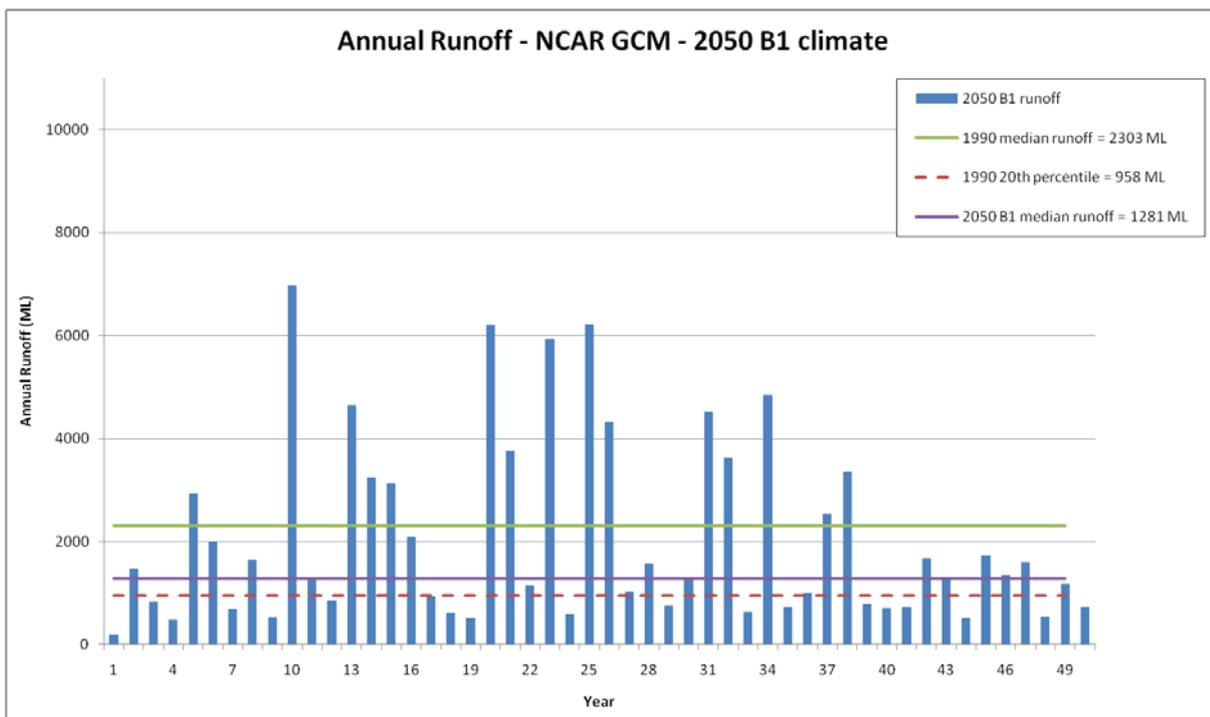
Figure 91. Annual runoff simulated for the Tod Reservoir, based on rainfall and PET input data generated by the NCAR-CCSM3 GCM for a 2050 climate and B1 emissions
