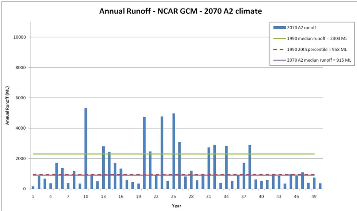
Figure 94. Annual runoff simulated for the Tod Reservoir, based on rainfall and PET input data generated by the NCAR-CCSM3 GCM for a 2070 climate and A2 emissions
