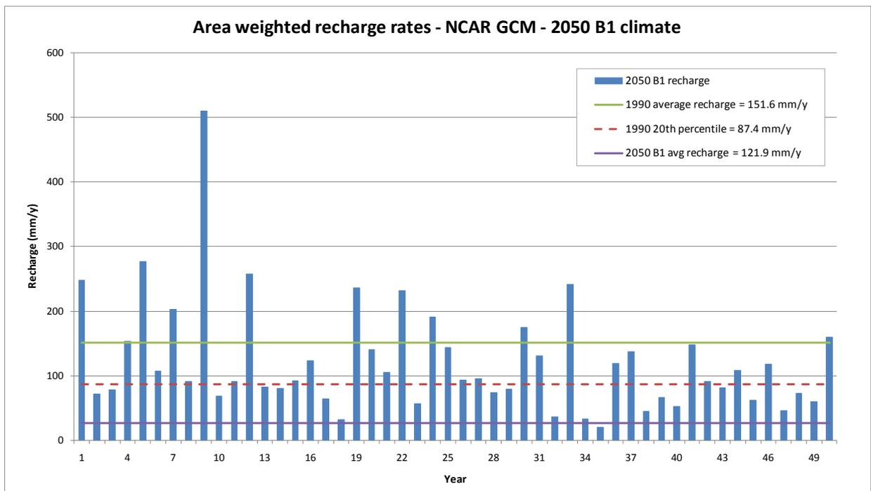
Figure 45. Annual area-weighted recharge rates produced by the LEACHG model for the Southern Basins PWA, using rainfall and PET input data generated by the NCAR-CCSM3 GCM for a 2050 climate and B1 emissions
