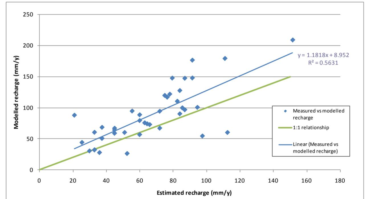
Figure 77. LEACHM modelled recharge for soil B3 versus estimated recharge for Obswell SLE047
