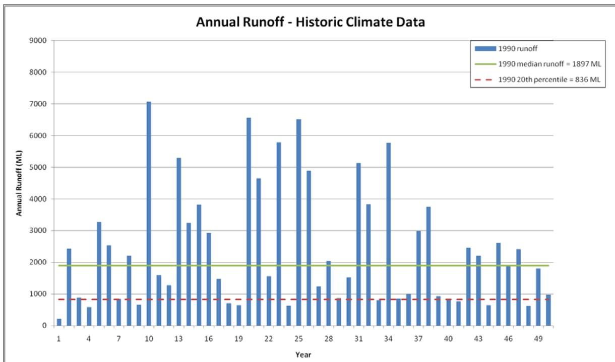
**Figure 51. Annual runoff simulated over 50 years for the Tod Reservoir, based on historically measured rainfall and PET data. Year 1 on the x axis represents 1960**
