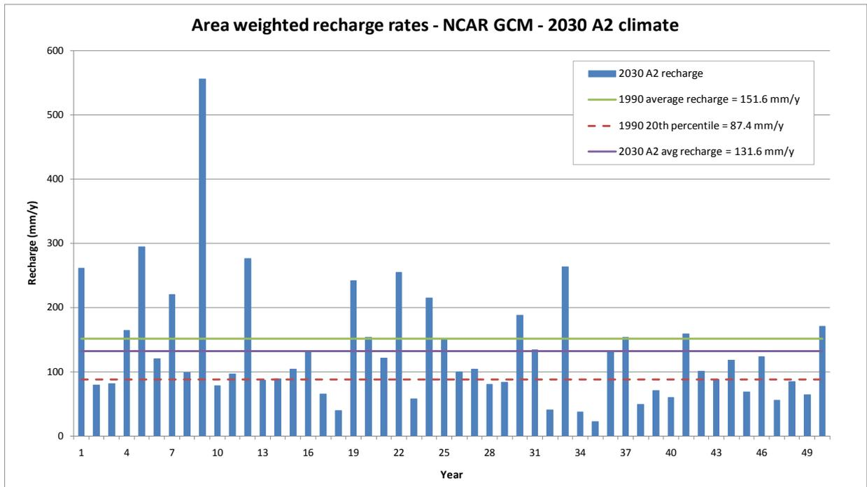
Figure 44. Annual area-weighted recharge rates produced by the LEACHG model for the Southern Basins PWA, using rainfall and PET input data generated by the NCAR-CCSM3 GCM for a 2030 climate and A2 emissions
