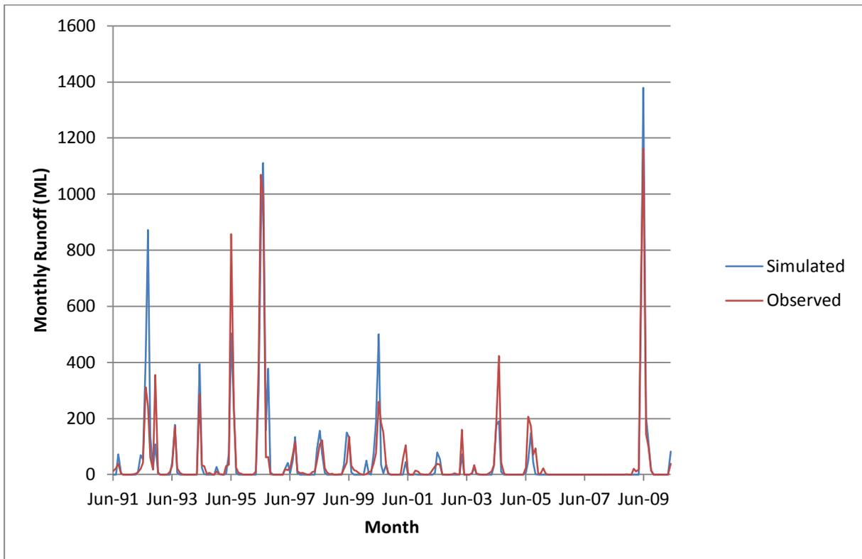
Figure 15. Simulated and observed monthly runoff for the Toolillie Gully catchment
