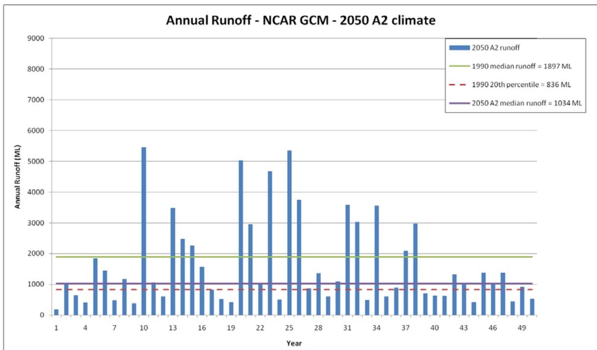
Figure 55. Annual runoff simulated for the Tod Reservoir, based on rainfall and PET input data generated by the NCAR-CCSM3 GCM for a 2050 climate and A2 emissions
