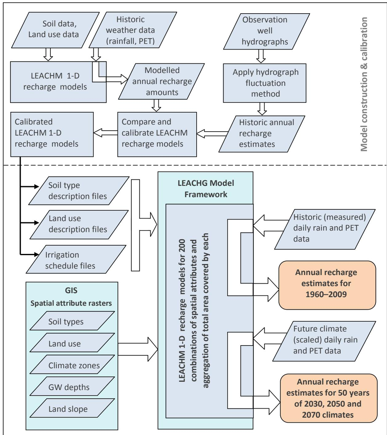
Figure 10. Flowchart of groundwater recharge modelling framework applied to the Eyre Peninsula PWAs
