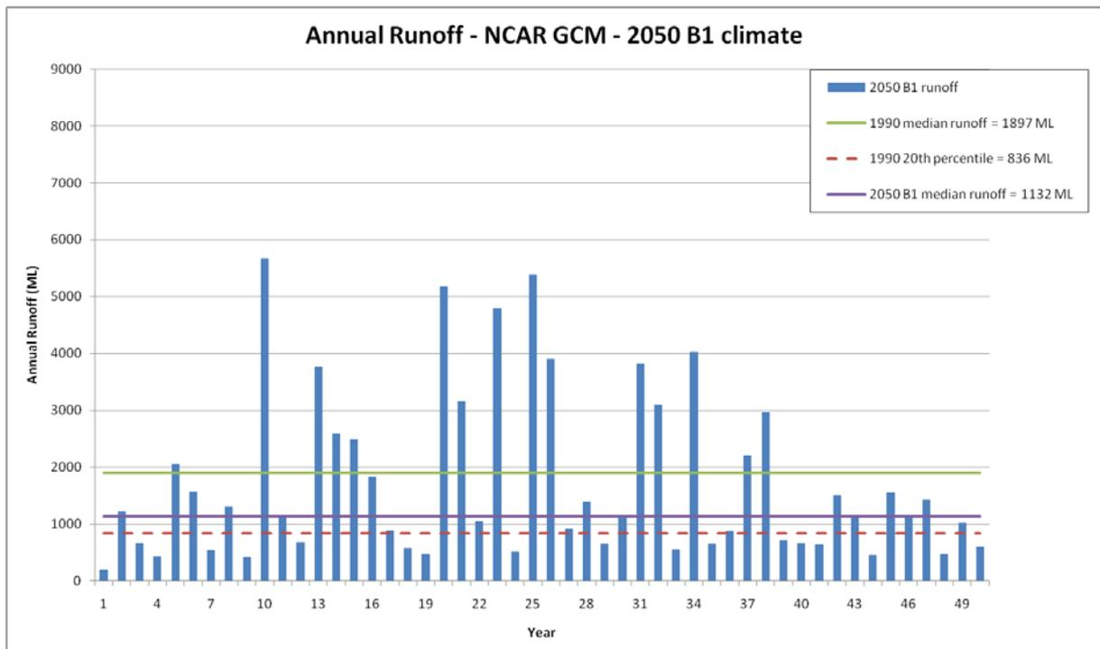
Figure 54. Annual runoff simulated for the Tod Reservoir, based on rainfall and PET input data generated by the NCAR-CCSM3 GCM for a 2050 climate and B1 emissions
