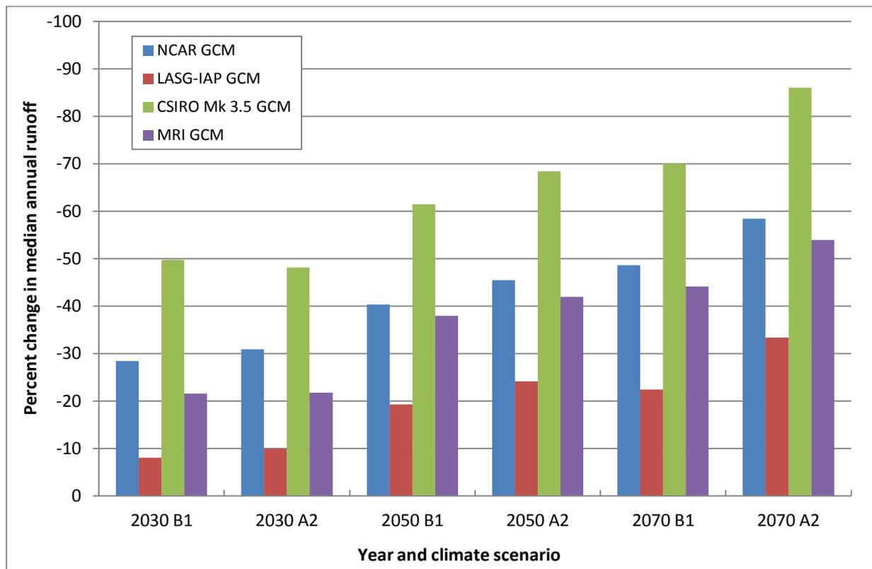
**Figure 50. Projected changes in average annual runoff for runoff to the Tod Reservoir (no diversions, current farm dam storage)**
