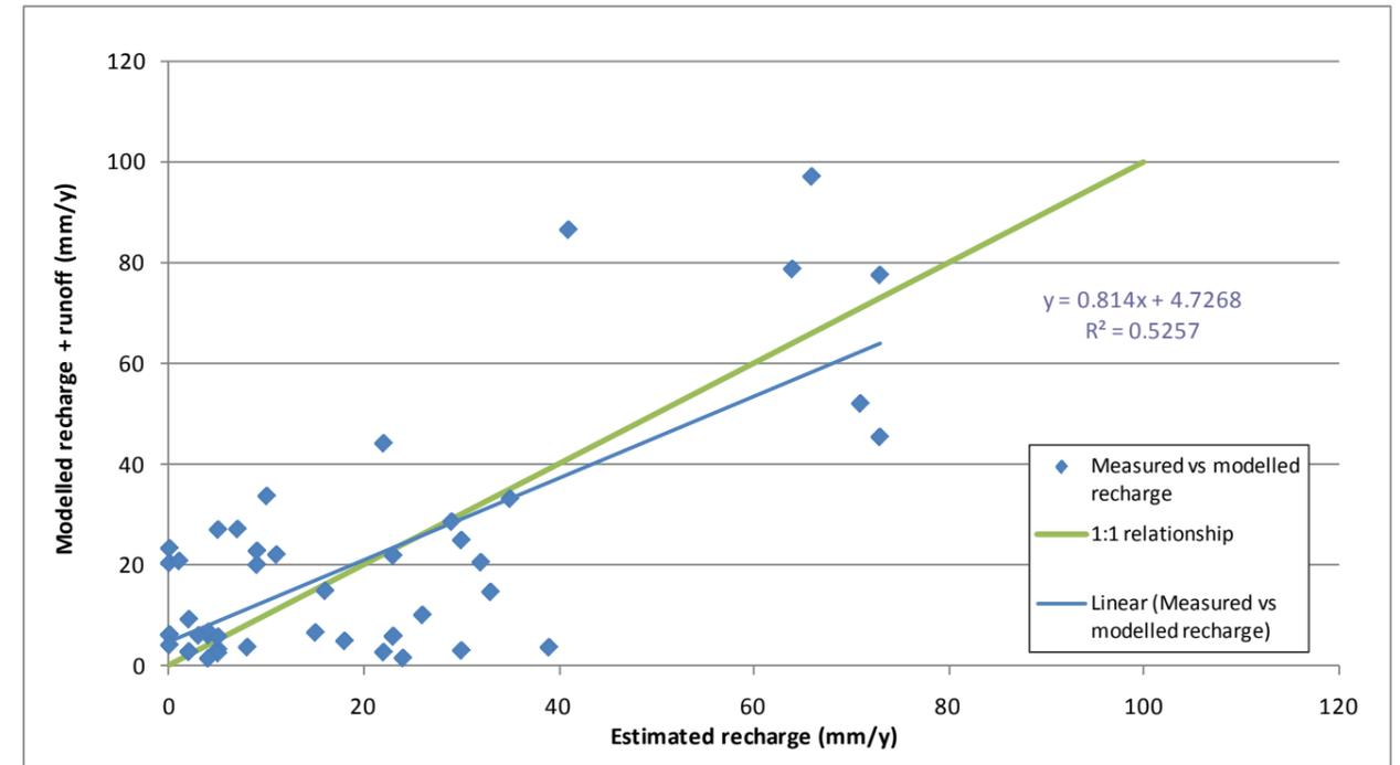
Figure 65. LEACHM modelled recharge for soil A1 versus estimated recharge for Obswell SQR031
