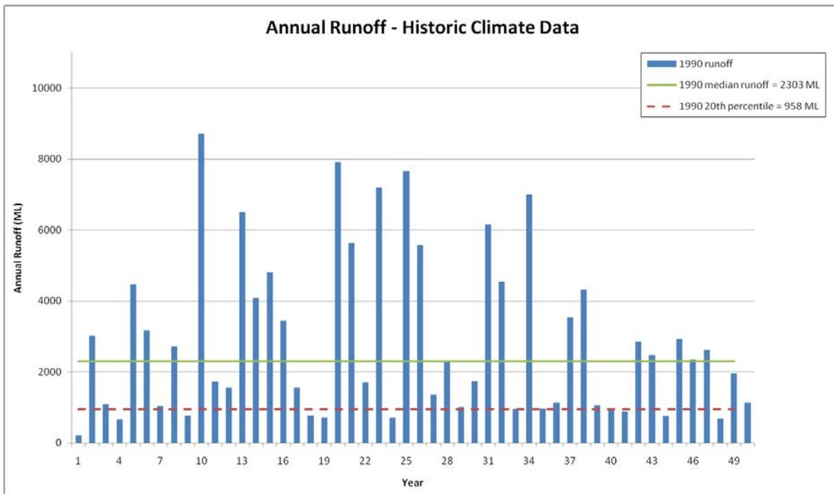
Figure 88. Annual runoff simulated over 50 years for the Tod Reservoir, based on historically measured rainfall and PET data. Year 1 on the x axis represents 1960
