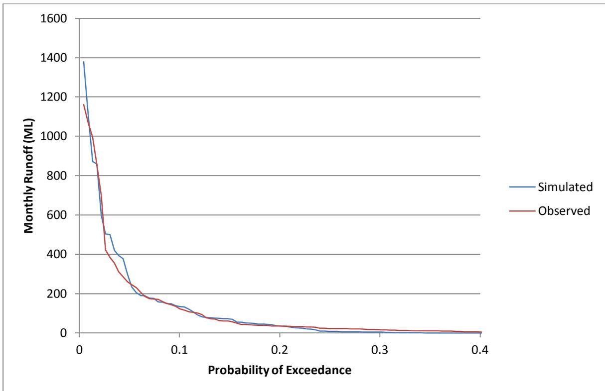
Figure 16. Simulated and observed monthly flow duration curve for the Toolillie Gully catchment
