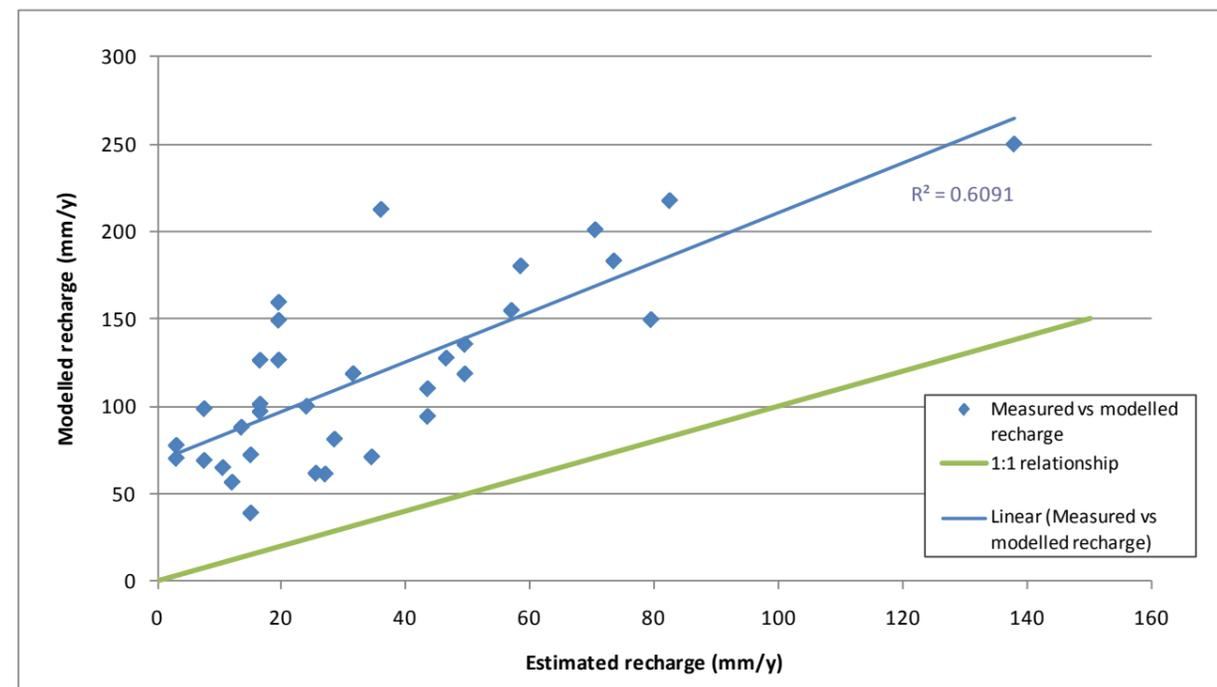
Figure 74. LEACHM modelled recharge for soil B3 versus estimated recharge for Obswell ULE139
