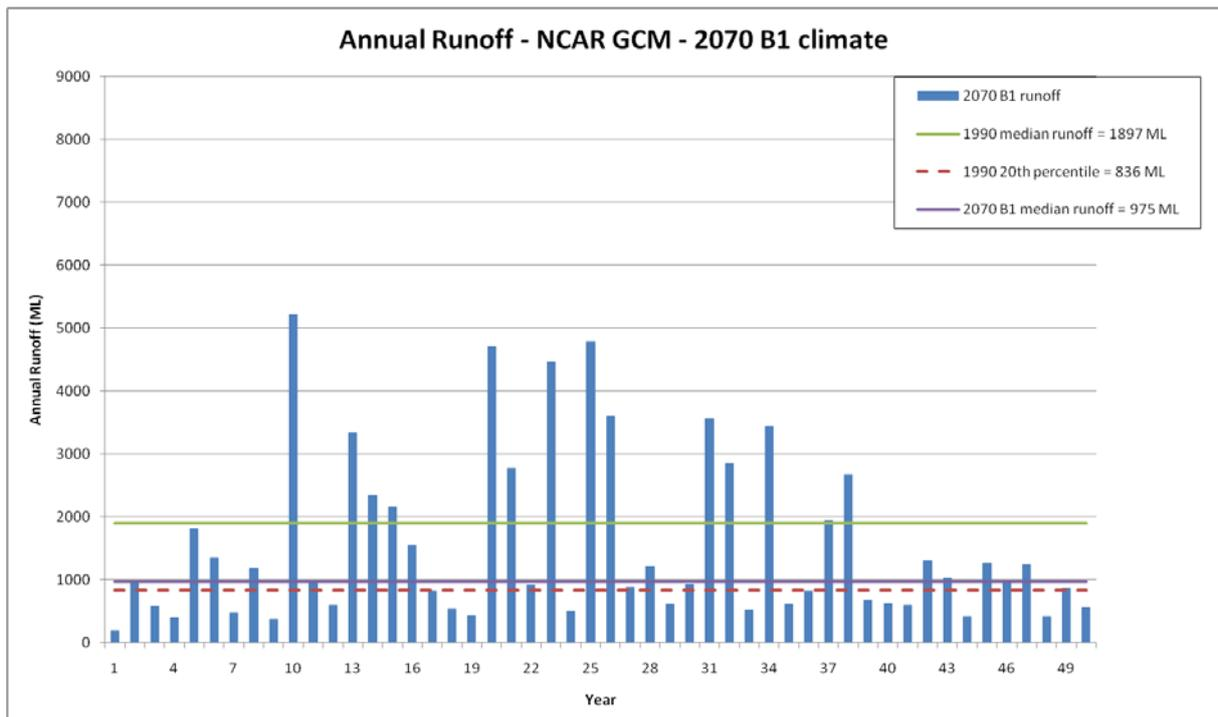
Figure 56. Annual runoff simulated for the Tod Reservoir, based on rainfall and PET input data generated by the NCAR-CCSM3 GCM for a 2070 climate and B1 emissions
