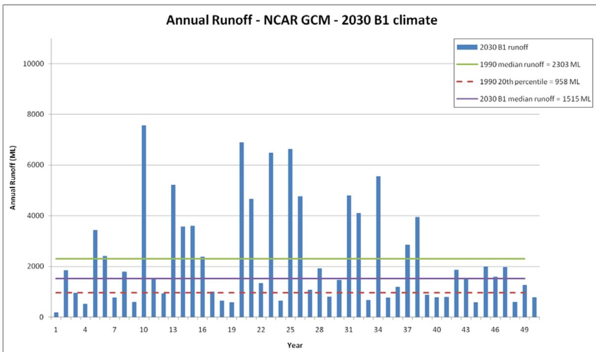
Figure 89. Annual runoff simulated for the Tod Reservoir, based on rainfall and PET input data generated by the NCAR-CCSM3 GCM for a 2030 climate and B1 emissions
