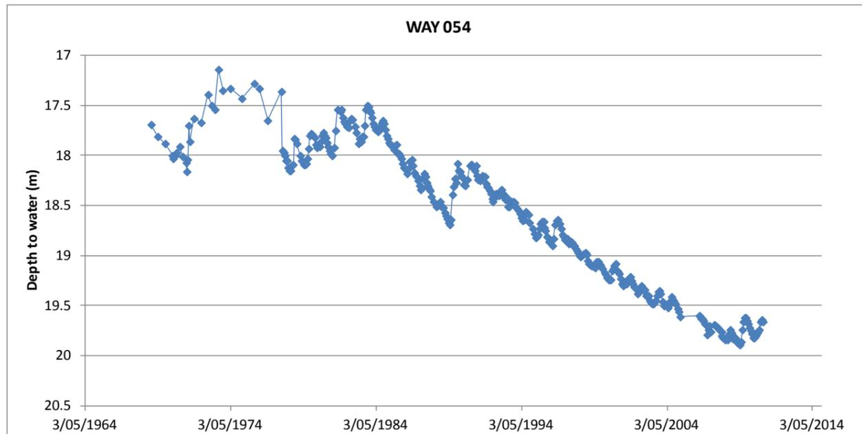
Figure 70. Observed groundwater levels in Obswell WAY054
