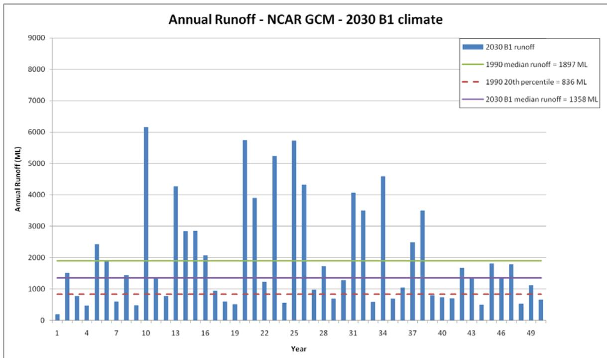
Figure 52. Annual runoff simulated for the Tod Reservoir, based on rainfall and PET input data generated by the NCAR-CCSM3 GCM for a 2030 climate and B1 emissions
