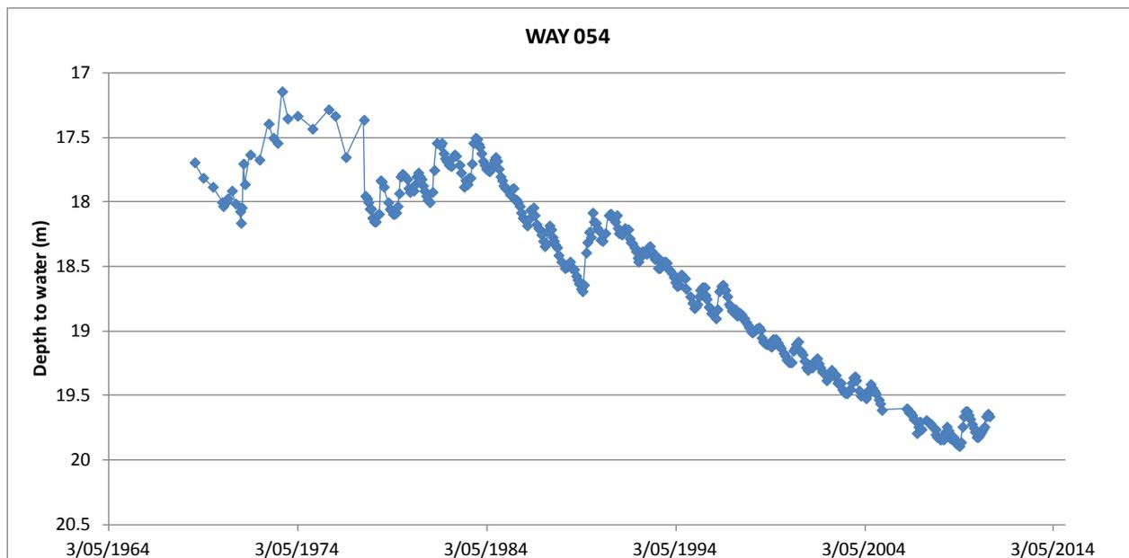
**Figure 8. Groundwater levels in observation well WAY054**
