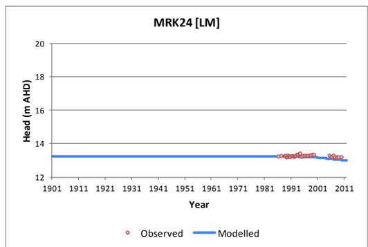
**Figure 4.5(d). Hydrograph comparison between observed and modelled for Woolpunda (Lower Mannum Formation)**
