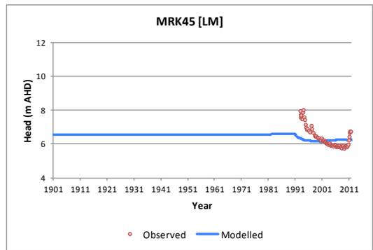
Figure 4.5(e). Hydrograph comparison between observed and modelled for Woolpunda (Lower Mannum Formation)
