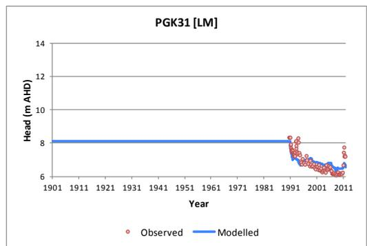
**Figure 4.5(j). Hydrograph comparison between observed and modelled for Woolpunda (Lower Mannum Formation)**
