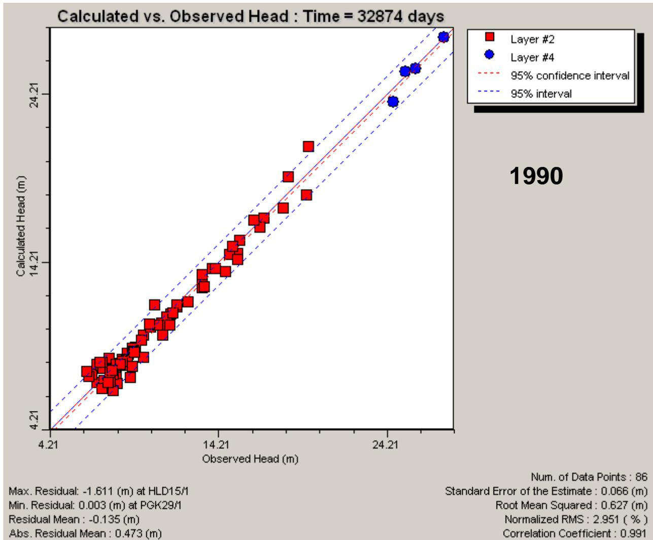
**Figure 4.8. Scaled Root Mean Square (SRMS) at 1990**
