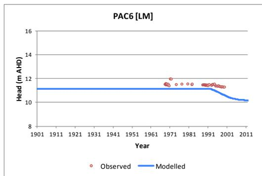
**Figure 4.5(f). Hydrograph comparison between observed and modelled for Woolpunda (Lower Mannum Formation)**
