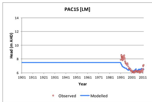
**Figure 4.5(g). Hydrograph comparison between observed and modelled for Woolpunda (Lower Mannum Formation)**
