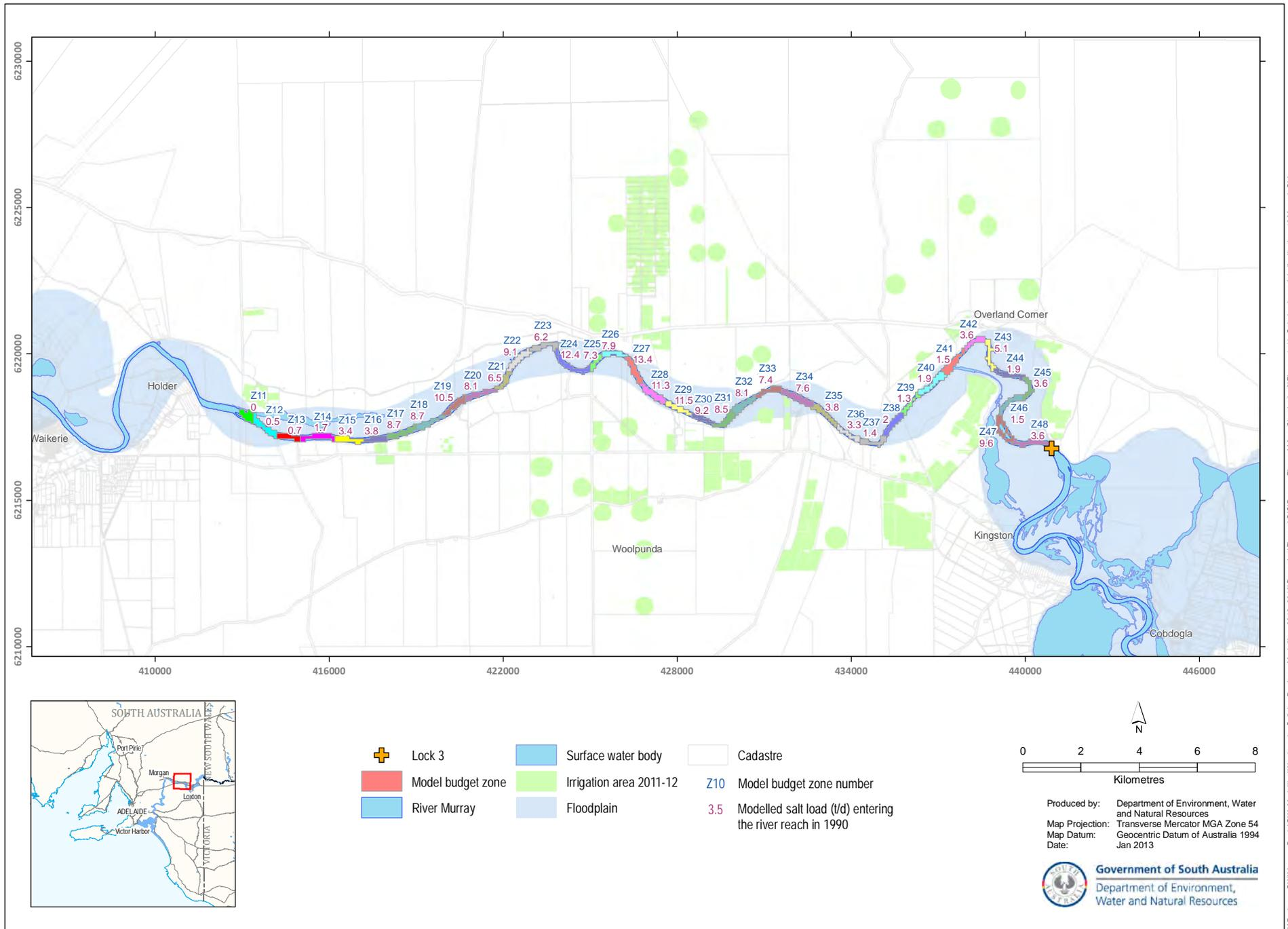
Figure 4.11. Modelled salt load spatial distribution at 1990
