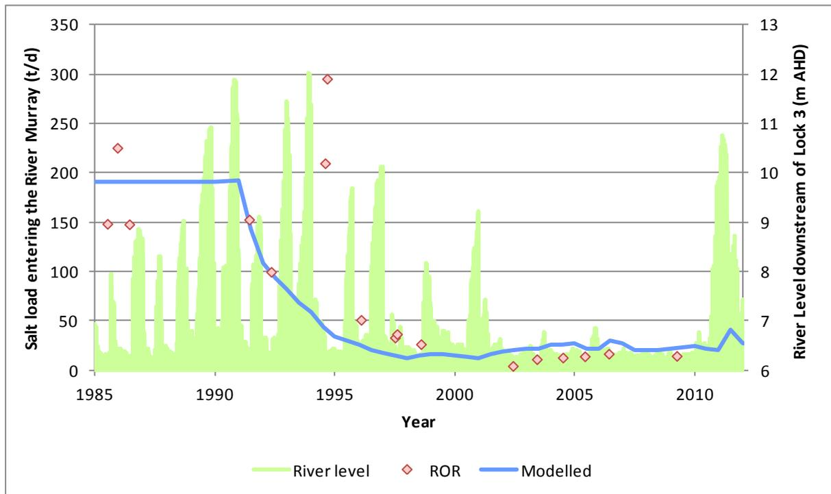
Figure 4.14 Salt load comparison between Run-of-River measurements and the calibrated model outputs for Woolpunda
