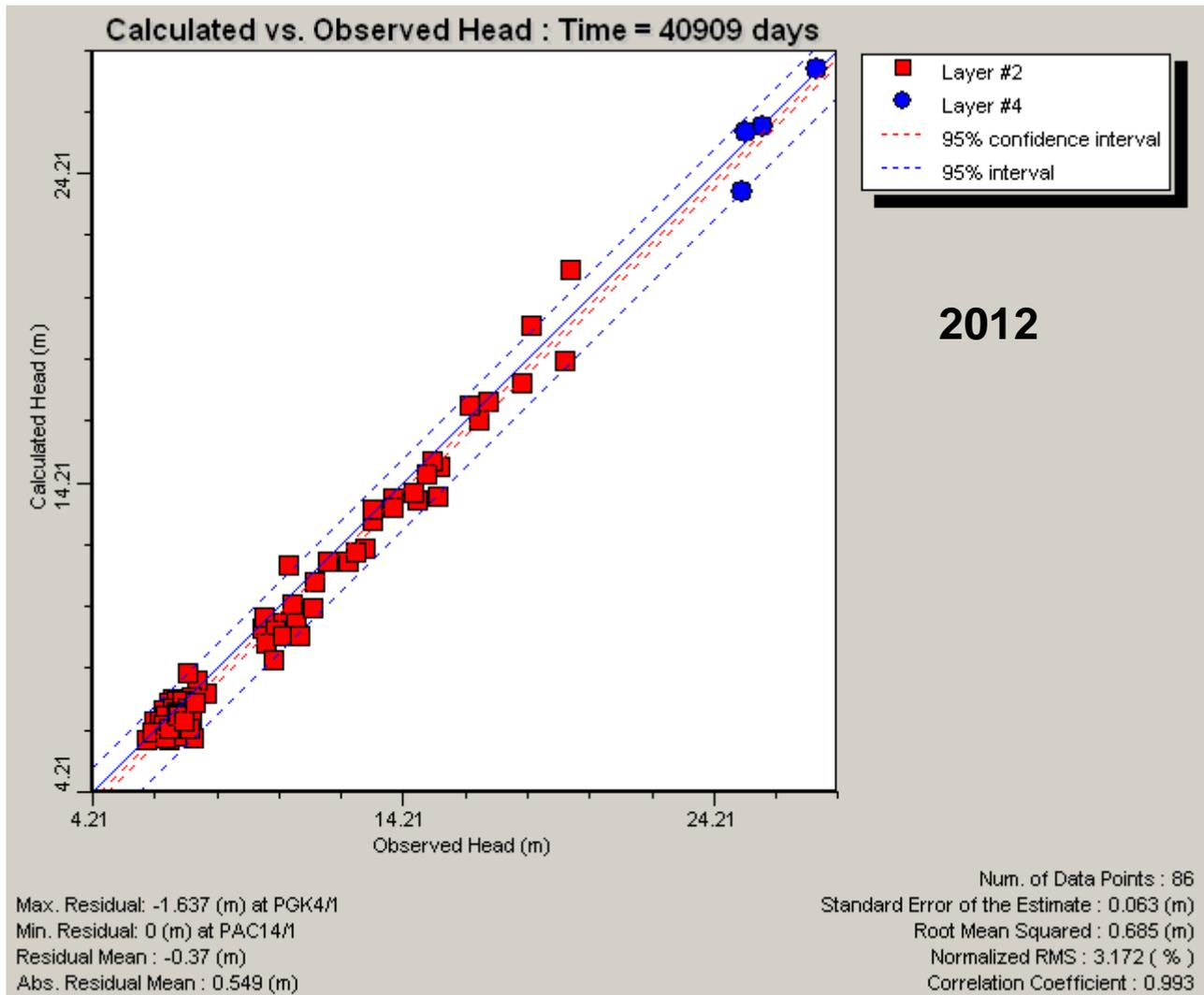
**Figure 4.10. Scaled Root Mean Square (SRMS) at 2012**
