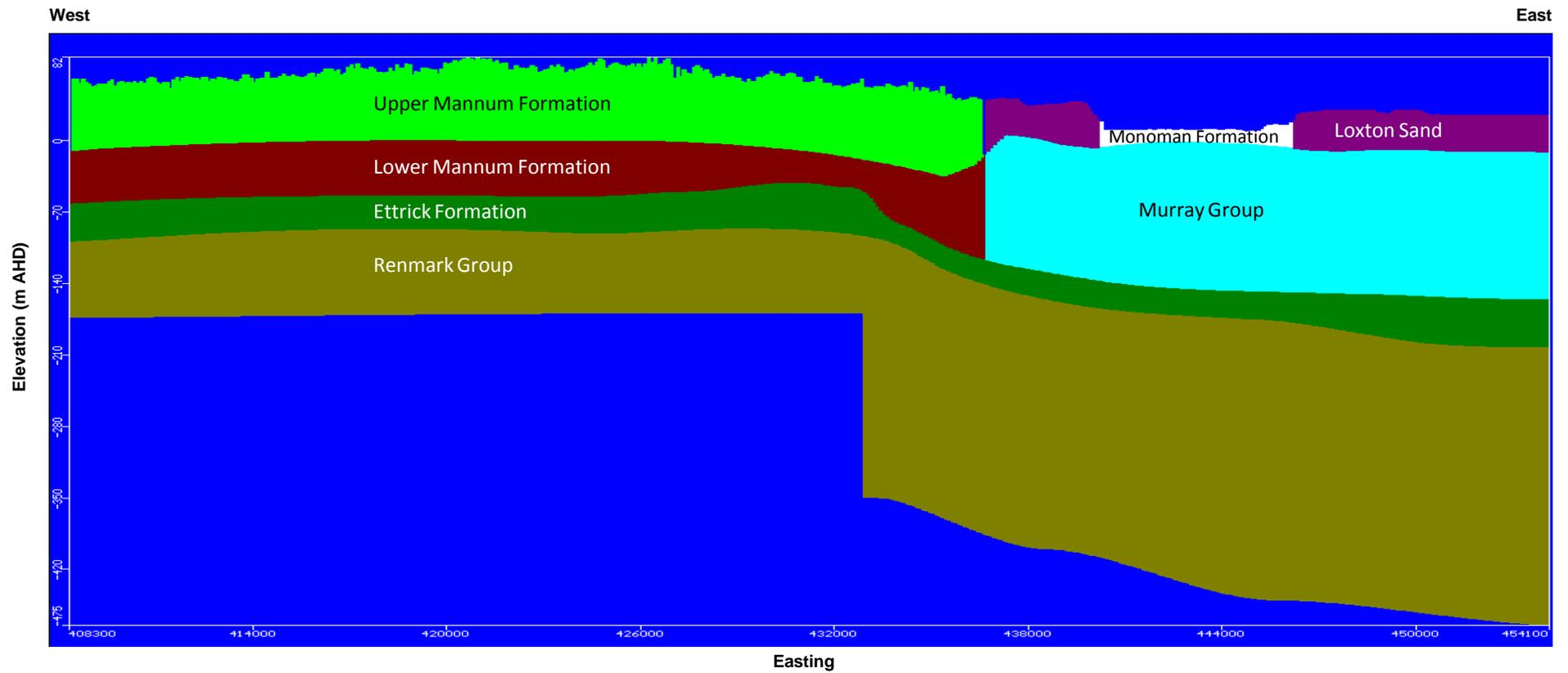
Figure 3.4. Model layers (east-west cross-section through model row 366, N6212150)
