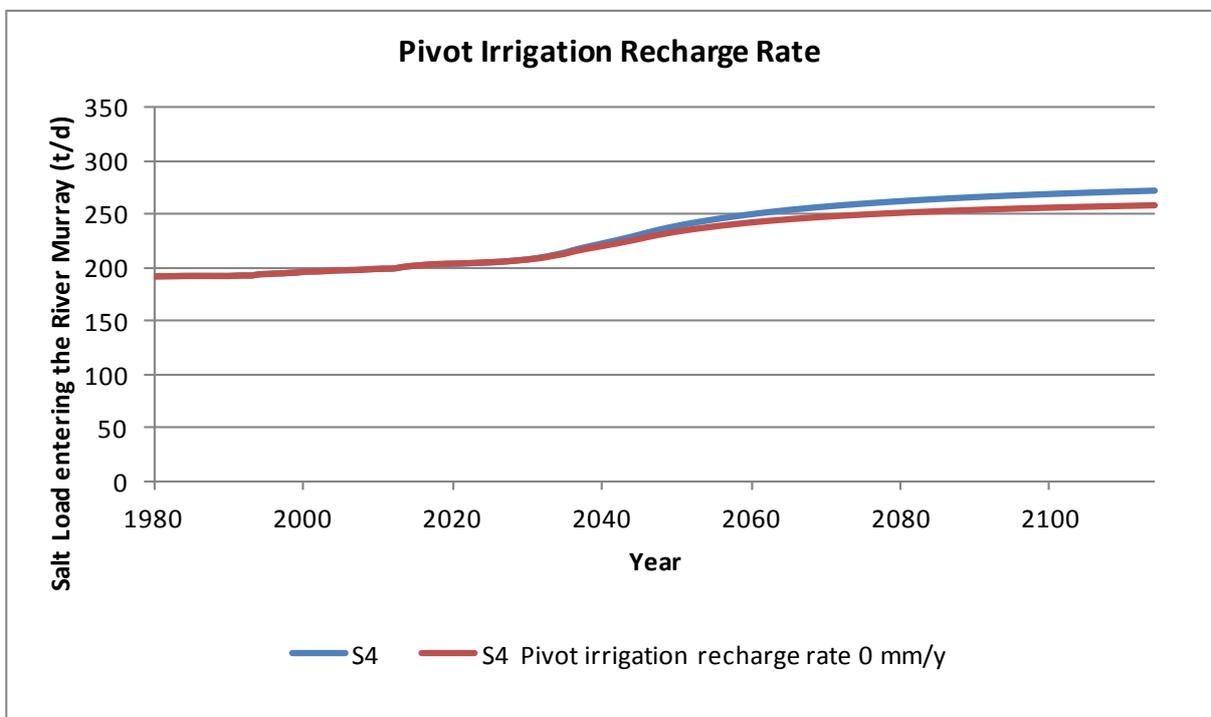
Figure 6.5 Uncertainty of pivot irrigation recharge rate in salt loads for the Woolpunda Reach
