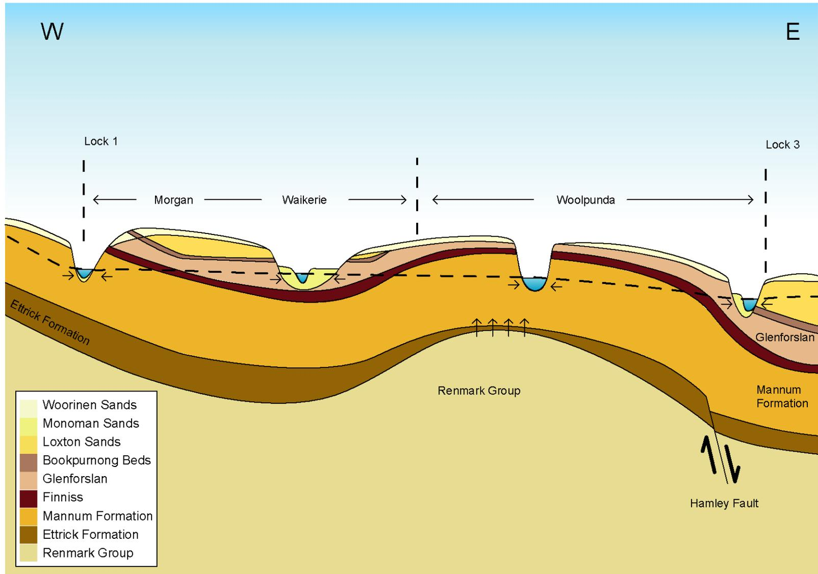
Figure 1.2. Lock 3 to Morgan hydrogeological conceptual model (After Yan, Li and Woods 2012)
