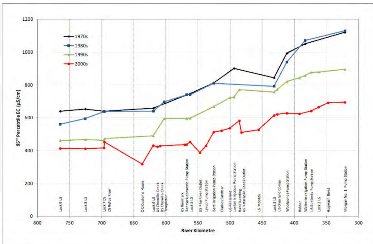
Figure 2.13 In-stream salinity 95 percentile versus river km for selected flows (AWE 2012)
