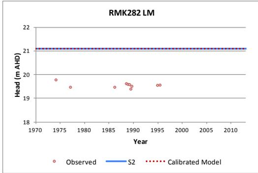
**Figure 6.7(b). Hydrographs near the north and south boundaries for Scenario 2 (Lower Mannum Formation)**
