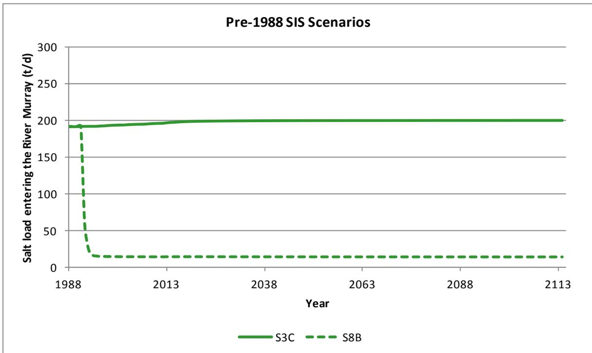
**Figure 5.2** Predicted total salt loads entering the River Murray from the Woolpunda Reach for Pre-1988 scenarios
