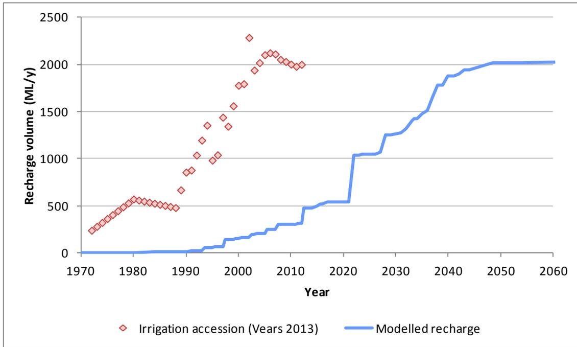
**Figure 4.15** Comparison between calculated accession estimates (Years 2013) and the calibrated modelled recharge volume for permanent irrigation
