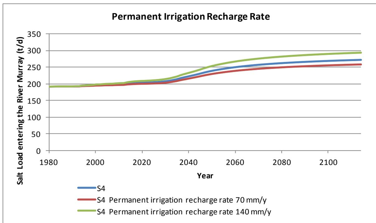
Figure 6.4 Uncertainty of permanent irrigation recharge rate in salt loads for the Woolpunda Reach
