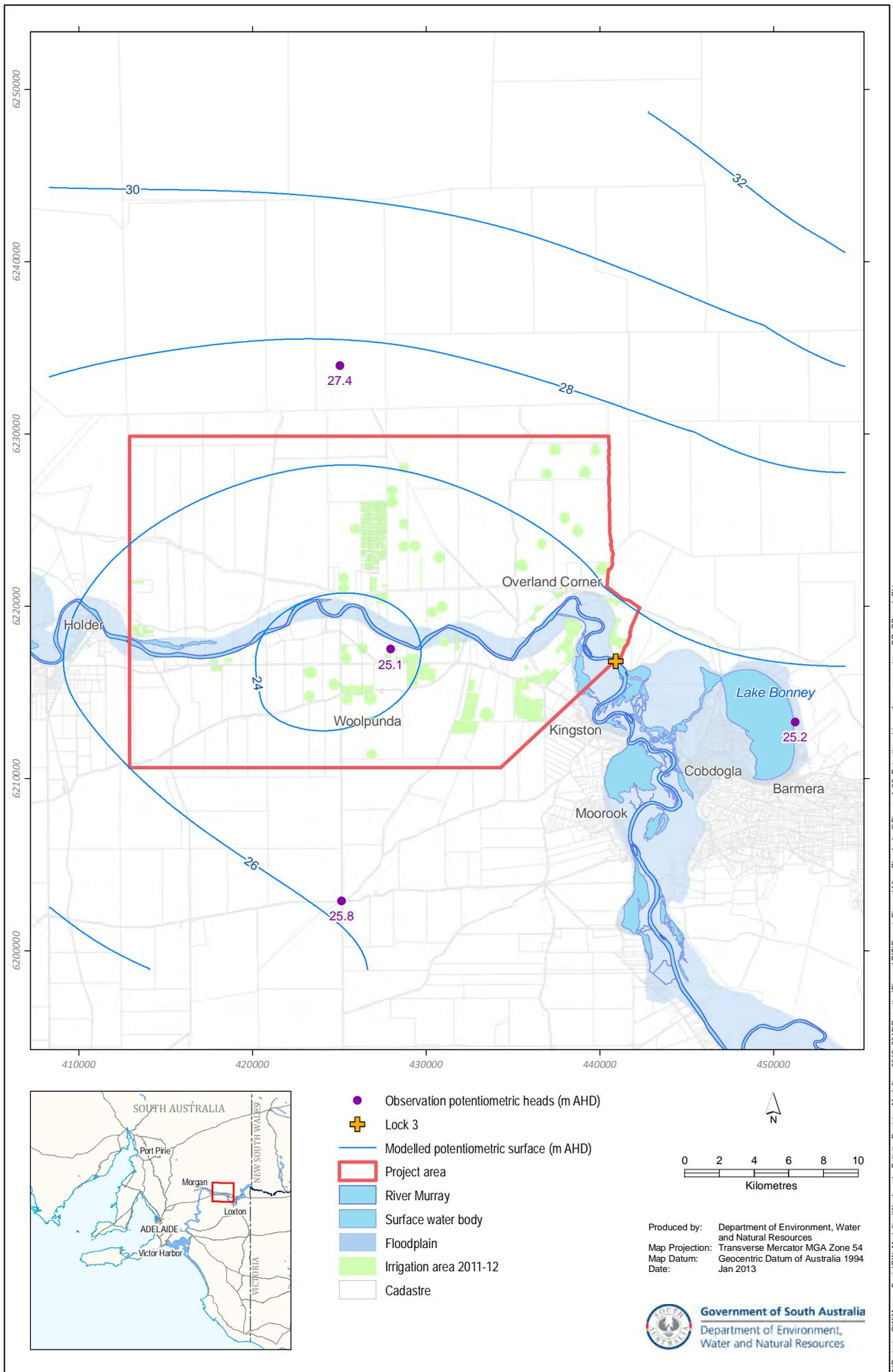
Figure 4.2. Comparison of observed and modelled potentiometric heads for model layer 4 (Renmark Group in steady-state conditions)
