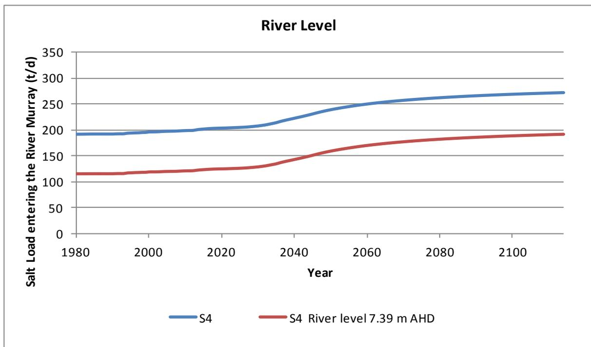
Figure 6.3 Uncertainty of river level in salt loads for the Woolpunda reach
