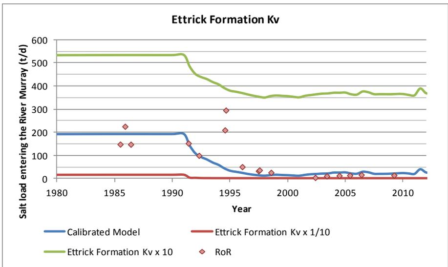
**Figure 6.2(a). Sensitivity of salt loads for the Woolpunda reach**
