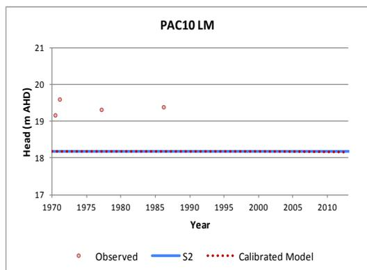
**Figure 6.7(a). Hydrographs near the north and south boundaries for Scenario 2 (Lower Mannum Formation)**
