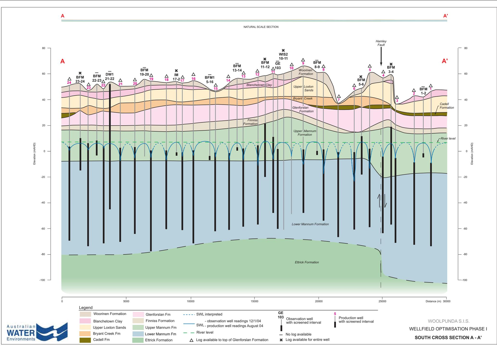
Figure 2.3. Cross-section through the southern wellfield of the Woolpunda SIS (AWE 2007a)
