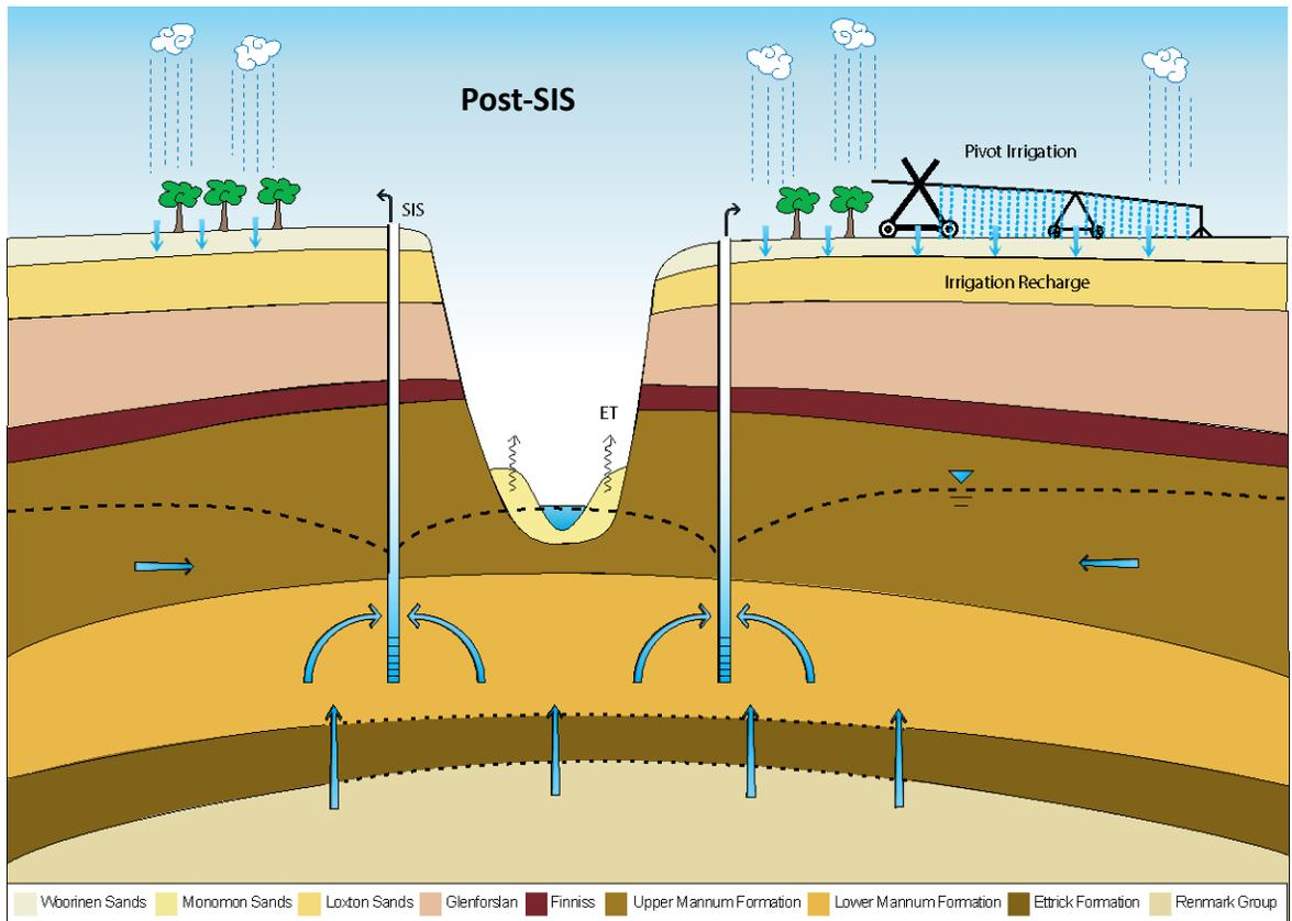
**Figure 2.17. Woolpunda hydrogeological conceptual model**
