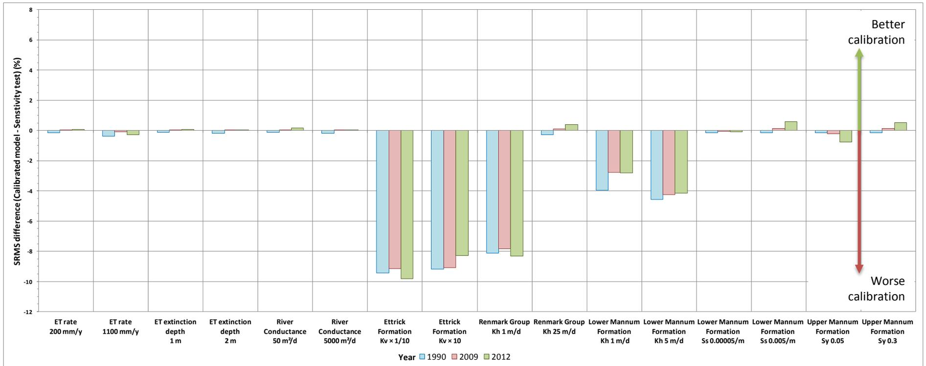
Figure 6.1. Sensitivity of calibration fit to observed heads (SRMS)
