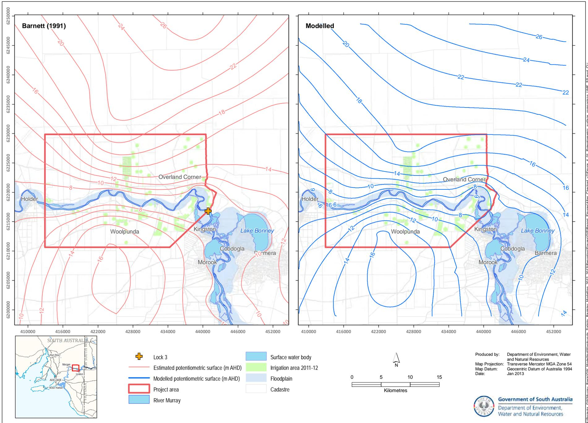
Figure 4.1. Comparison of estimated (Barnett 1991) and modelled potentiometric surface for model layer 1 (Upper Mannum Formation and Loxton Sands in steady-state conditions)
