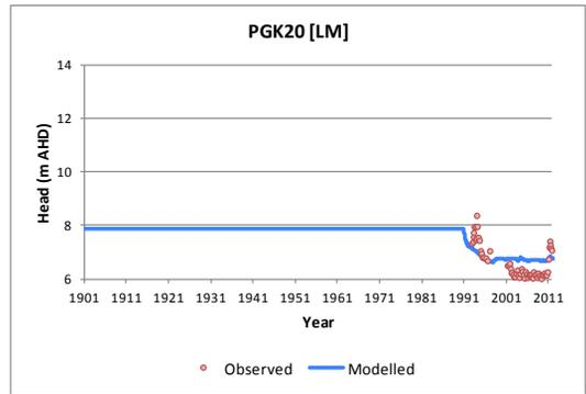
**Figure 4.5(i). Hydrograph comparison between observed and modelled for Woolpunda (Lower Mannum Formation)**
