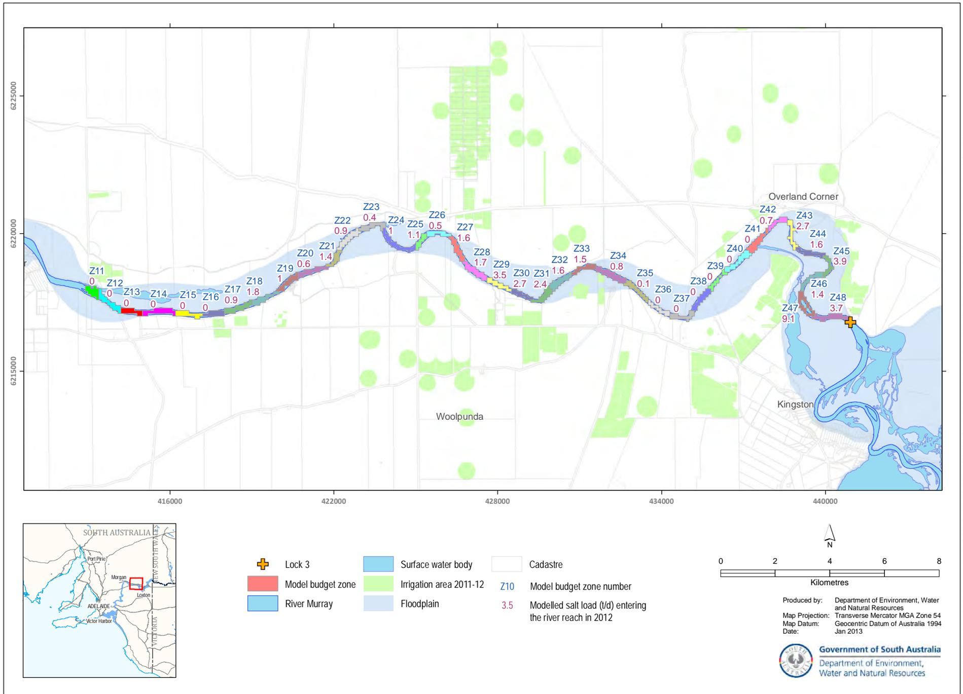
Figure 4.13. Modelled salt load spatial distribution at 2012
