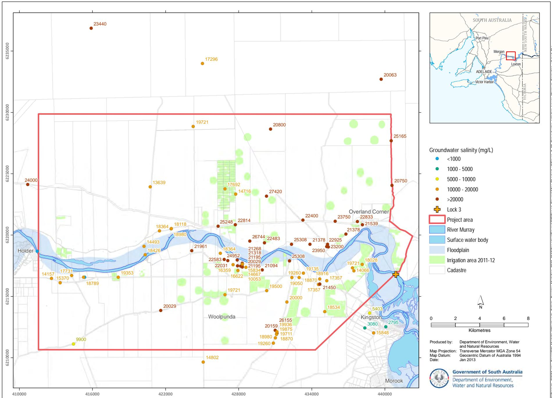
Figure 2.7. Groundwater salinities for the Lower Mannum Formation (After AWE 2013a)
