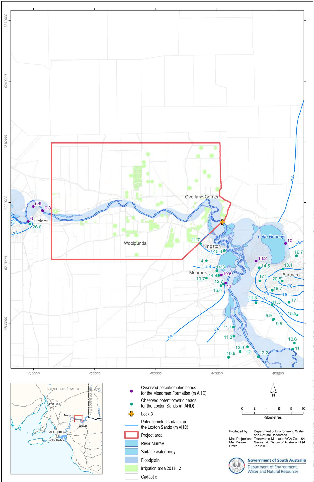
Figure 2.8. Potentiometric surface for the Loxton Sands and observed potentiometric heads for the Monoman Formation 2009 (After AWE 2013a)
