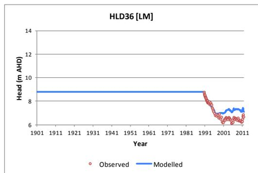
**Figure 4.5(b). Hydrograph comparison between observed and modelled for Woolpunda (Lower Mannum Formation)**
