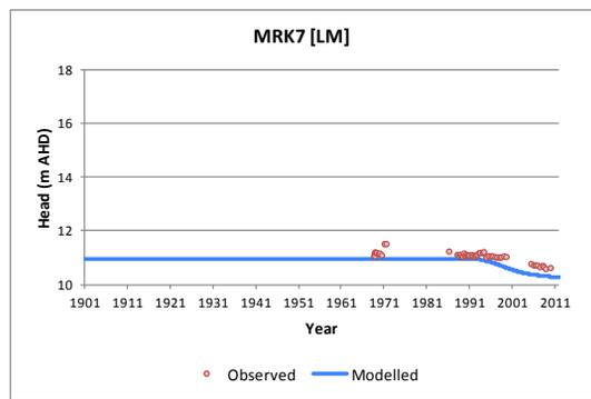
**Figure 4.5(c). Hydrograph comparison between observed and modelled for Woolpunda (Lower Mannum Formation)**
