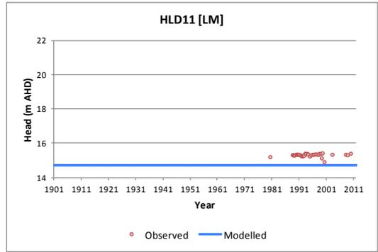
**Figure 4.5(a). Hydrograph comparison between observed and modelled for Woolpunda (Lower Mannum Formation)**
