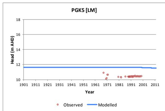
**Figure 4.5(h). Hydrograph comparison between observed and modelled for Woolpunda (Lower Mannum Formation)**
