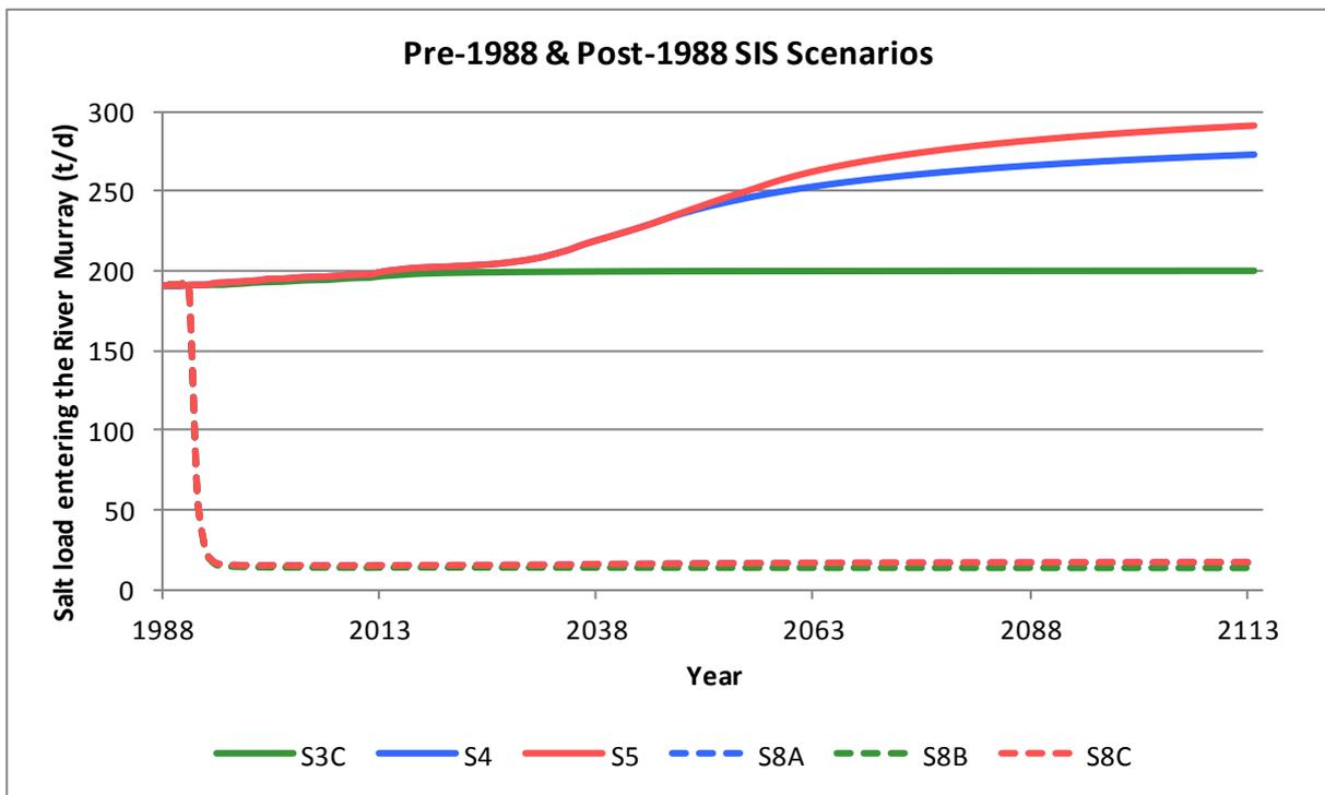
Figure 5.3 Predicted total salt loads entering the River Murray from the Woolpunda Reach for Pre-1988 and Post-1988 scenarios
