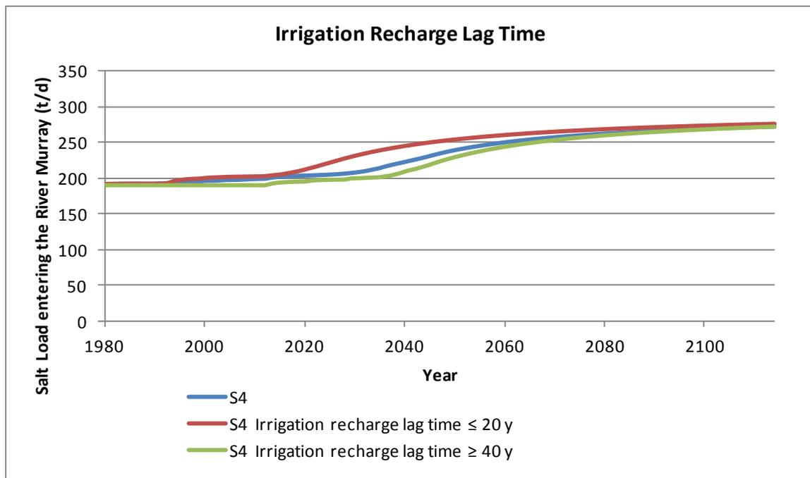
Figure 6.6 Uncertainty of irrigation recharge lag time in salt loads for the Woolpunda Reach
