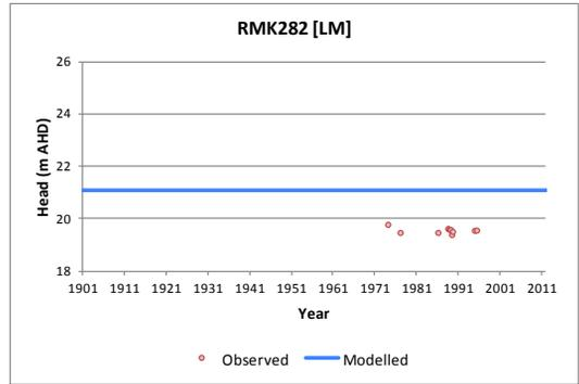
**Figure 4.5(k). Hydrograph comparison between observed and modelled for Woolpunda (Lower Mannum Formation)**
