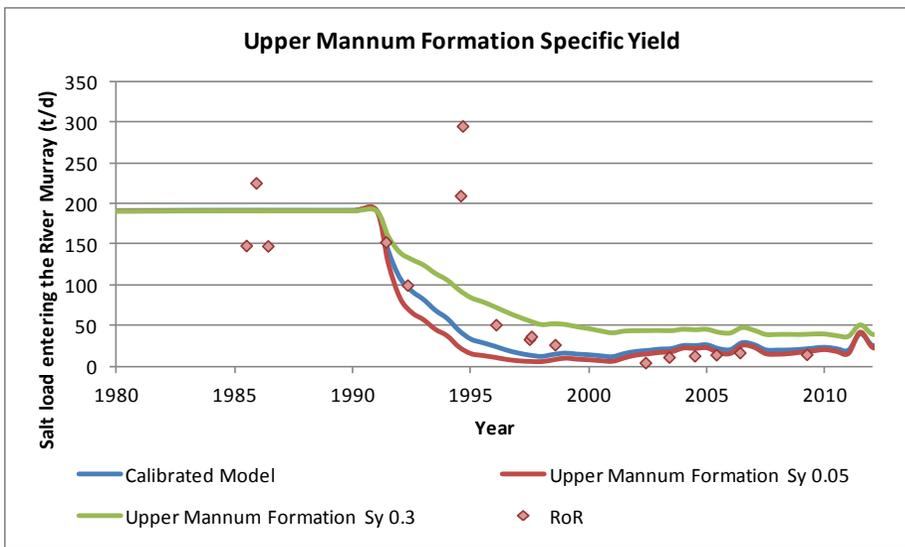
Figure 6.2(b). Sensitivity of salt loads for the Woolpunda reach
