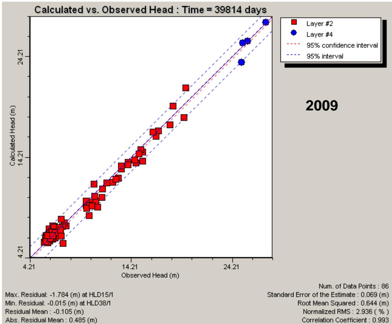
**Figure 4.9. Scaled Root Mean Square (SRMS) at 2009**
