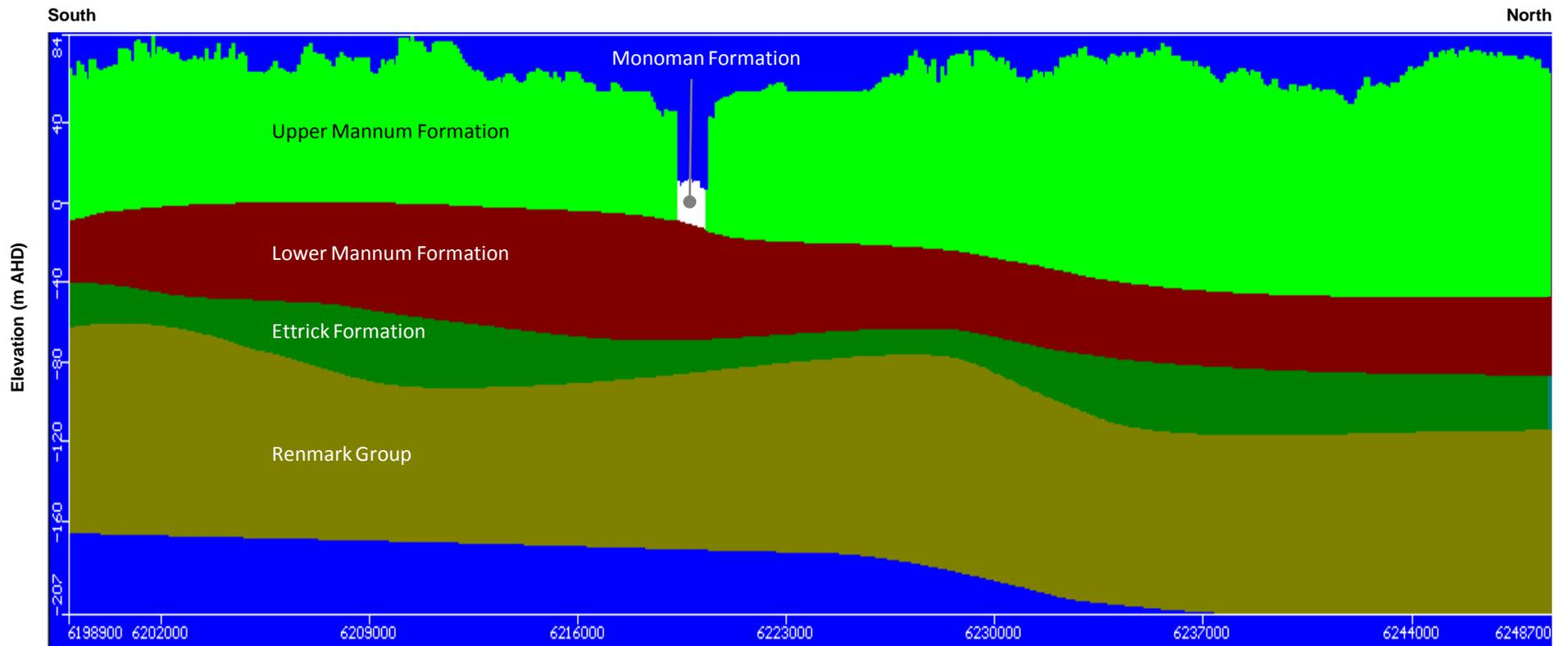
Figure 3.3. Model layers (north-south cross-section through model column 155, E423750)
