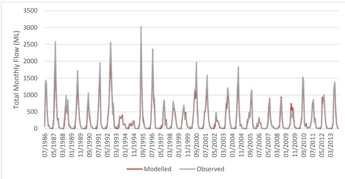
Figure 8. Calibration results for site A5030502 – Scott Creek
