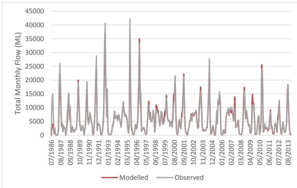
Figure 10. Calibration results for site A5030504 – Houlgraves Weir
