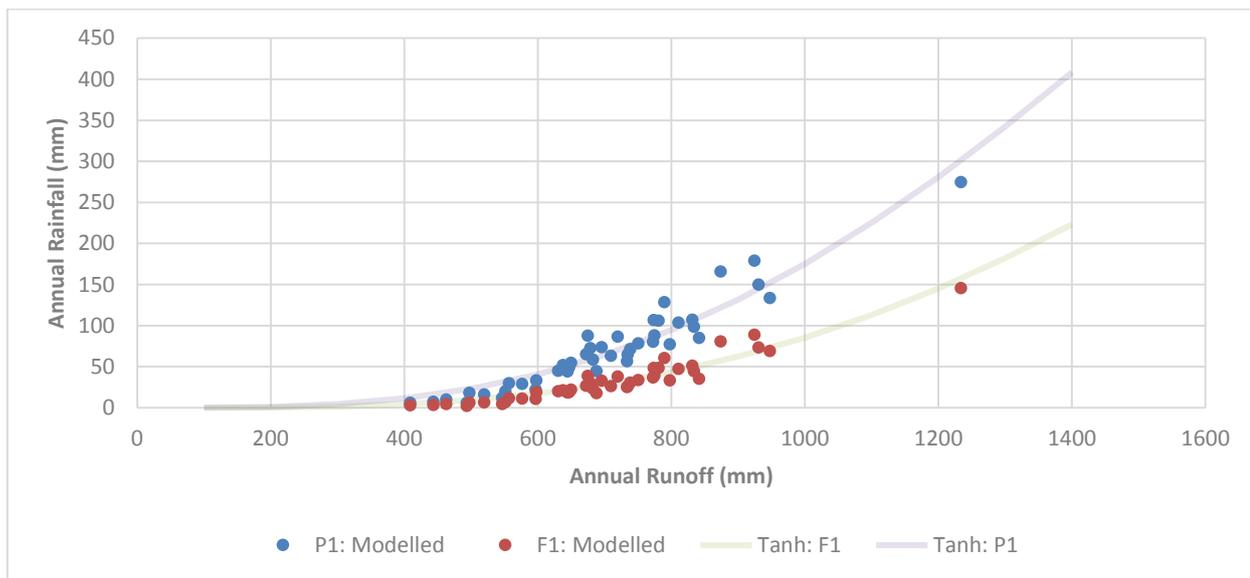
**Figure 15. Rainfall-runoff curves for functional units pasture (P1) and forested (F1) for sub-catchment #3478**
