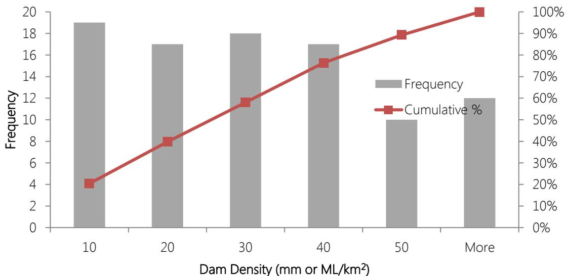
**Figure 4. Histogram showing distribution of dam density by modelled sub-catchment**
