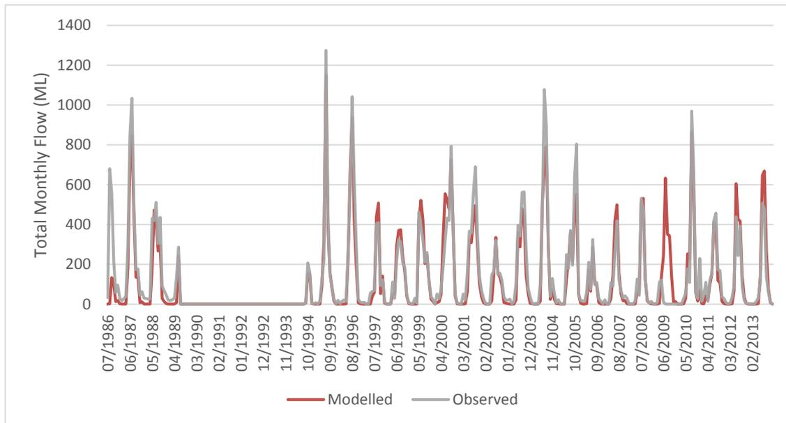
Figure 14. Calibration results for site A4261001 Onkaparinga River upstream of Hahndorf dissipator
