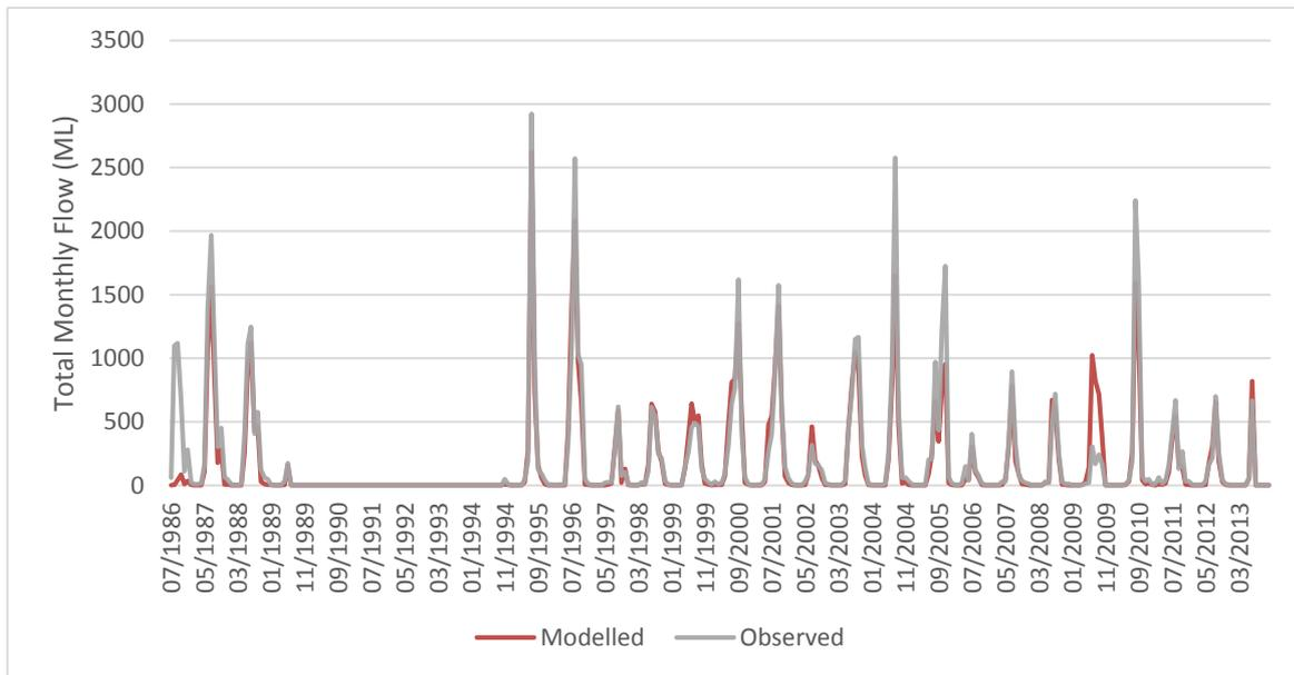
Figure 12. Calibration results for site A5030507 – Aldgate Creek
