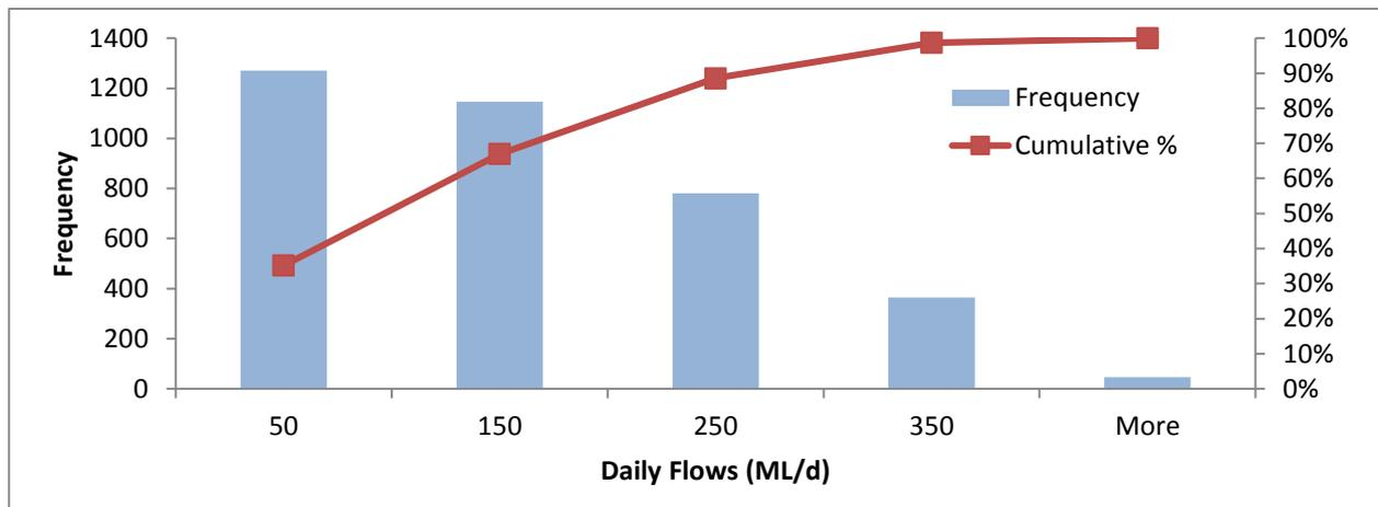
**Figure 6. Distribution of gauged daily flows during the dry season, used to derive additional inflows**
