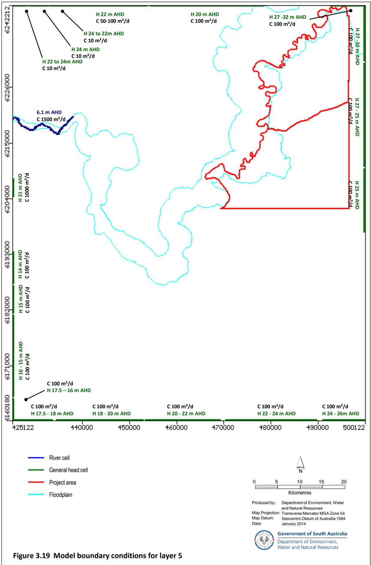
Figure 3.19 Model boundary conditions for layer 5
