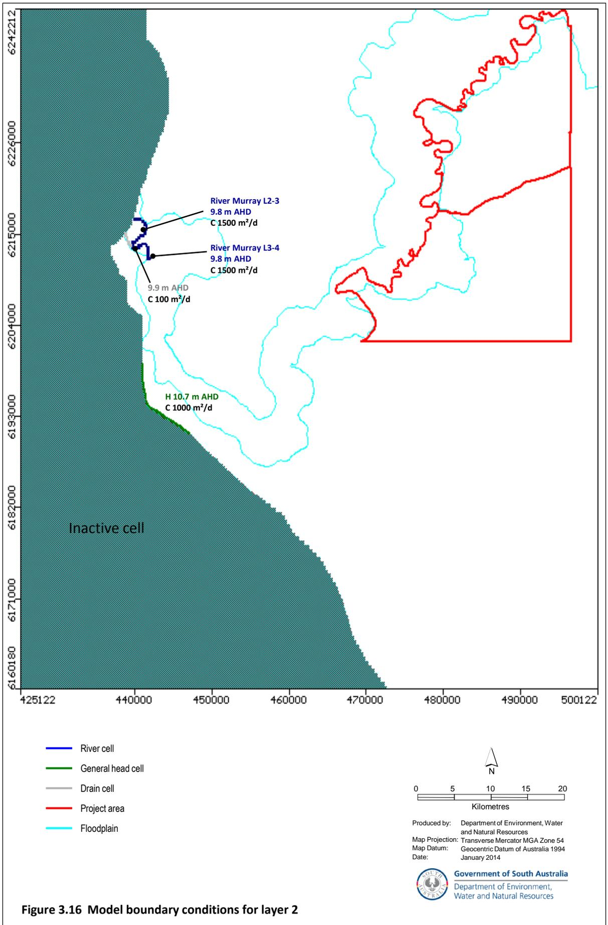
**Figure 3.16 Model boundary conditions for layer 2**
