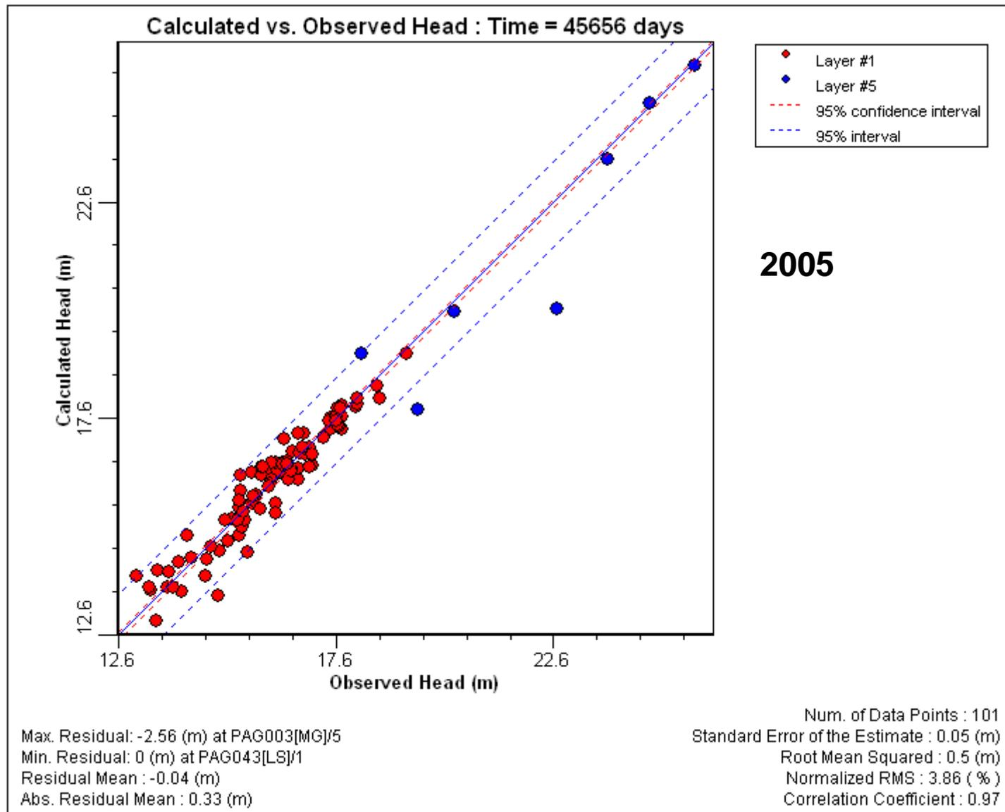
**Figure 4.12. Scaled Root Mean Square (SRMS) at 2005**
