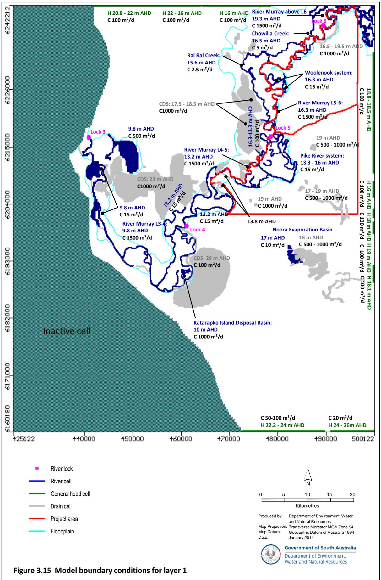
Figure 3.15 Model boundary conditions for layer 1
