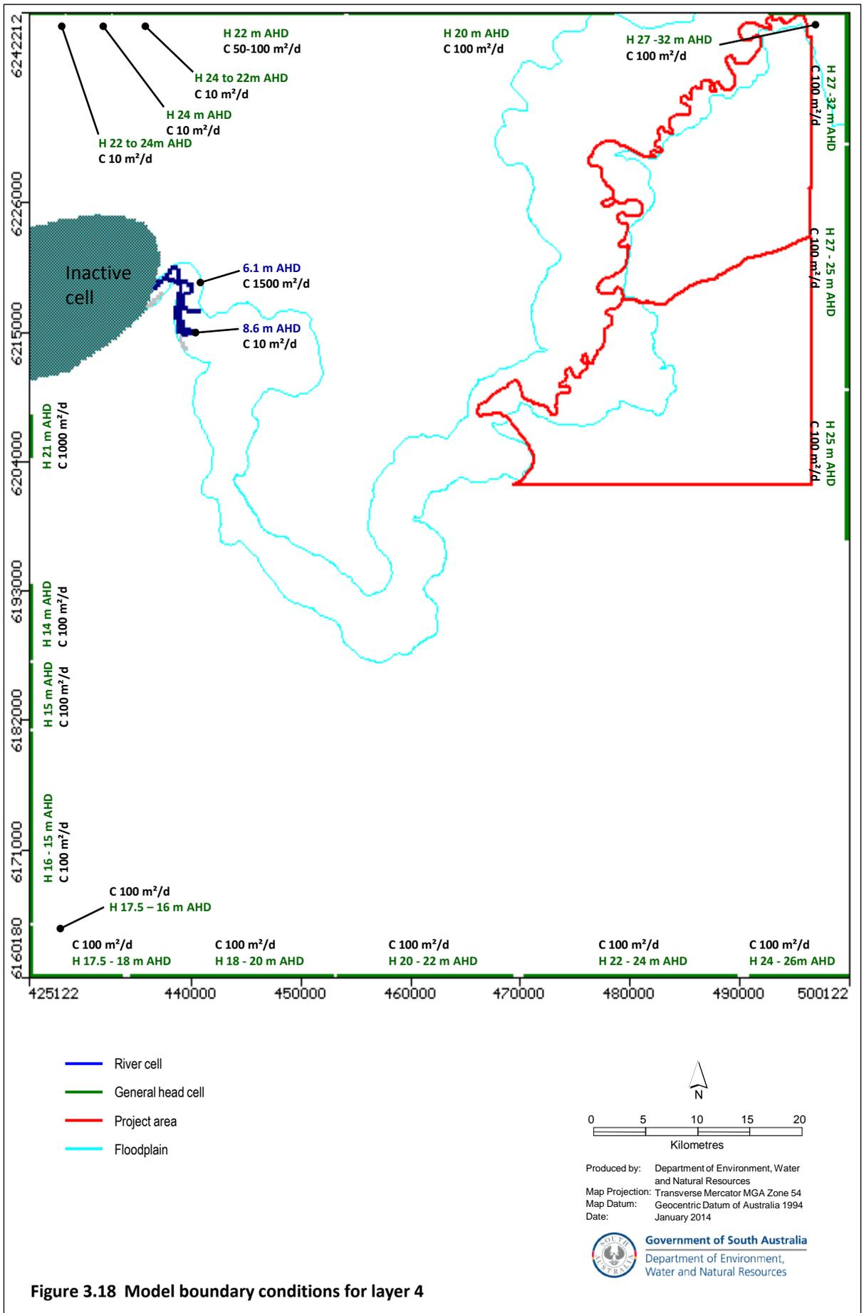
Figure 3.18 Model boundary conditions for layer 4
