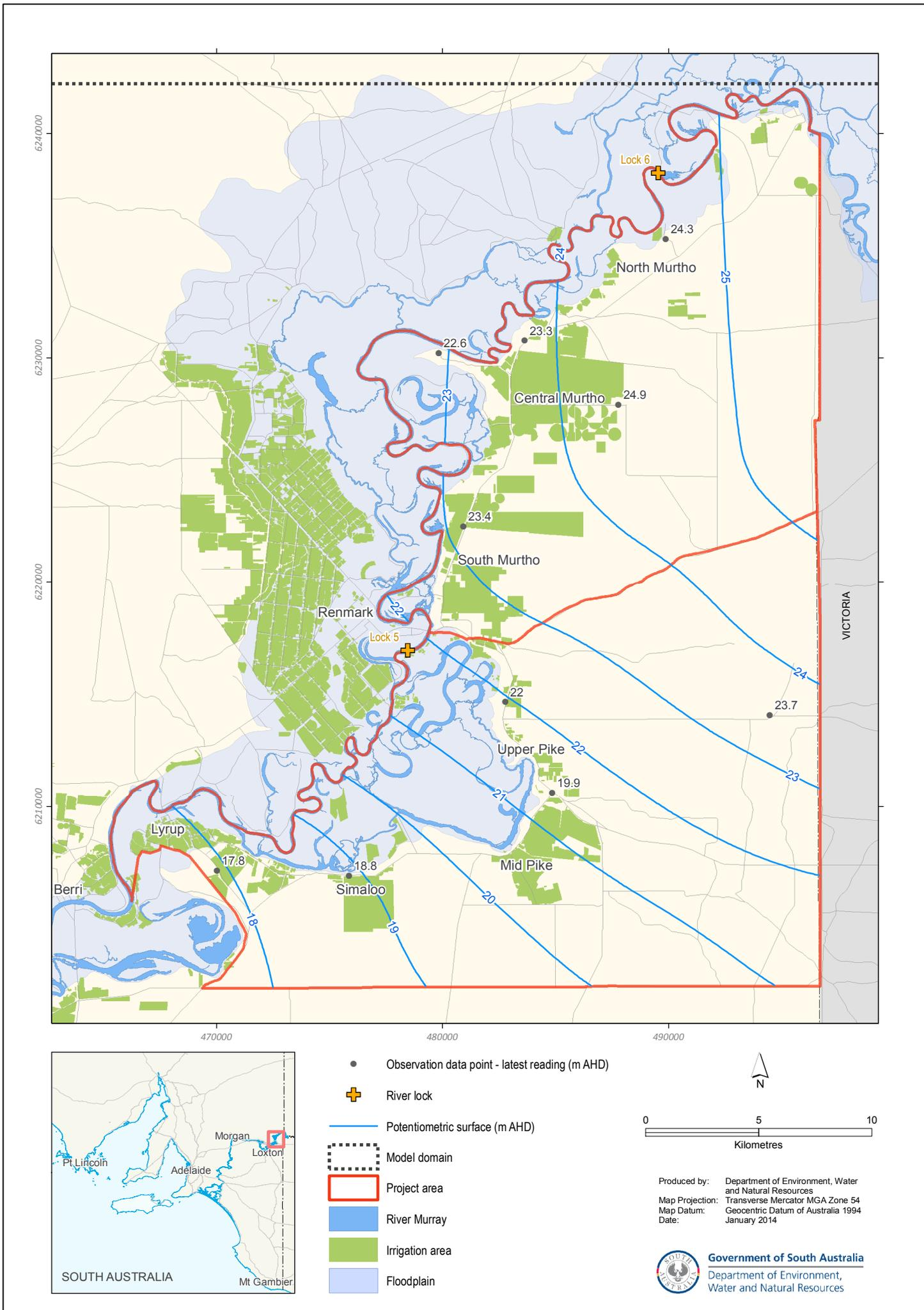
Figure 2.4. Potentiometric surface for the Murray Group Limestone
