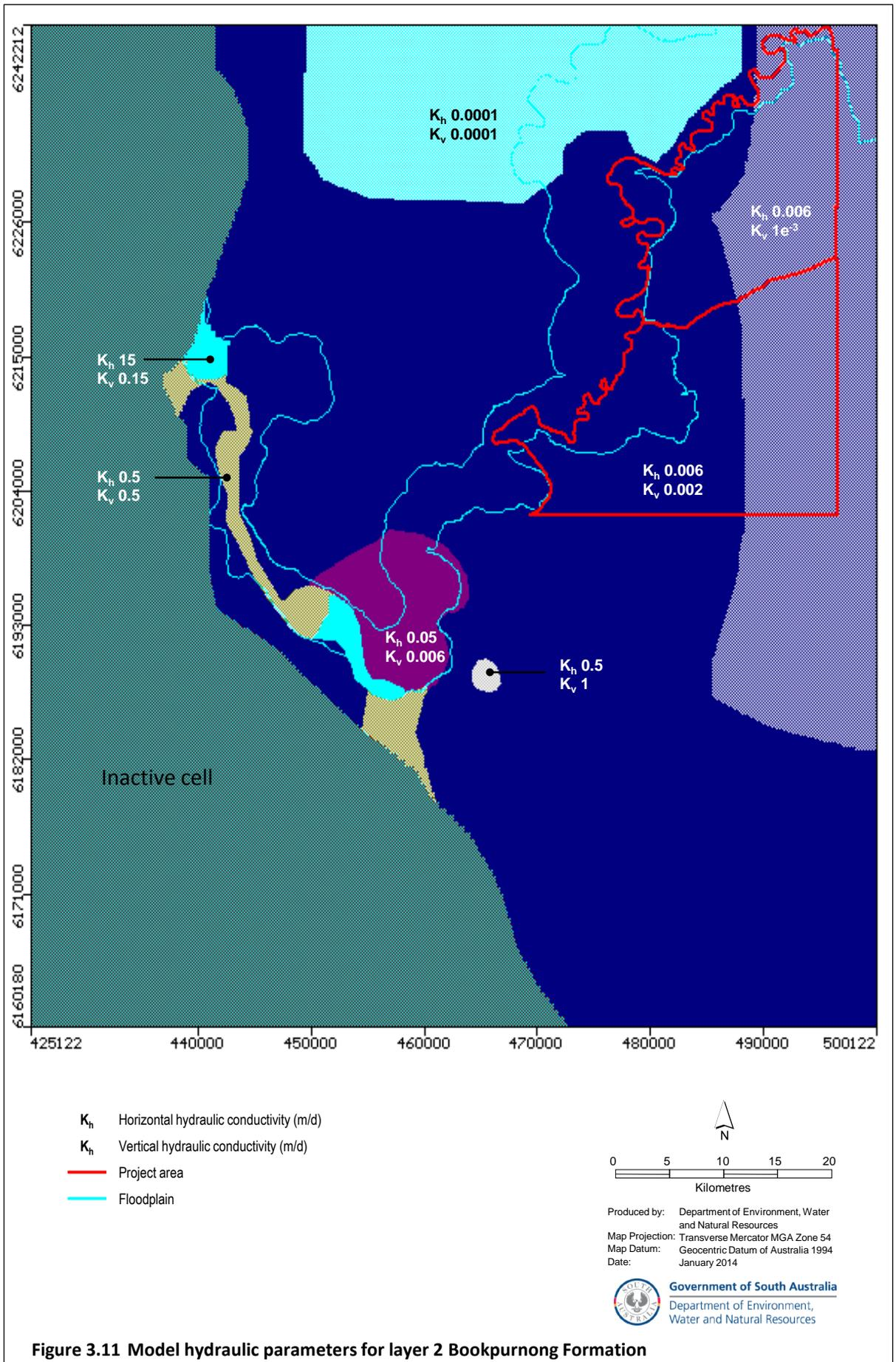
**Figure 3.11 Model hydraulic parameters for layer 2 Bookpurnong Formation**
