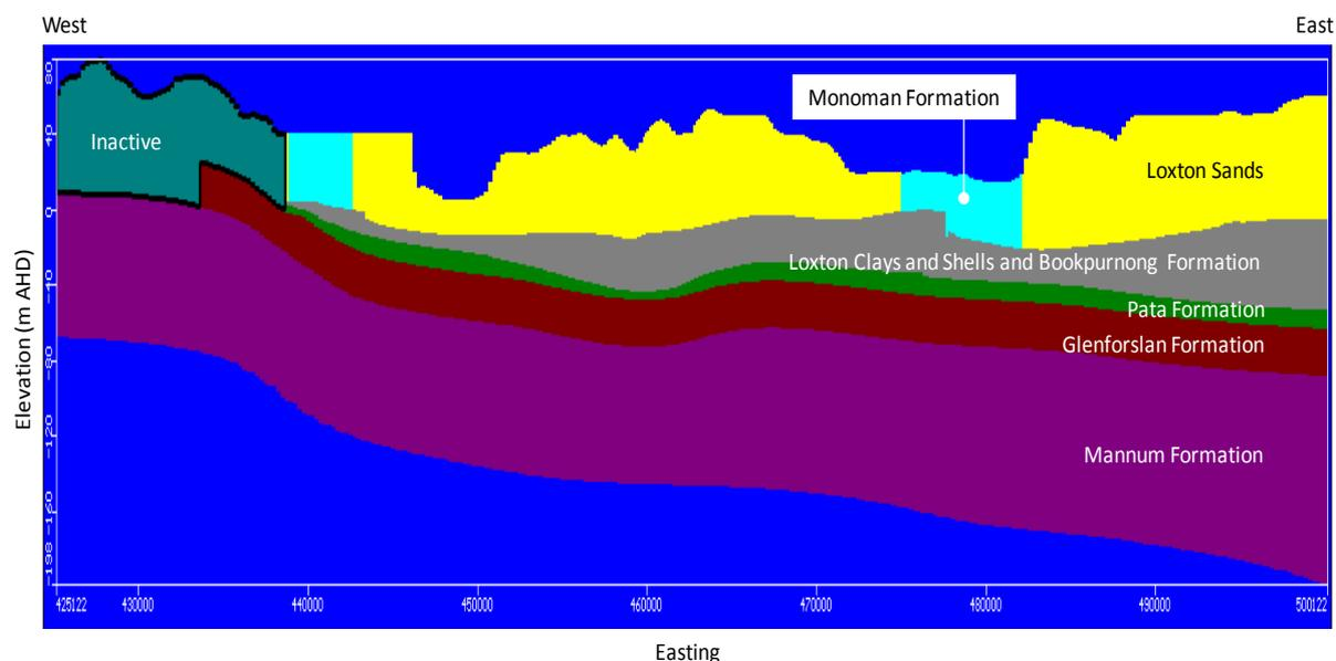
Figure 3.3 Model layers (east-west cross-section through model row 217, N6215000)
