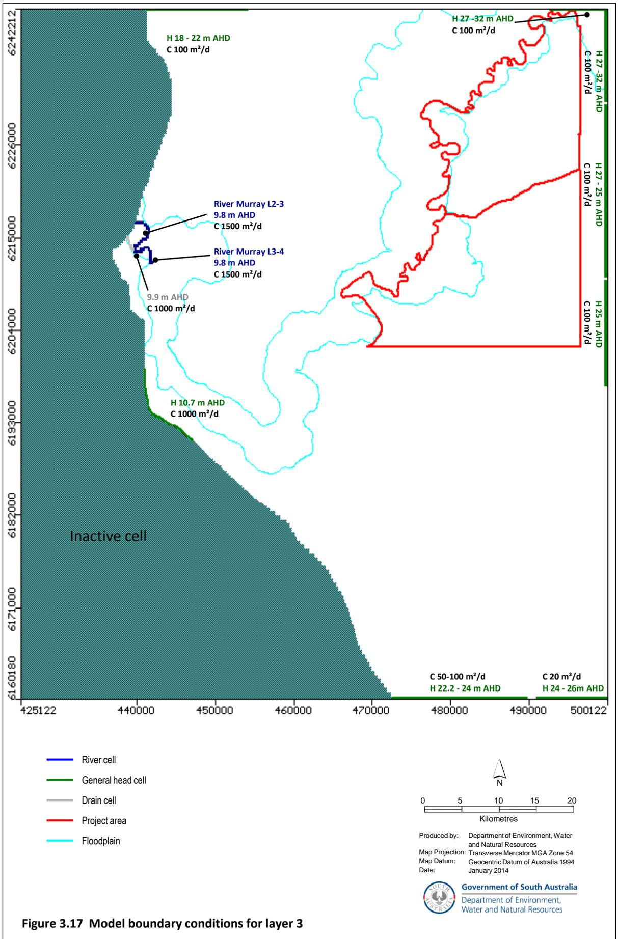
Figure 3.17 Model boundary conditions for layer 3
