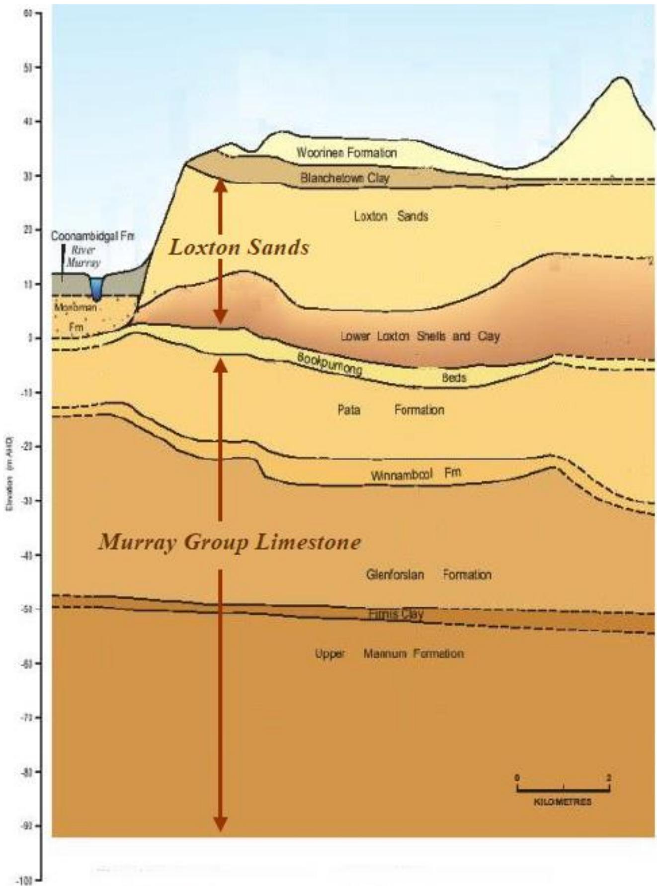
Figure 3 Hydrogeological cross-section of the Riverland environment (Yan et al, 2005a)
