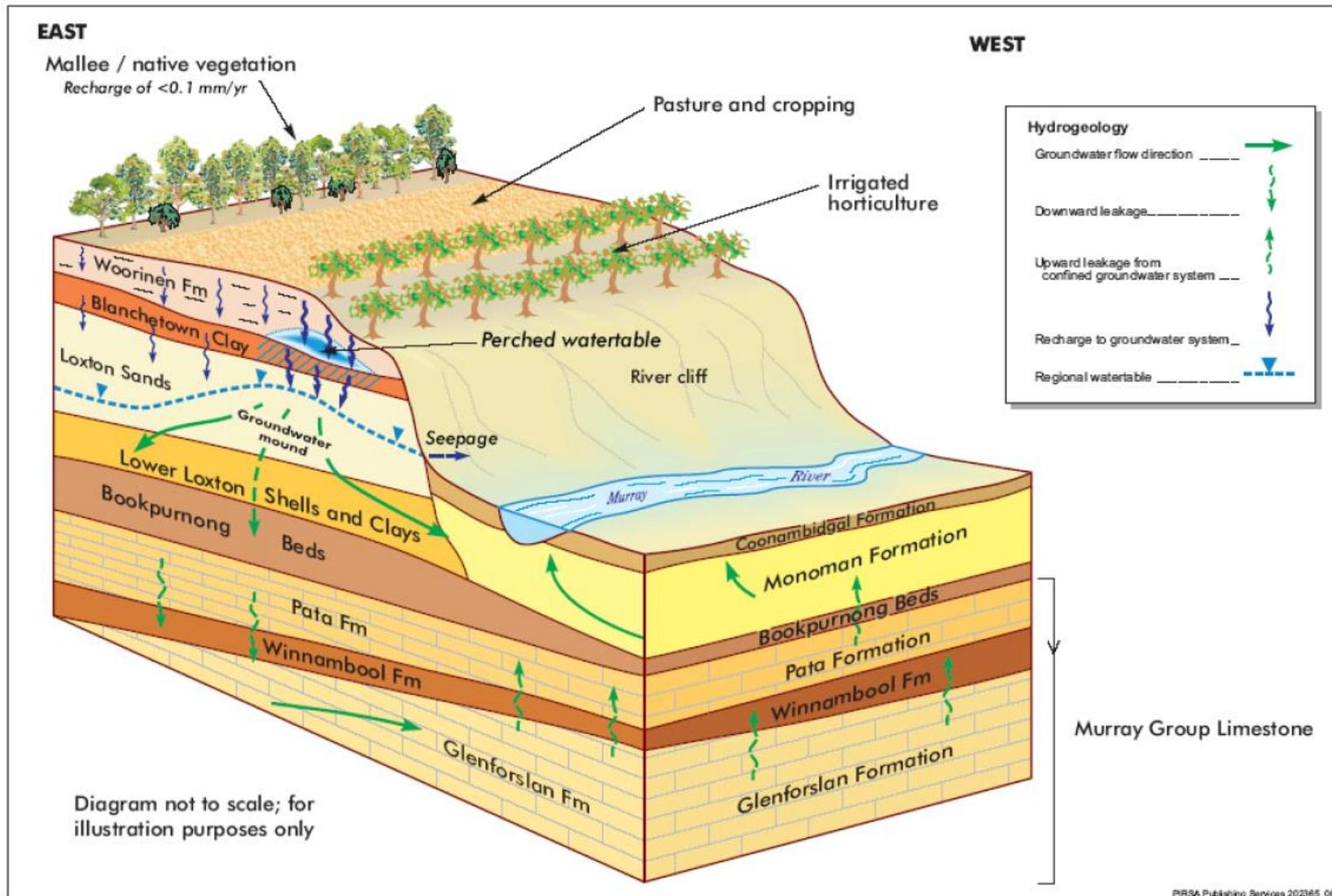
Figure 4 Hydrogeological conceptual processes of the Riverland environment (Yan et al, 2005a)
