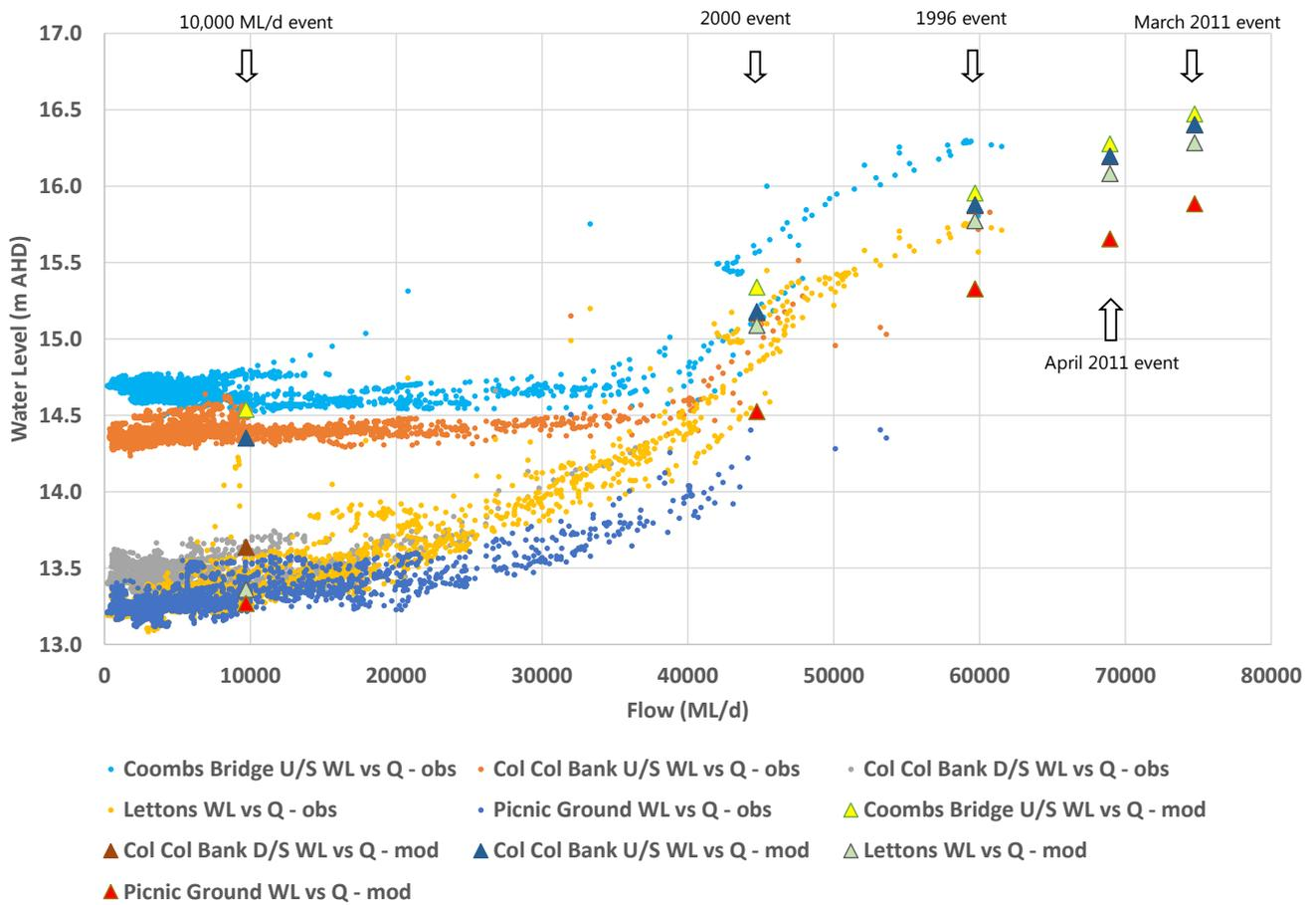
**Figure 2.5 Comparison of Pike Floodplain water levels with Lock 5 flow – historical record and modelled events**
