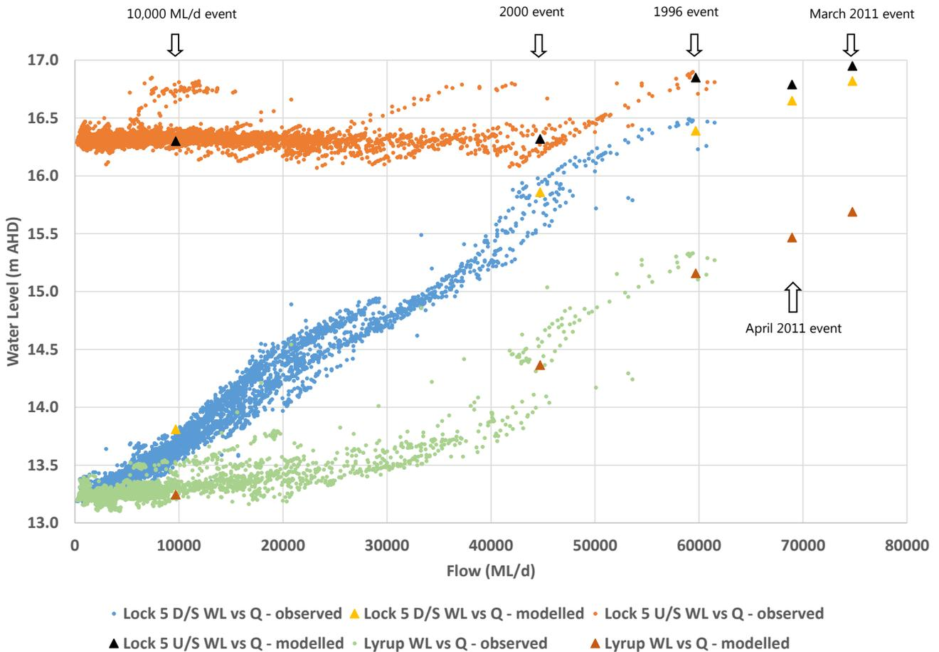
**Figure 2.4 Comparison of River Murray water levels with Lock 5 flow – historical record and modelled events**
