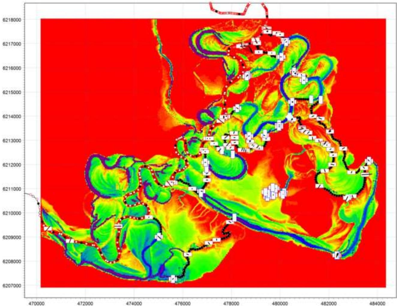
**Figure 2.1 MIKE FLOOD 1-D/2-D coupled model of Pike Floodplain**
